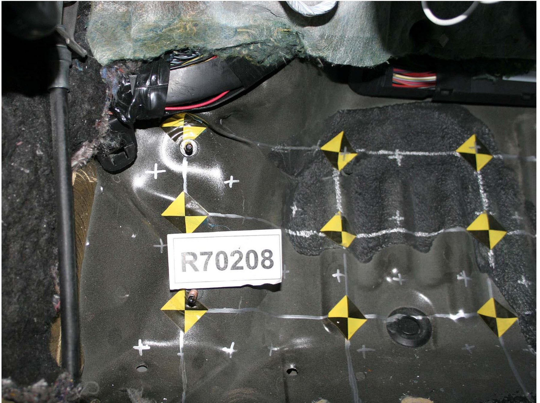
Figure A-302: Test Vehicle Post-Test Foot Rest, Sill Height
