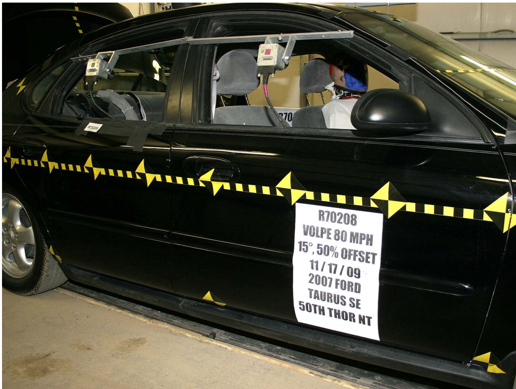
Figure A-33: Test Vehicle Pre-Test Front \frac{3}{4} View of Right Side Doors
