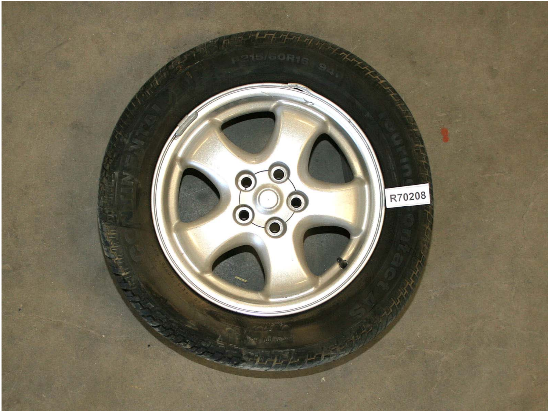
Figure A-130: Test Vehicle Post-Test Right Front Wheel Damage (Outside)
