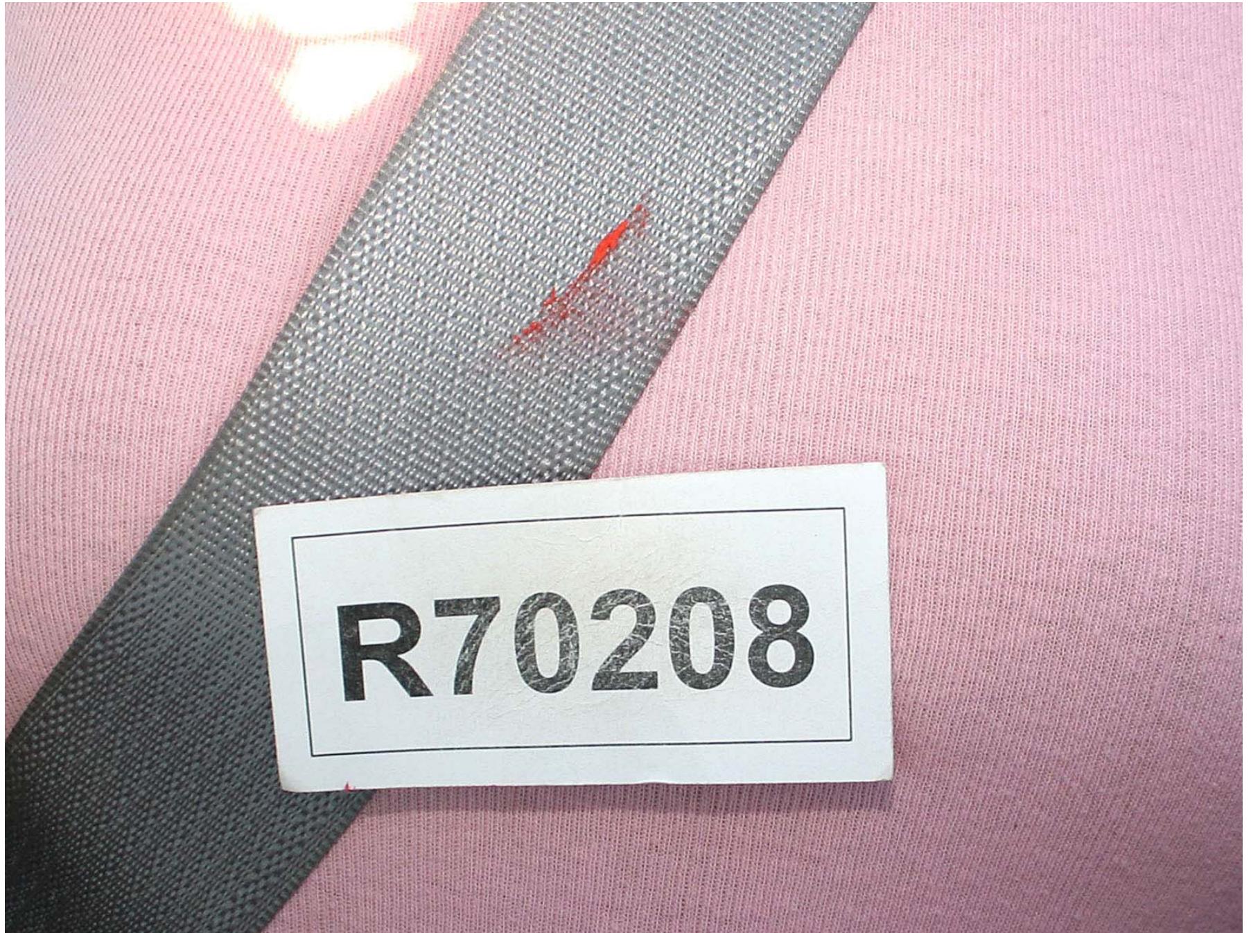
Figure A-276: Test Vehicle Post-Test Passenger Dummy Contact, Chest
