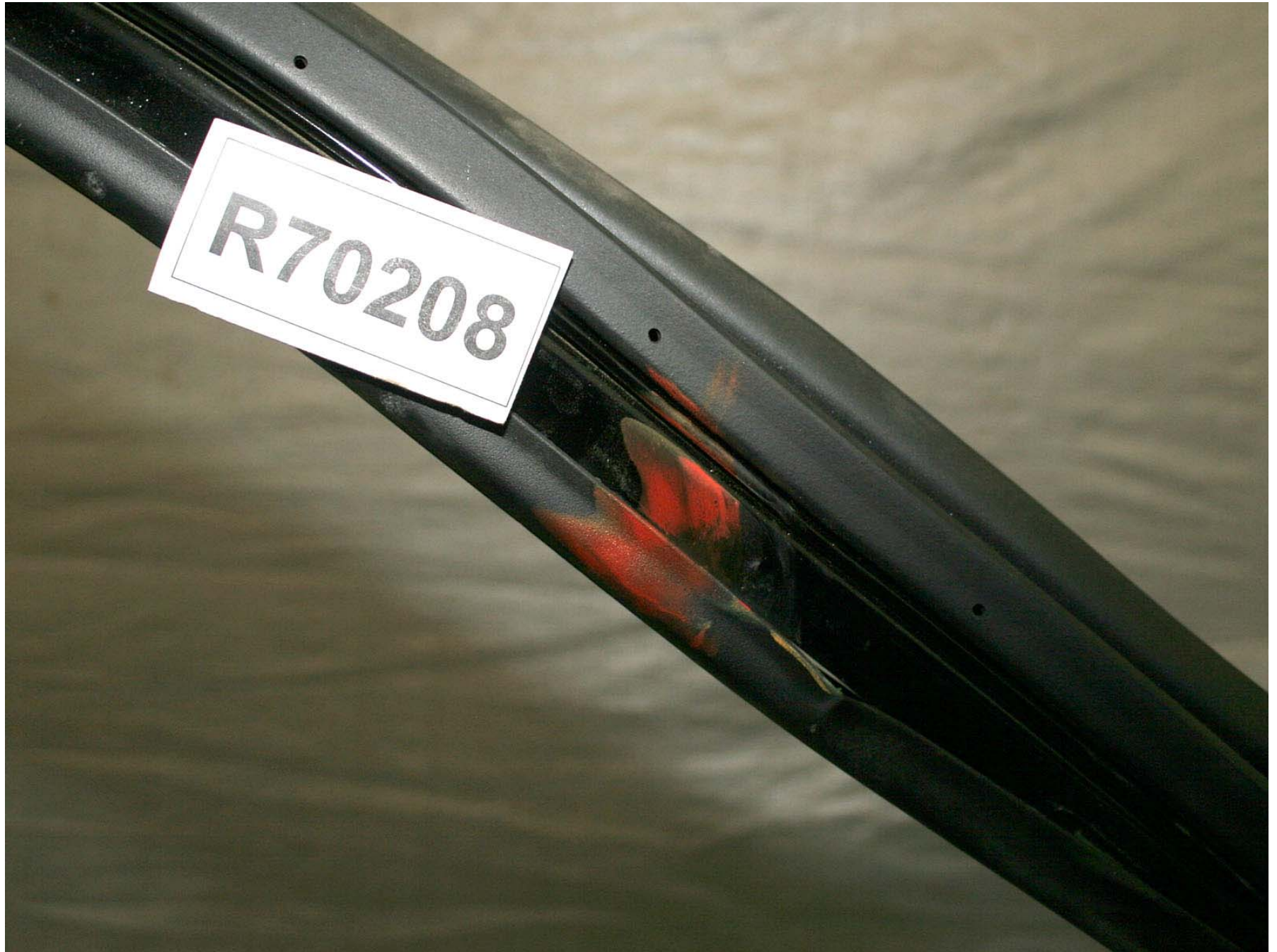
Figure A-251: Test Vehicle Post-Test Driver Dummy Contact, Door Frame
