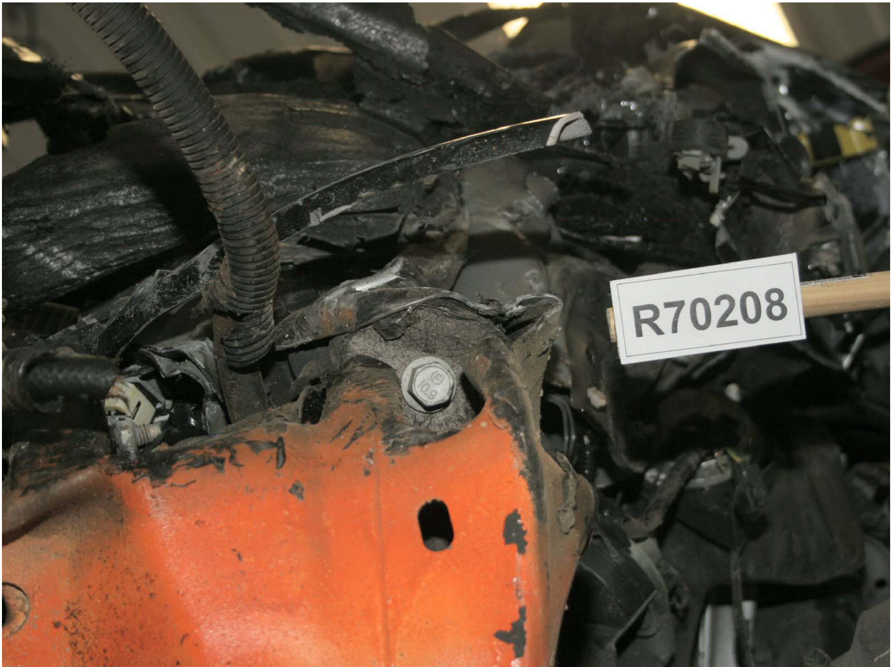
Figure A-165: Test Vehicle Post-Test Left Front Sub-Frame Mounting Point
