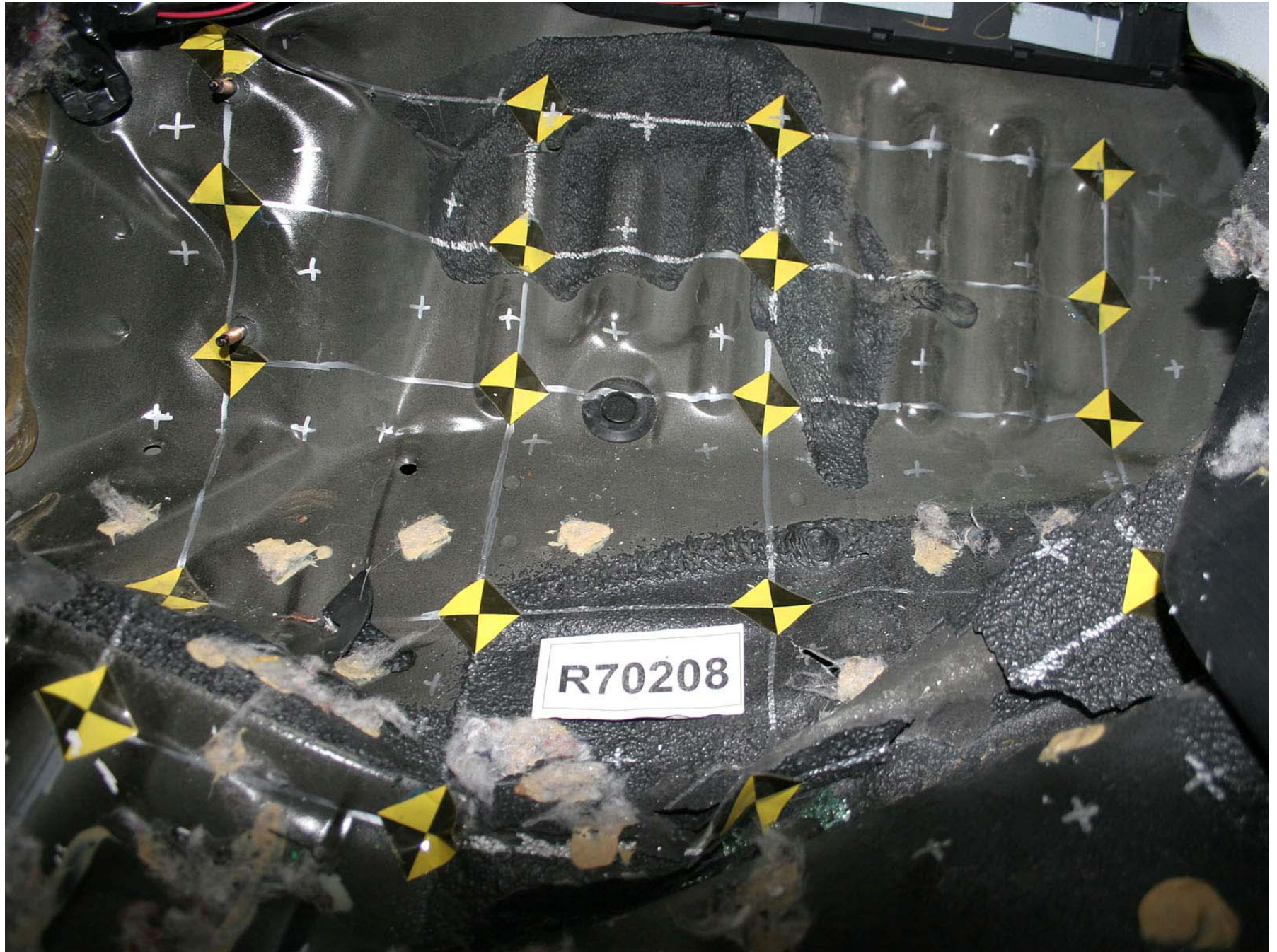
Figure A-288: Test Vehicle Post-Test Driver Floorpan, Sill Height
