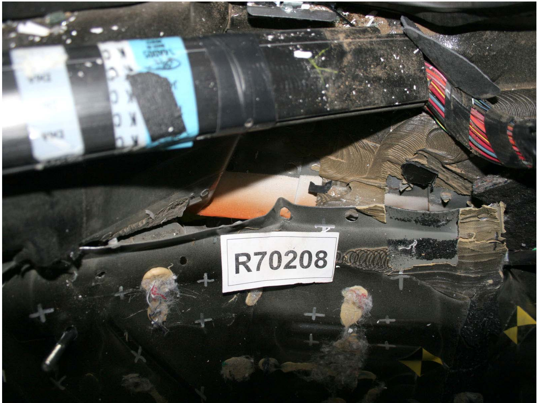
Figure A-314: Test Vehicle Post-Test Driver Side Floorpan Close Up
