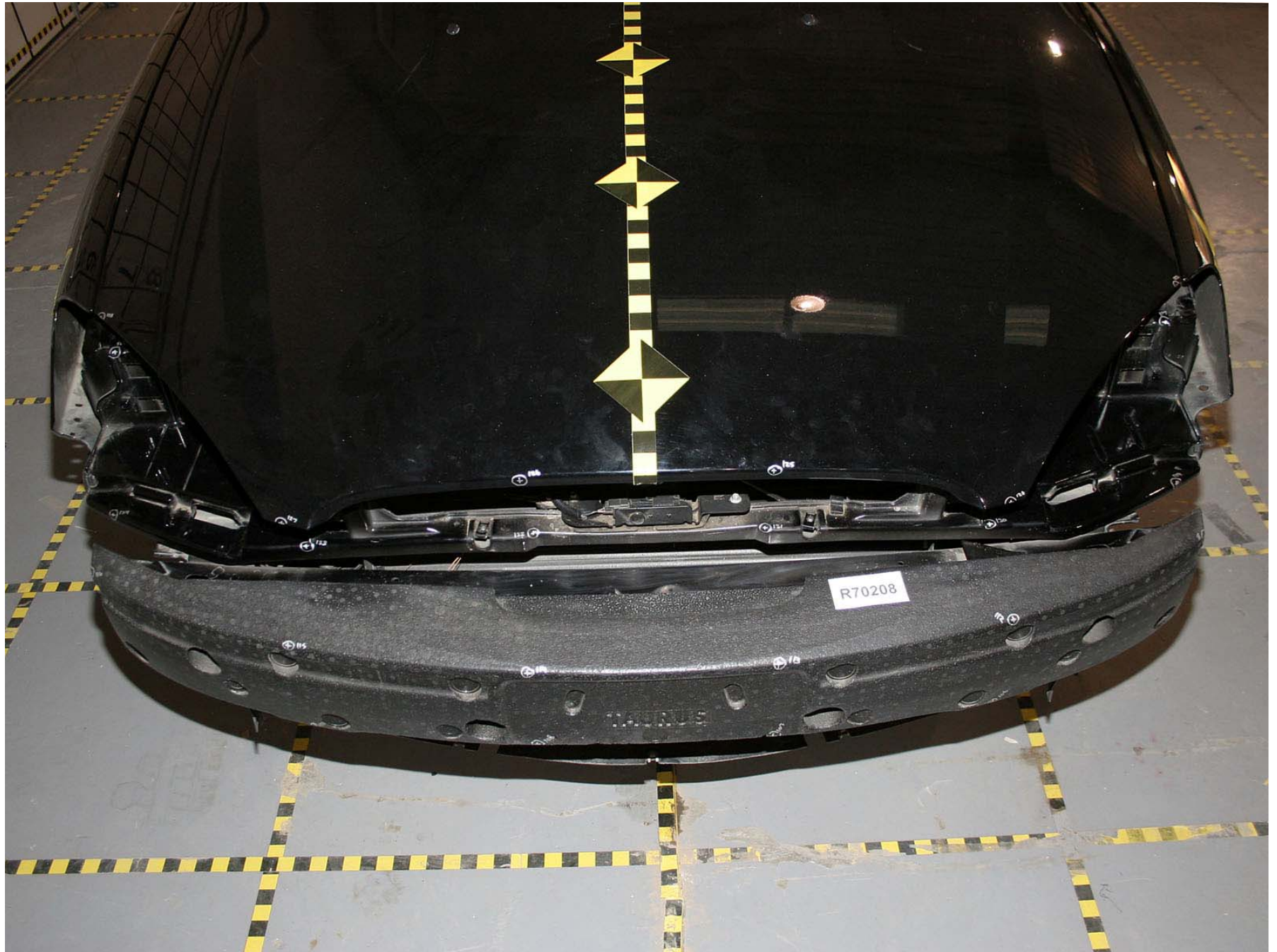
Figure A-303: Test Vehicle Pre-Test Structural Member Crush Measurement (Hood Closed)
