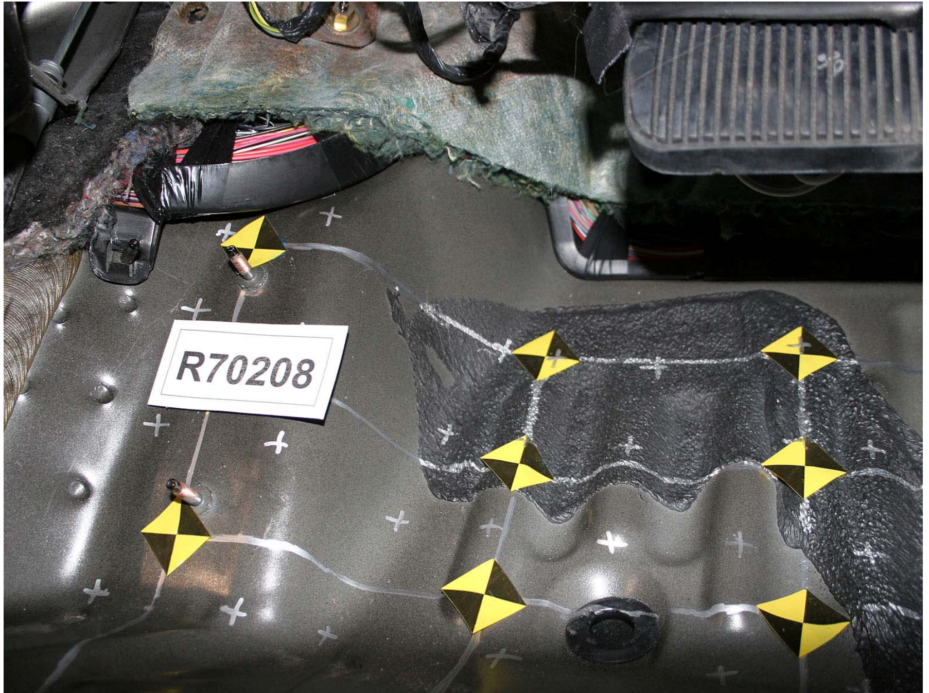
Figure A-301: Test Vehicle Pre-Test Foot Rest, Sill Height
