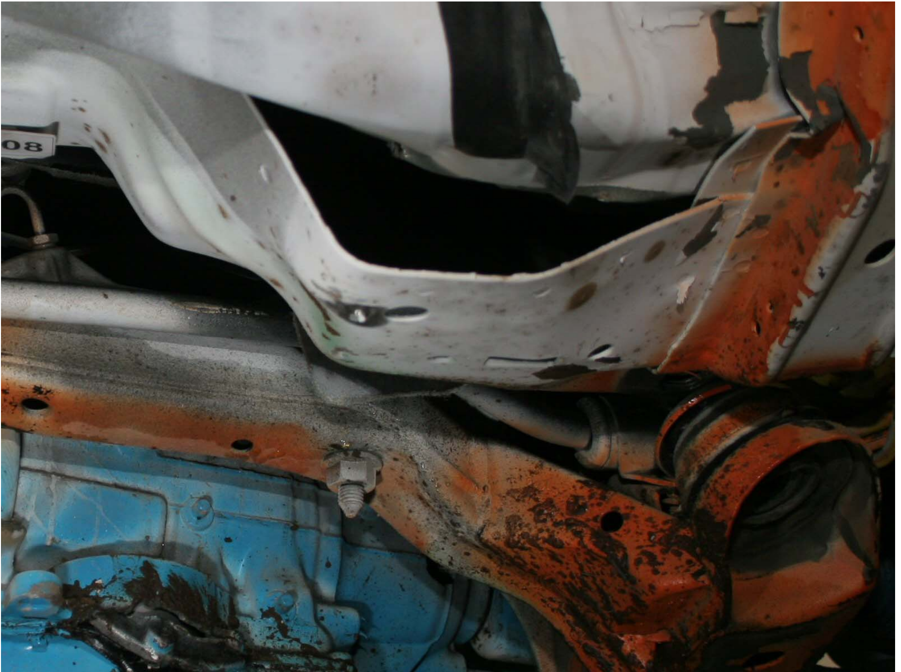
Figure A-219: Test Vehicle Post-Test Sway Bar Right Side Mounting Bolts
