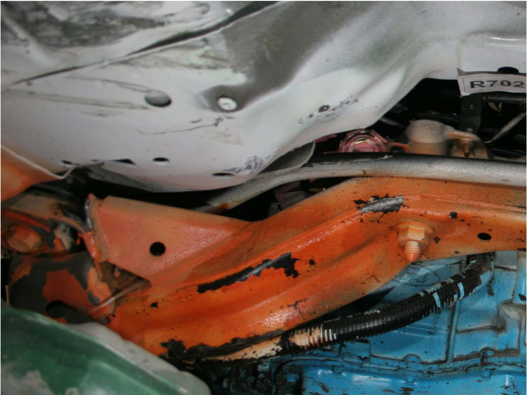
Figure A-217: Test Vehicle Post-Test Sway Bar Left Side Mounting Bolts
