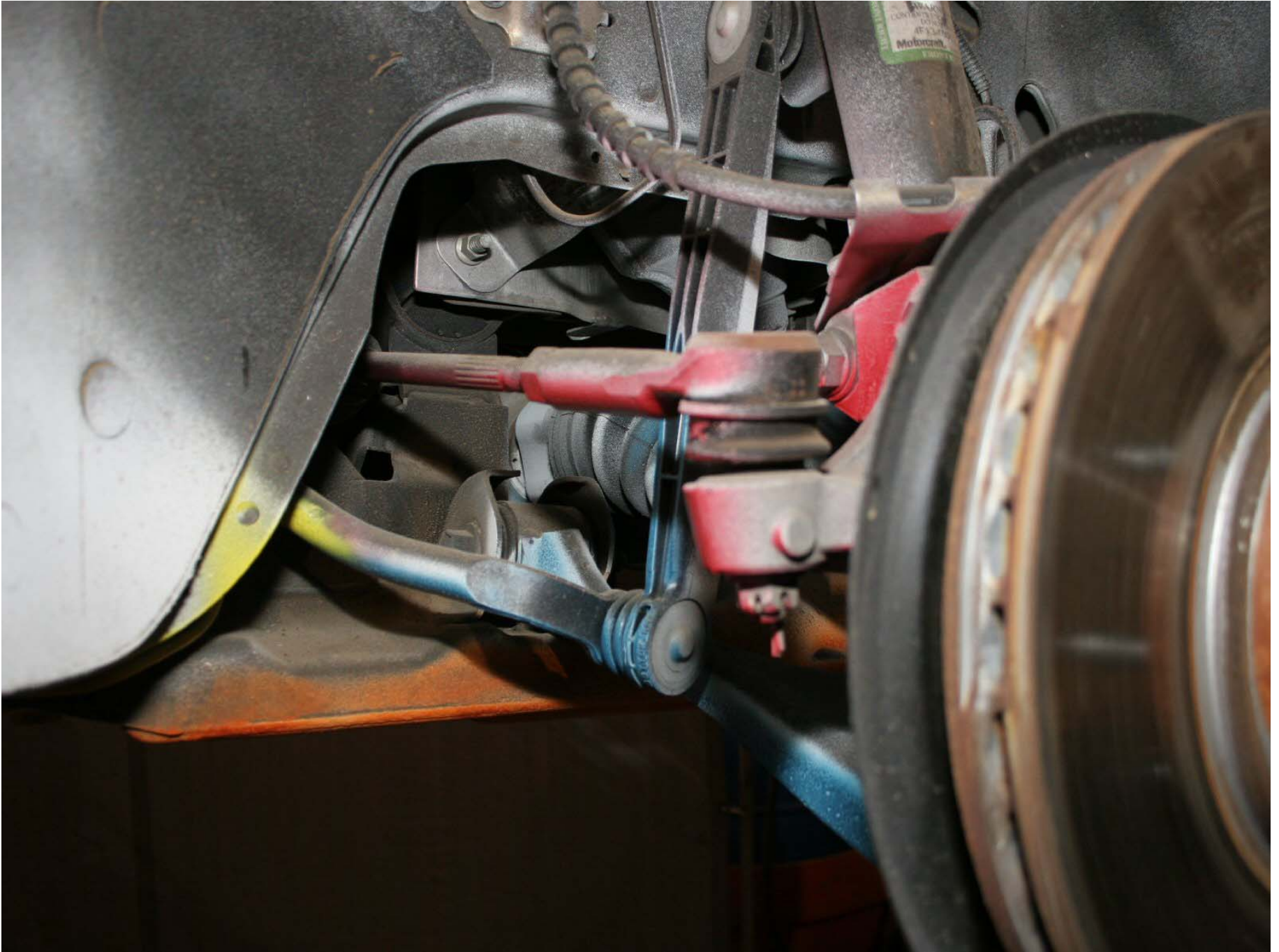
Figure A-190: Test Vehicle Pre-Test Right Side Tie Rod and Sway Bar Attachments Points
