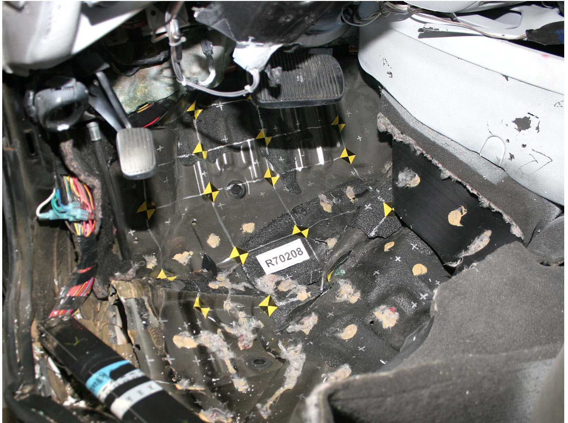
Figure A-280: Test Vehicle Pre-Test Driver Floorpan Left \frac{3}{4} View, Seat Cushion Height
