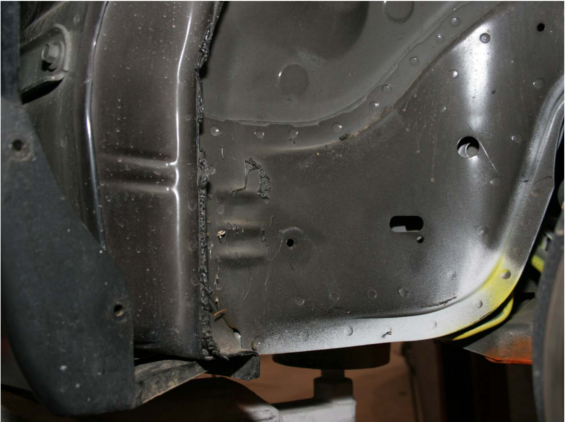
Figure A-188: Test Vehicle Pre-Test Right Side Frame to A-Pillar Joint
