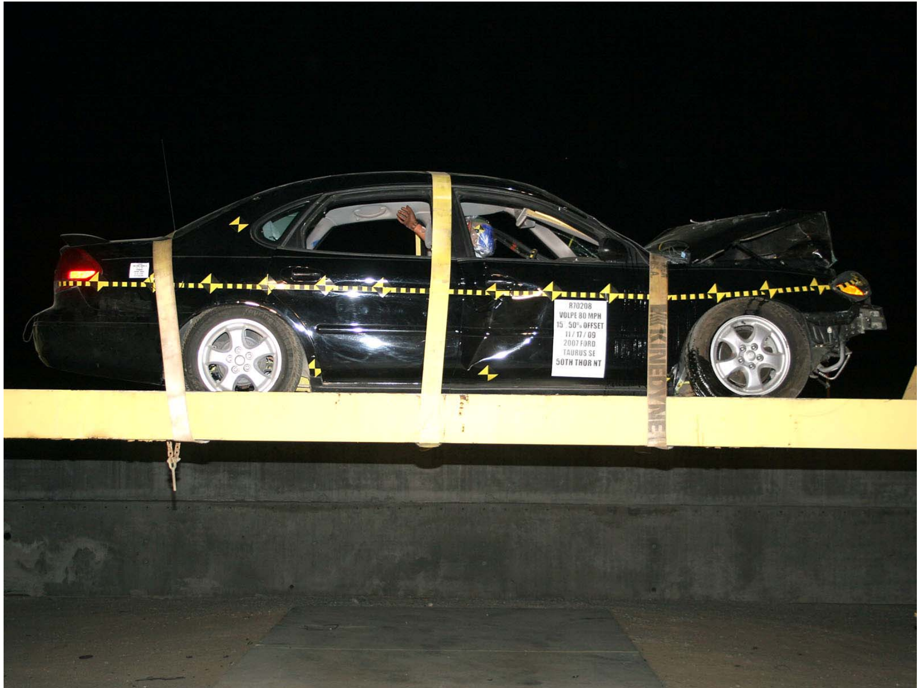
Figure A-327: Test Vehicle on Rollover Device (360°)
