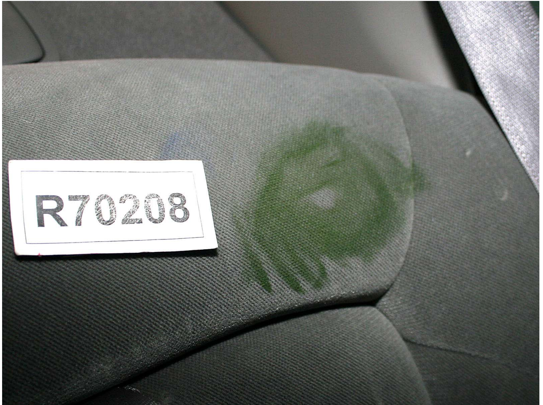
Figure A-278: Test Vehicle Post-Test Passenger Dummy Contact, Seat-Back
