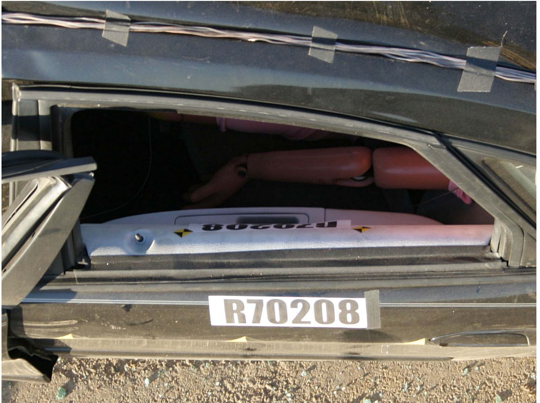
Figure A-271: Test Vehicle Post-Test Passenger Dummy Clearance from Door
