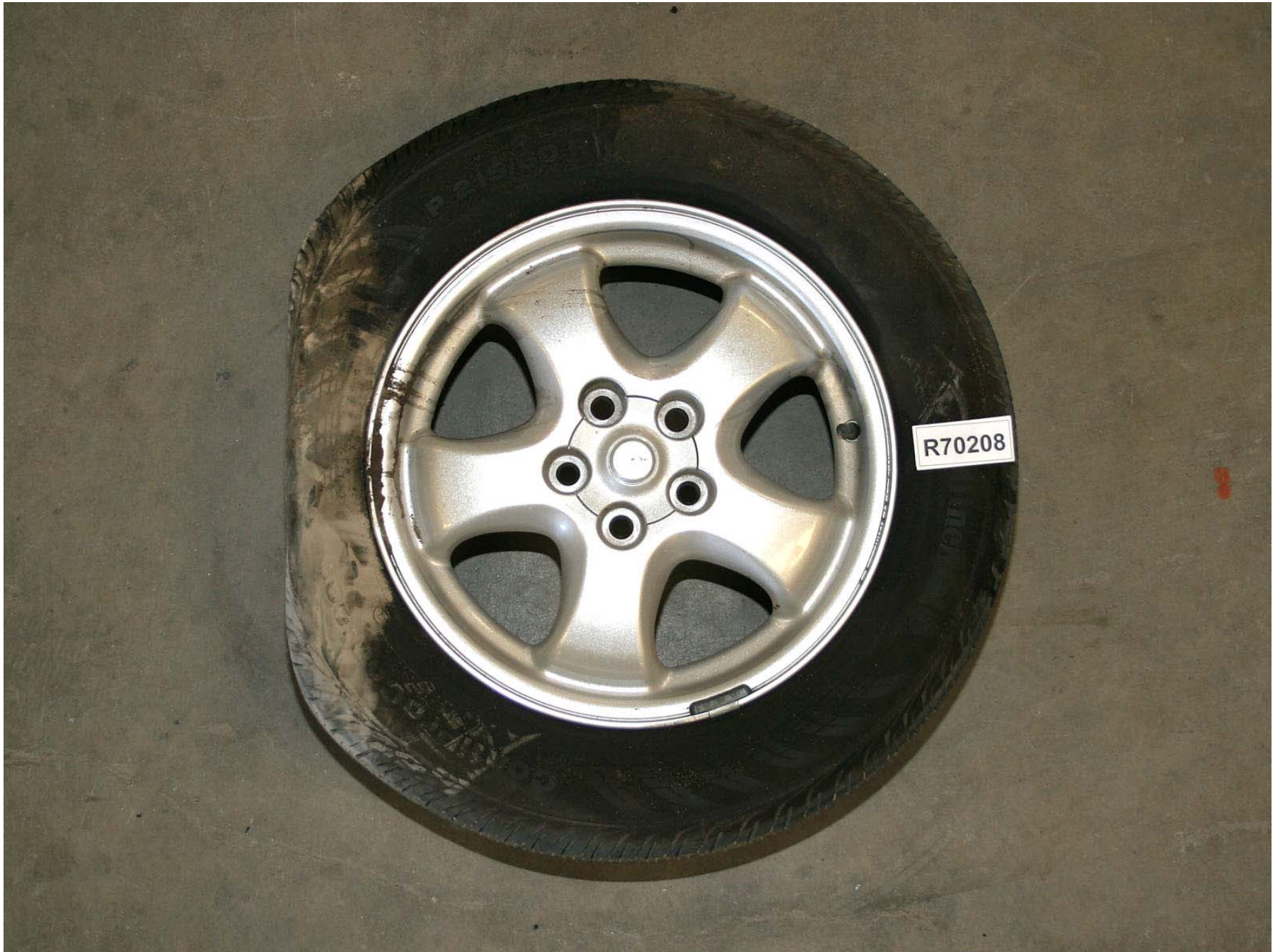
Figure A-120: Test Vehicle Post-Test Left Front Wheel Damage (Outside)
