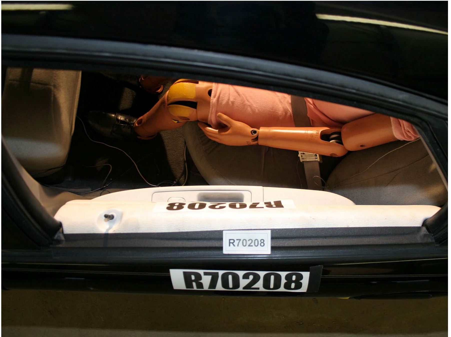
Figure A-270: Test Vehicle Pre-Test Passenger Dummy Clearance from Door
