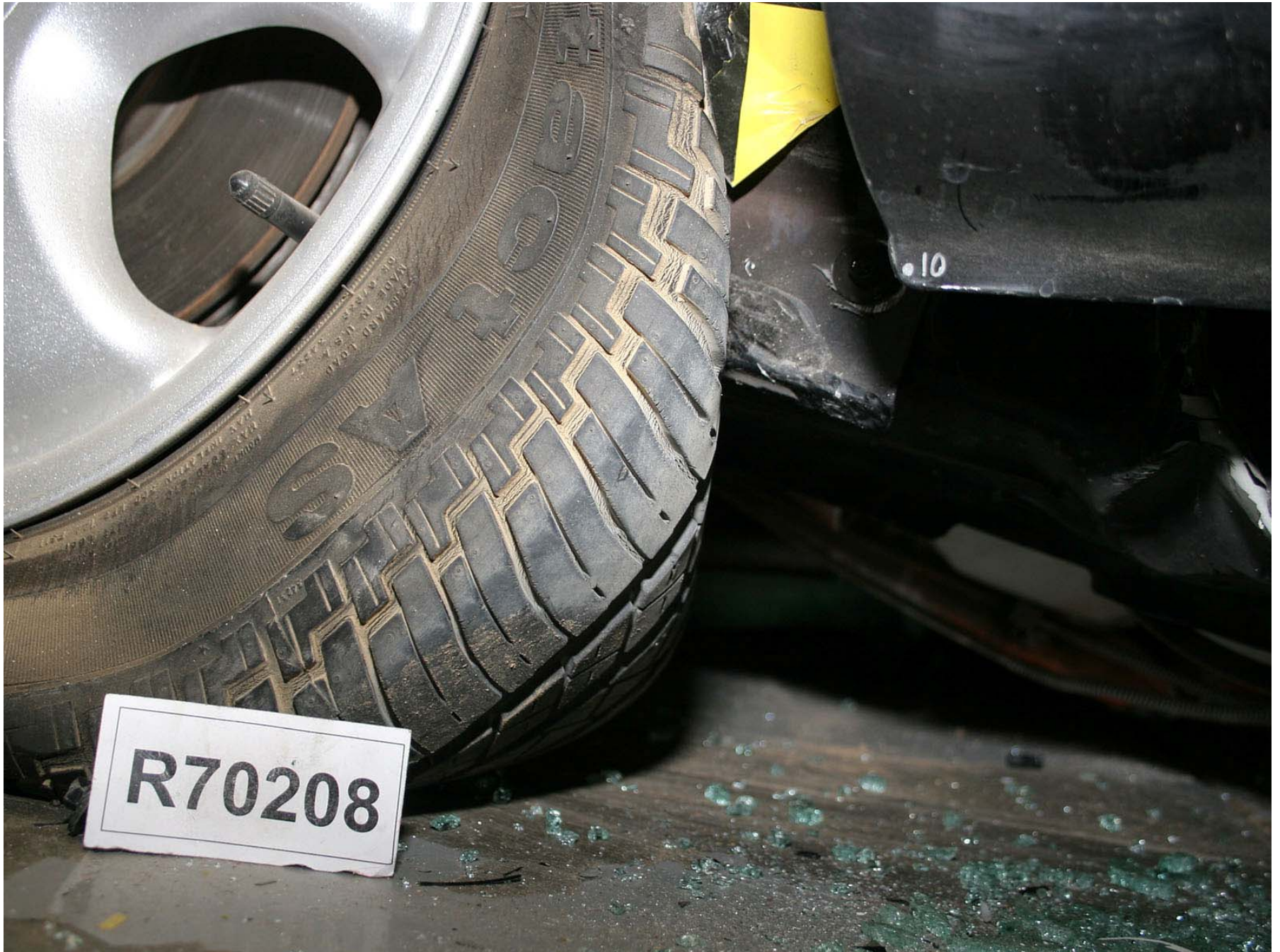
Figure A-119: Test Vehicle Post-Test Left Front Wheel A-Pillar/Rocker Contact
