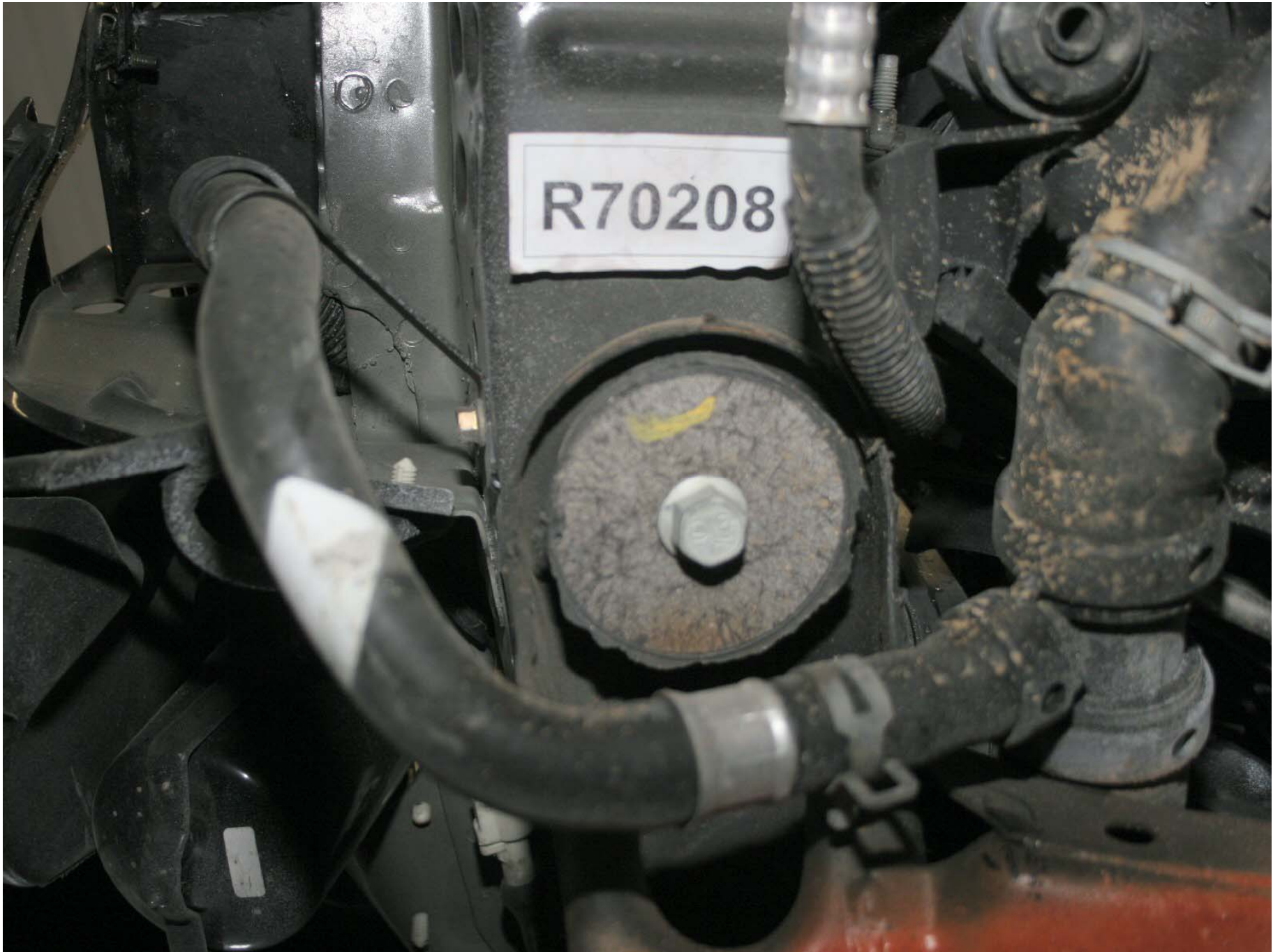
Figure A-201: Test Vehicle Post-Test Right Front Sub-Frame Mounting Point
