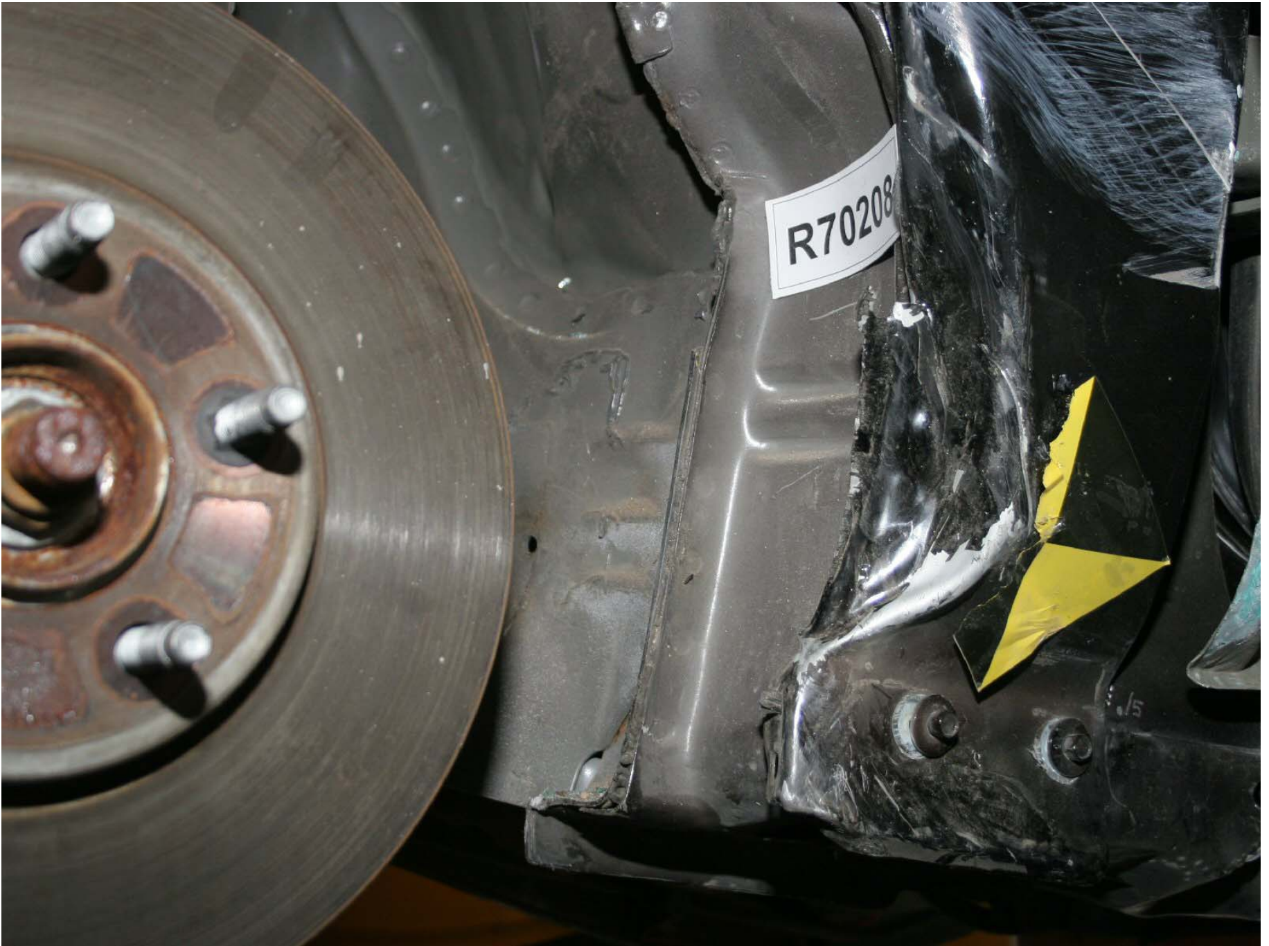
Figure A-157: Test Vehicle Post-Test Left Side Frame to A-Pillar Joint
