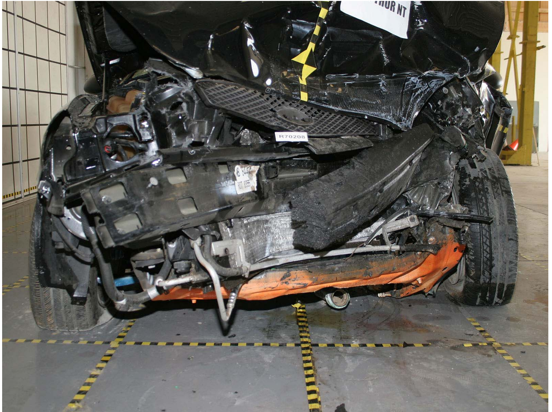
Figure A-306: Test Vehicle Post-Test Structural Member Crush Measurement (Hood Closed)
