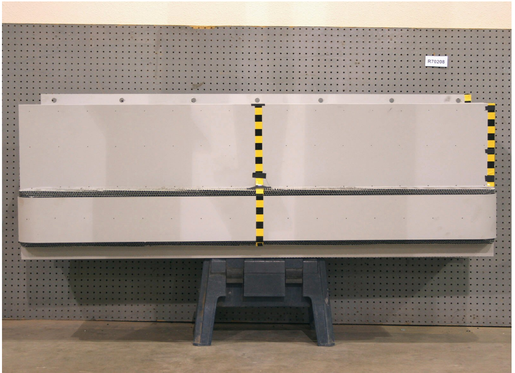
Figure A-315: Test Vehicle Pre-Test Front View of Deformable Barrier
