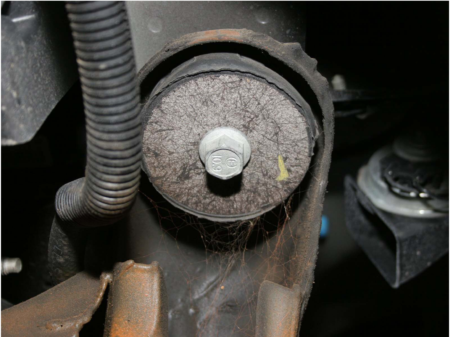
Figure A-164: Test Vehicle Pre-Test Left Front Sub-Frame Mounting Point
