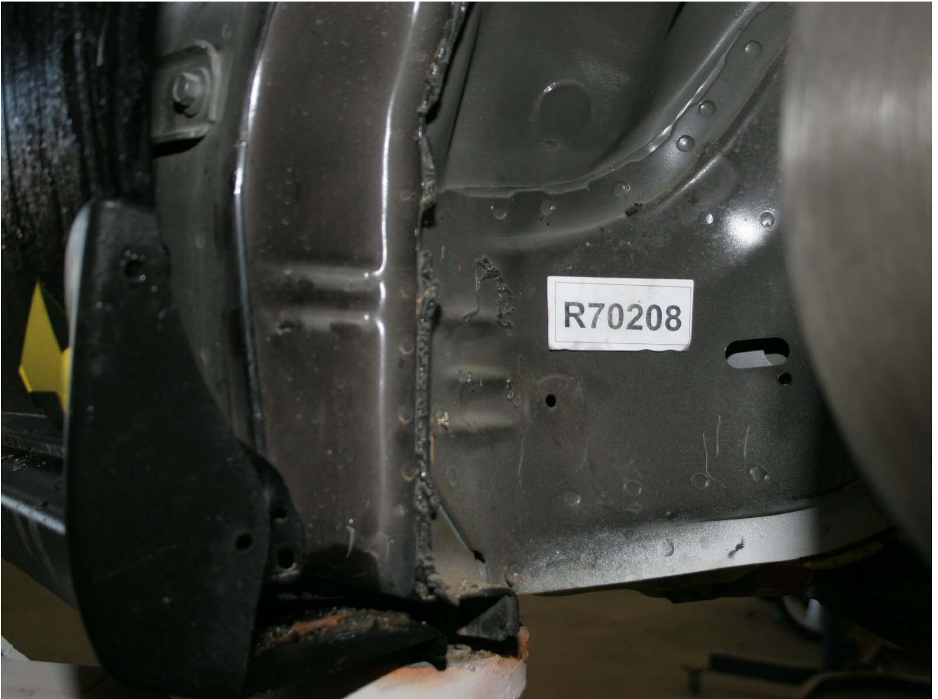
Figure A-189: Test Vehicle Post-Test Right Side Frame to A-Pillar Joint
