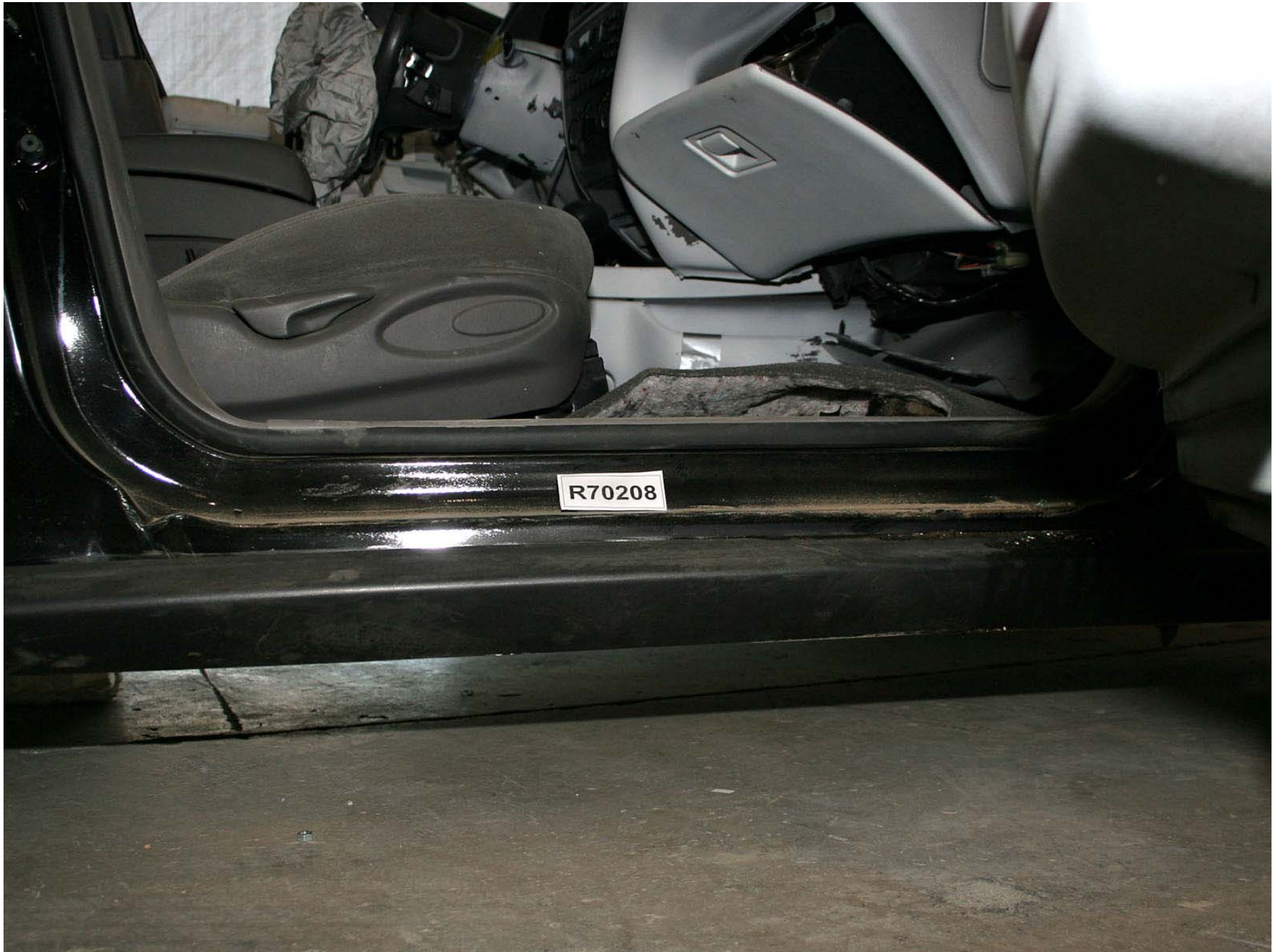
Figure A-94: Test Vehicle Post-Test Right Front Sill Side View, Door Open
