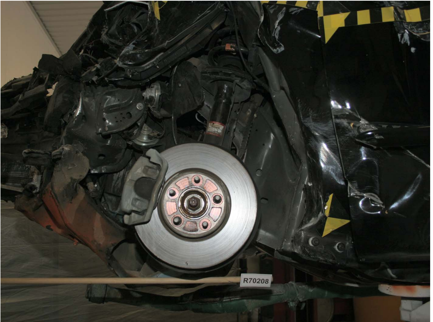
Figure A-137: Test Vehicle Post-Test Left Front Wheel Well (Tire Off), Inner Fender Removed
