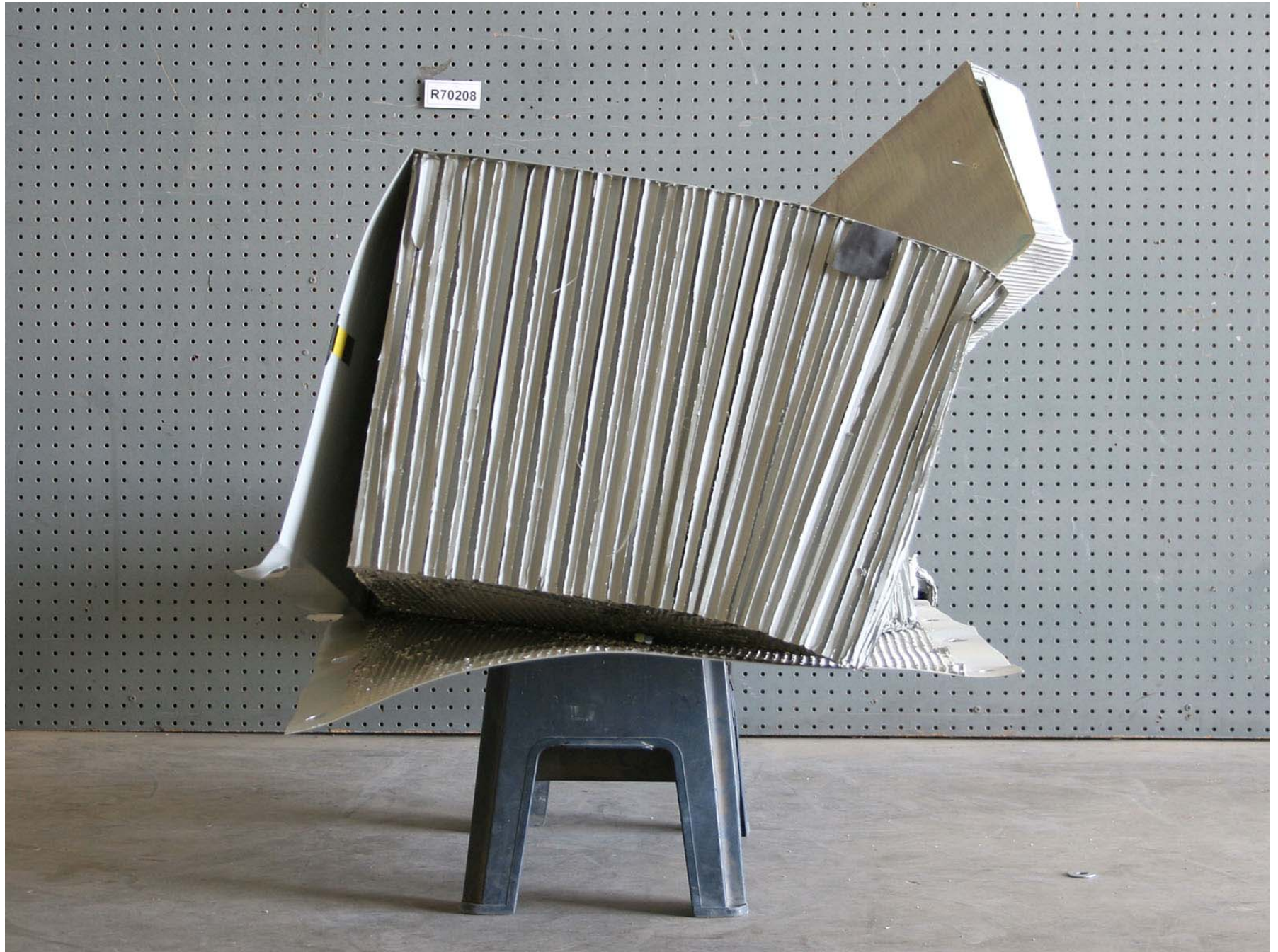
Figure A-320: Test Vehicle Post-Test Right Side View of Deformable Barrier
