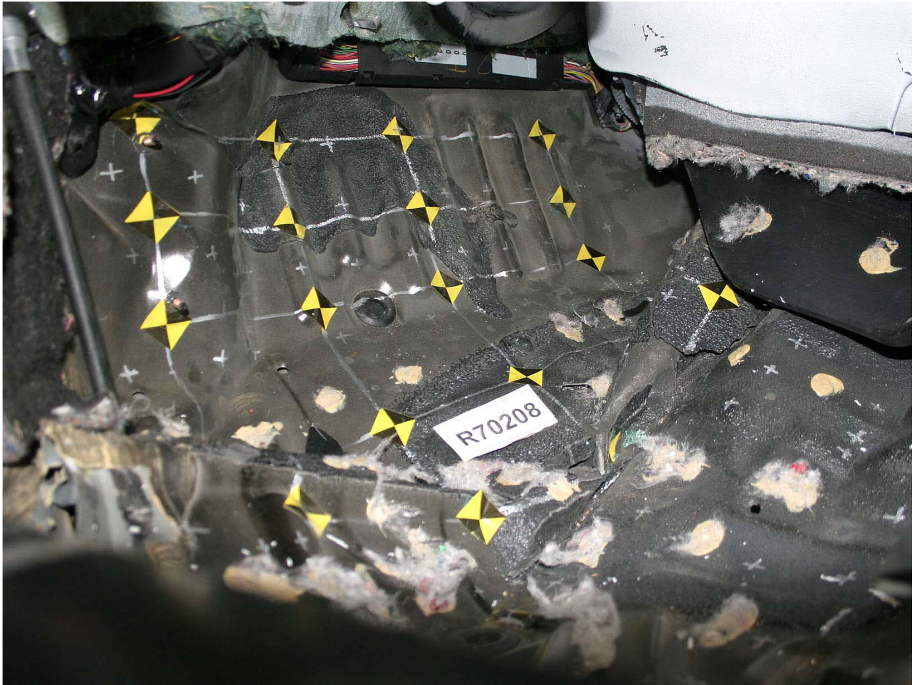
Figure A-284: Test Vehicle Post-Test Driver Floorpan Left \frac{3}{4} View, Sill Height
