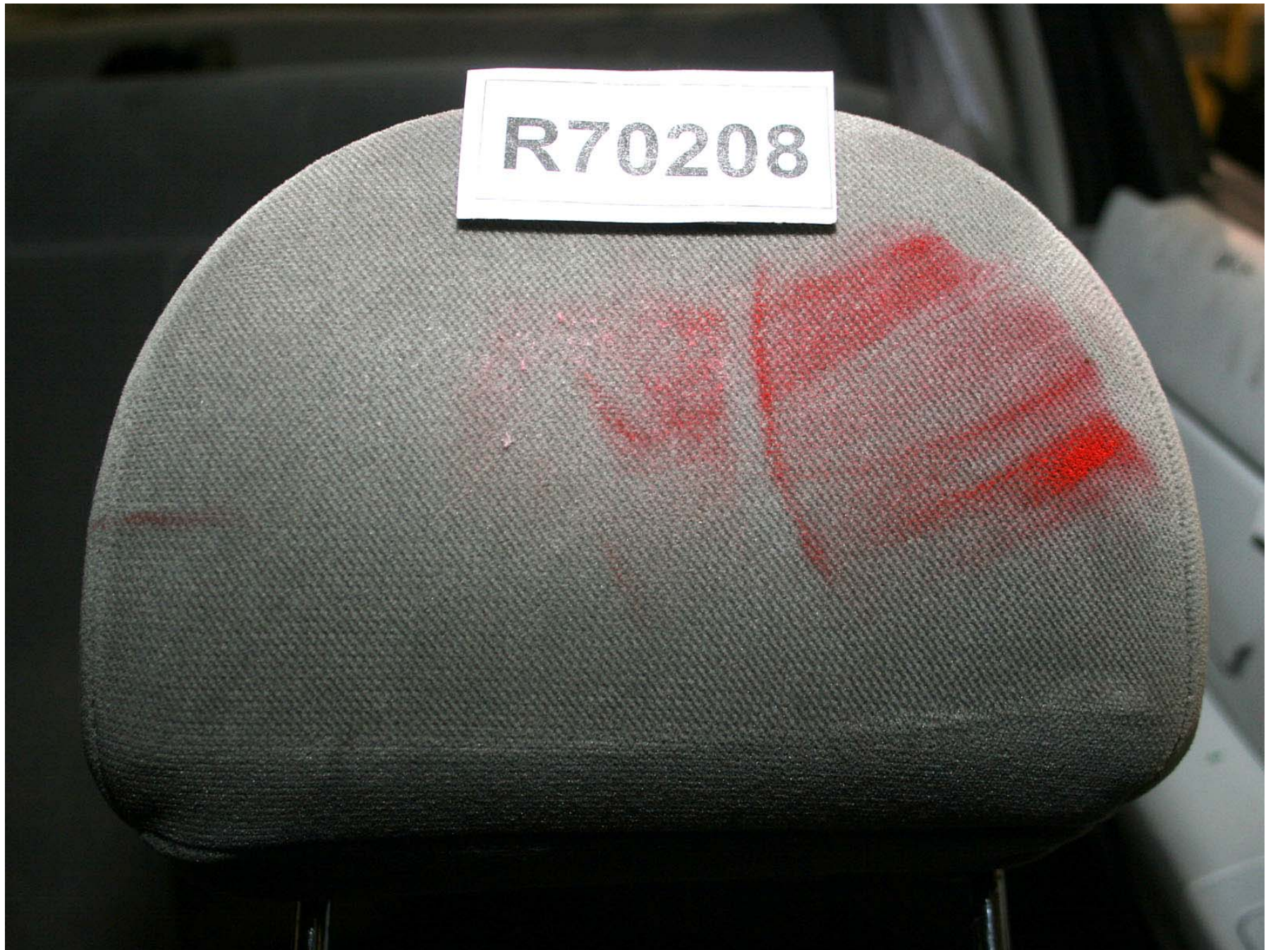
Figure A-252: Test Vehicle Post-Test Driver Dummy Contact, Headrest
