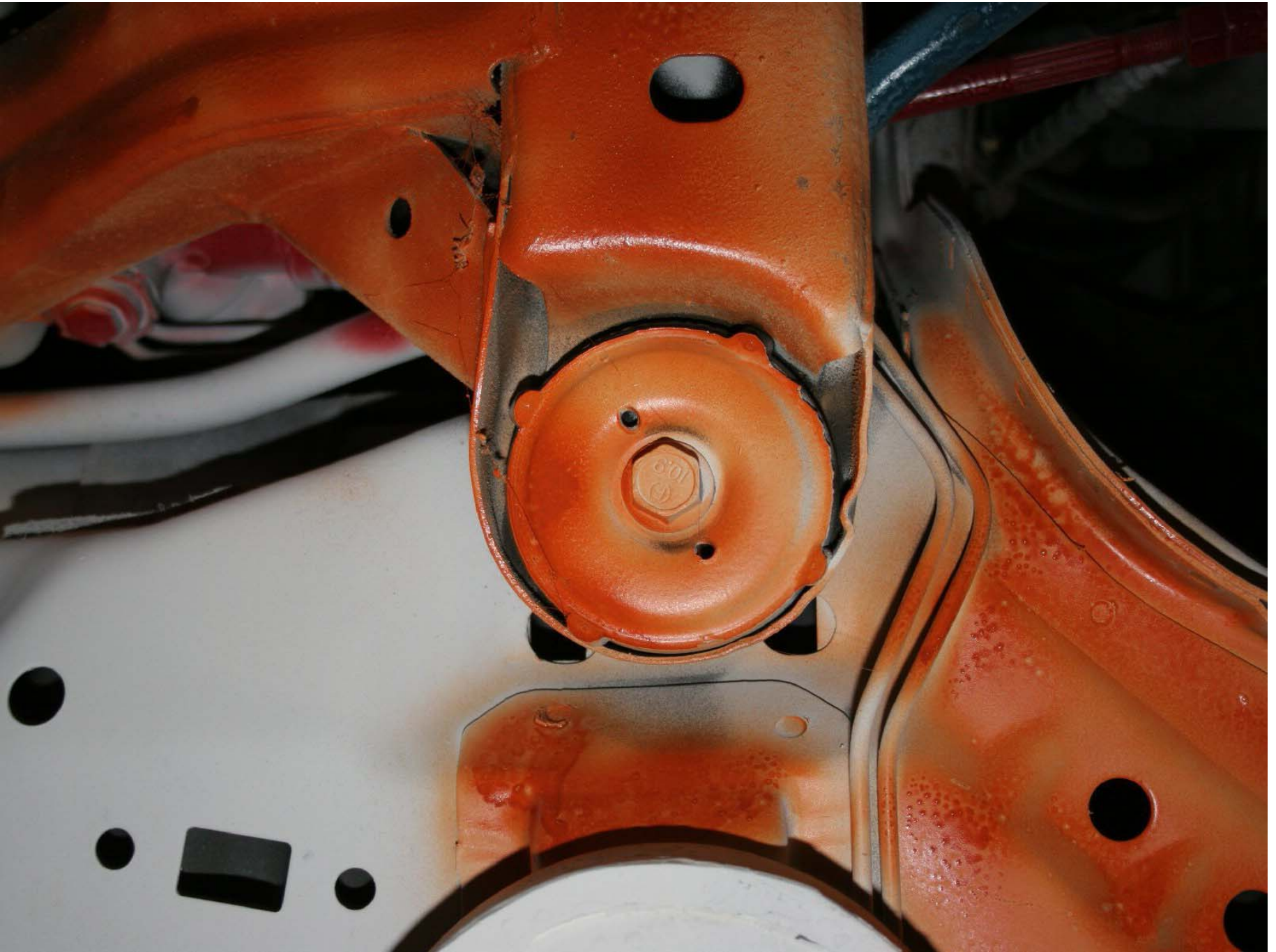
Figure A-166: Test Vehicle Pre-Test Left Rear Sub-Frame Mounting Point
