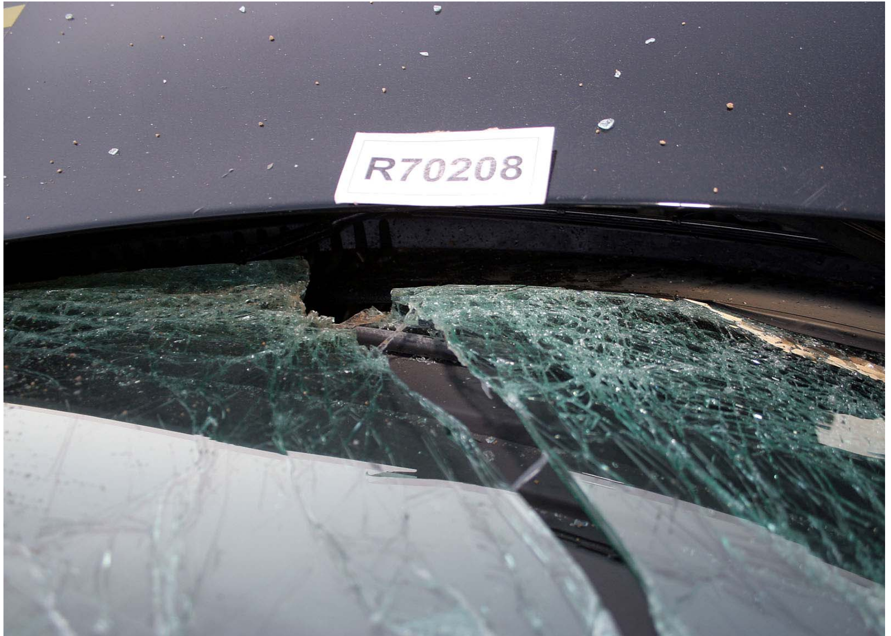
Figure A-312: Test Vehicle Post-Test Windshield Separation Close Up
