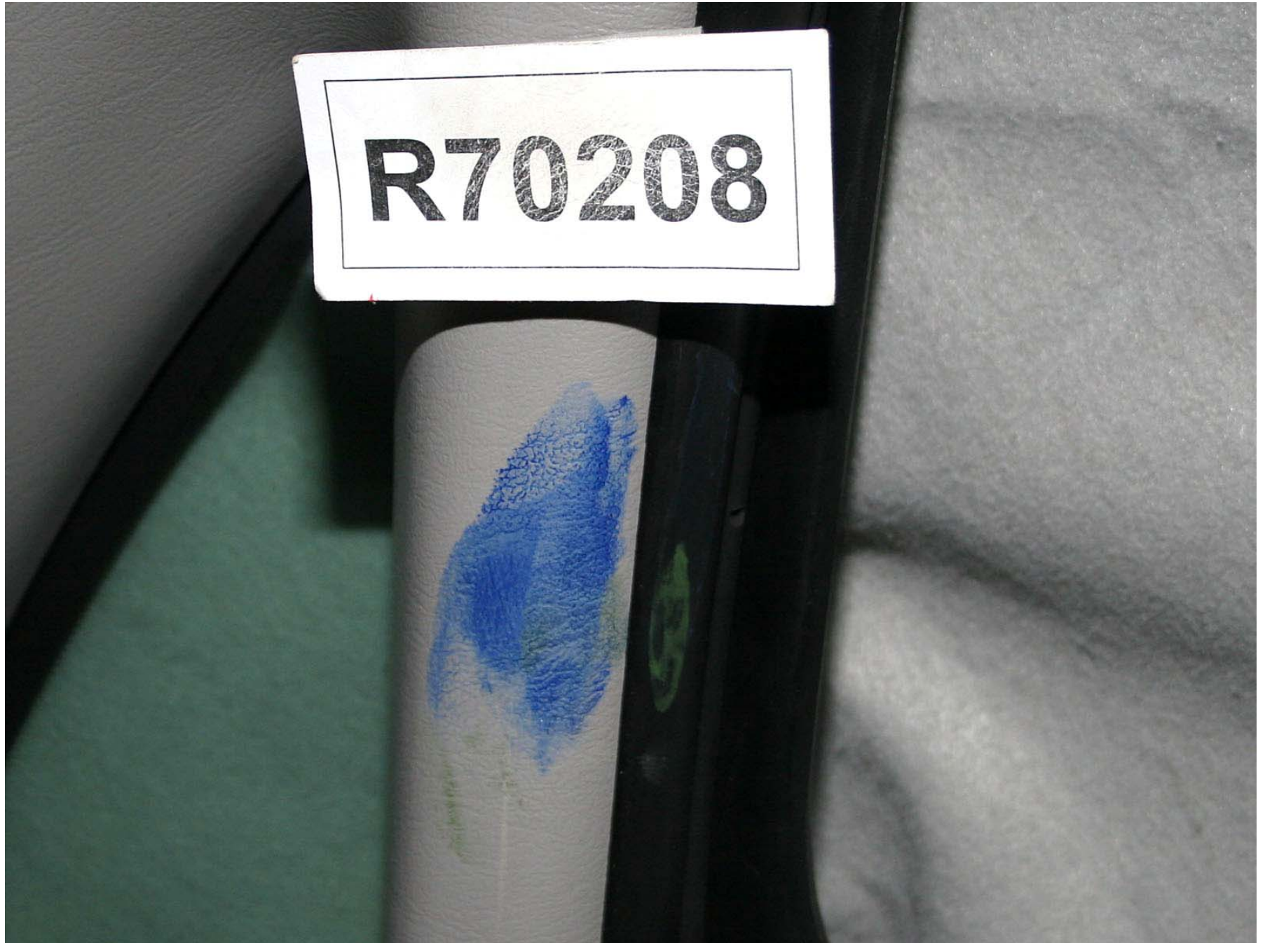
Figure A-277: Test Vehicle Post-Test Passenger Dummy Contact, C-Pillar
