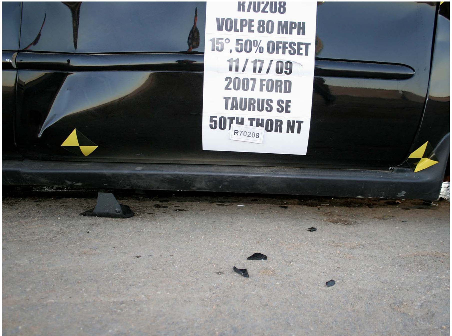
Figure A-92: Test Vehicle Post-Test Right Front Sill Side View, Door Closed
