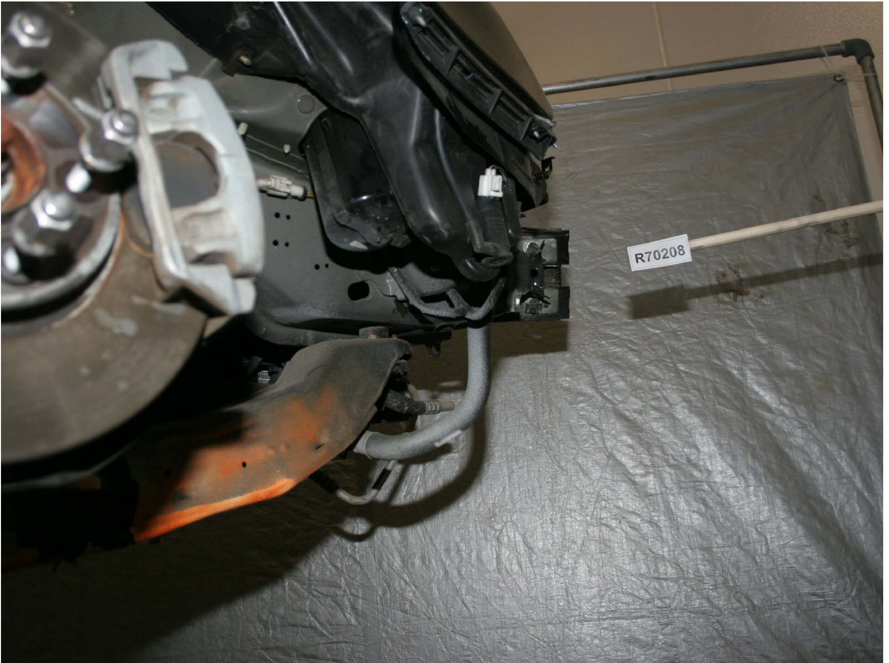
Figure A-195: Test Vehicle Post-Test Right Side Crush Initiators
