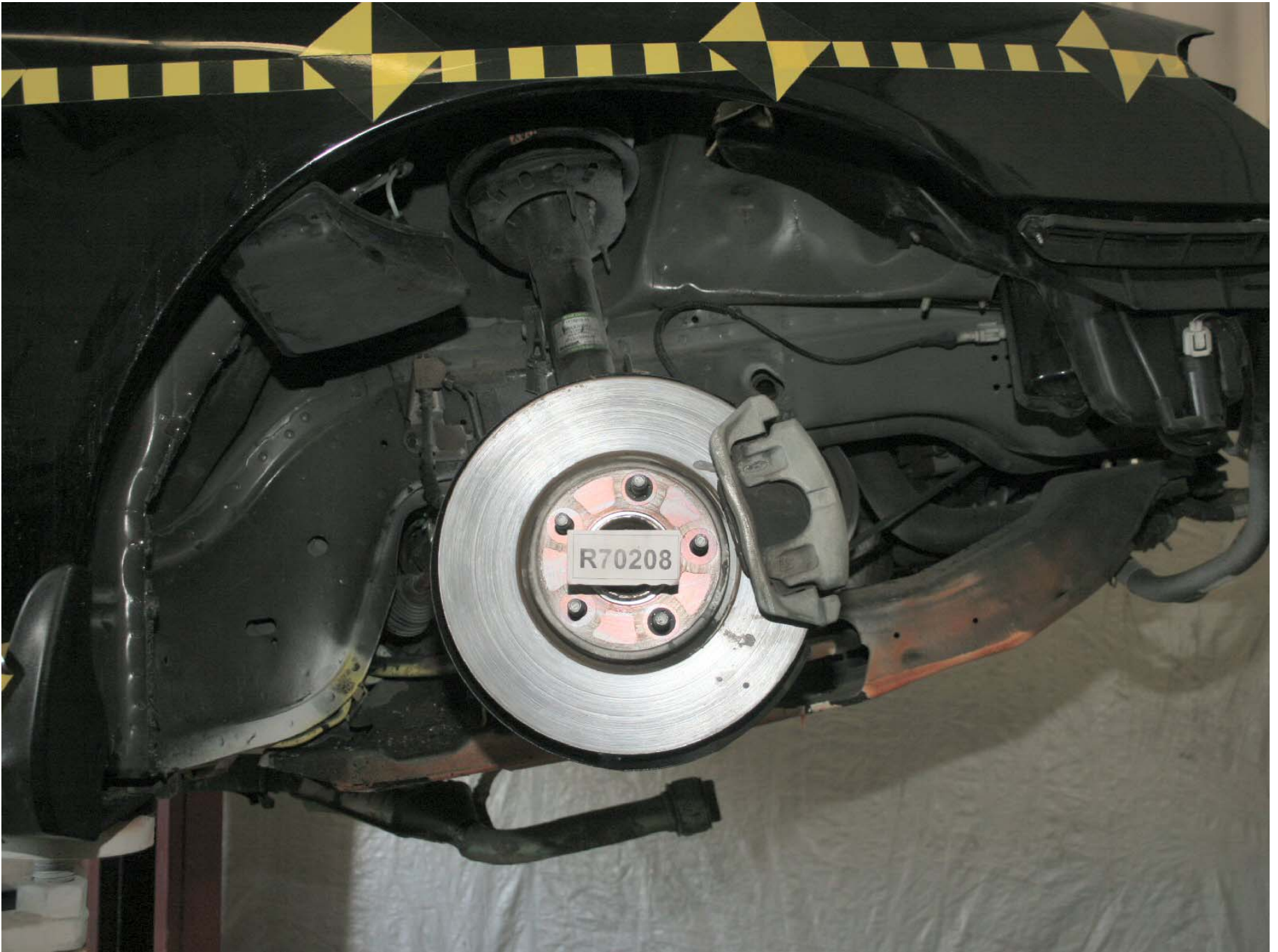
Figure A-173: Test Vehicle Post-Test Right Front Wheel Well (Tire Off), Inner Fender Removed
