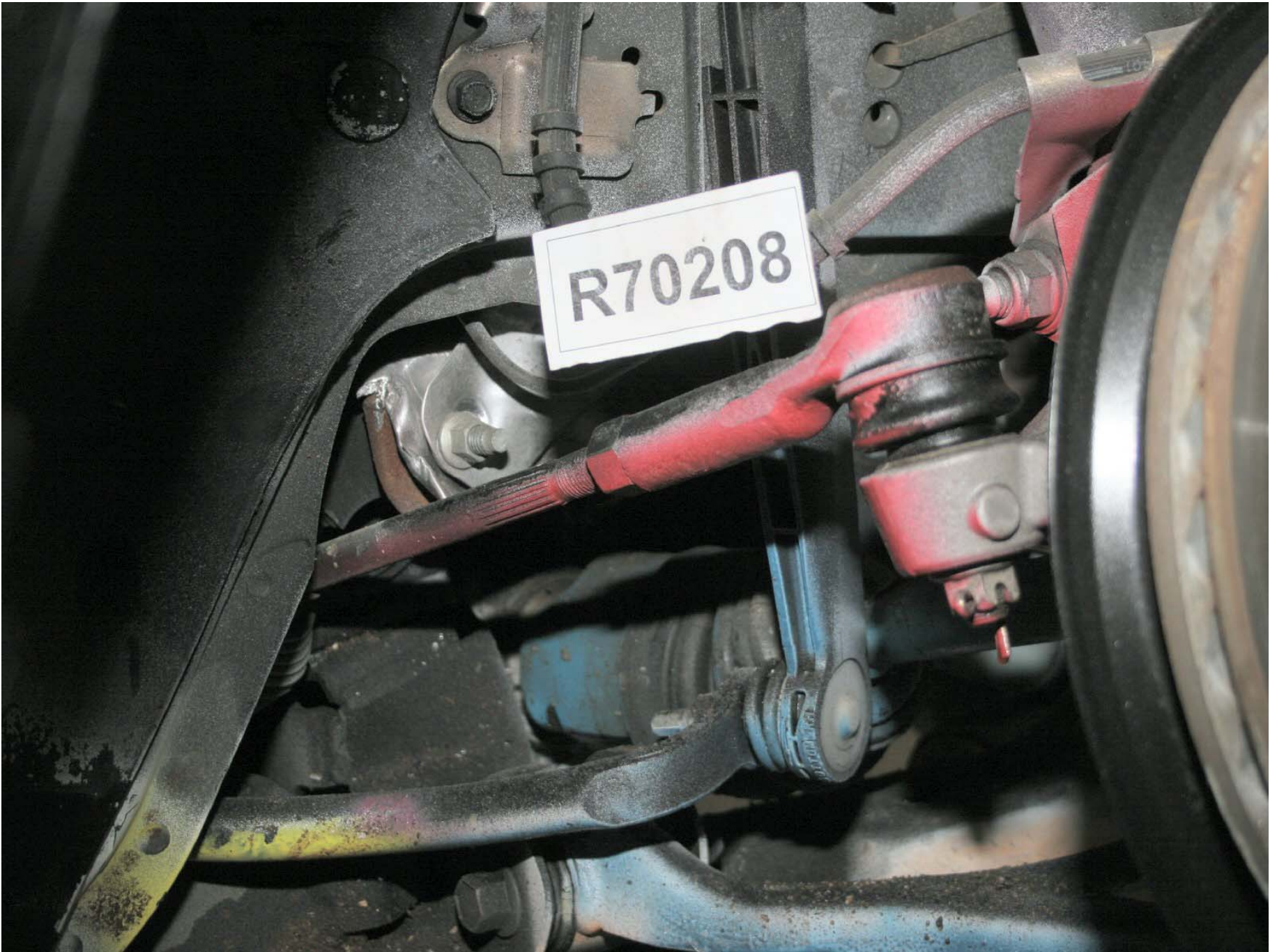
Figure A-191: Test Vehicle Post-Test Right Side Tie Rod and Sway Bar Attachments Points
