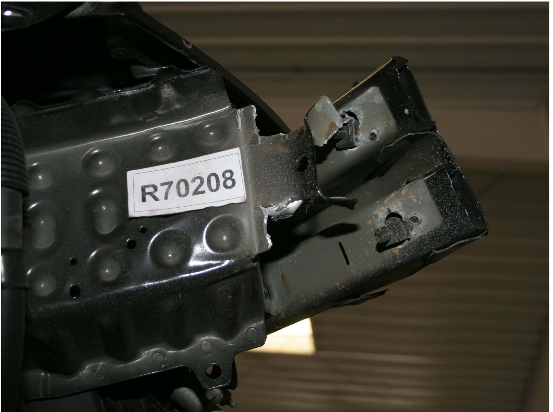
Figure A-199: Test Vehicle Post-Test Right Side Bumper Attachment Point
