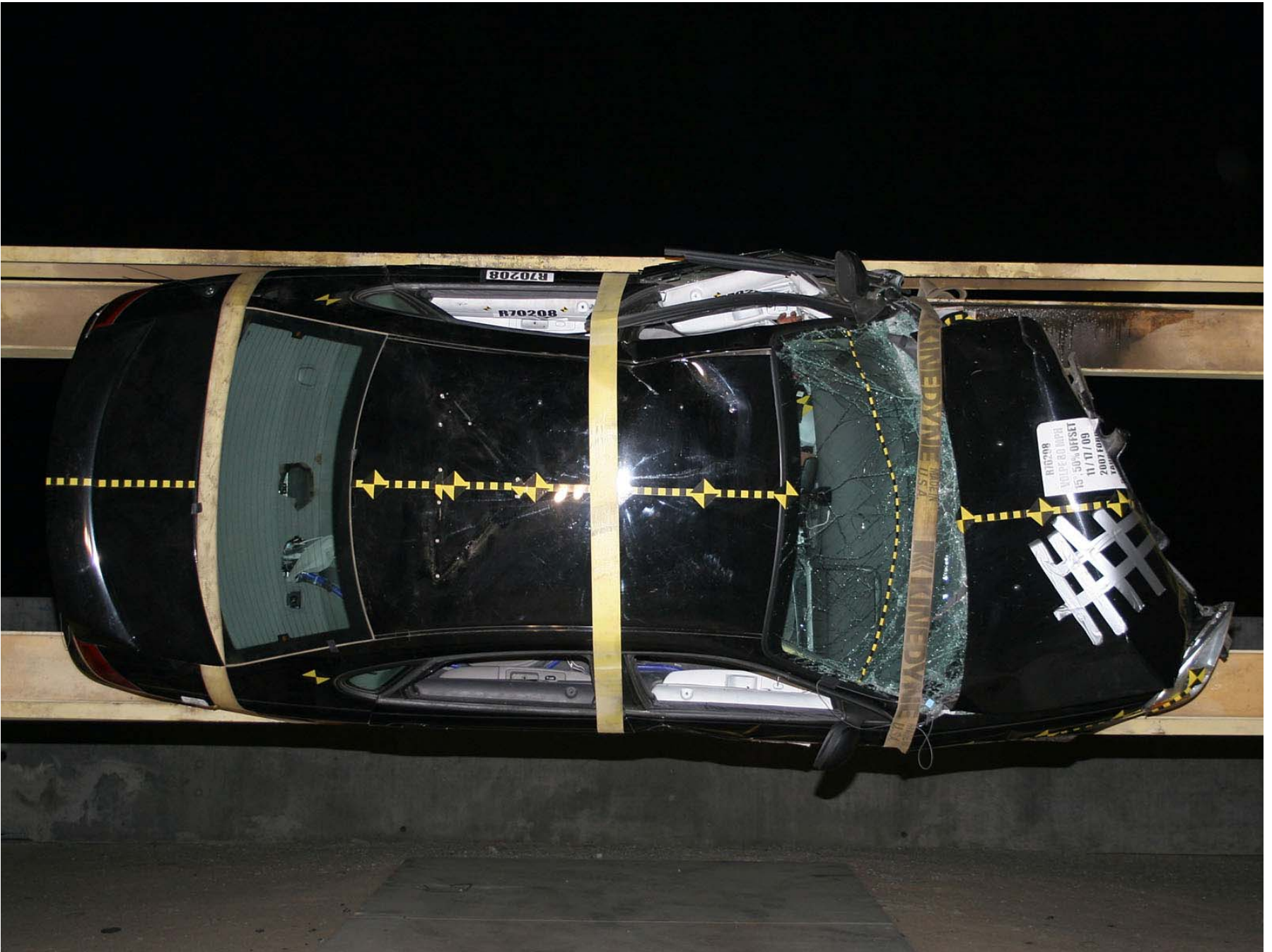
Figure A-324: Test Vehicle on Rollover Device (90°)
