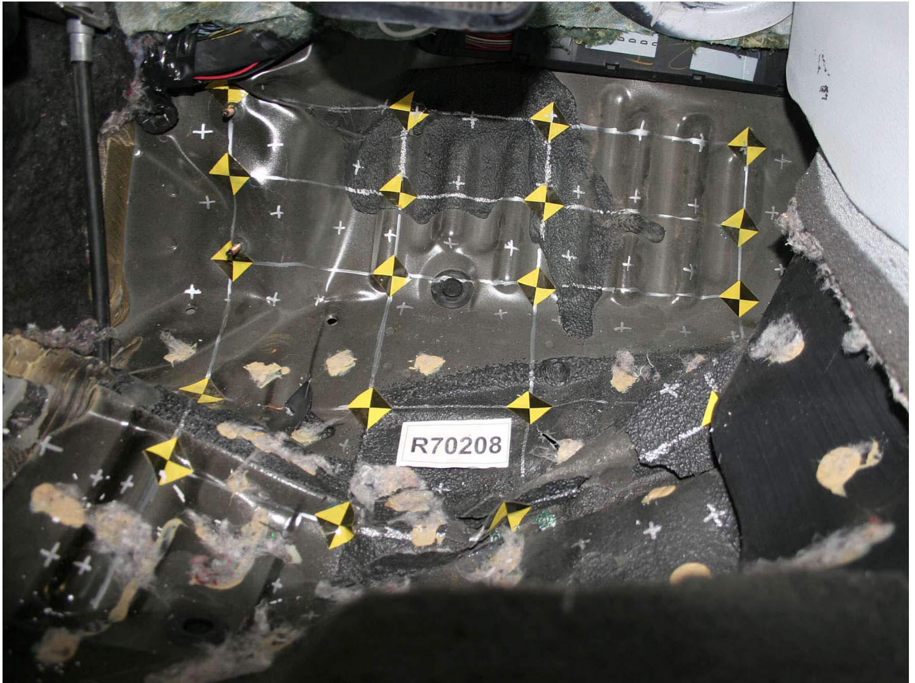
Figure A-286: Test Vehicle Post-Test Driver Floorpan, Seat Cushion Height
