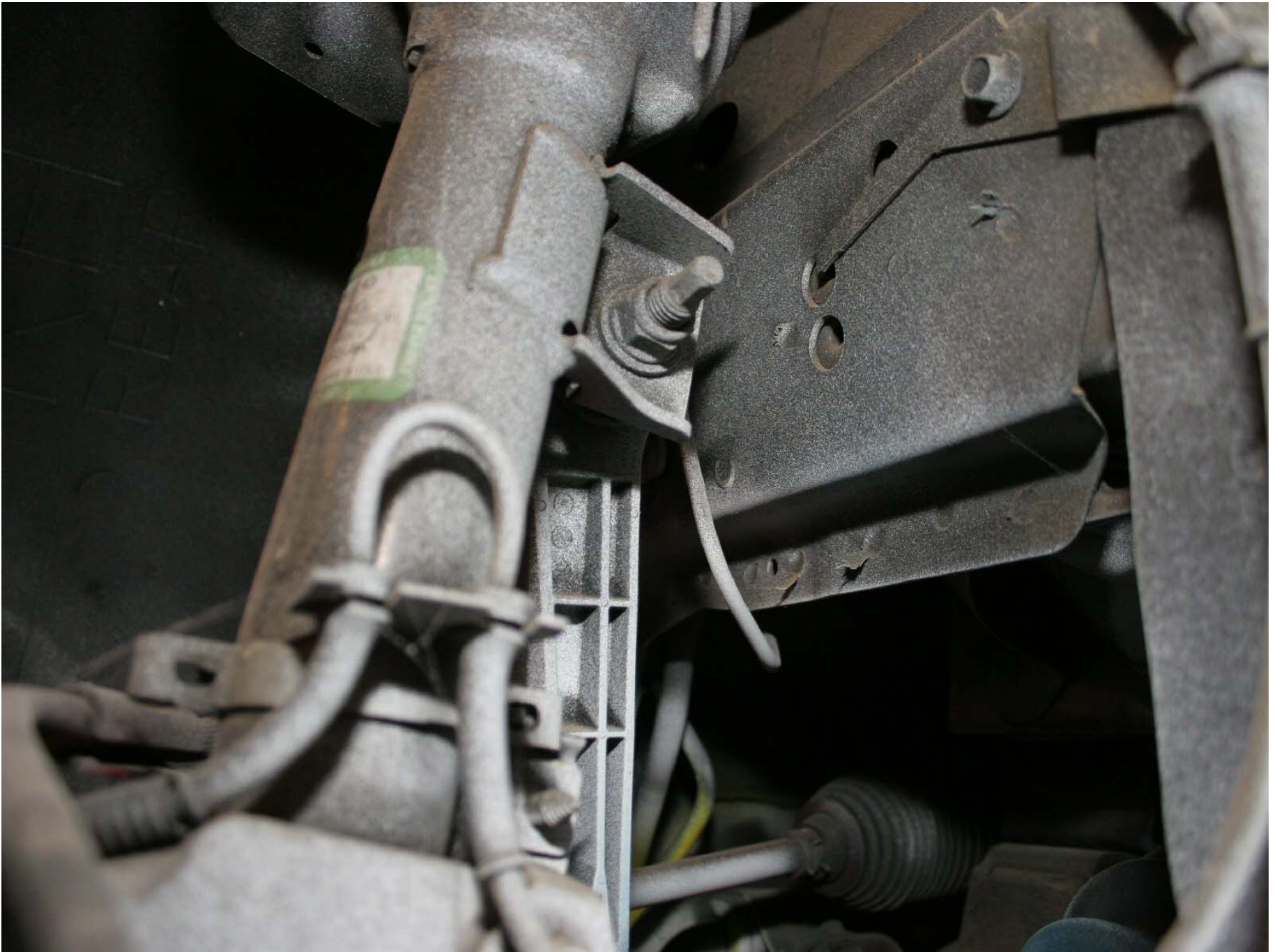
Figure A-192: Test Vehicle Pre-Test Right Side Upper Sway Bar Attachment Point
