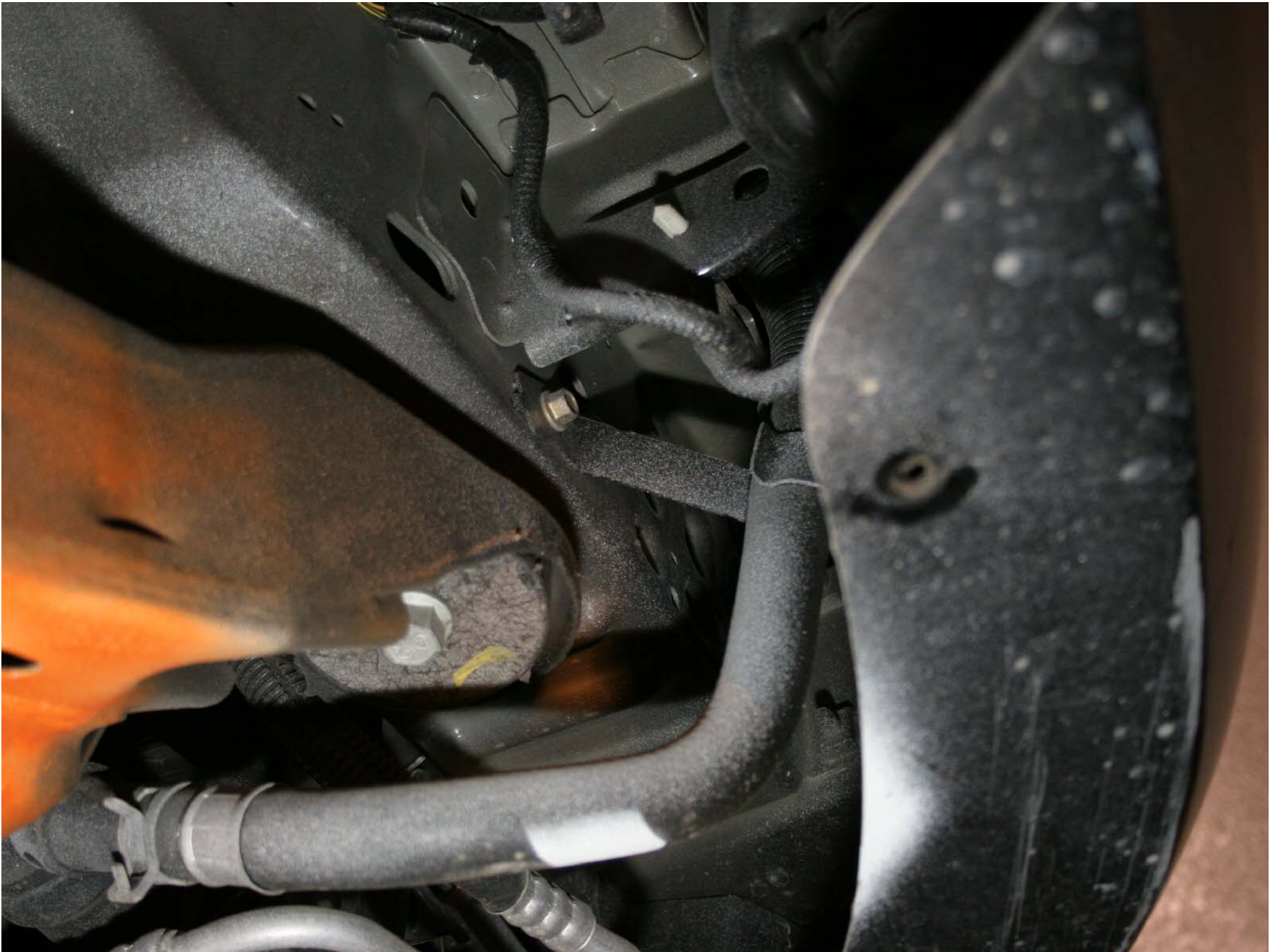
Figure A-194: Test Vehicle Pre-Test Right Side Crush Initiators
