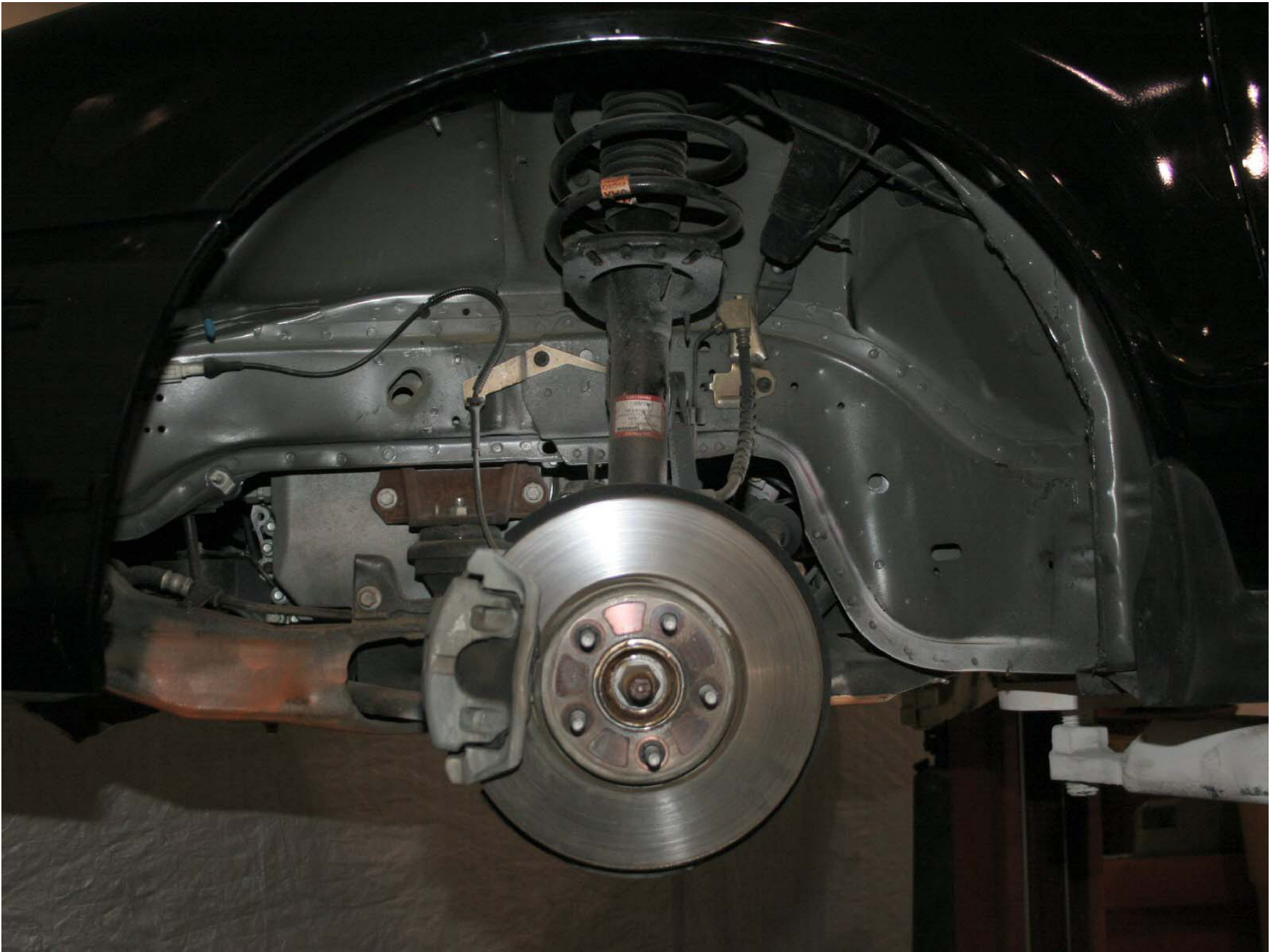
Figure A-136: Test Vehicle Pre-Test Left Front Wheel Well (Tire Off), Inner Fender Removed
