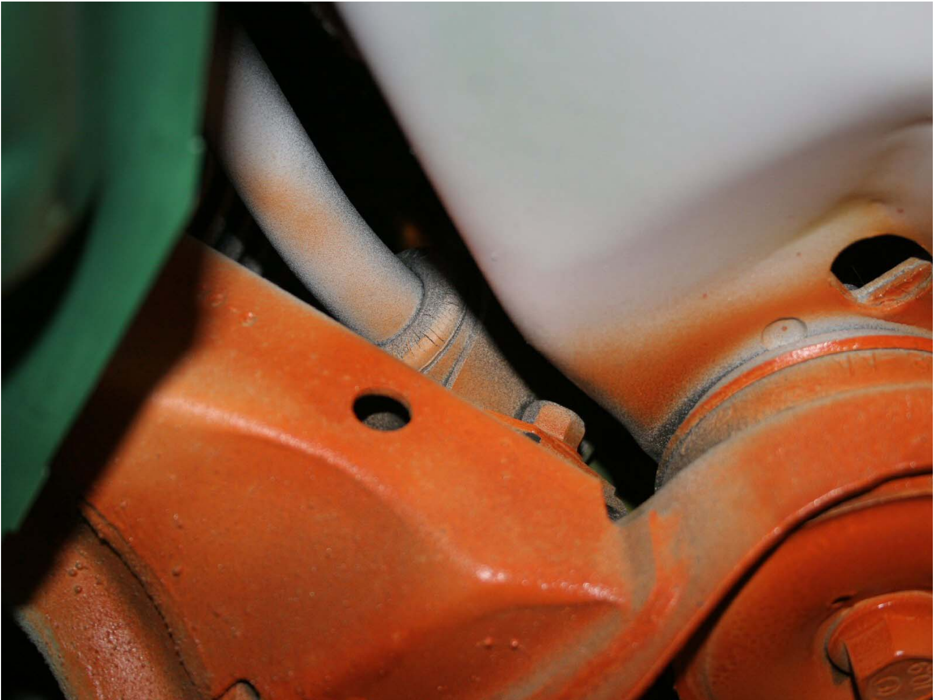
Figure A-218: Test Vehicle Pre-Test Sway Bar Right Side Mounting Bolts
