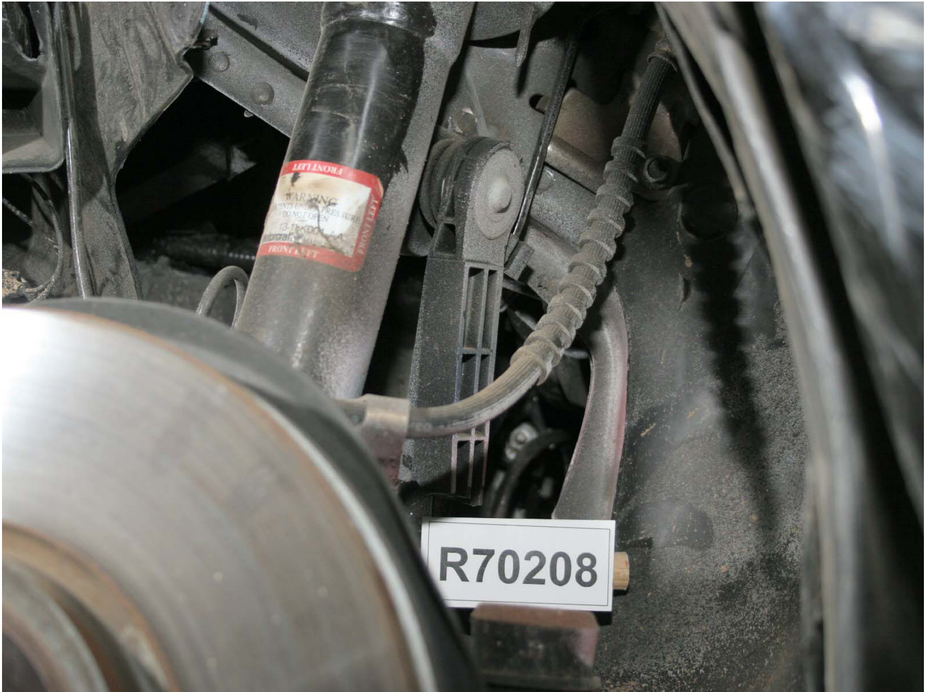
Figure A-155: Test Vehicle Post-Test Left Side Upper Sway Bar Attachment Point
