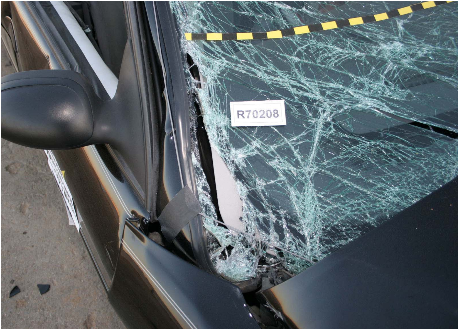
Figure A-311: Test Vehicle Post-Test Windshield Separation
