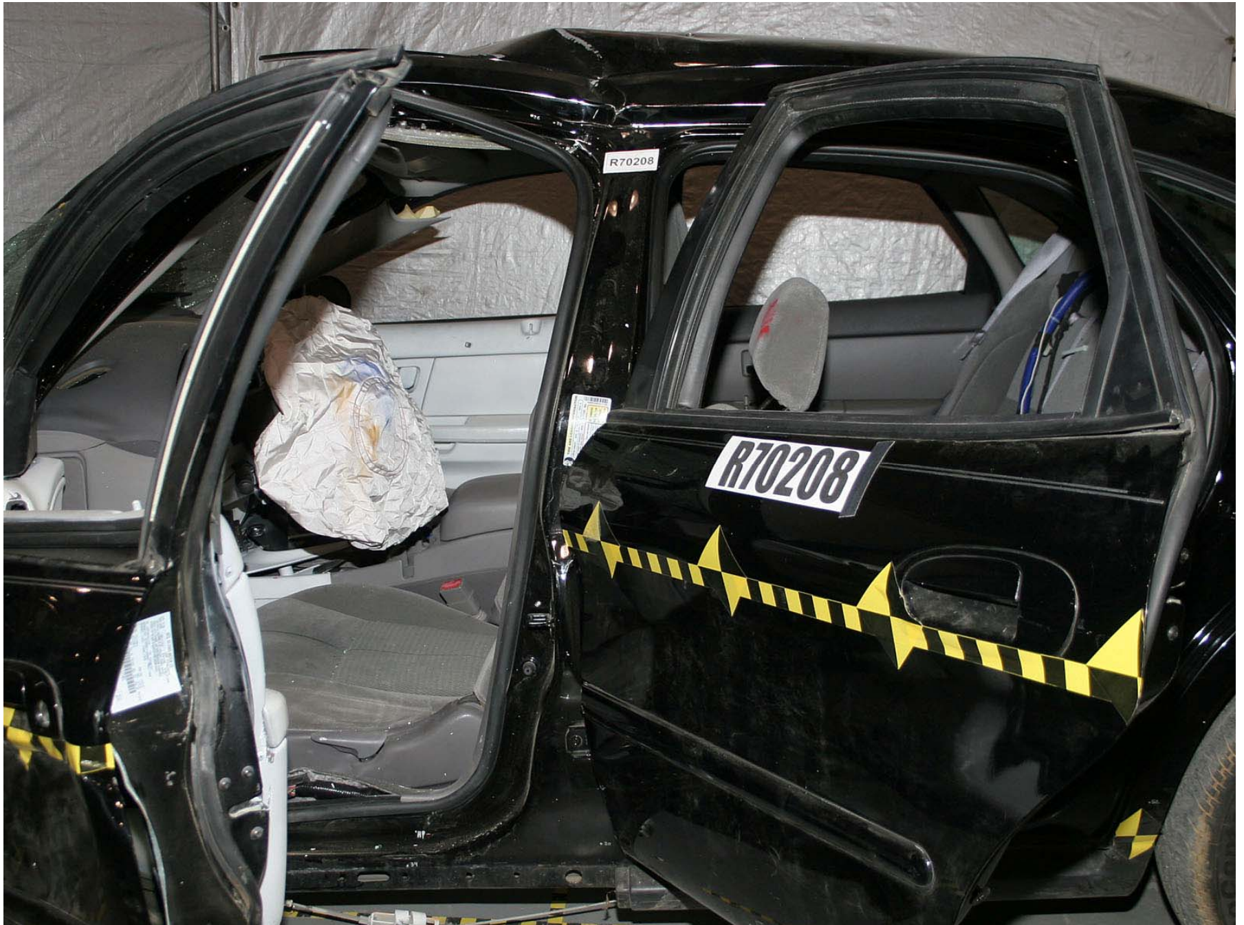
Figure A-56: Test Vehicle Post-Test Left Side B-Pillar Side View
