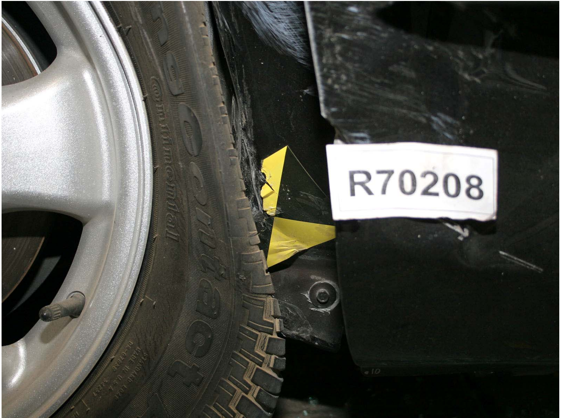
Figure A-118: Test Vehicle Post-Test Left Front Wheel A-Pillar/Rocker Contact
