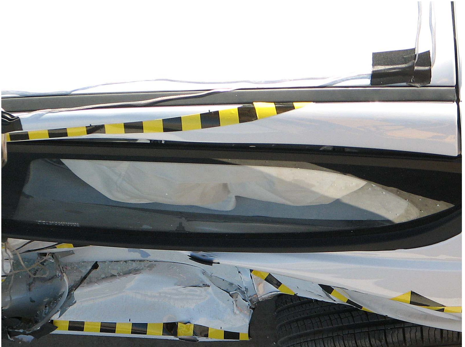
Figure A-46: Post-Test Passenger Dummy Clearance From Door
