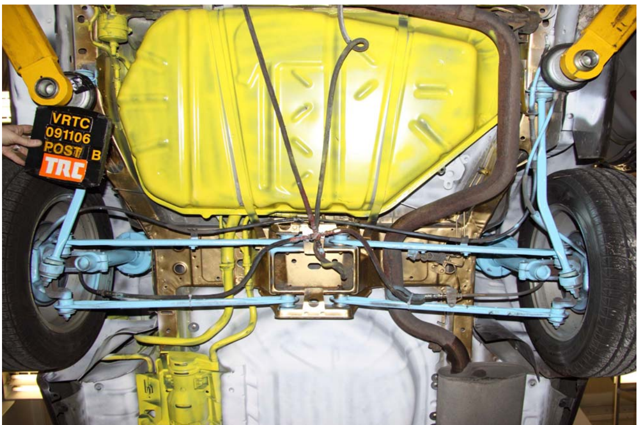
Figure A-70 Post-Test Bullet Vehicle Mid Rear Underbody View
