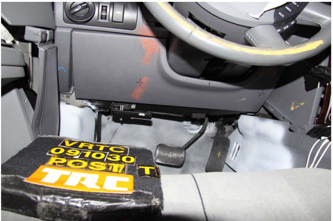
Figure A-123 Post-Test Target Vehicle Driver Dummy Knee Contact View
