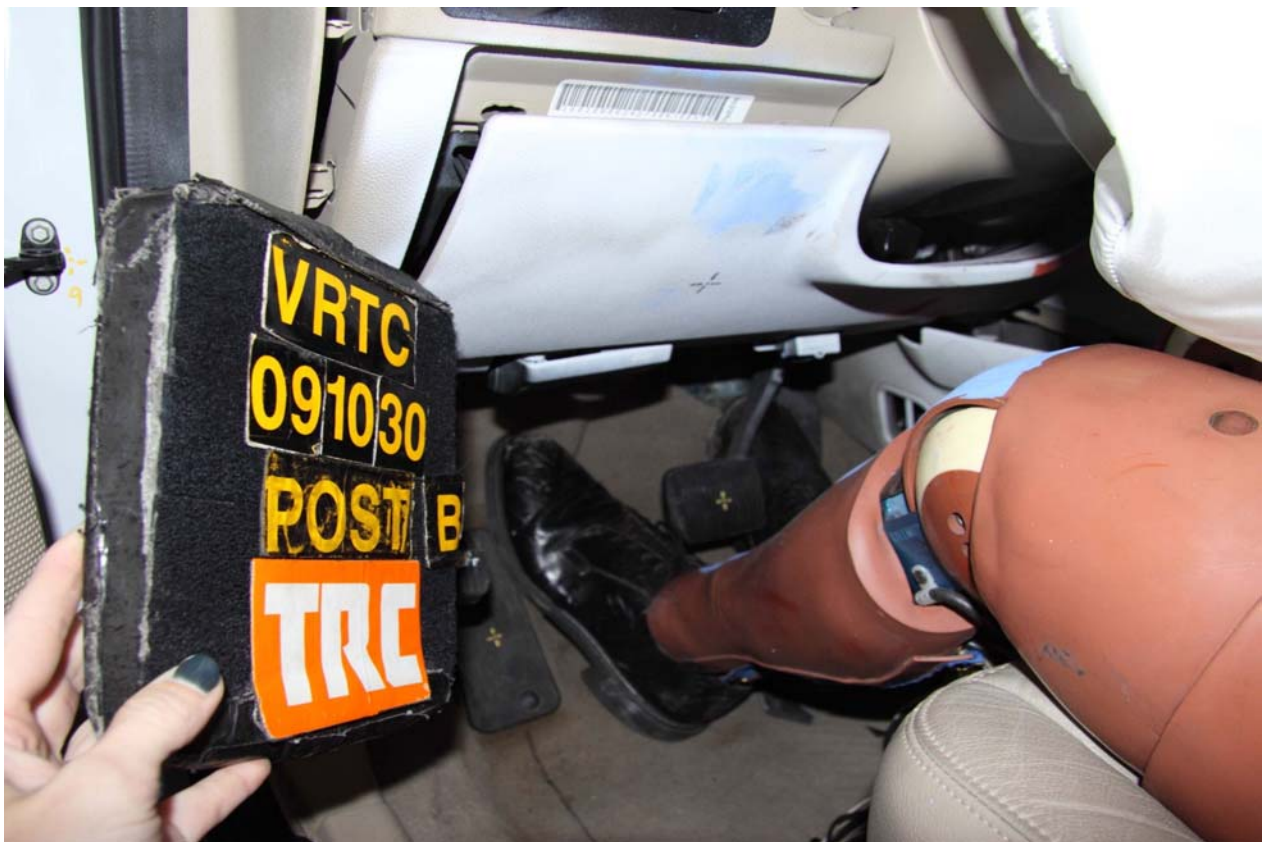
Figure A-98 Post-Test Bullet Vehicle Driver Dummy Knee Bolster View
