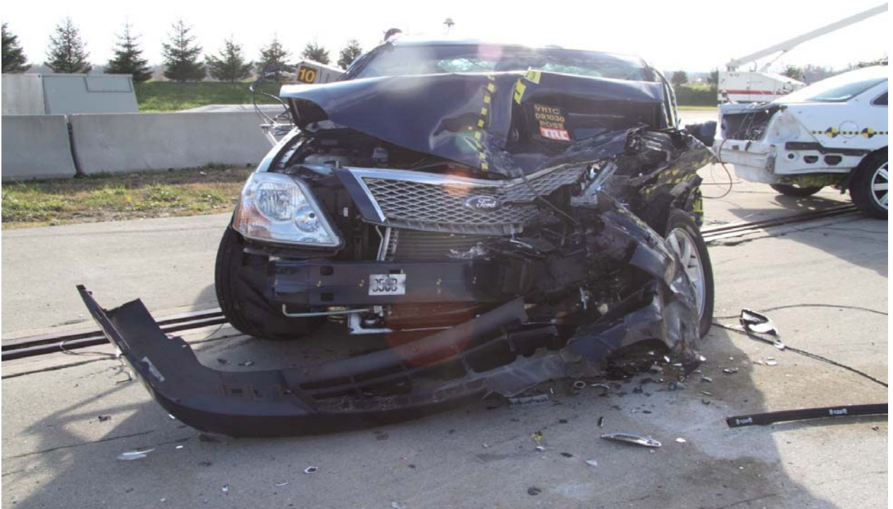
Figure A-18 Post-Test Target Vehicle Front View
