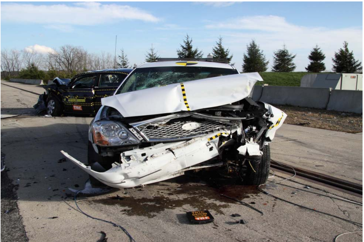
Figure A-46 Post-Test Bullet Vehicle Front View
