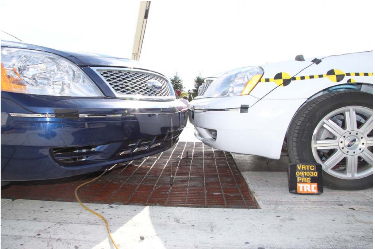
Figure A-15 Pre-Test Impact Alignment – View 1
