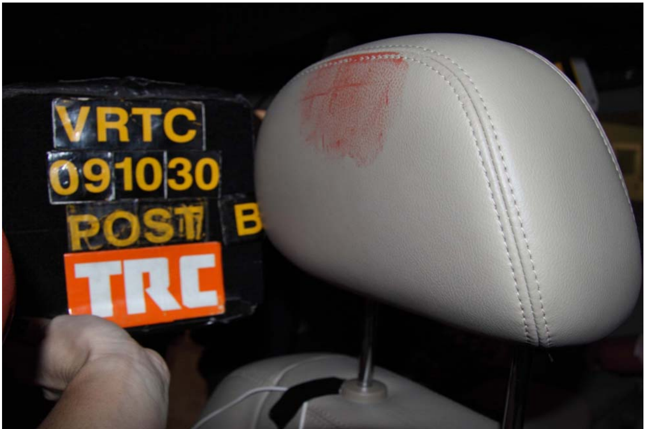
Figure A-126 Post-Test Bullet Vehicle Driver Dummy Head Contact - View 2
