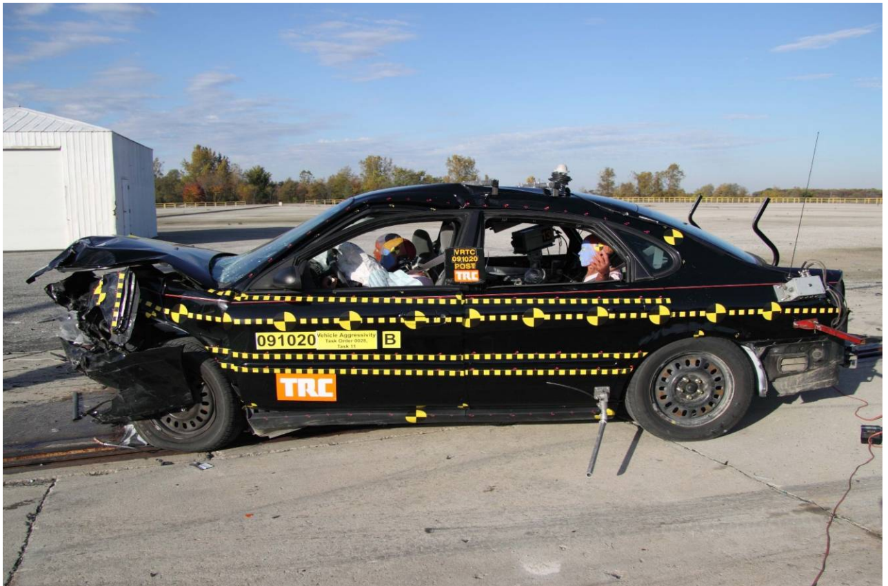
Figure A-48 Post-Test Bullet Vehicle Left Side View
