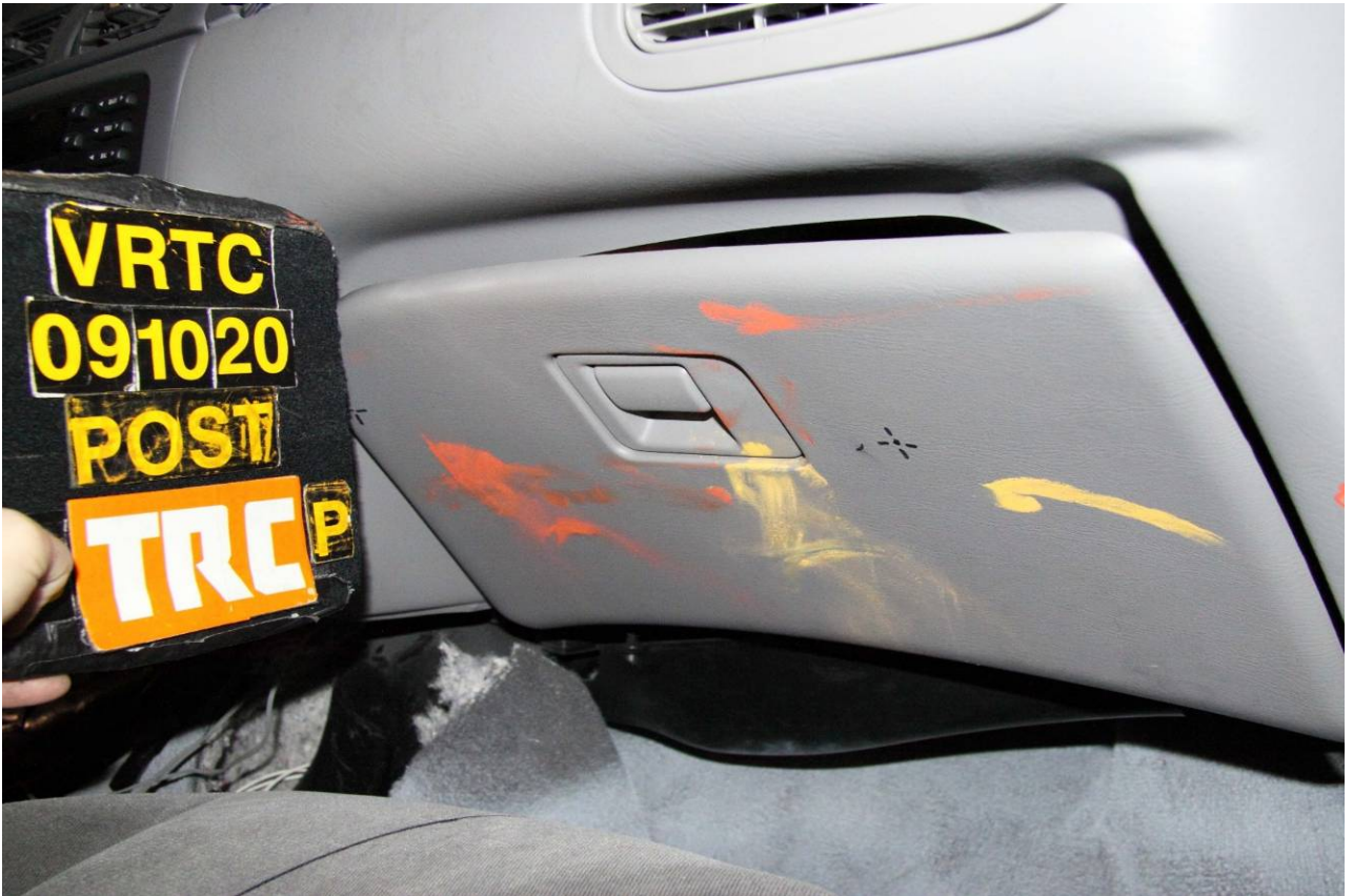
Figure A-122 Post-Test Bullet Vehicle Right Front Passenger Dummy Knee Contact - View 1
