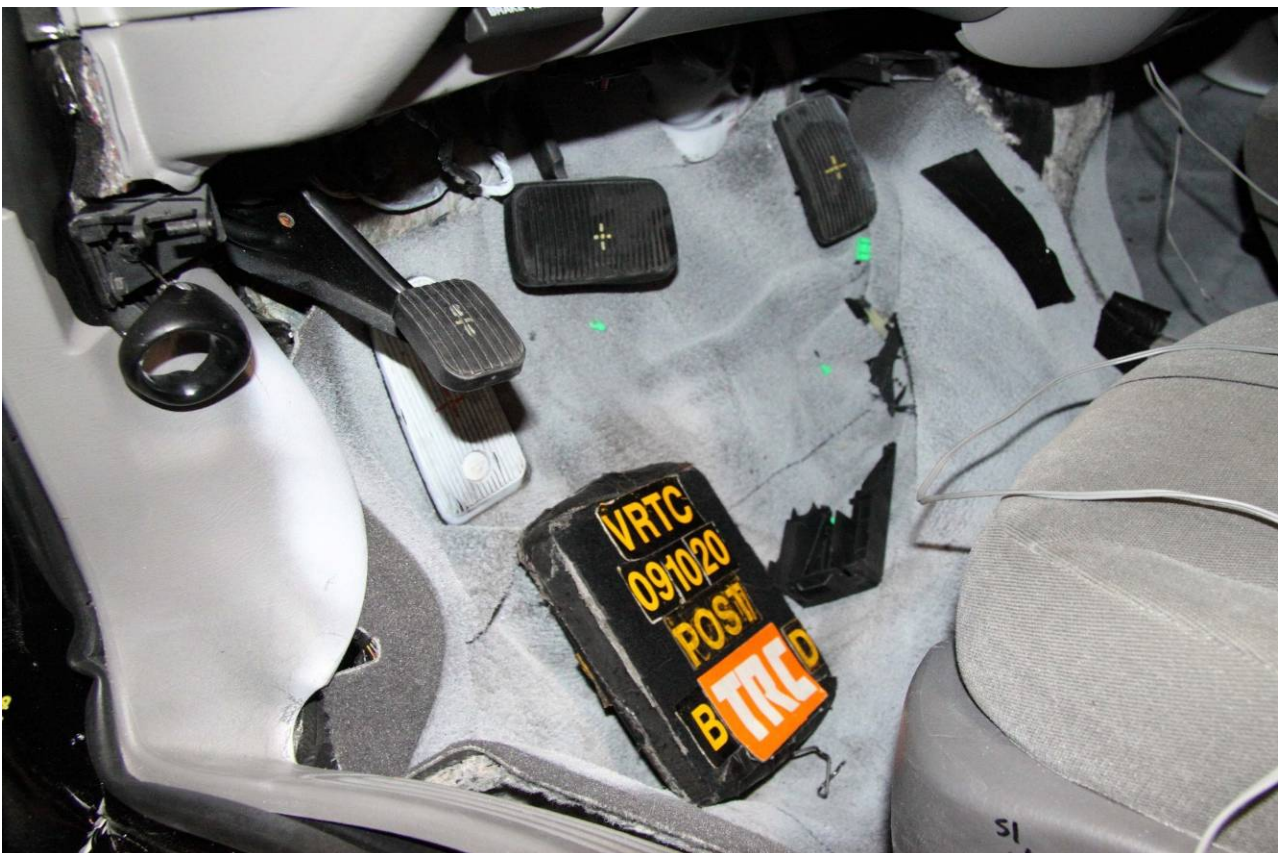
Figure A-119 Post-Test Bullet Vehicle Driver Dummy Toe board Deformation View
