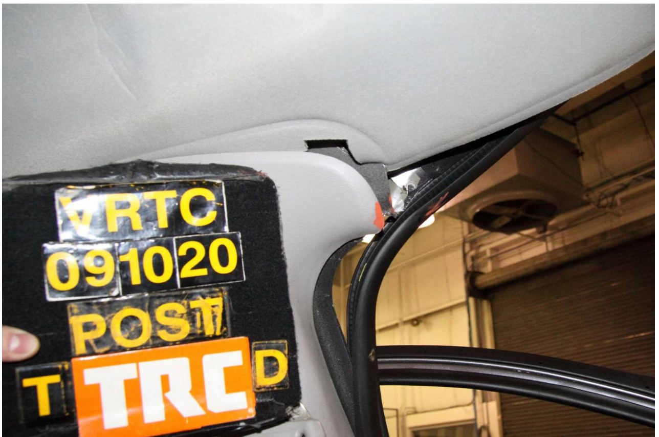
Figure A-115 Post-Test Target Vehicle Driver B-Pillar Damage View
