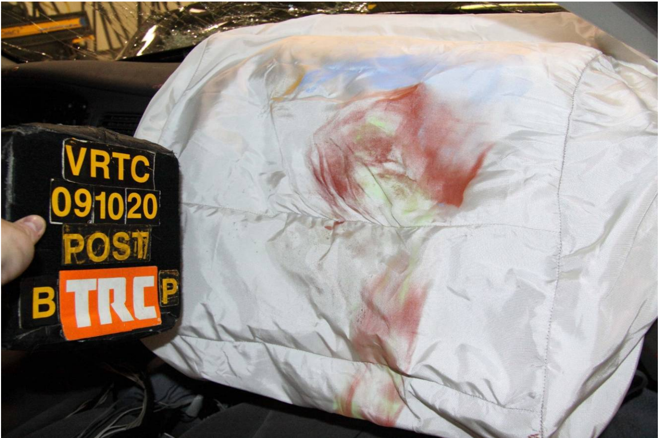
Figure A-120 Post-Test Bullet Vehicle Right Front Passenger Dummy Head Contact -View 1
