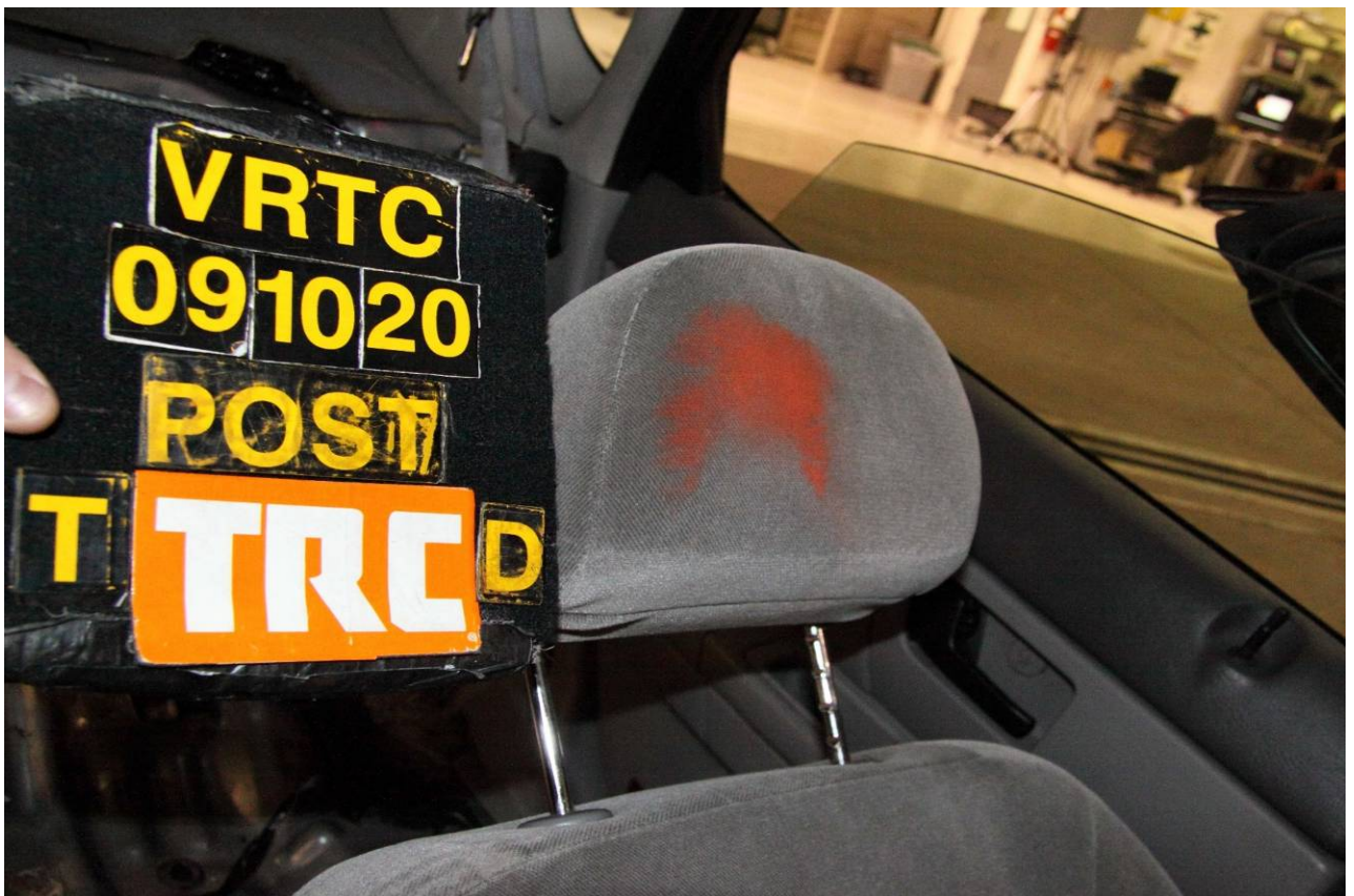
Figure A-111 Post-Test Target Vehicle Driver Dummy Head Contact - View 2
