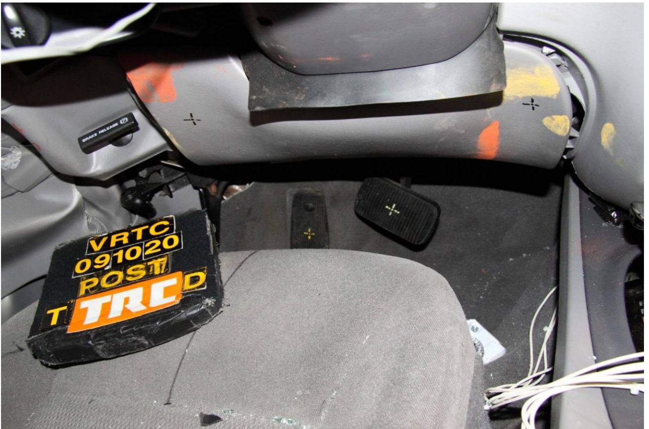
Figure A-113 Post-Test Target Vehicle Driver Dummy Knee Contact - View 2
