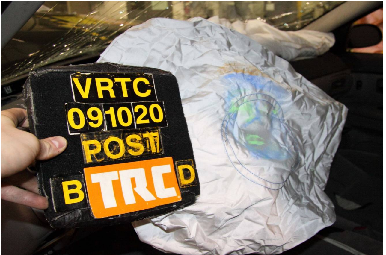
Figure A-116 Post-Test Bullet Vehicle Driver Dummy Head Contact - View 1
