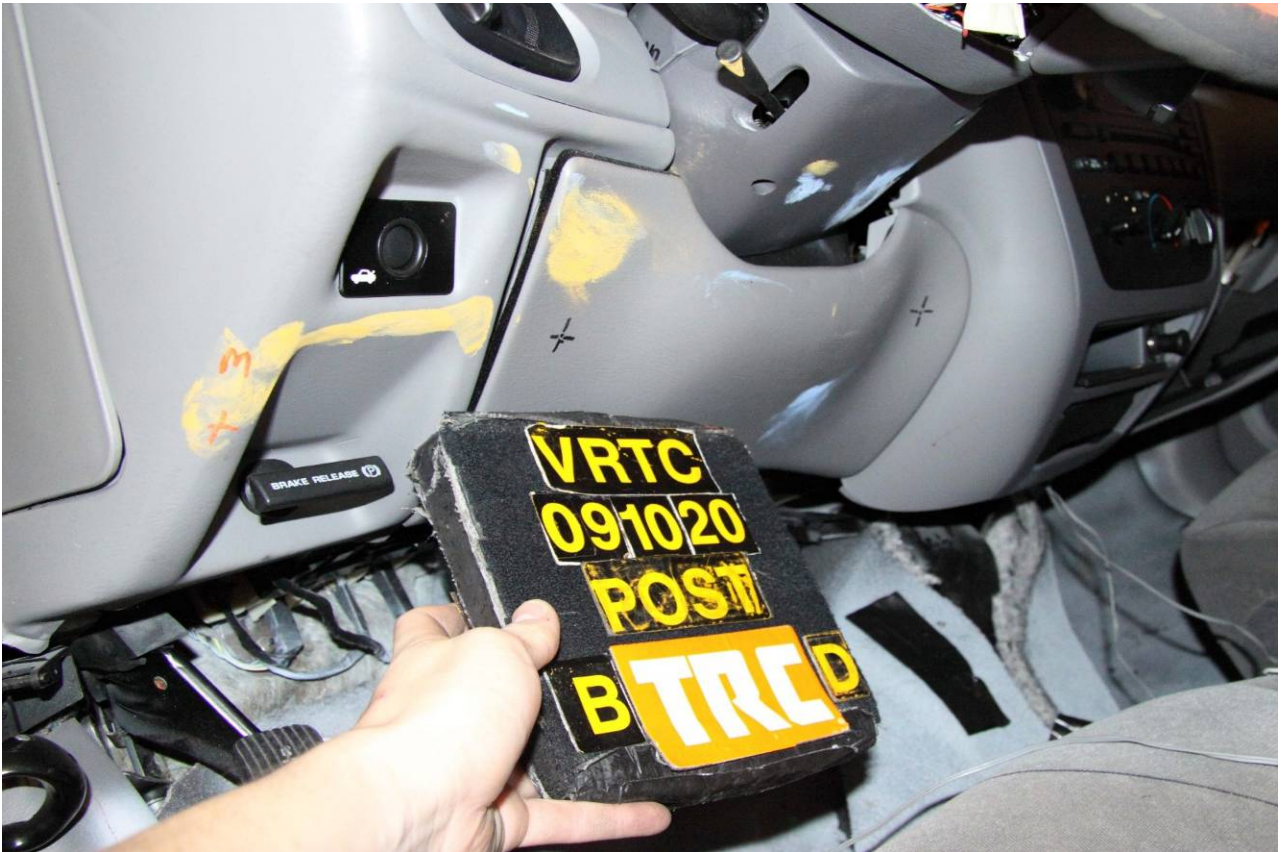
Figure A-118 Post-Test Bullet Vehicle Driver Dummy Knee Contact – View
