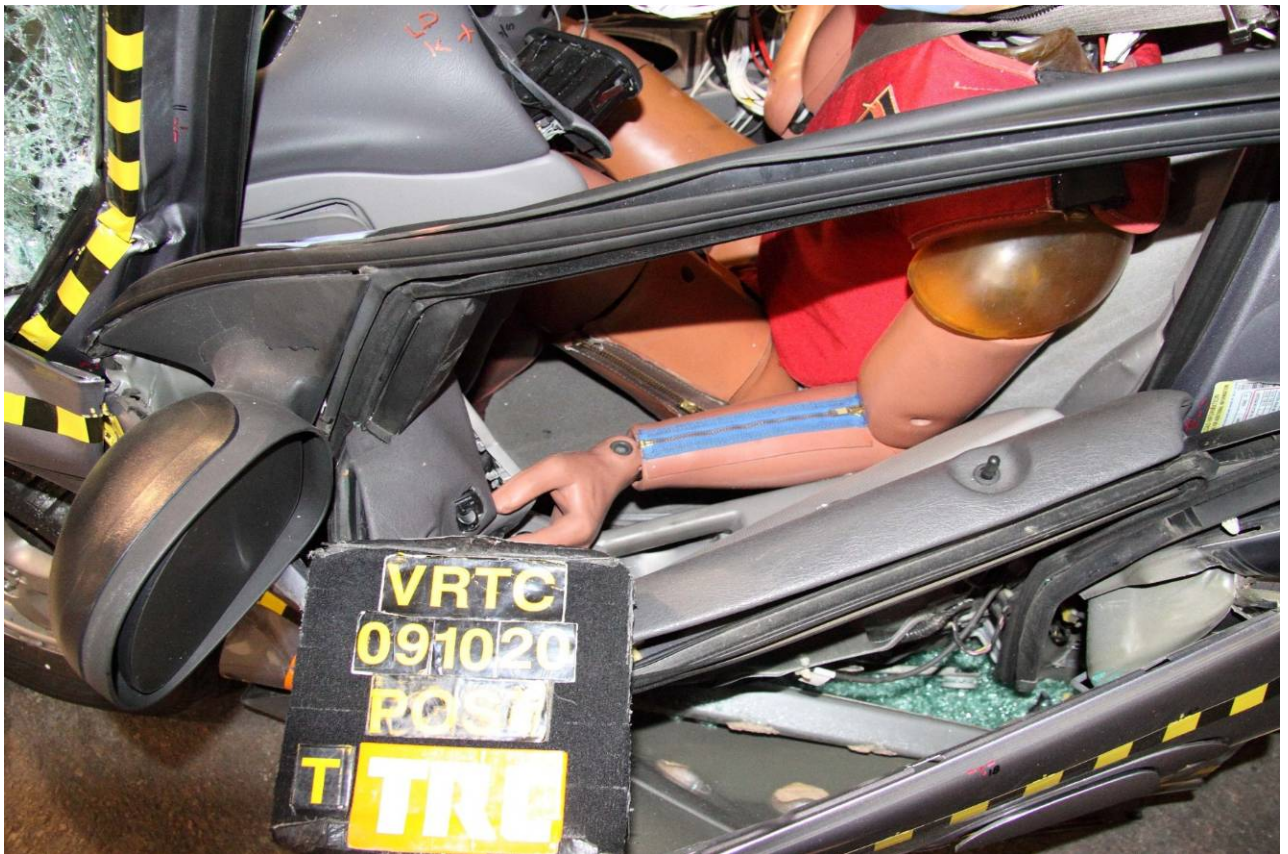
Figure A-114 Post-Test Target Vehicle Driver Door Damage View
