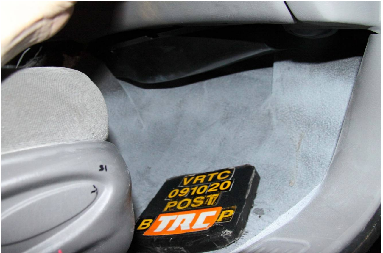
Figure A-123 Post-Test Bullet Vehicle Right Front Passenger Dummy Toe Board Deformation View
