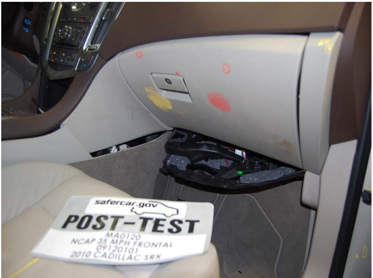
Post-Test Passenger Dummy Knee Contact
