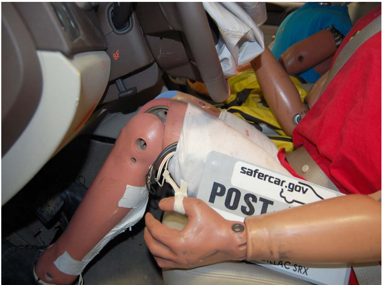
Post-Test Driver Side Knee Bolster
