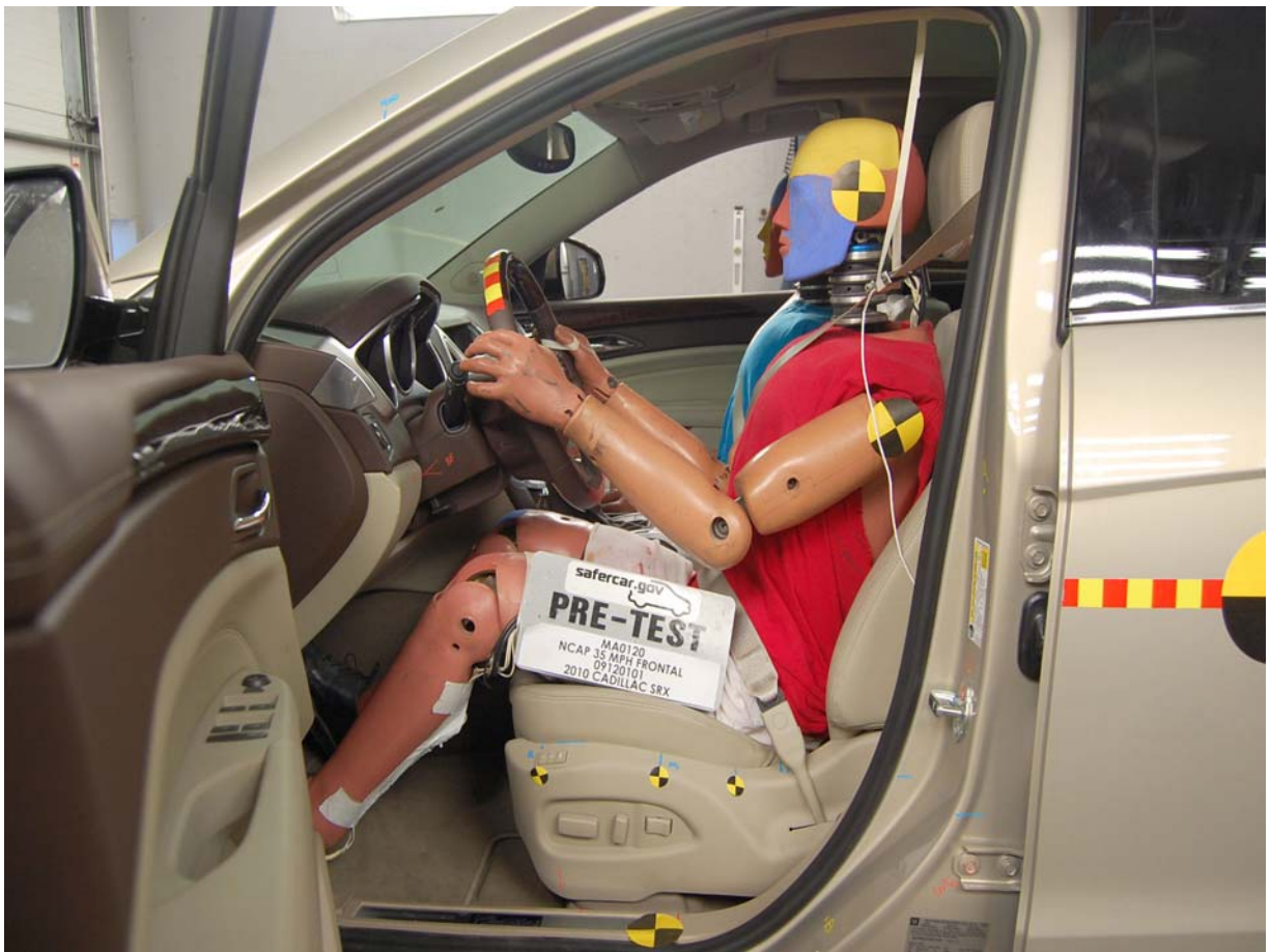
Pre-Test Driver Dummy (Door Open)
