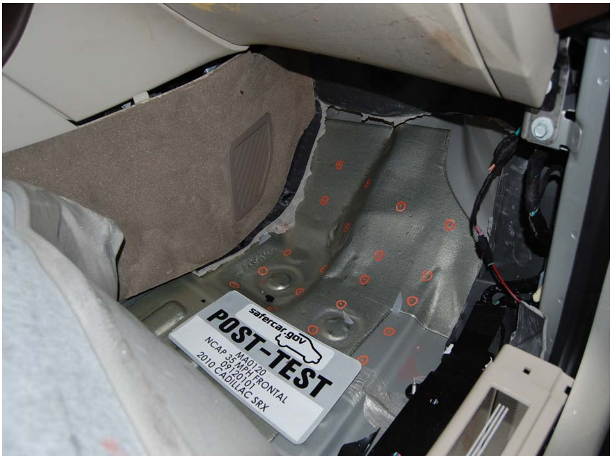
Post-Test Passenger Side Floor Pan
