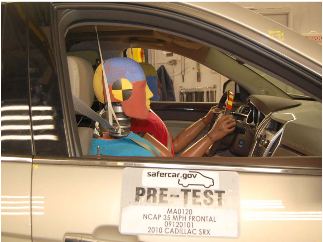
Pre-Test Passenger Dummy (Through Window)
