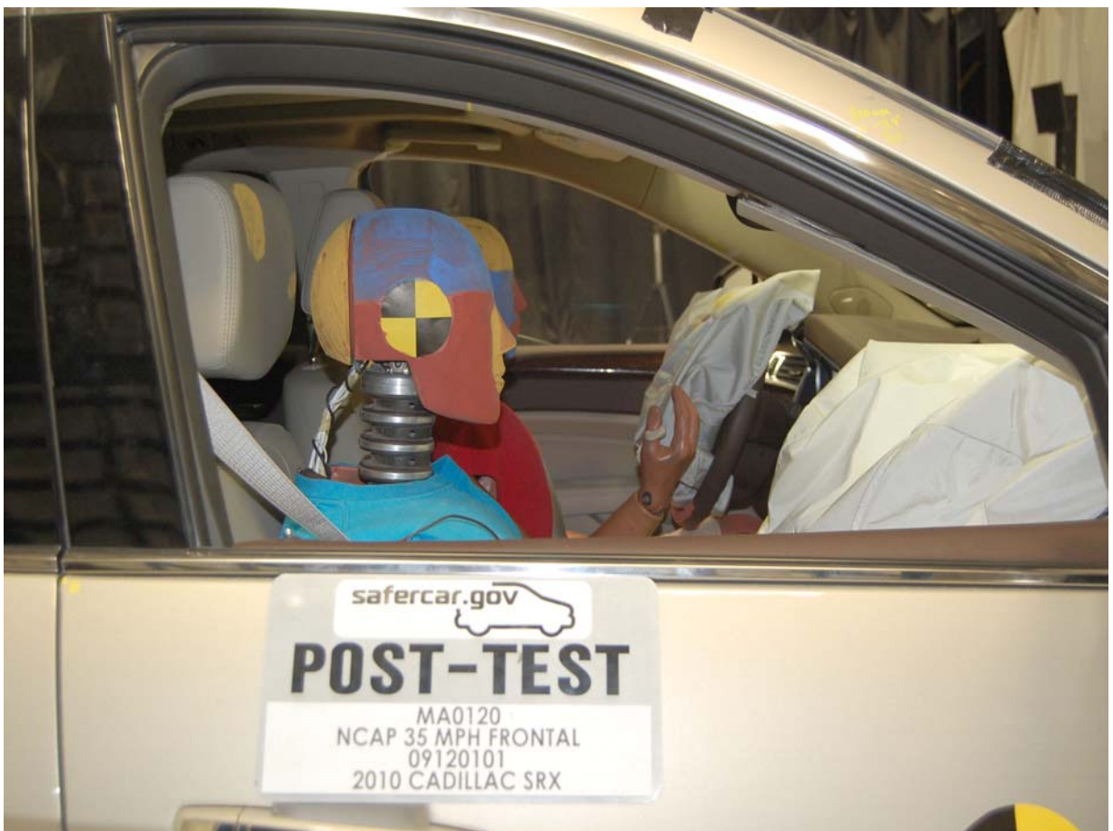
Post-Test Passenger Dummy (Through Window)
