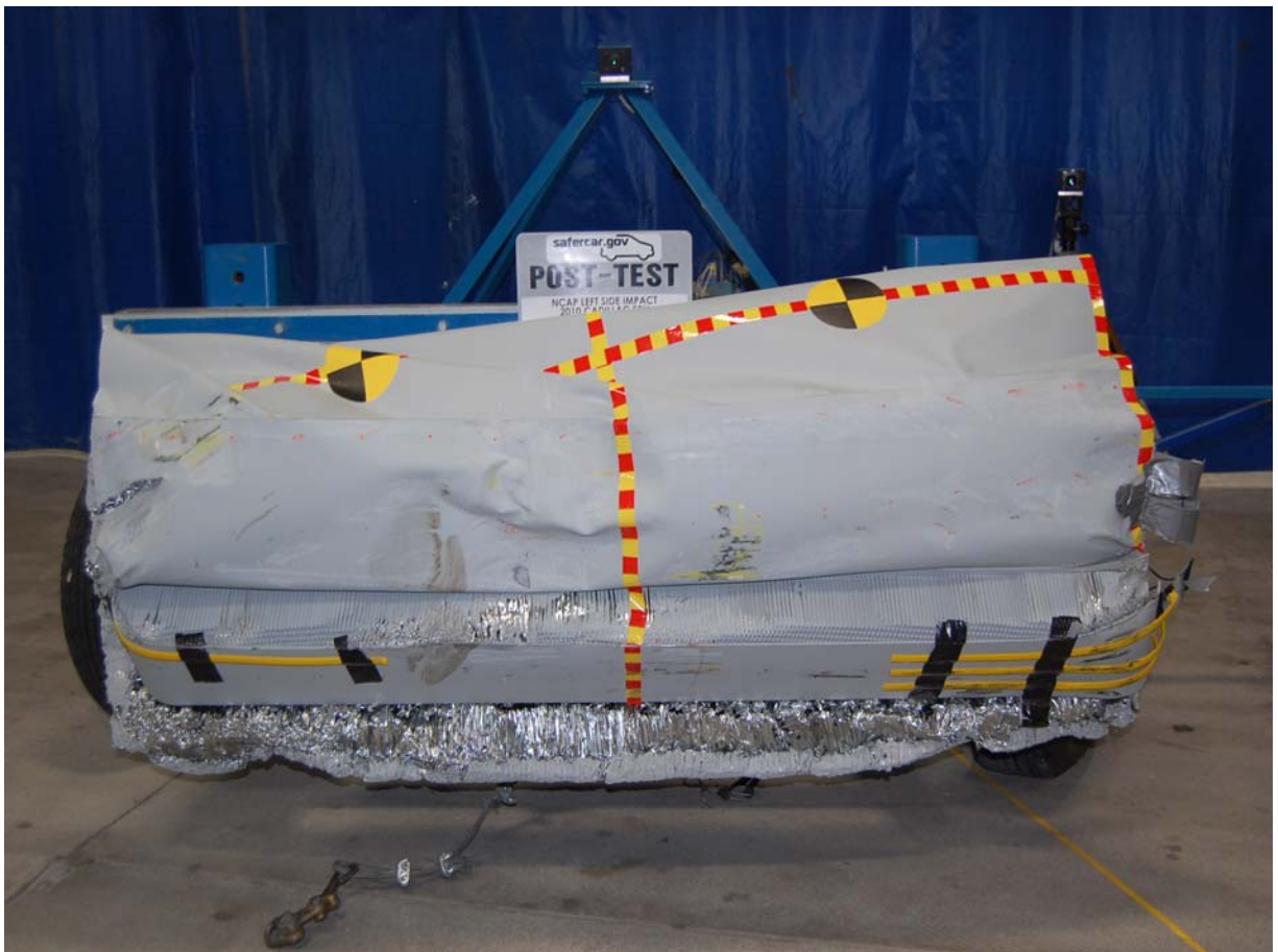
Post-Test Front View of Deformable Barrier
