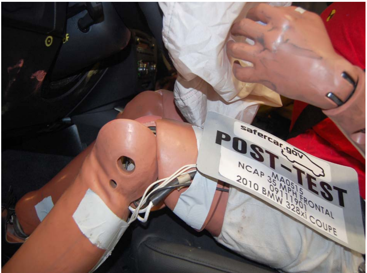
Post-Test Driver Side Knee Bolster
