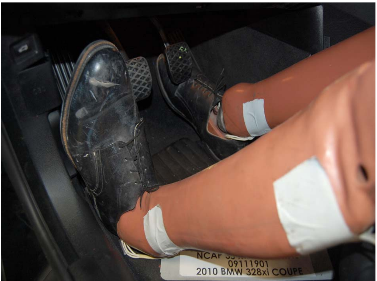
Post-Test Driver Dummy Feet
