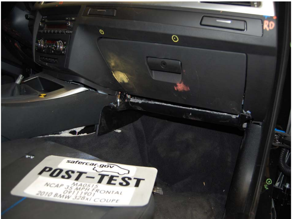
Post-Test Passenger Dummy Knee Contact
