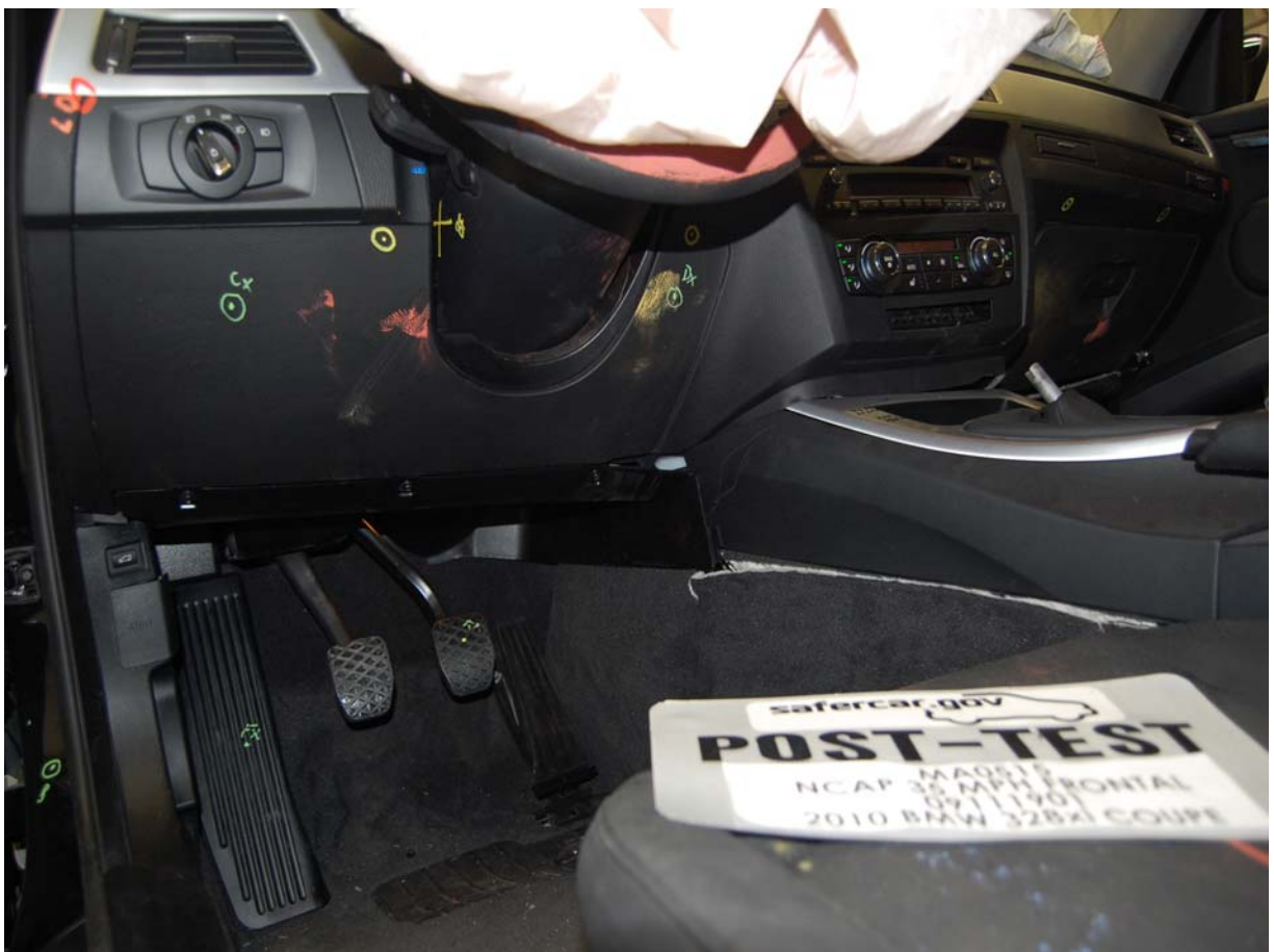
Post-Test Driver Dummy Knee Contact
