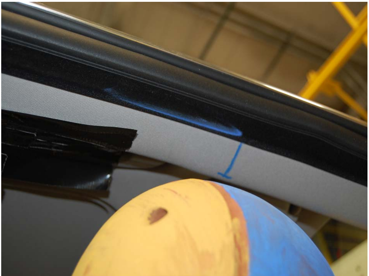
Post-Test Passenger Dummy Head Contact
