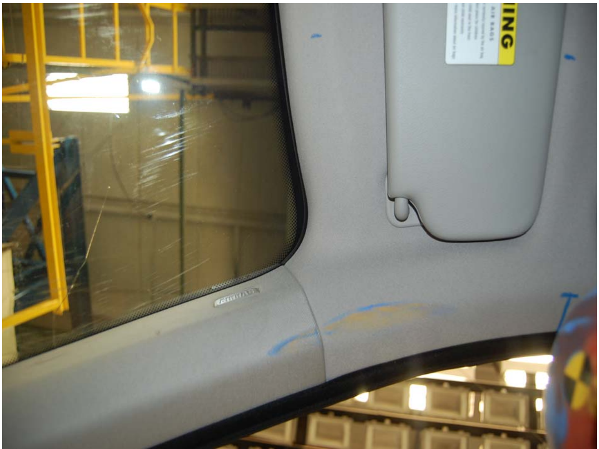
Post-Test Passenger Dummy Head Contact
