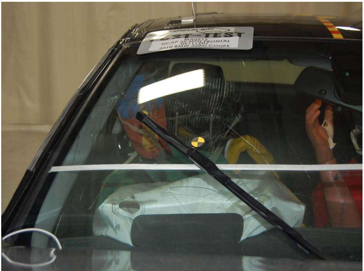
Post-Test Passenger Dummy Front View (Head Position)
