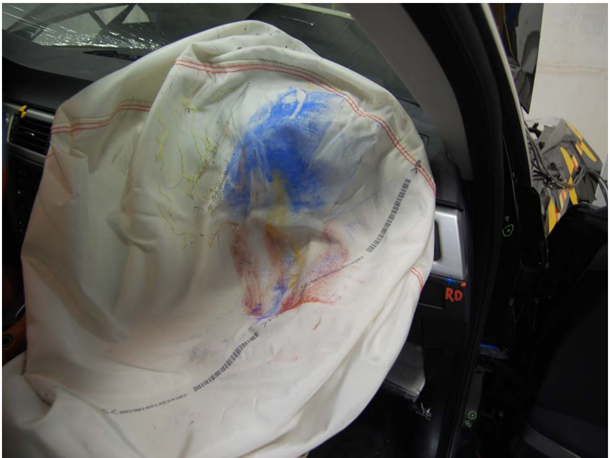
Post-Test Passenger Dummy Airbag Contact
