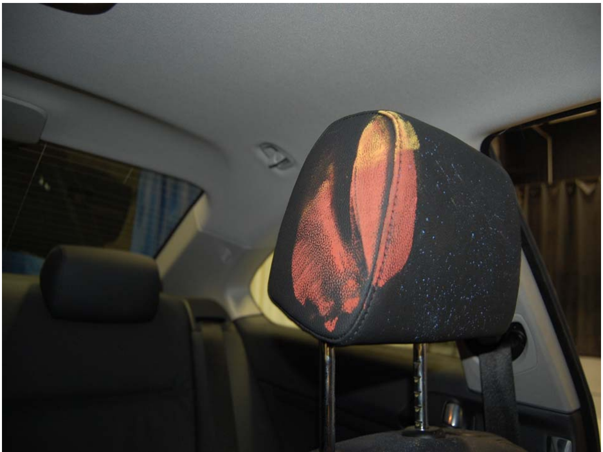
Post-Test Driver Dummy Head Contact
