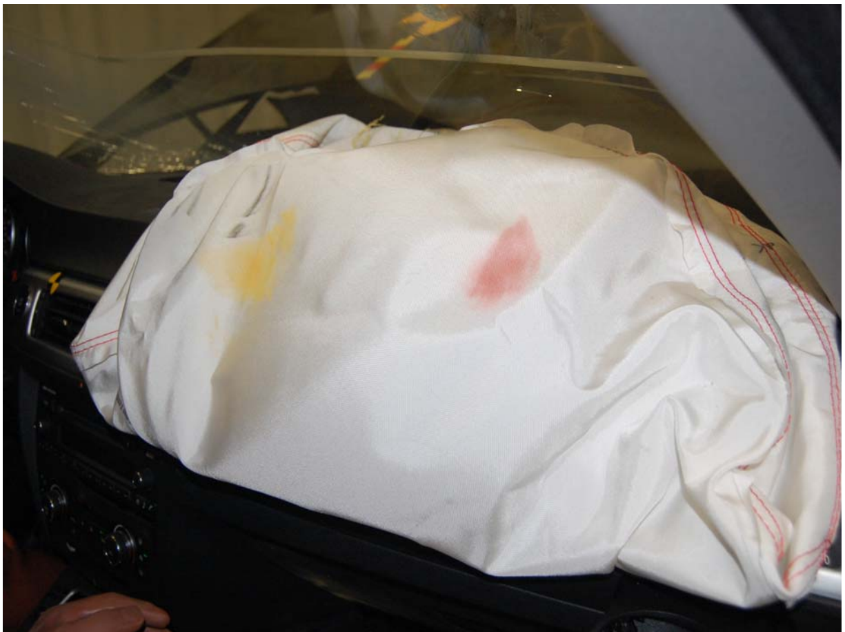
Post-Test Passenger Dummy Knee Contact w/Airbag
