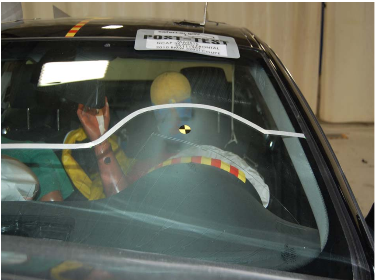
Post-Test Driver Dummy Front View (Head Position)
