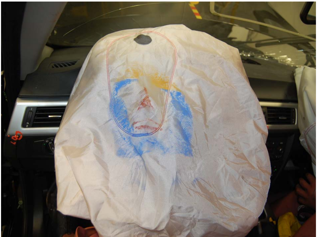
Post-Test Driver Dummy Airbag Contact
