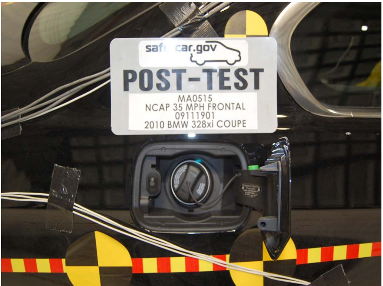
Post-Test Fuel Cap View
