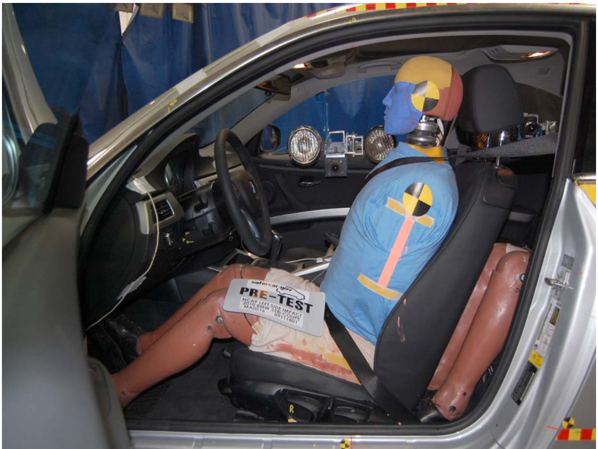
Pre-Test Driver Dummy (Door Open)
