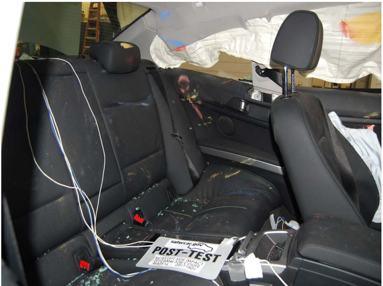
Post-Test Passenger Dummy Contact
