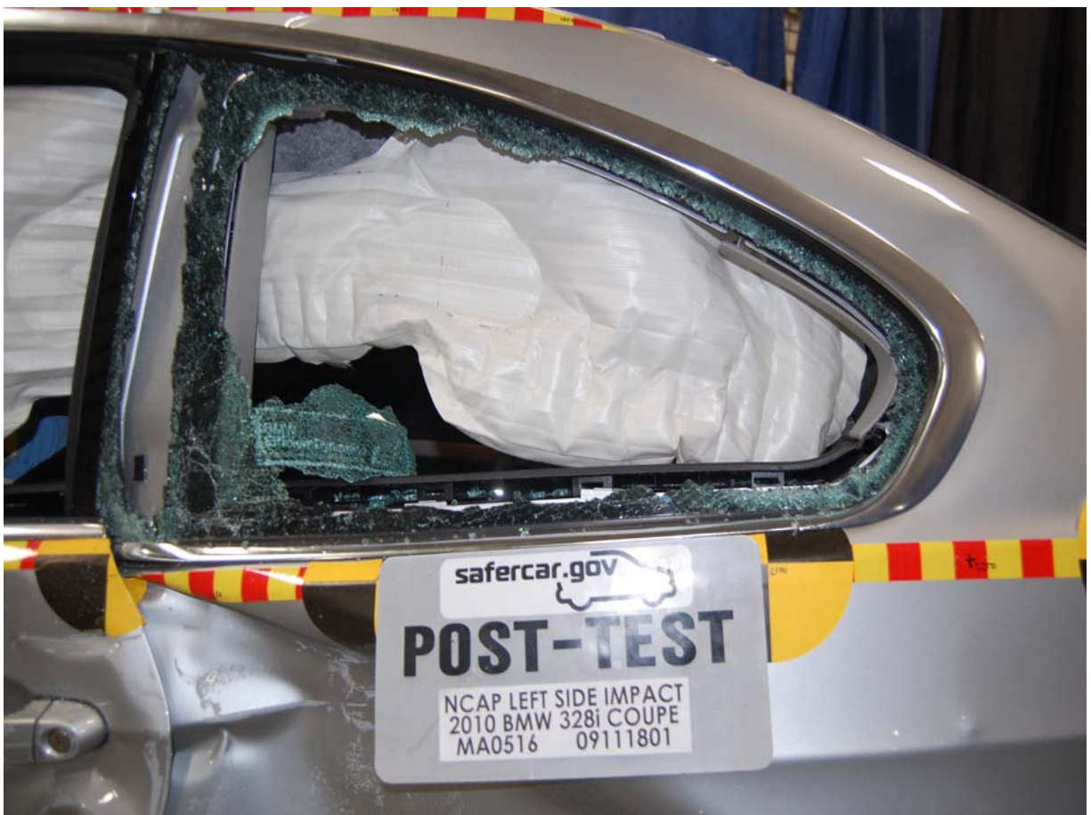
Post-Test Passenger Dummy (Through Window)
