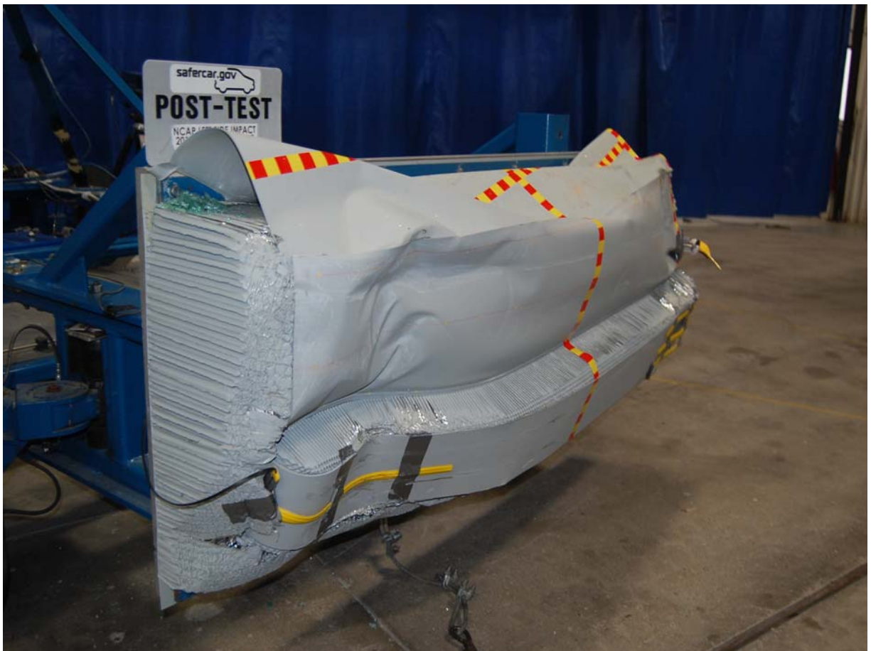
Post-Test Right Side View of Deformable Barrier
