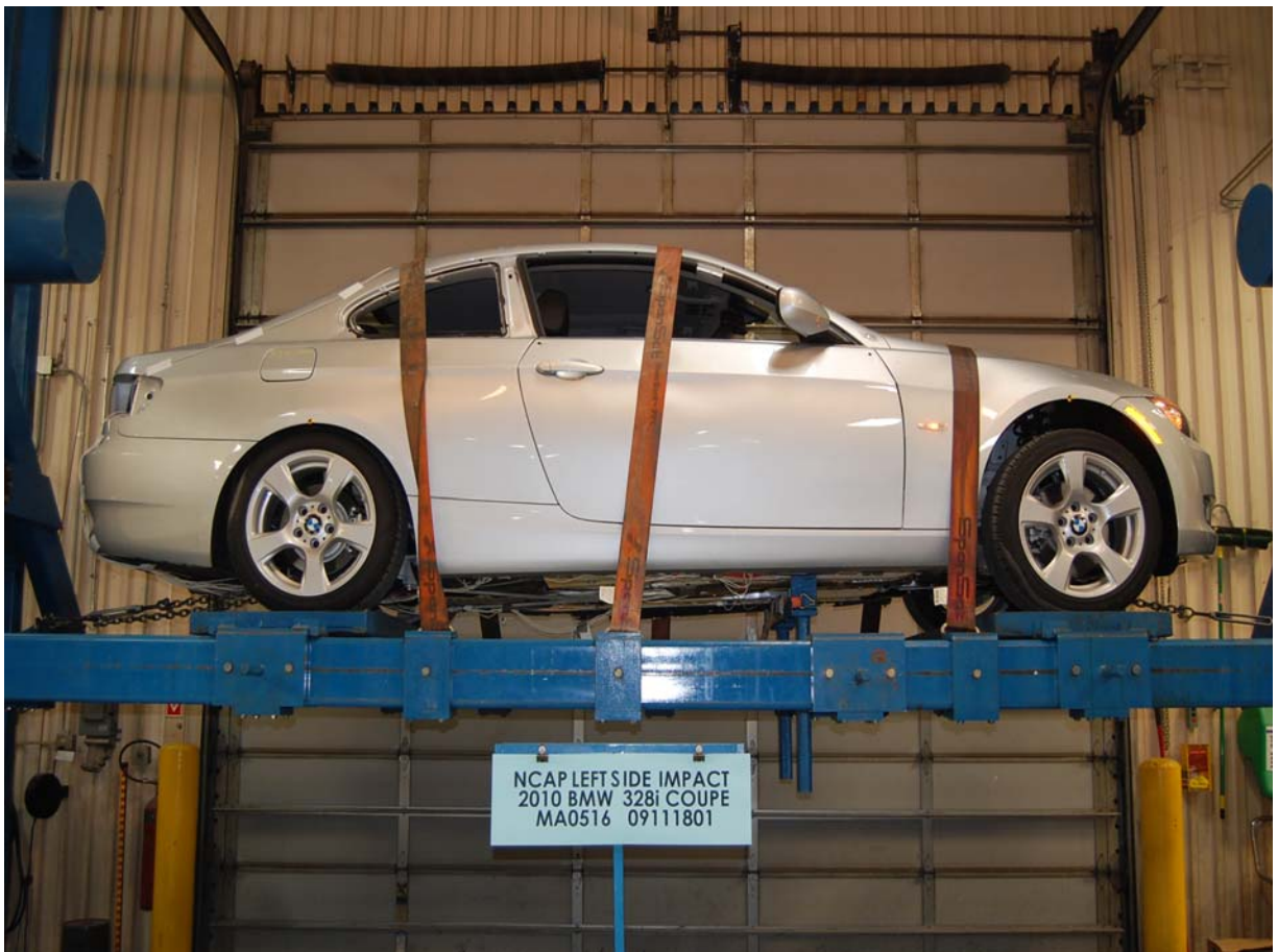
Vehicle on Rollover Device (360 Degrees)
