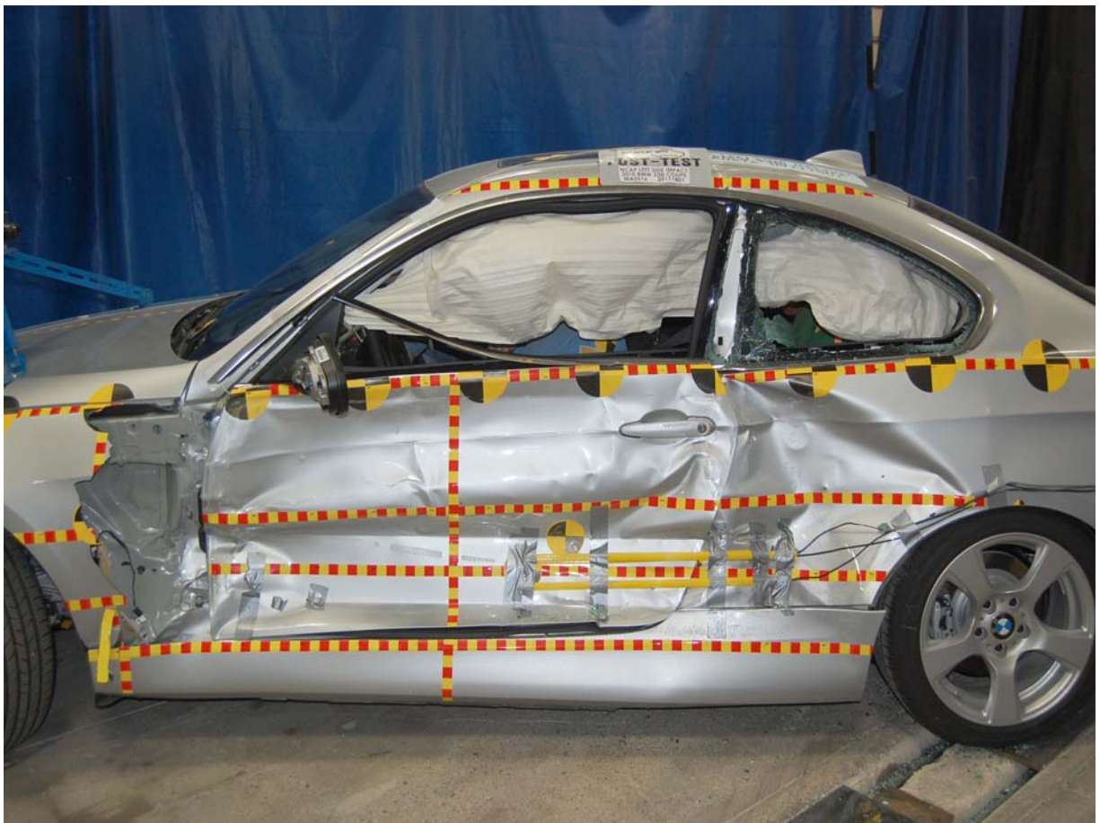
Post-Test Left Side Impact Close-up
