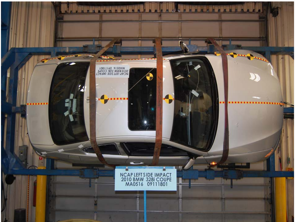
Vehicle on Rollover Device (90 Degrees)
