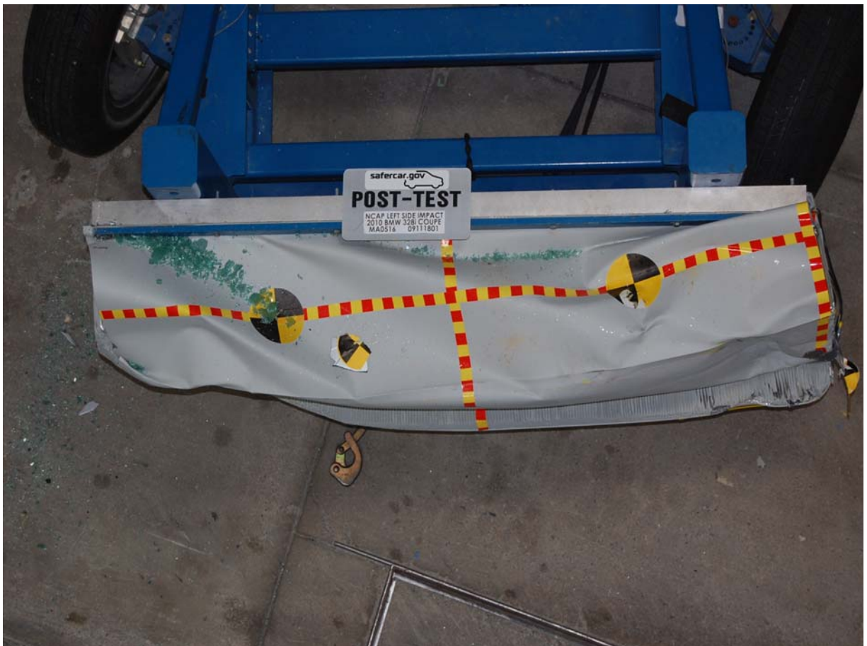
Post-Test Top View of Deformable Barrier
