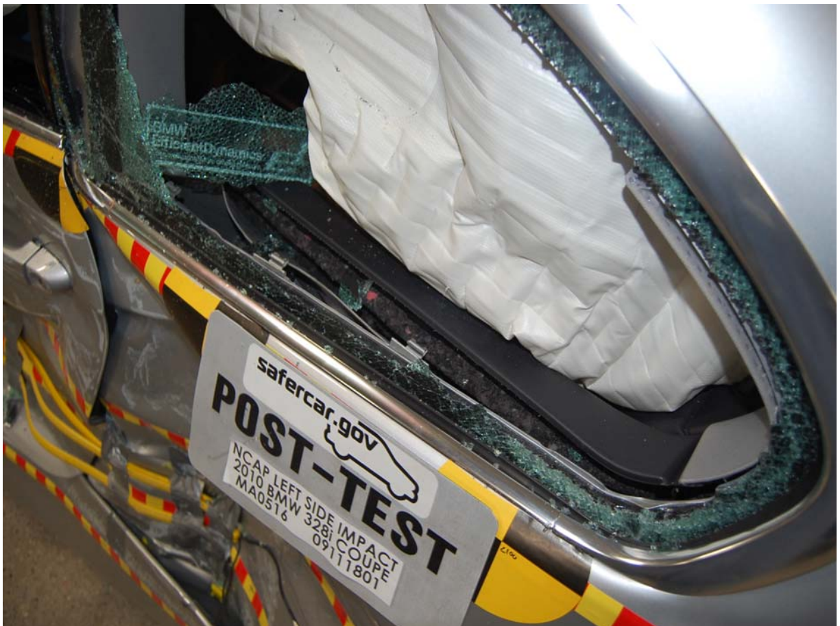
Post-Test Passenger Dummy Clearance From Door
