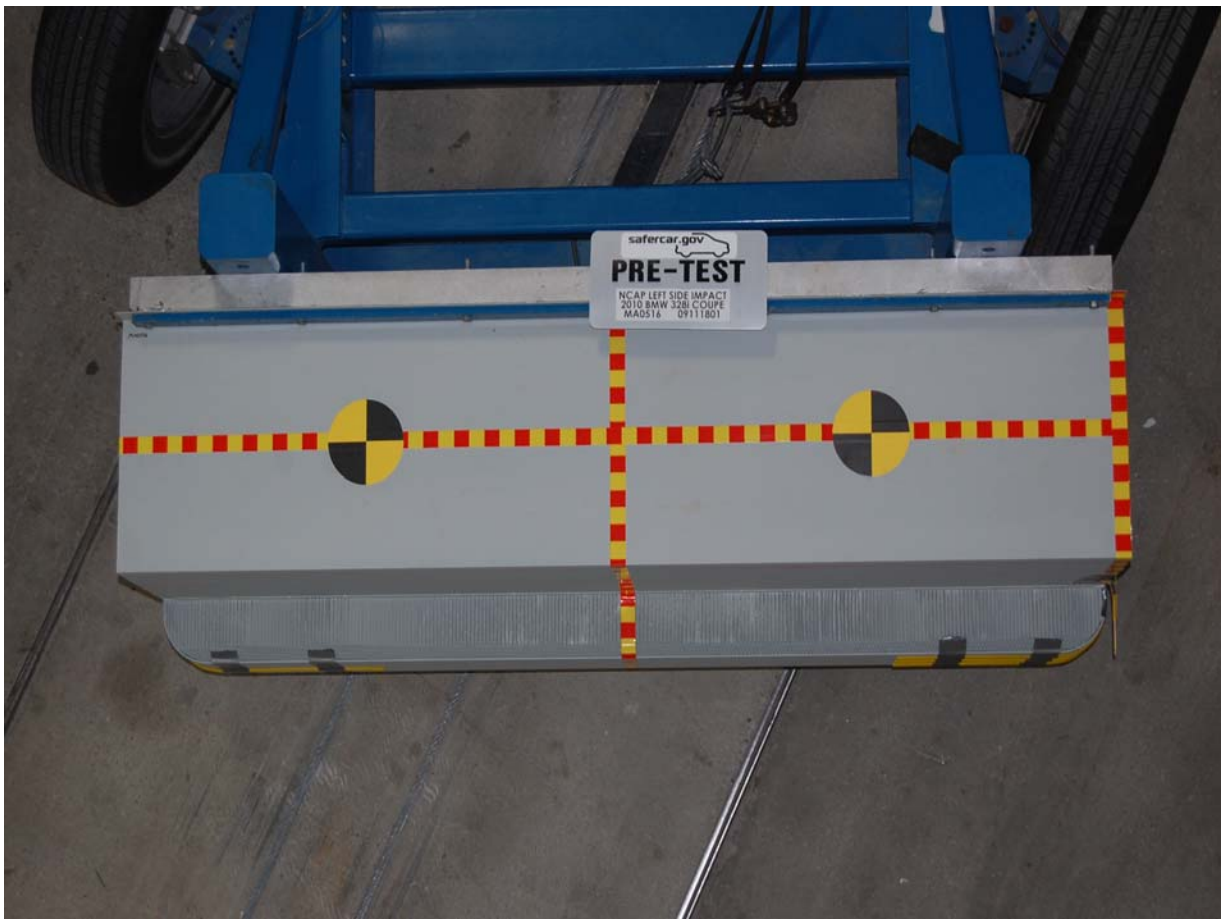
Pre-Test Top View of Deformable Barrier
