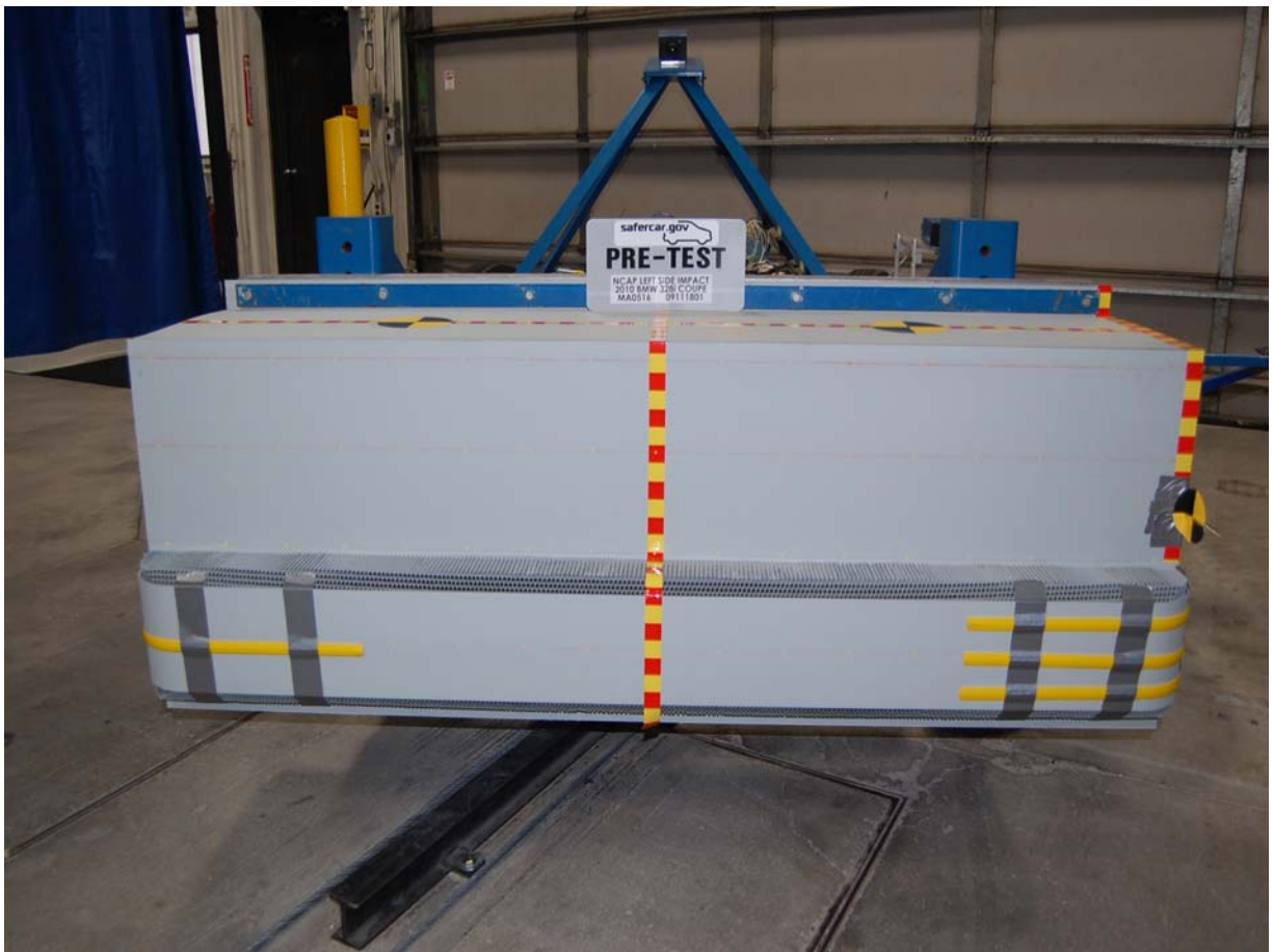
Pre-Test Front View of Deformable Barrier
