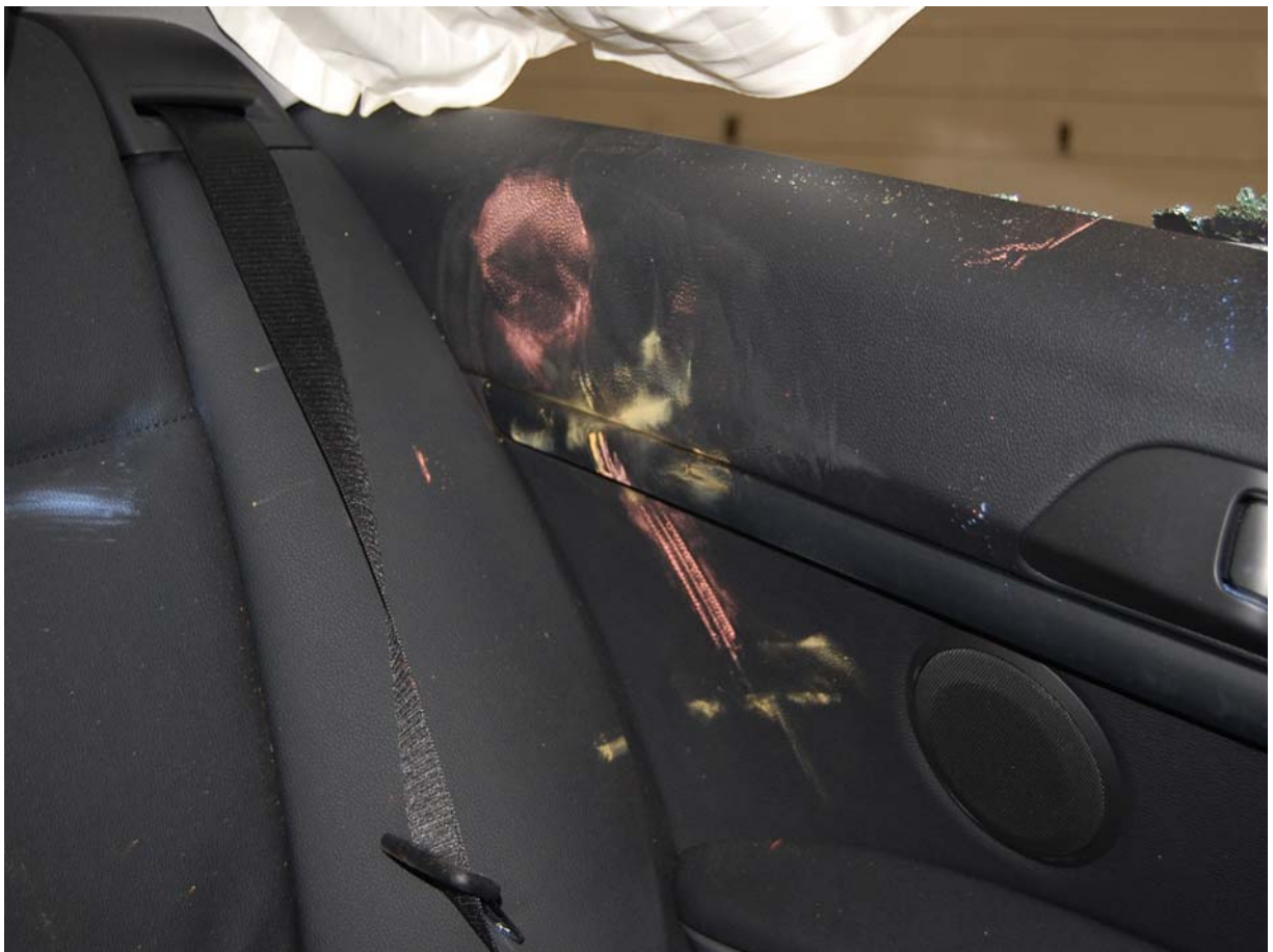
Post-Test Passenger Dummy Upper Torso Contact
