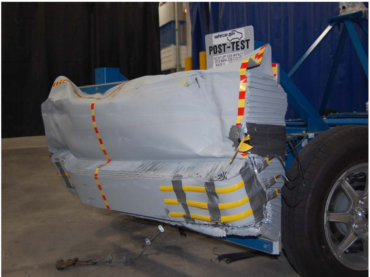
Post-Test Left Side View of Deformable Barrier
