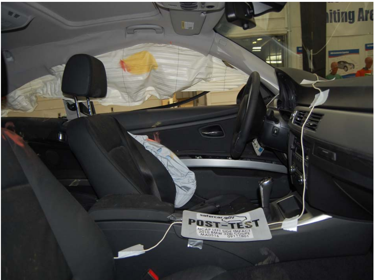
Post-Test Driver Dummy Contact
