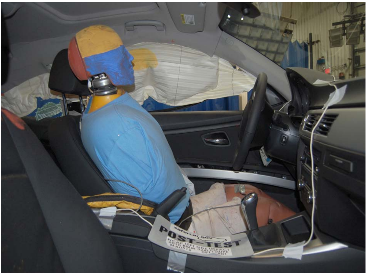
Post-Test Driver Dummy Right Side View
