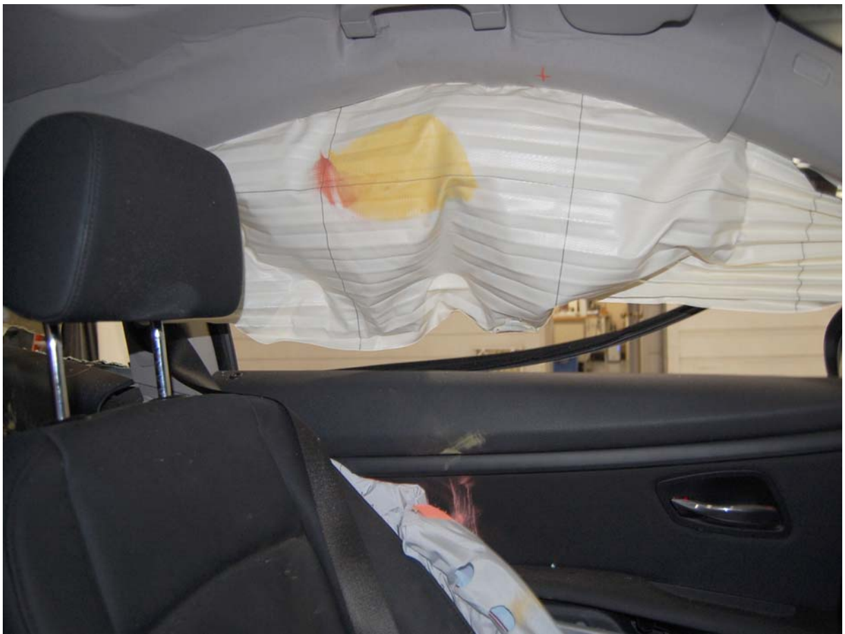
Post-Test Driver Dummy Head Contact View
