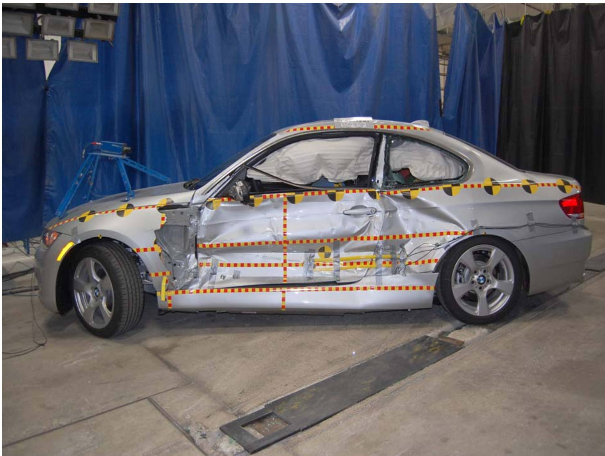
Post-Test Left Side View
