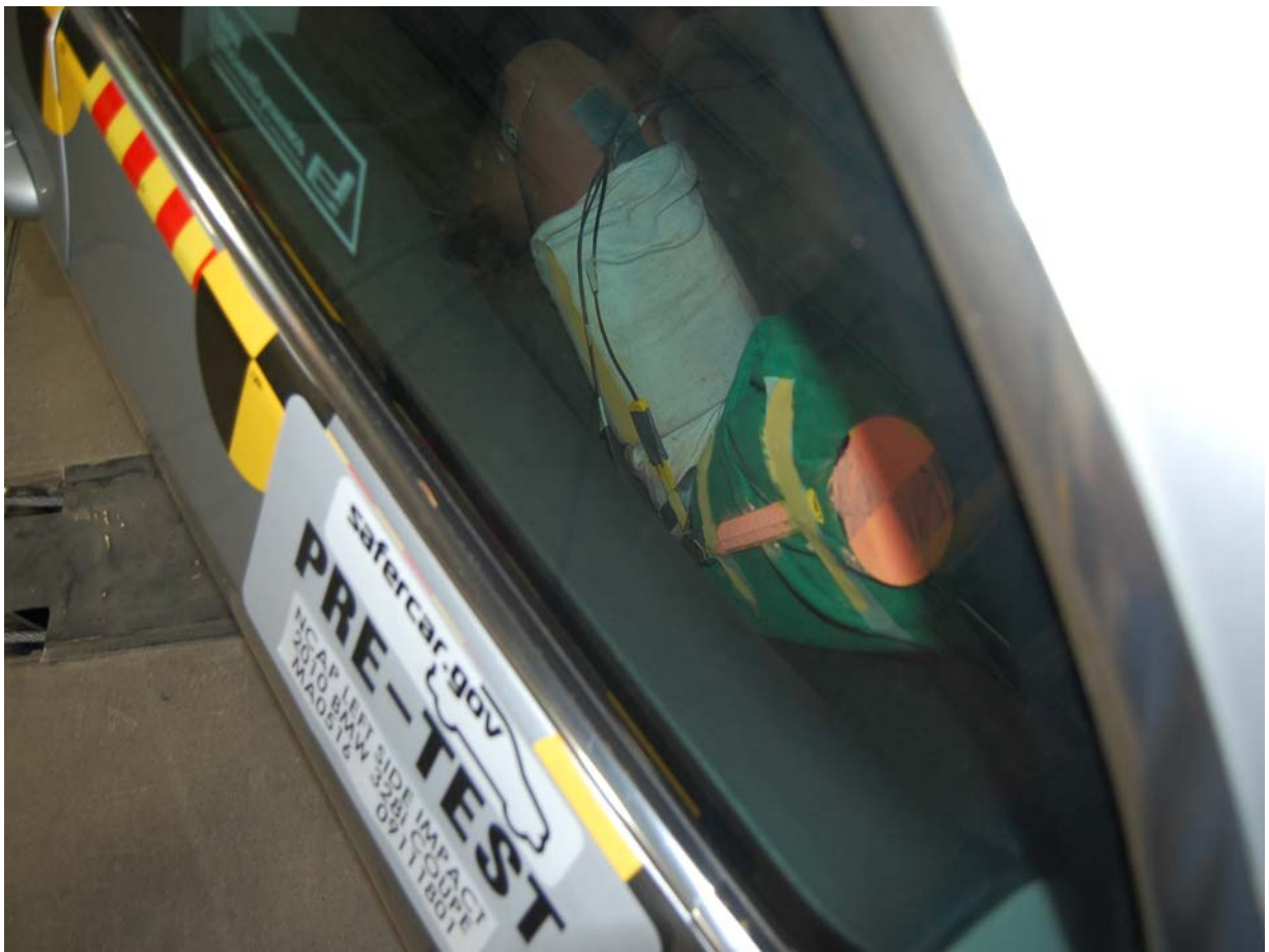
Pre-Test Passenger Dummy Clearance From Door
