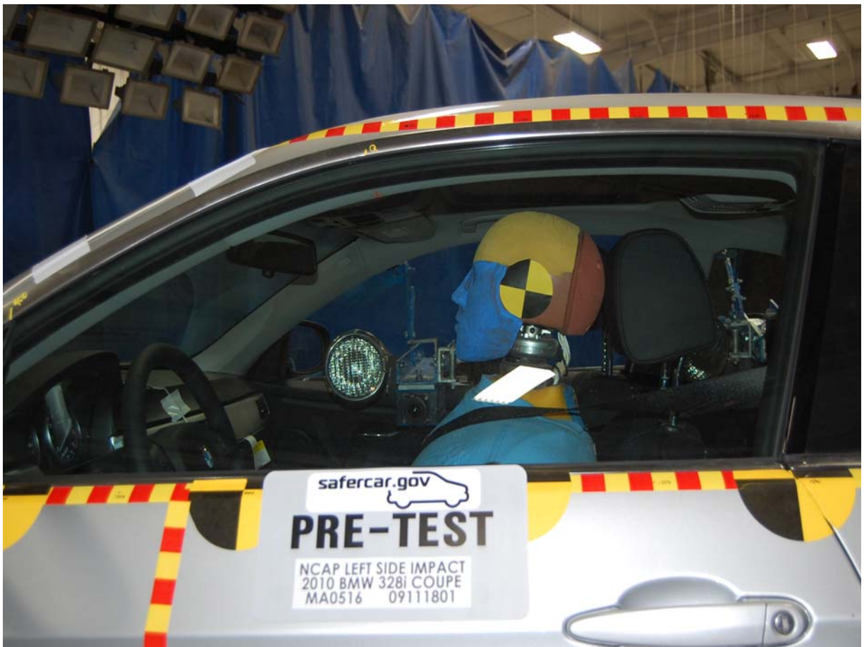
Pre-Test Driver Dummy (Through Window)
