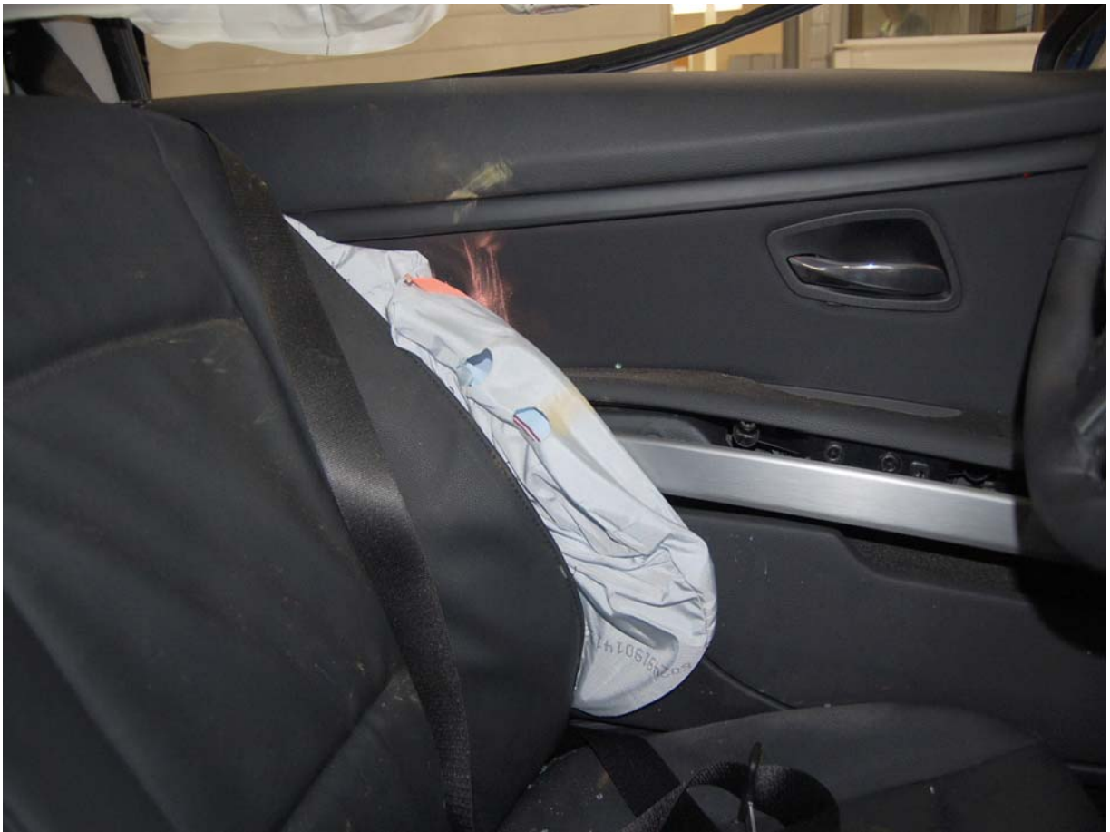
Post-Test Driver Dummy Torso Contact
