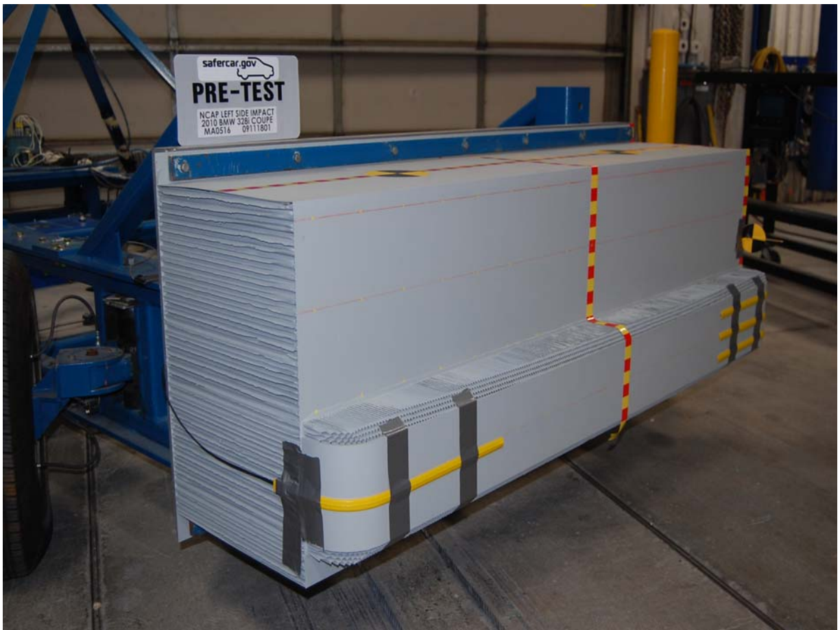
Pre-Test Right Side View of Deformable Barrier
