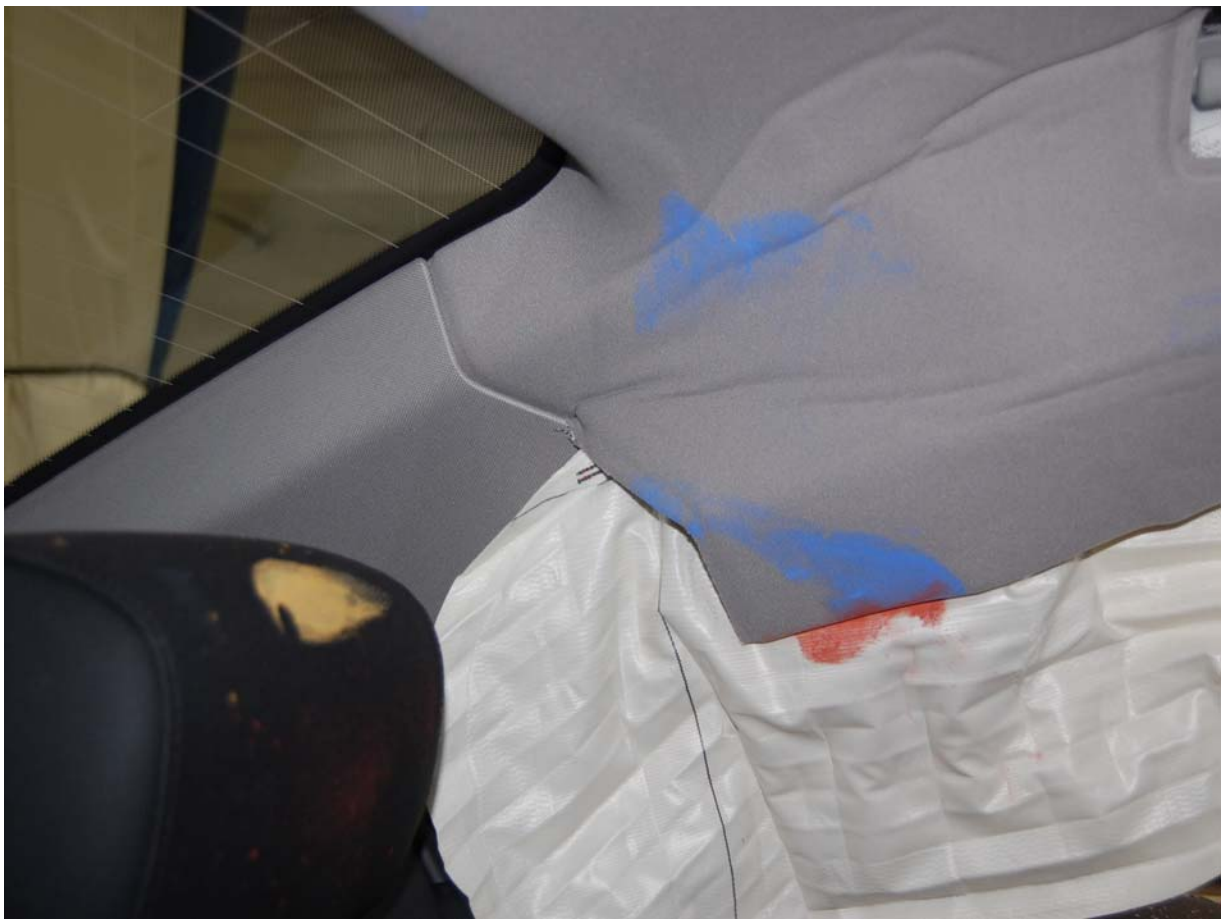
Post-Test Passenger Dummy Head Contact View
