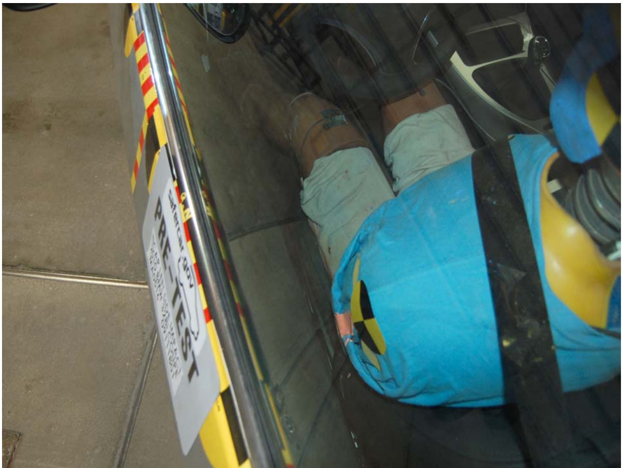
Pre-Test Driver Dummy Clearance From Door
