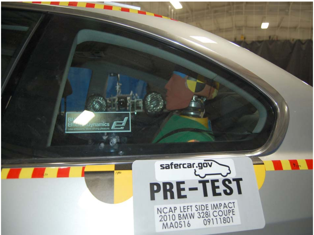
Pre-Test Passenger Dummy (Through Window)
