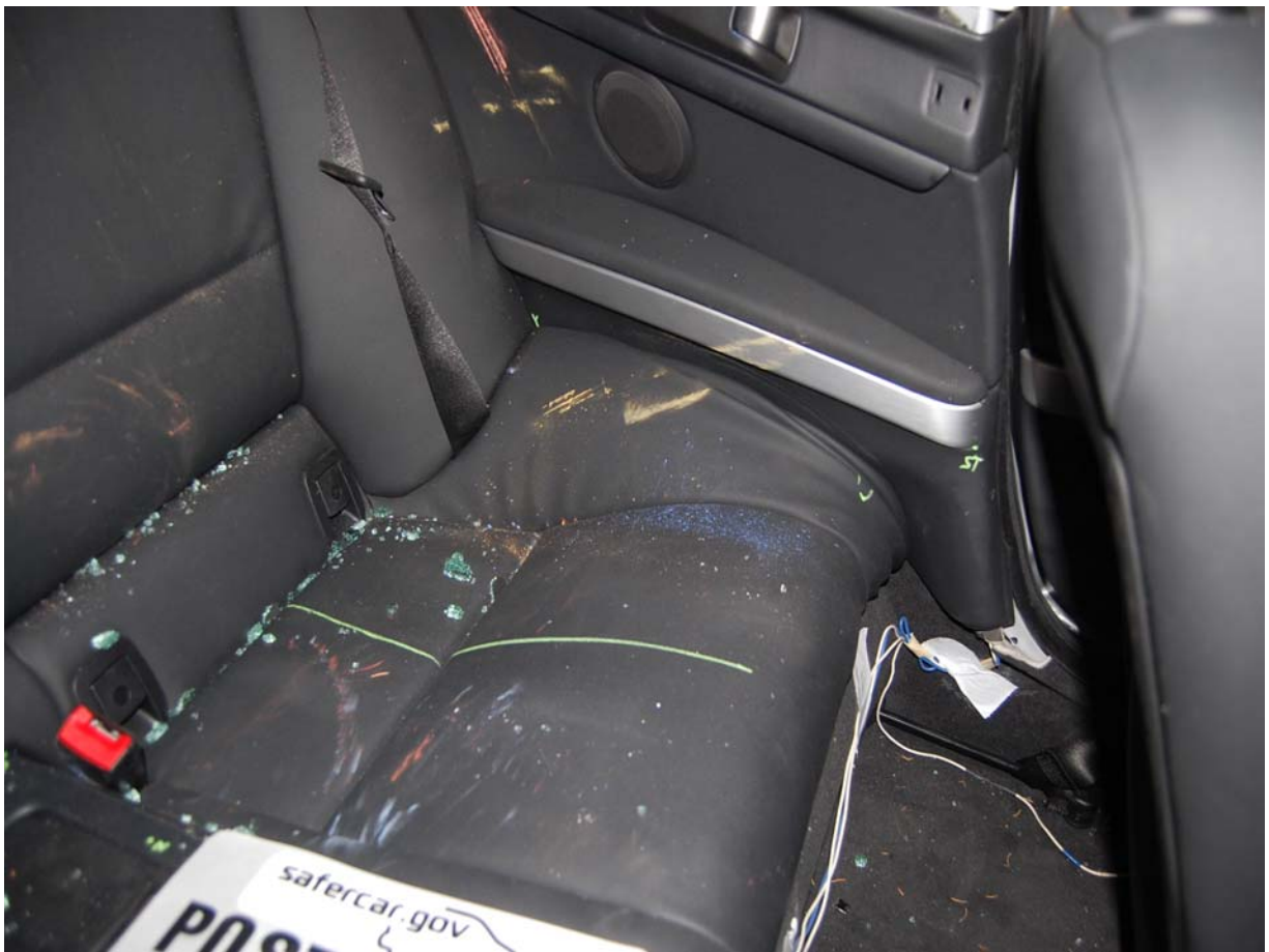
Post-Test Passenger Dummy Lower Torso Contact
