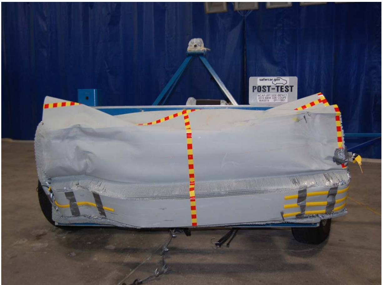
Post-Test Front View of Deformable Barrier
