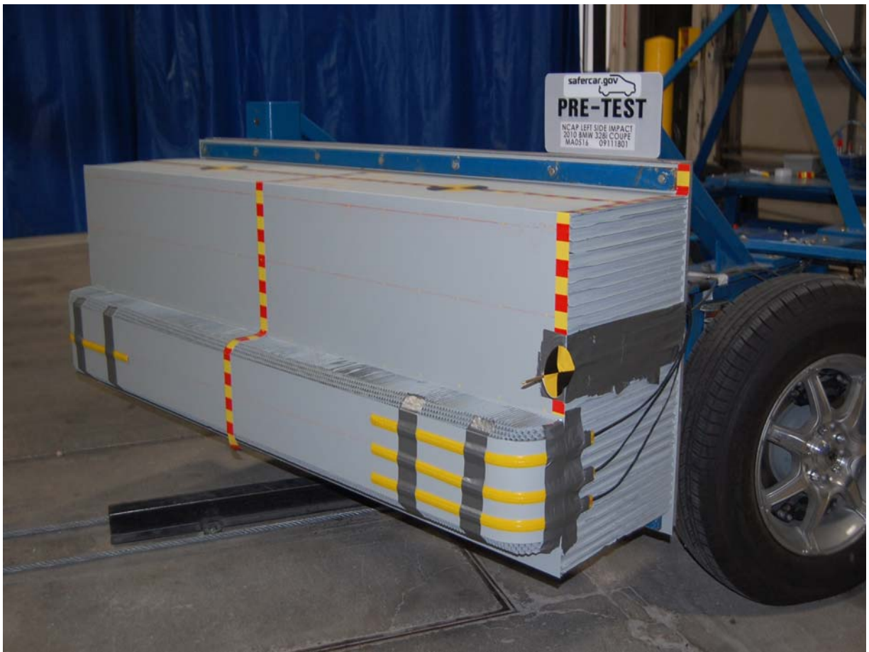
Pre-Test Left Side View of Deformable Barrier
