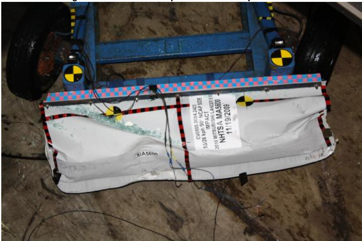
Figure A-28: Post-Test Top View of MDB Impactor Face
