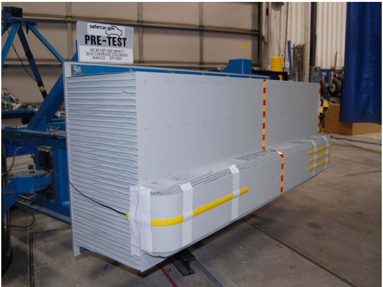
Pre-Test Right Side View of Deformable Barrier
