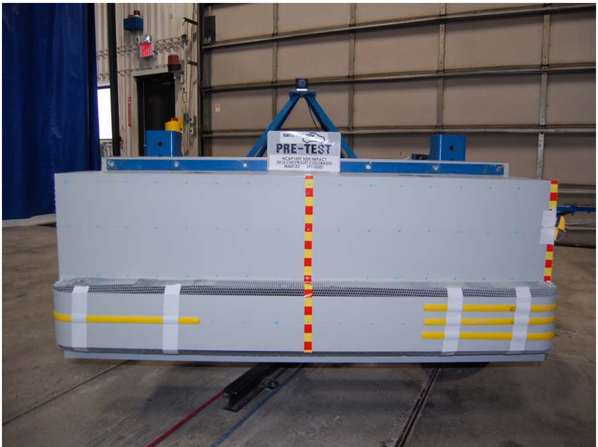
Pre-Test Front View of Deformable Barrier
