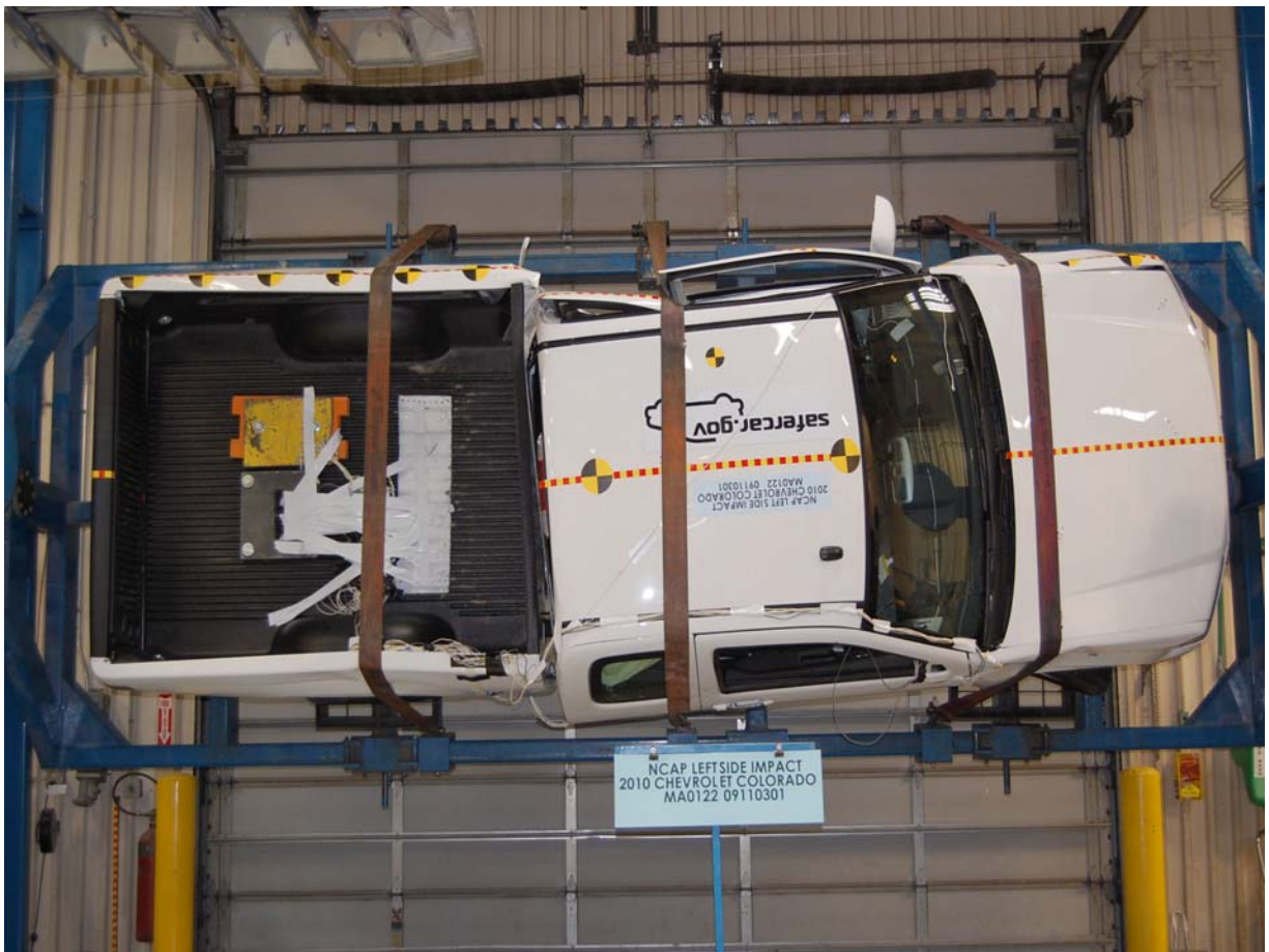
Vehicle on Rollover Device (270 Degrees)
