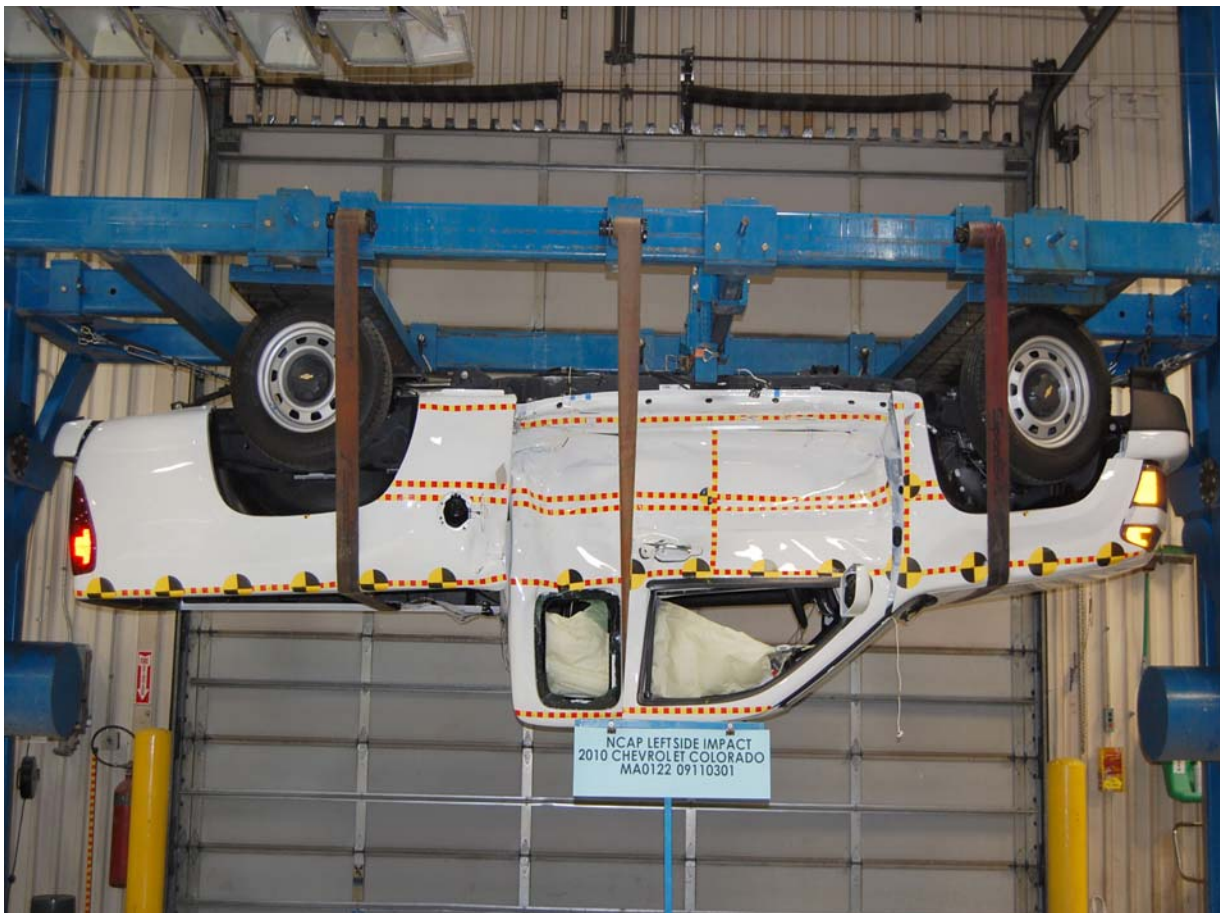
Vehicle on Rollover Device (180 Degrees)
