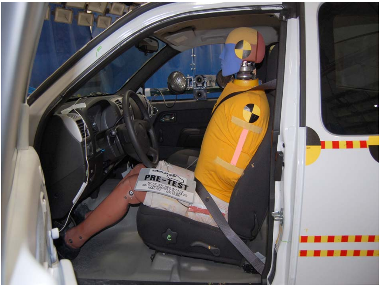
Pre-Test Driver Dummy (Door Open)
