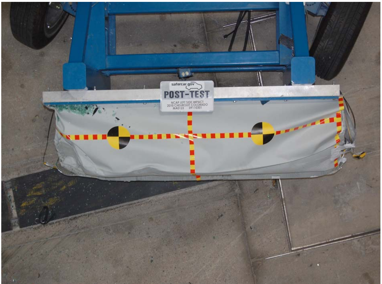
Post-Test Top View of Deformable Barrier
