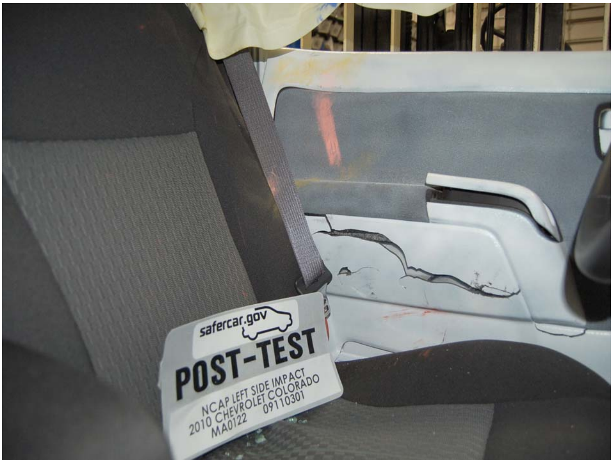
Post-Test Driver Dummy Torso Contact
