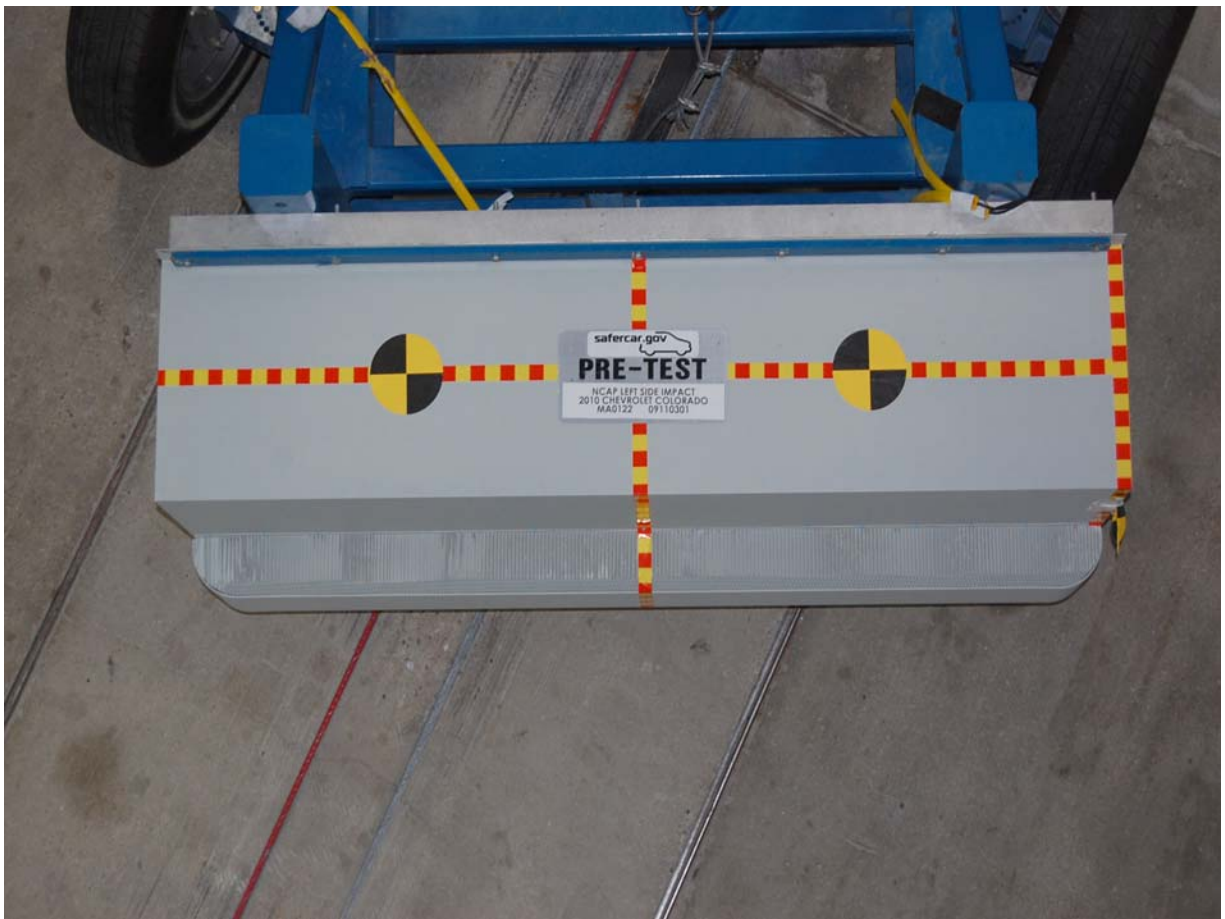
Pre-Test Top View of Deformable Barrier
