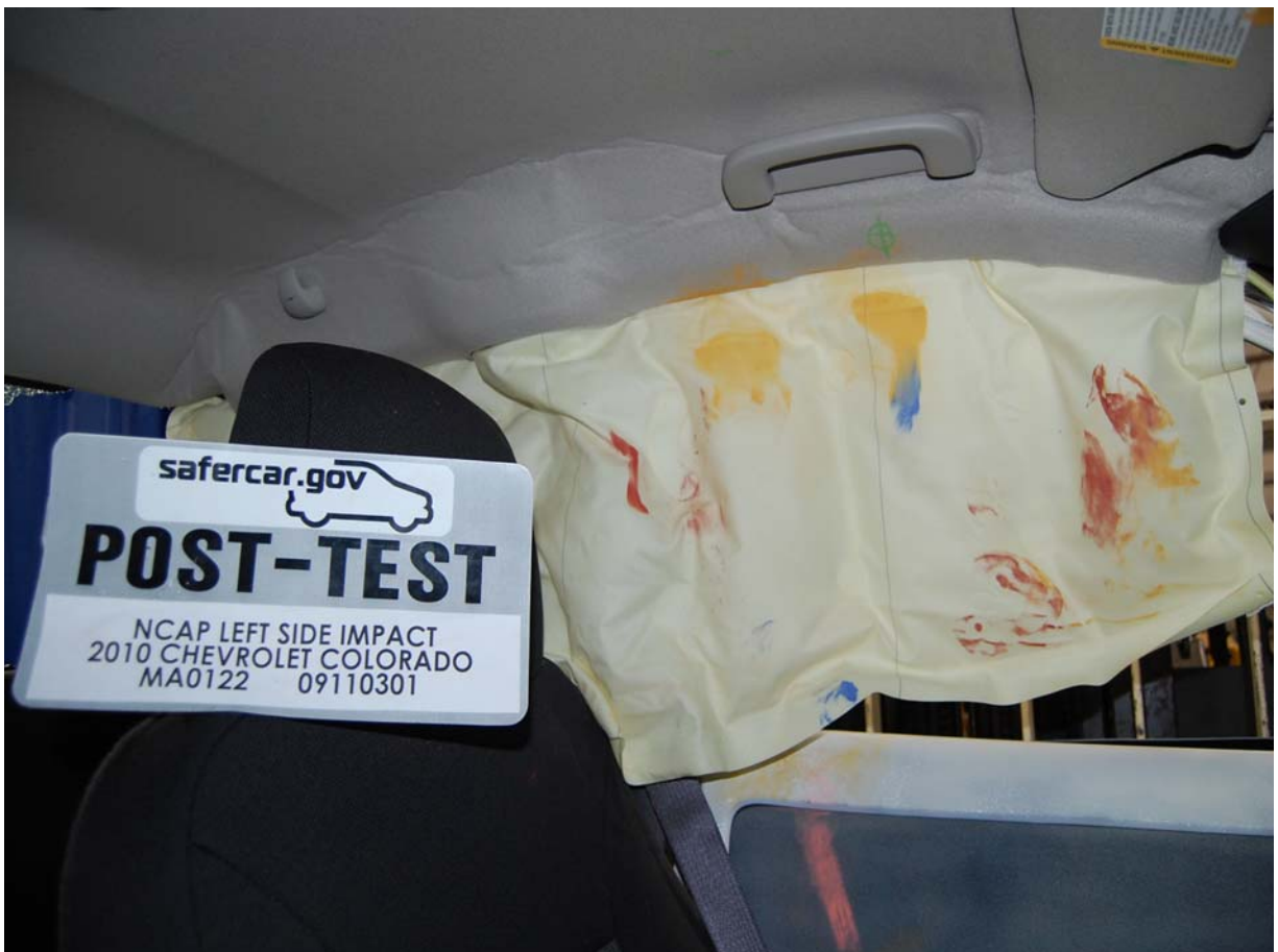
Post-Test Driver Dummy Head Contact View
