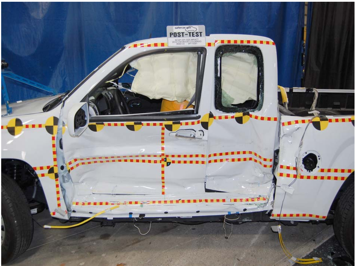
Post-Test Left Side Impact Close-up
