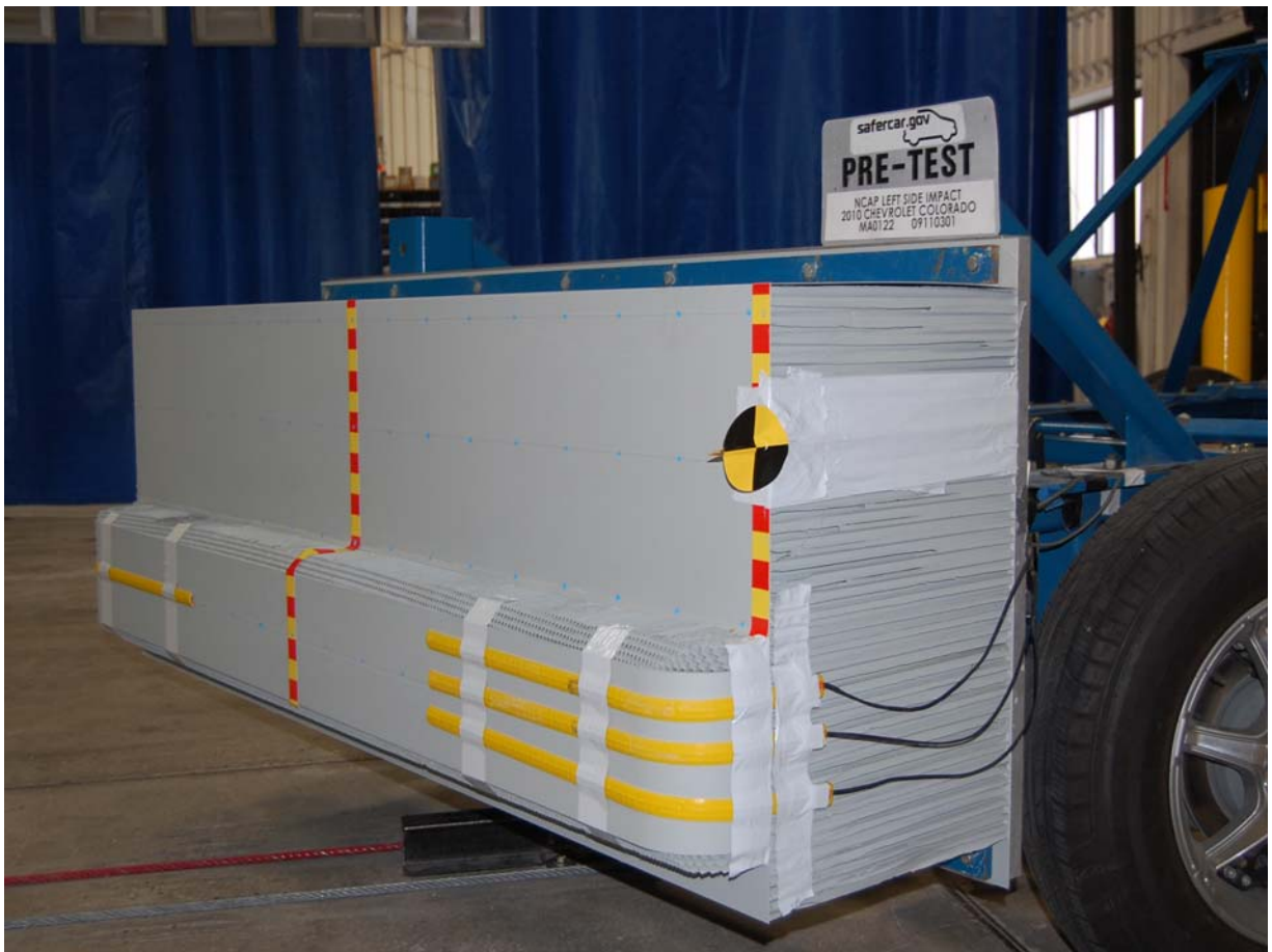
Pre-Test Left Side View of Deformable Barrier
