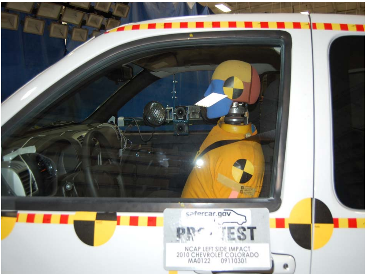
Pre-Test Driver Dummy (Through Window)
