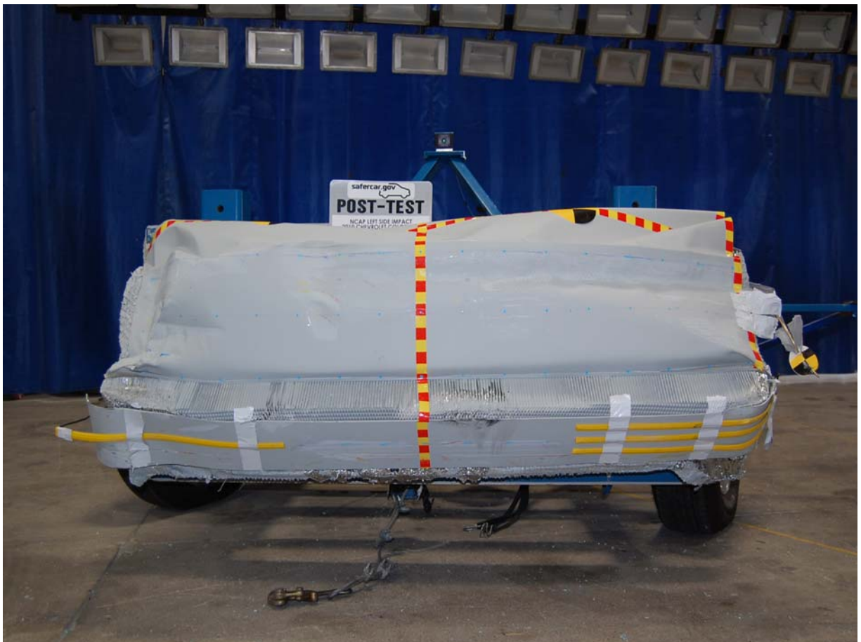
Post-Test Front View of Deformable Barrier
