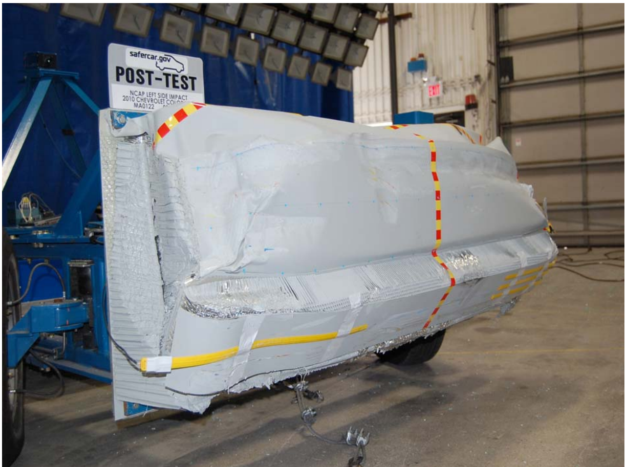
Post-Test Right Side View of Deformable Barrier
