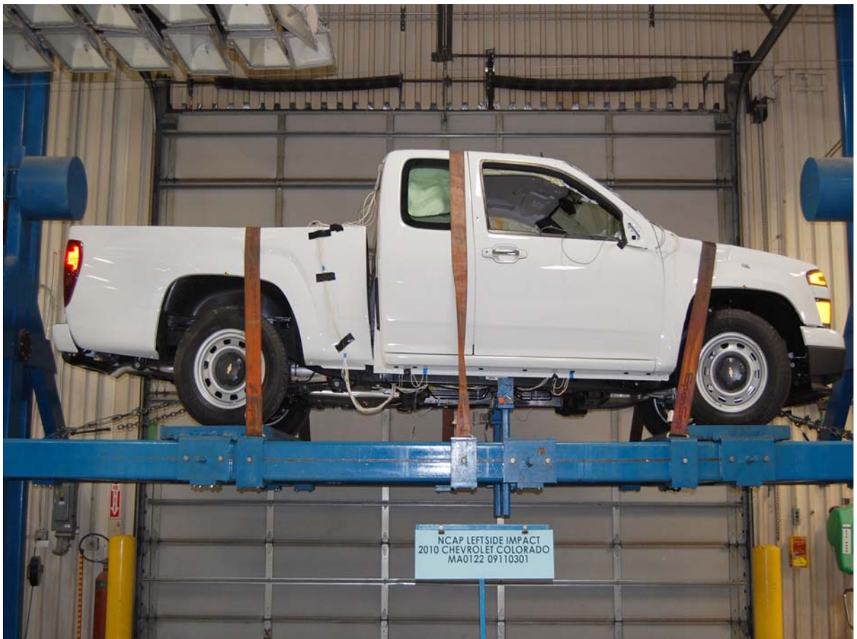
Vehicle on Rollover Device (360 Degrees)
