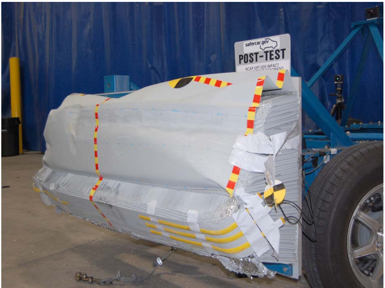
Post-Test Left Side View of Deformable Barrier
