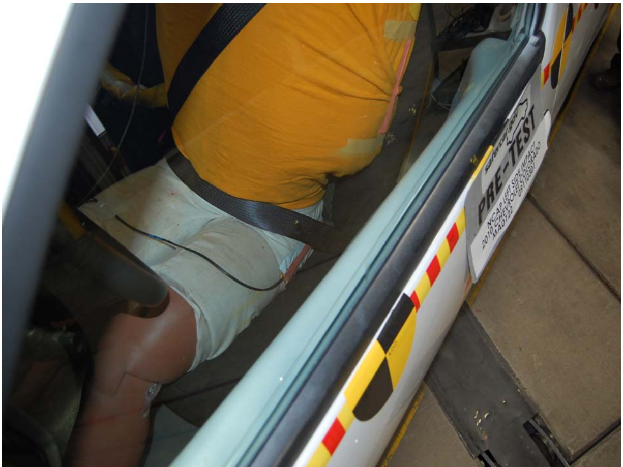
Pre-Test Driver Dummy Clearance From Door
