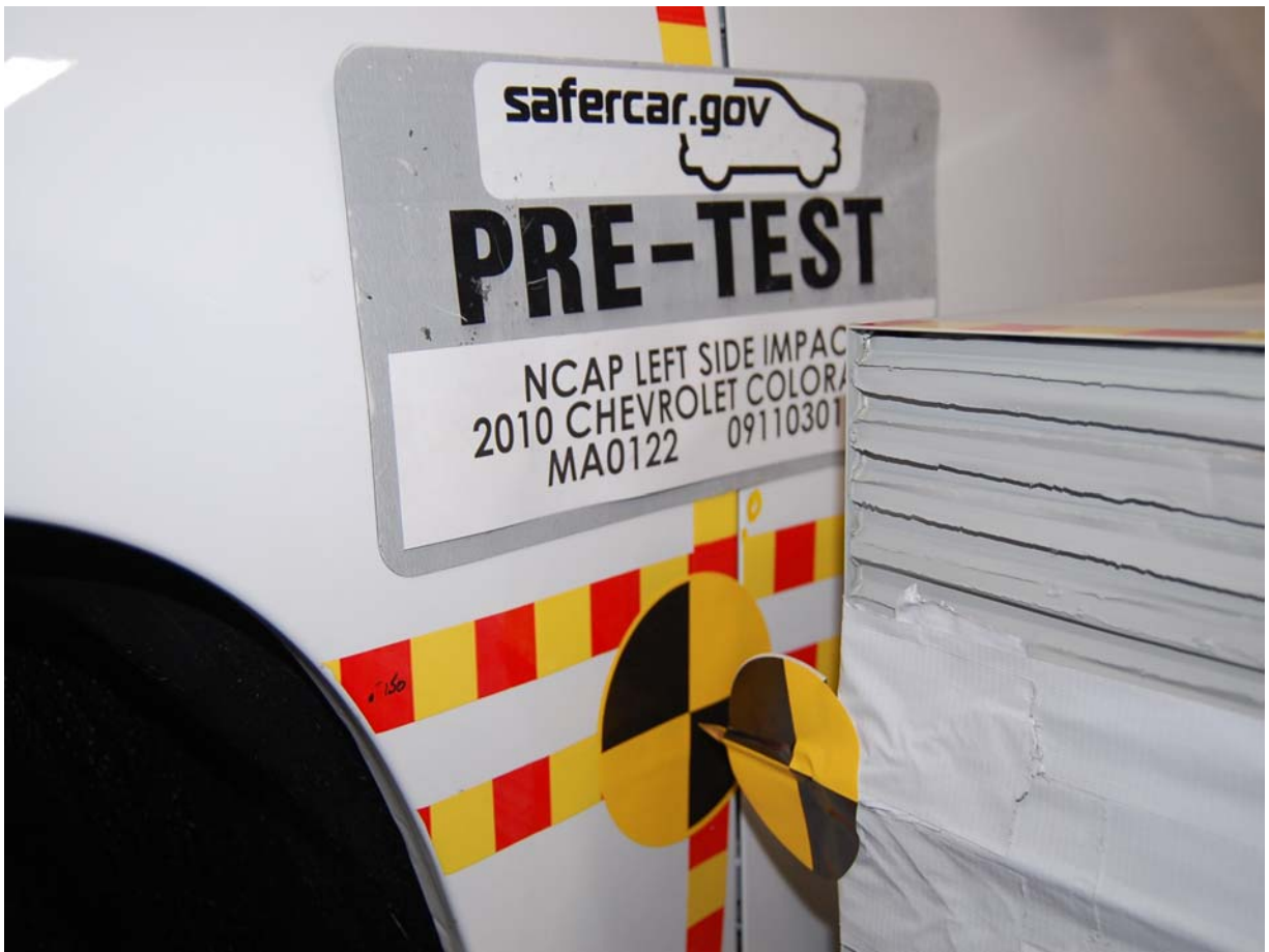
Pre-Test Left Impact Point
