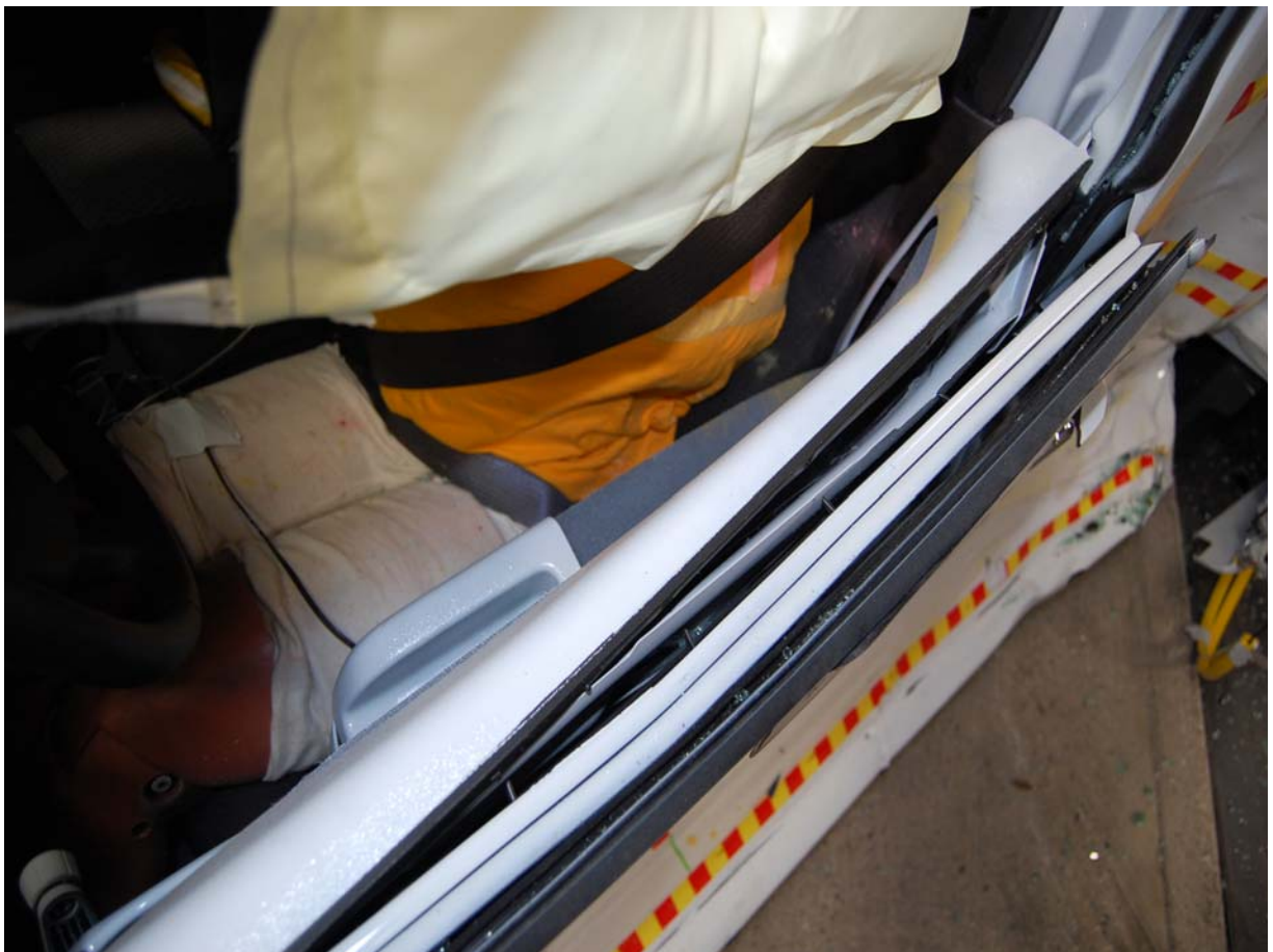
Post-Test Driver Dummy Clearance From Door
