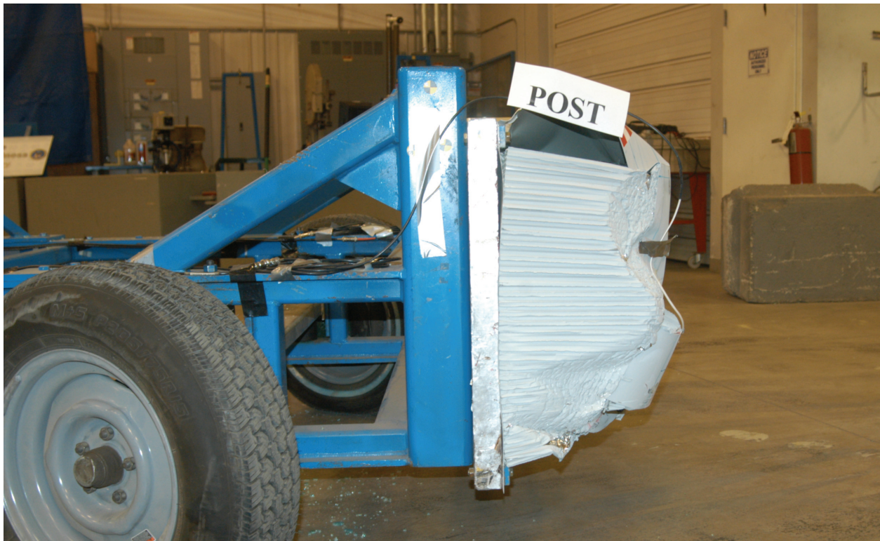
Figure A-56: Post test right side view of MDB barrier face
