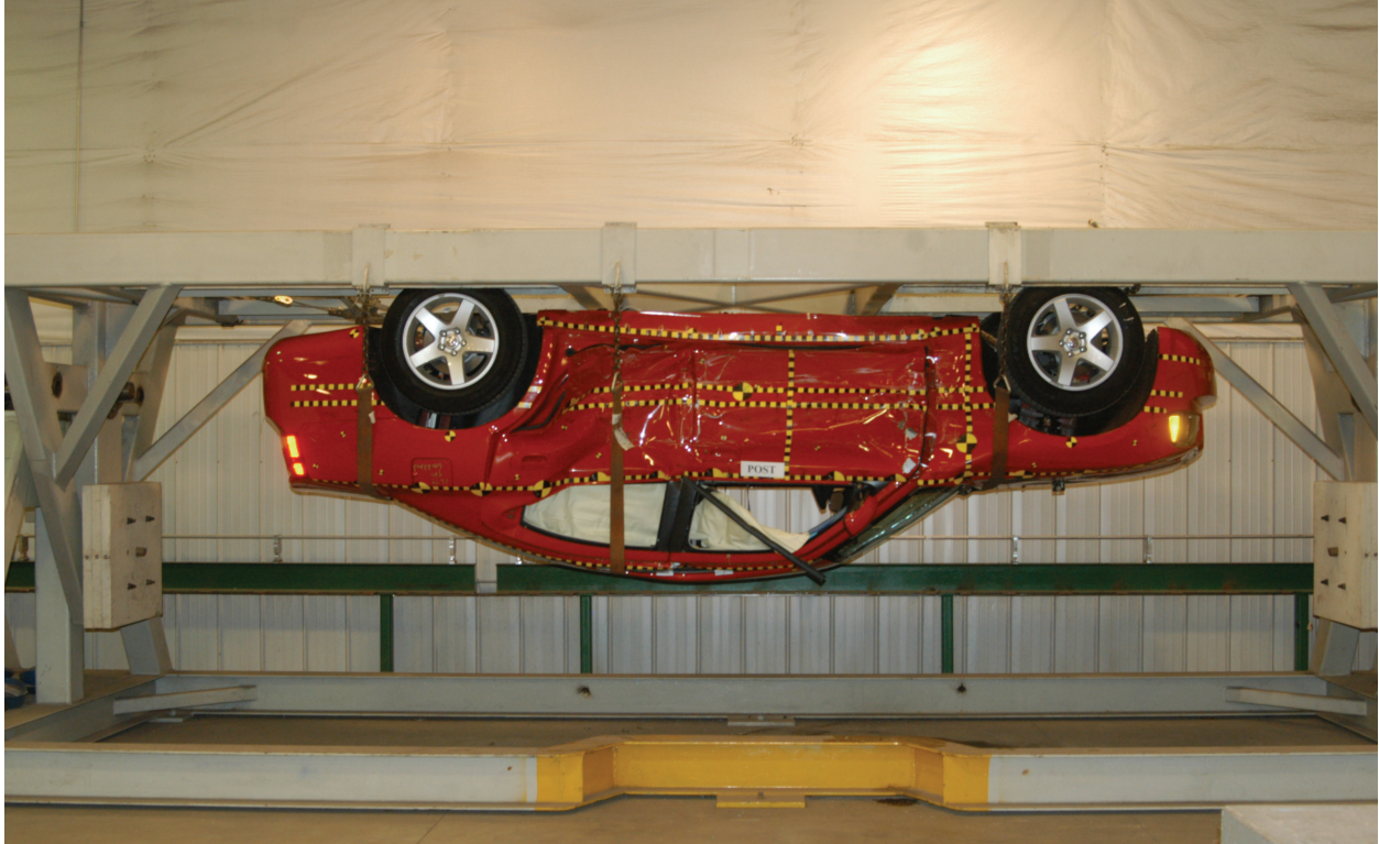
Figure A-61: FMVSS 301 180 degrees
