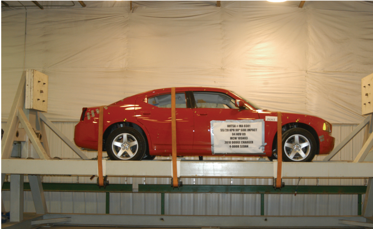
Figure A-59: FMVSS 301 0 degrees
