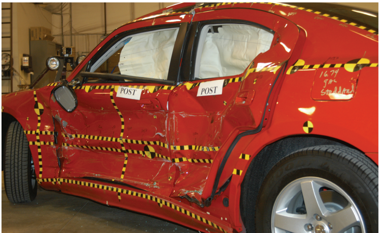
Figure A-30: Post test rear 3/4 view of left side doors
