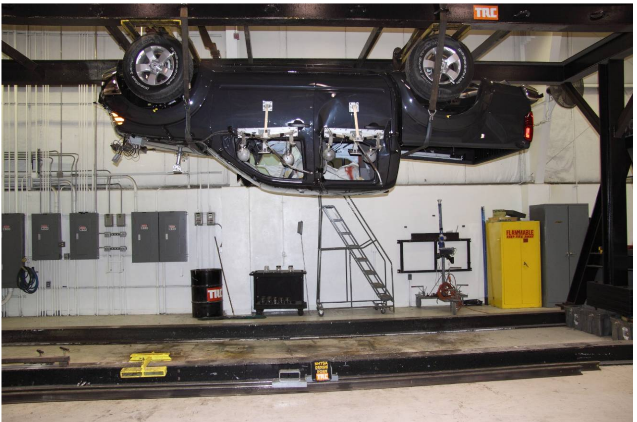
Figure A-82 FMVSS 301 Rollover View at 180°
