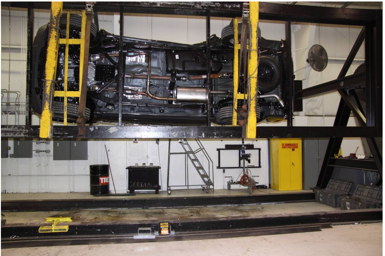
Figure A-83 FMVSS 301 Rollover View at 270°
