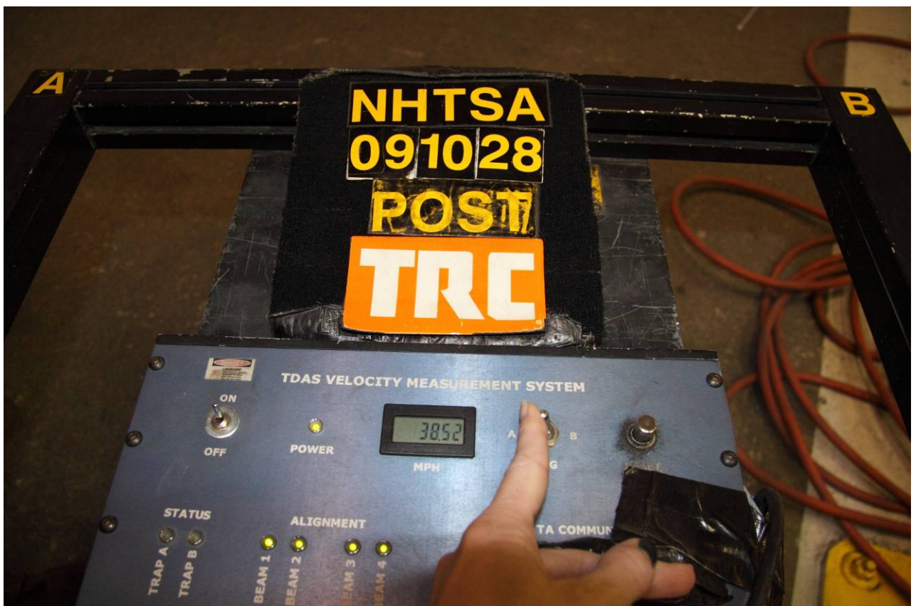
Figure A-76 Post-Test Redundant Light Trap Digital Readout
