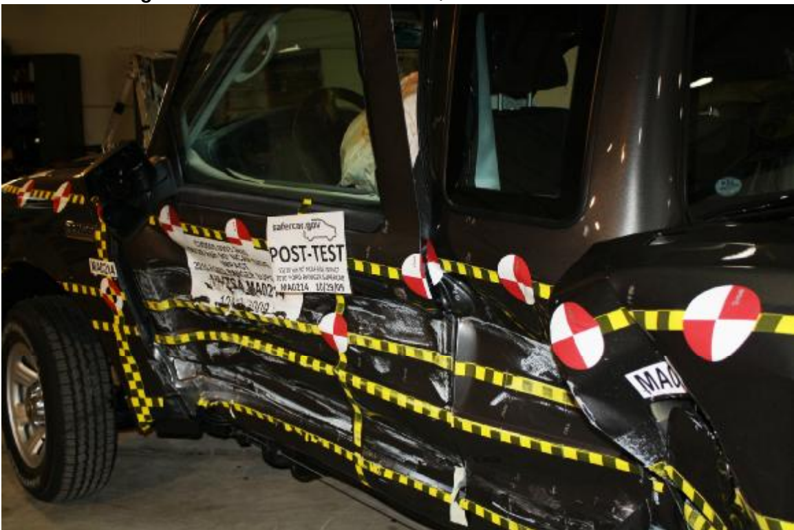
Figure A-46: Post-Test Left Rear \frac{3}{4} View of Left Side Doors
