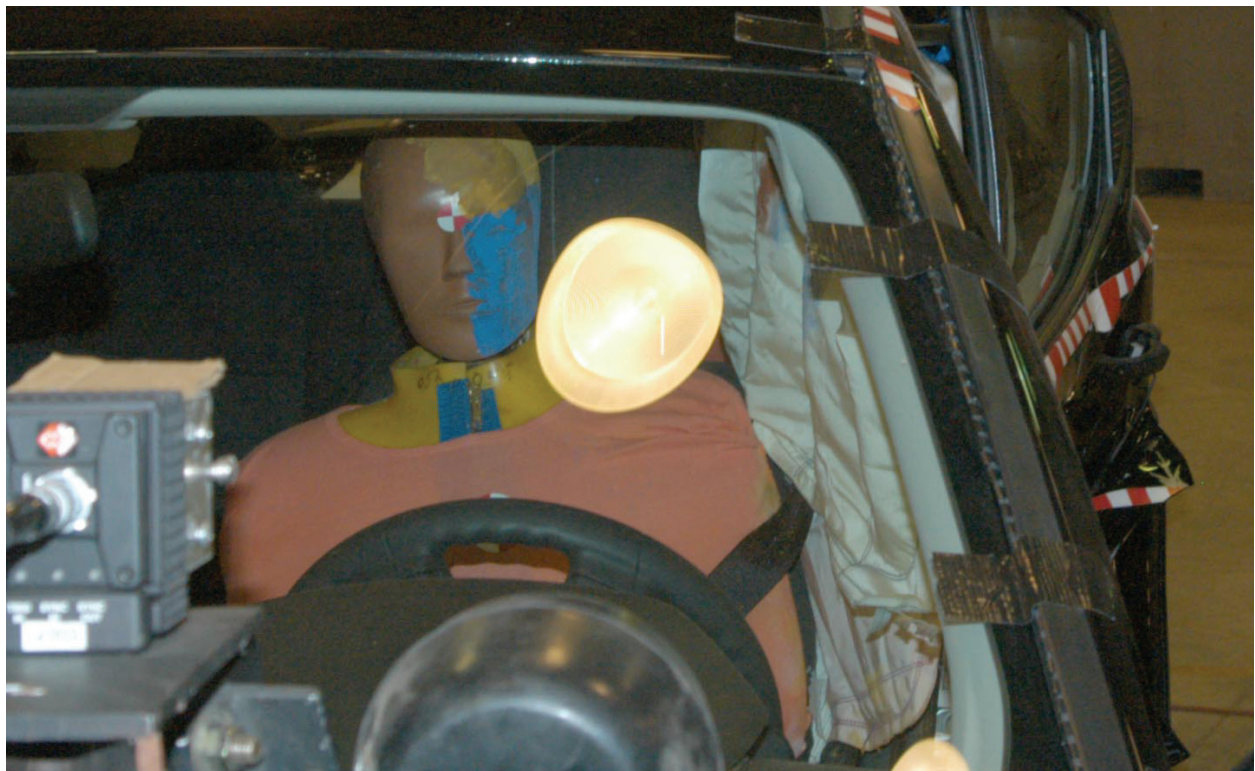
Figure A-38: Post test driver shoulder clearance
