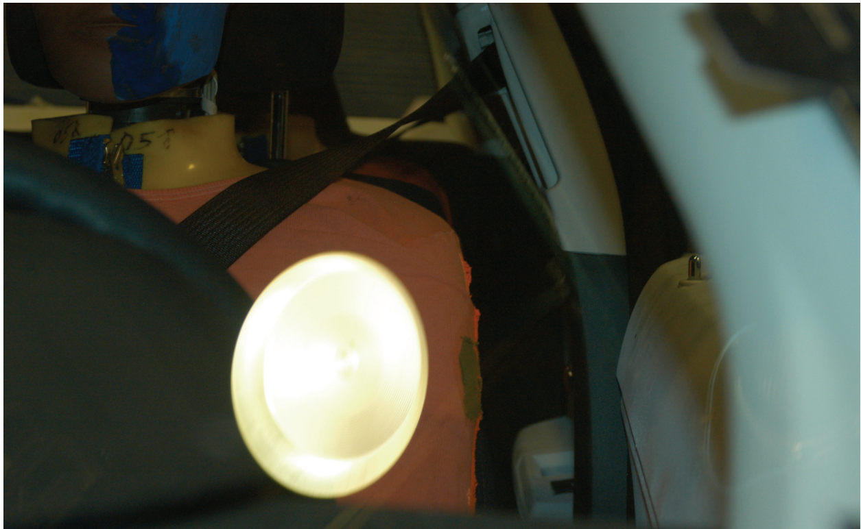
Figure A-37: Pre test driver shoulder clearance
