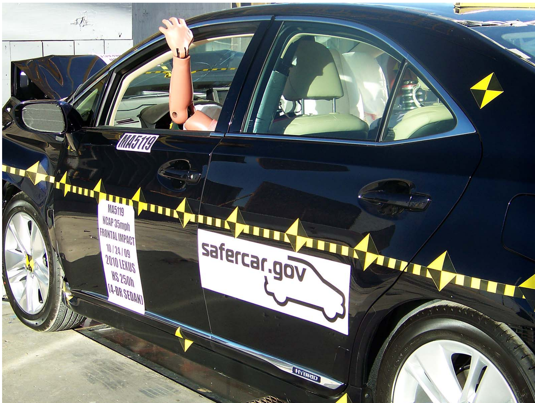
Figure A-21: Post-Test Left Side ¾ View of Doors After Impact
