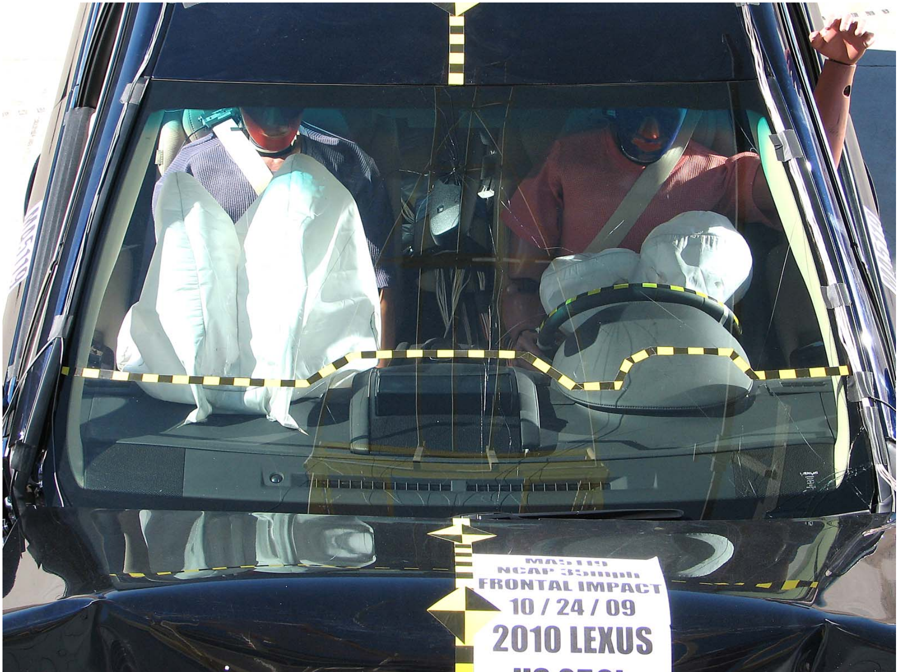
Figure A-24: Post-Test Windshield
