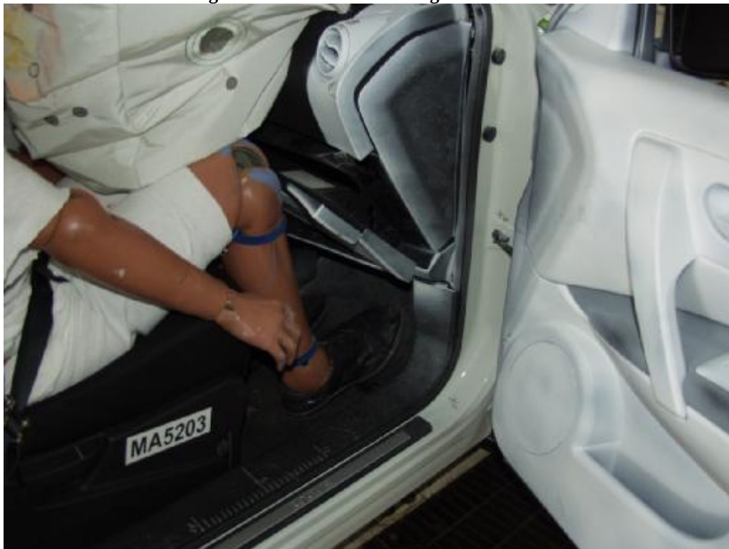
Figure A-51: Post-Test Passenger Feet View
