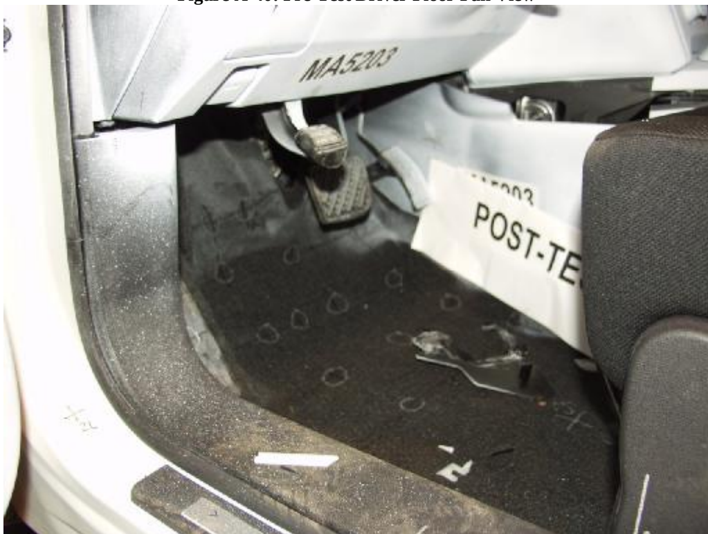
Figure A-41: Post-Test Driver Floor Pan View
