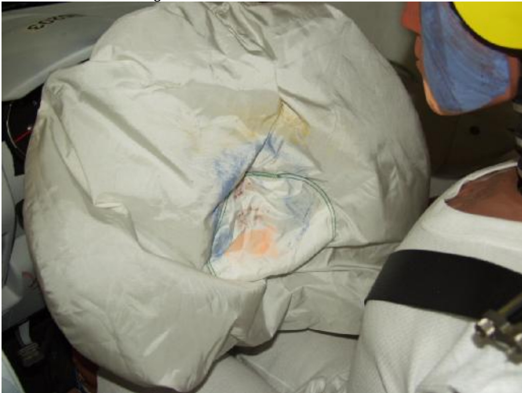
Figure A-43: Post-Test Driver Contact to Airbag
