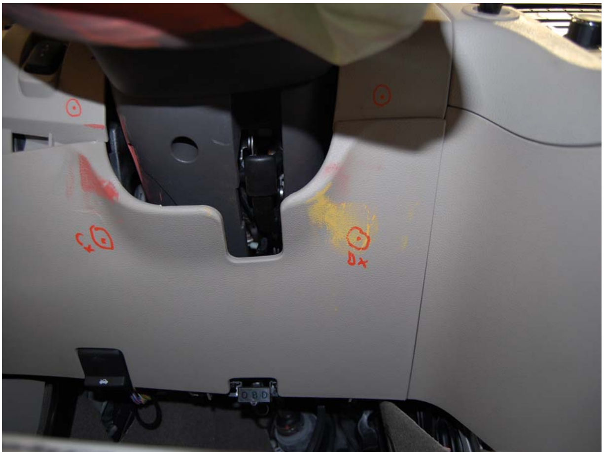
Post-Test Driver Dummy Knee Contact
