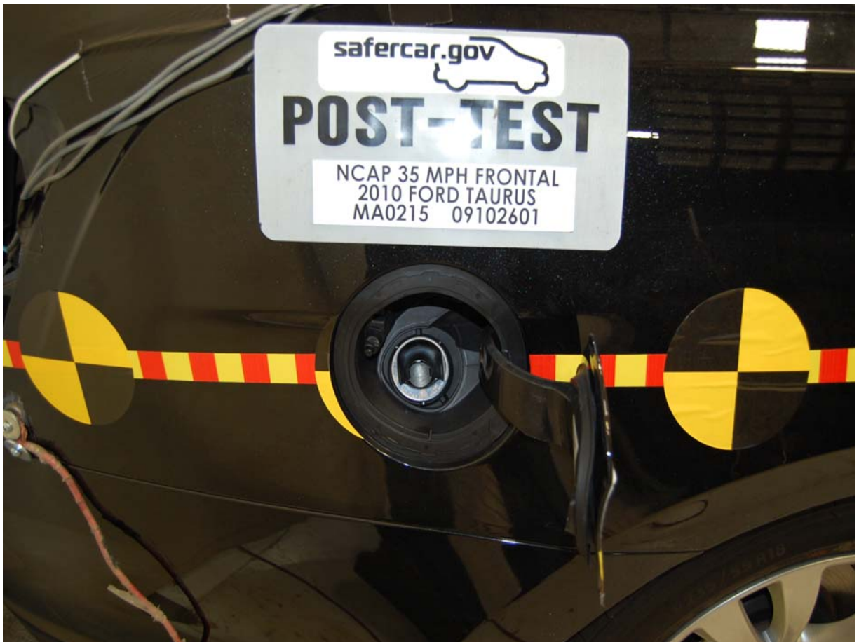
Post-Test Fuel Cap View
