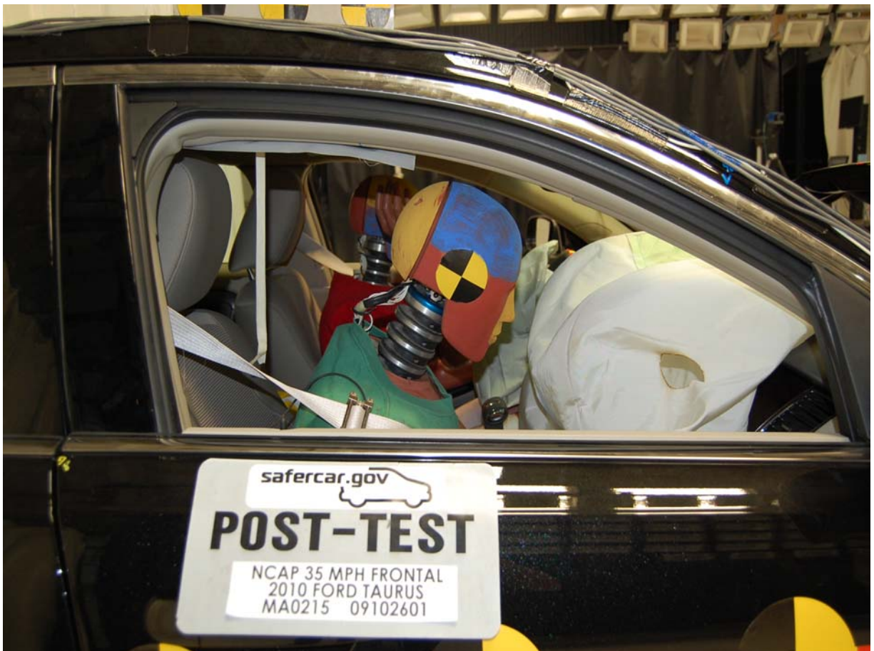
Post-Test Passenger Dummy (Through Window)
