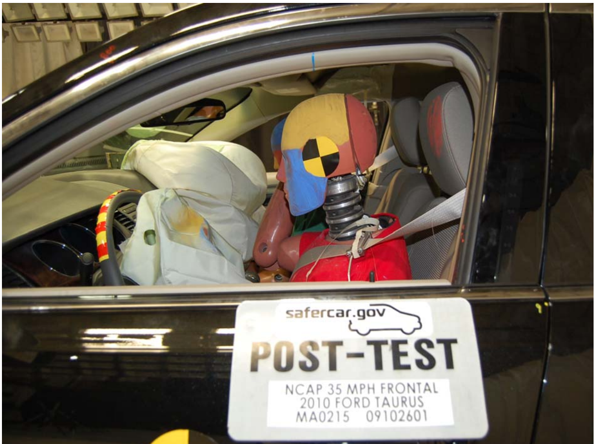
Post-Test Driver Dummy (Through Window)
