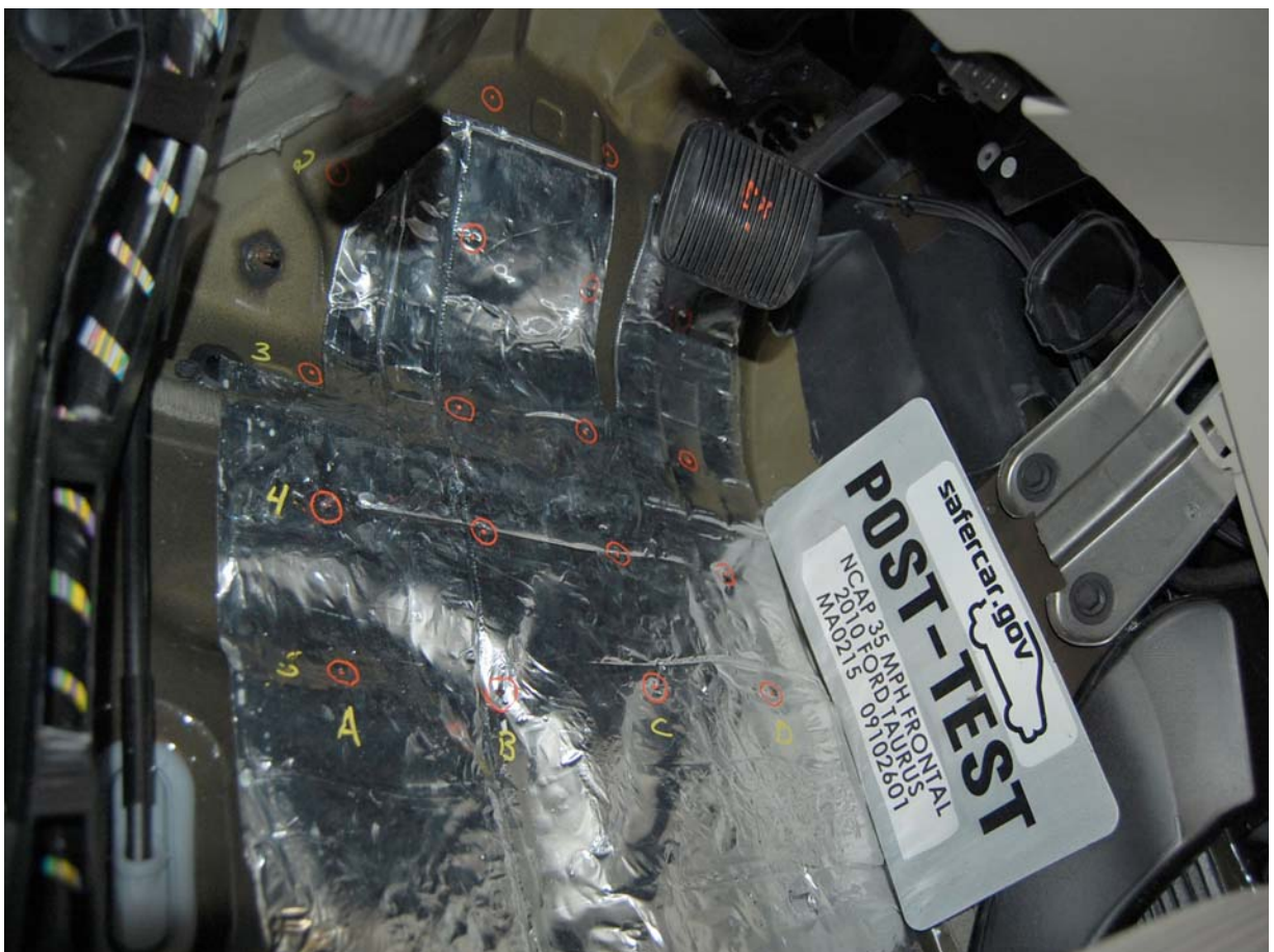
Post-Test Driver Side Floor Pan
