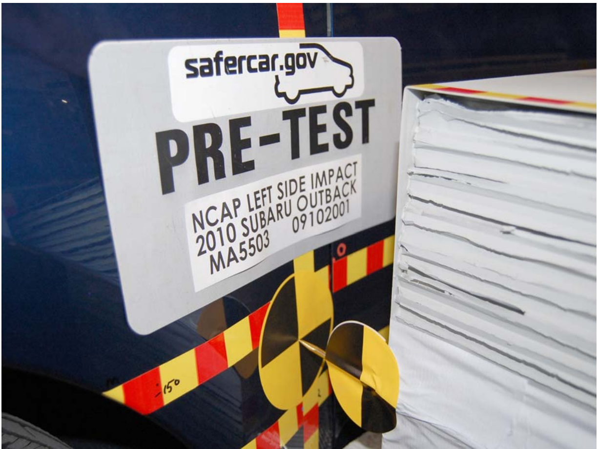
Pre-Test Left Impact Point
