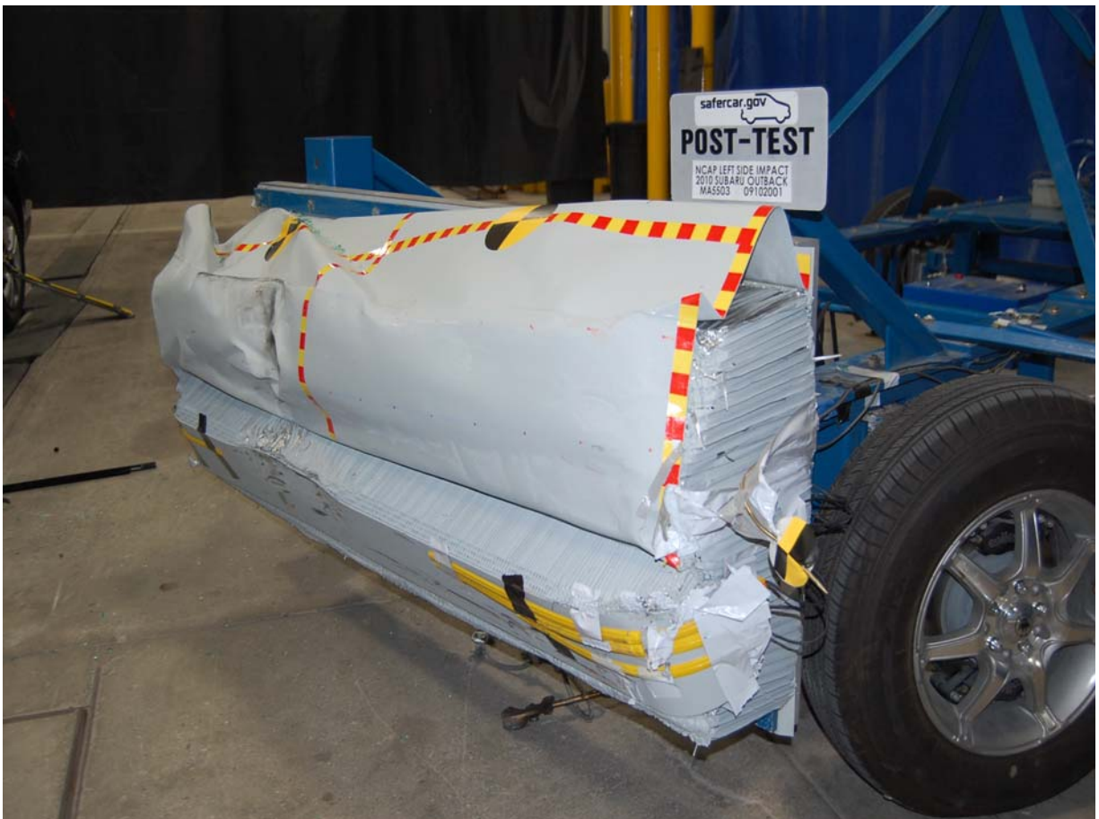
Post-Test Left Side View of Deformable Barrier
