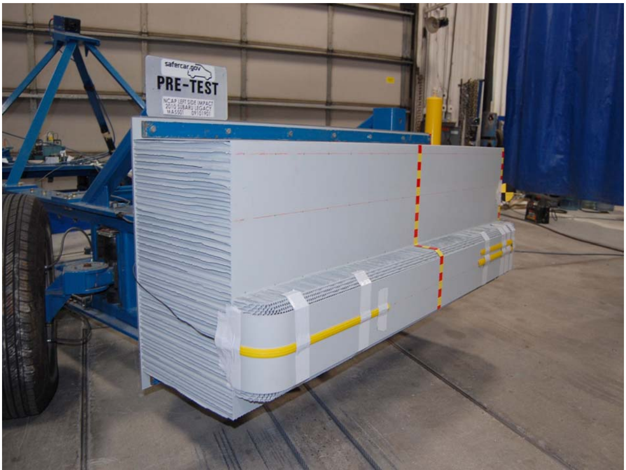
Pre-Test Right Side View of Deformable Barrier
