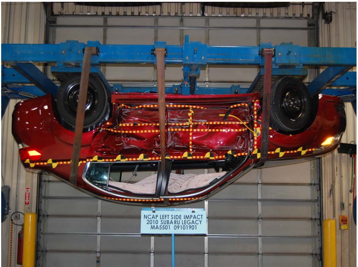
Vehicle on Rollover Device (180 Degrees)
