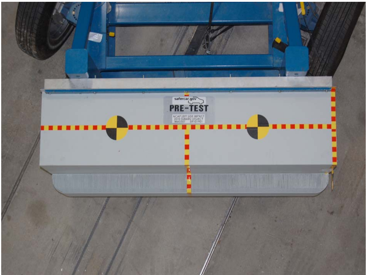
Pre-Test Top View of Deformable Barrier
