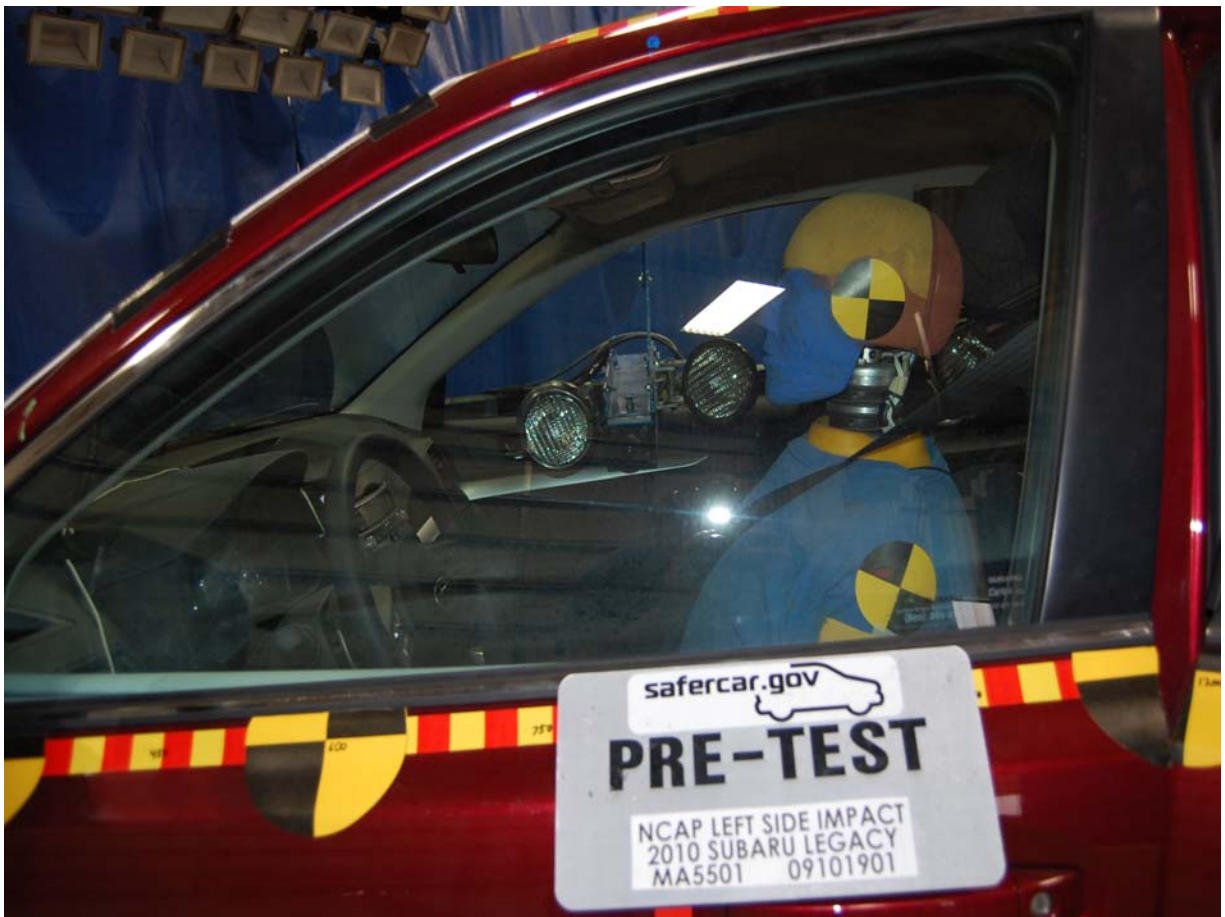
Pre-Test Driver Dummy (Through Window)
