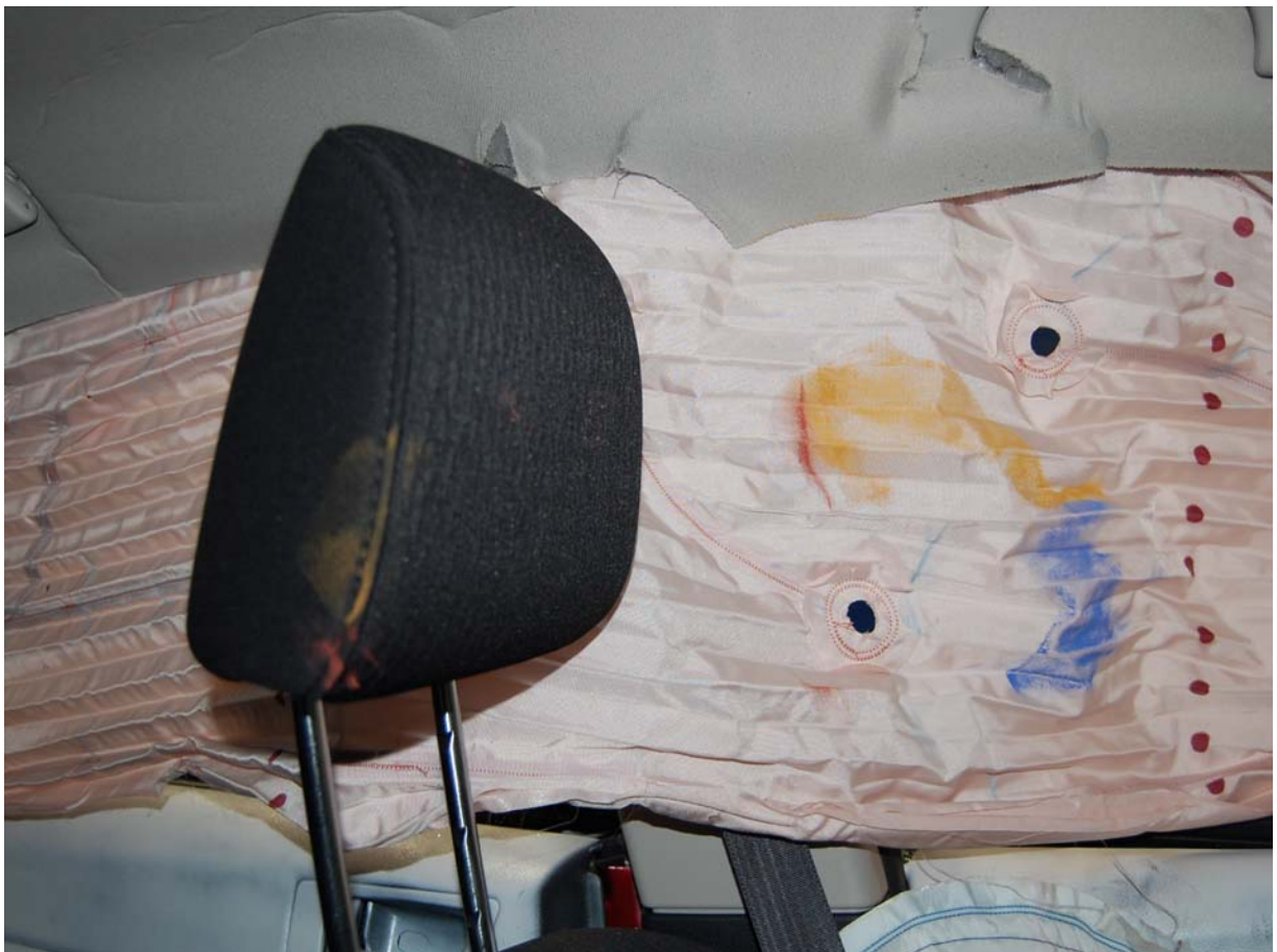
Post-Test Driver Dummy Head Contact View
