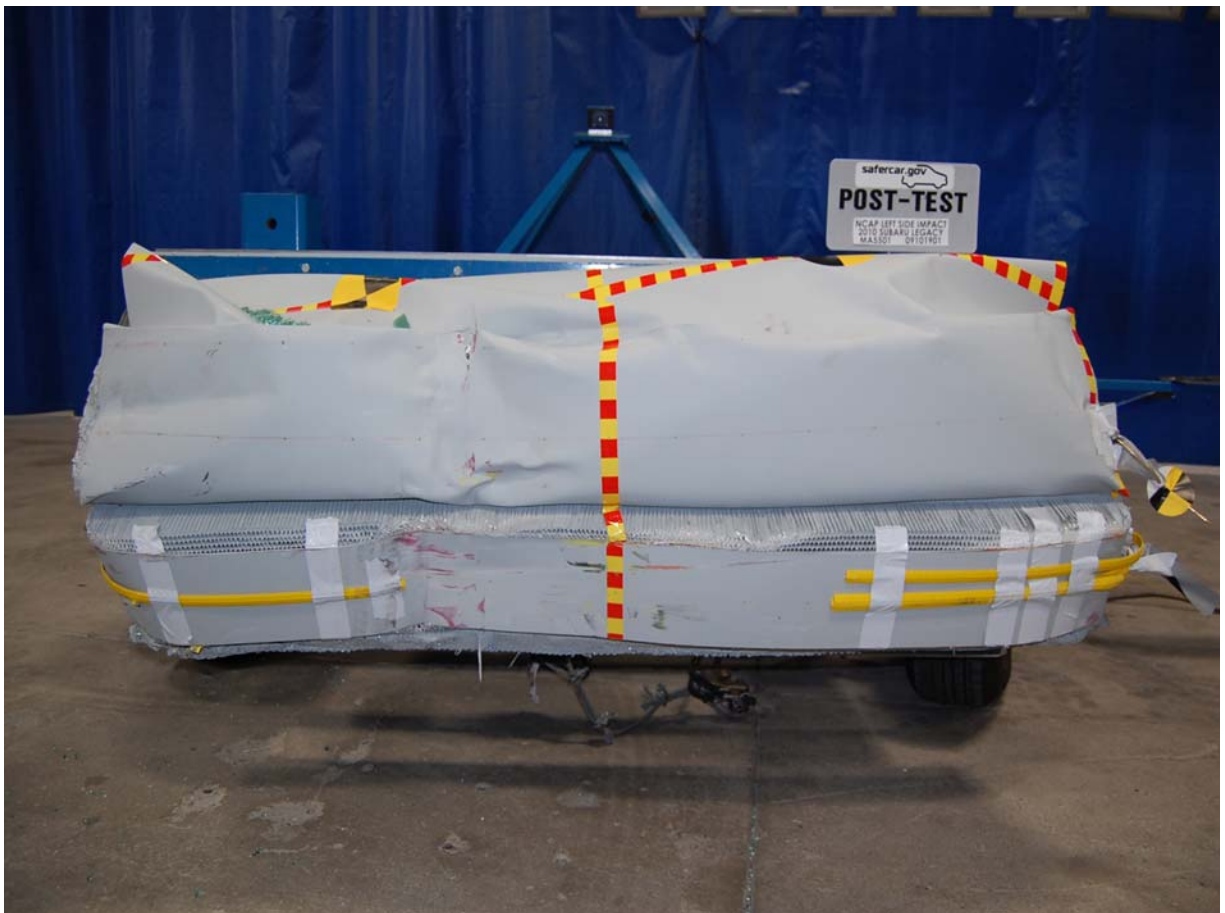
Post-Test Front View of Deformable Barrier
