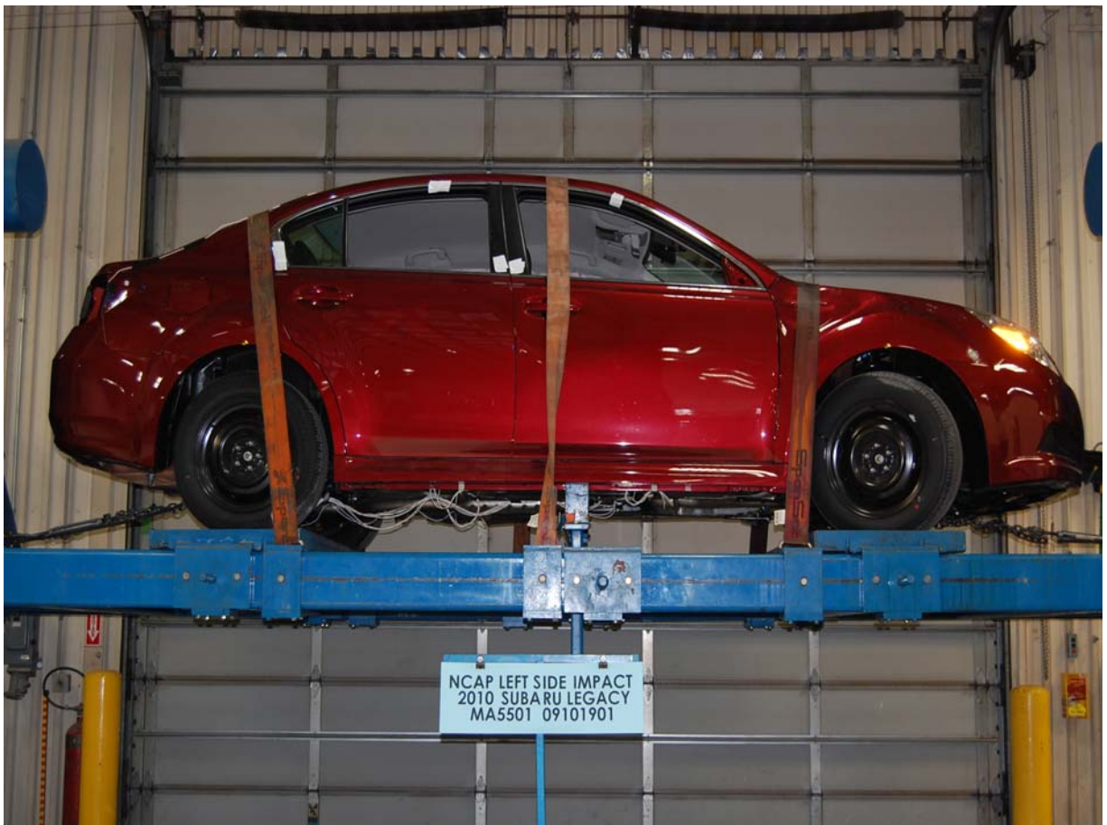
Vehicle on Rollover Device (360 Degrees)
