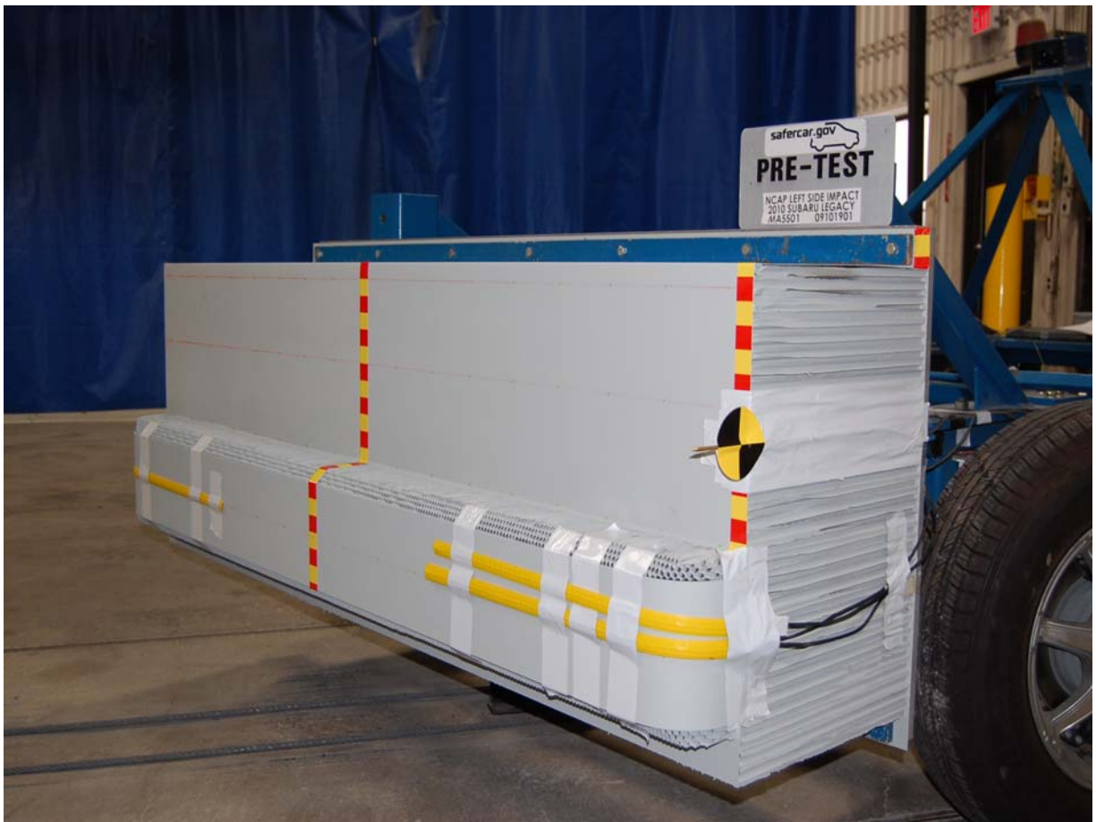
Pre-Test Left Side View of Deformable Barrier
