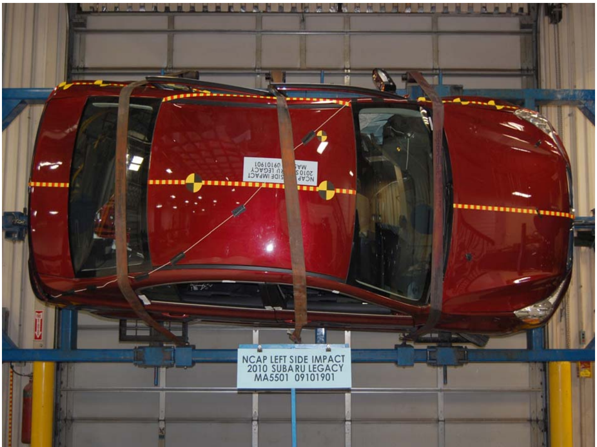
Vehicle on Rollover Device (90 Degrees)
