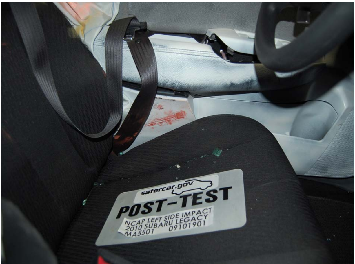
Post-Test Driver Dummy Lower Torso Contact
