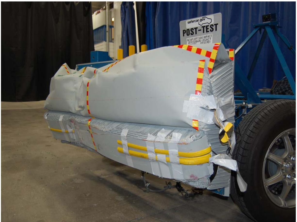
Post-Test Left Side View of Deformable Barrier
