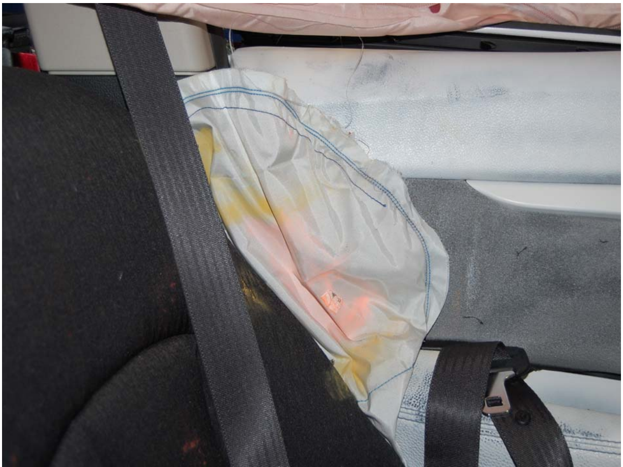
Post-Test Driver Dummy Upper Torso Contact
