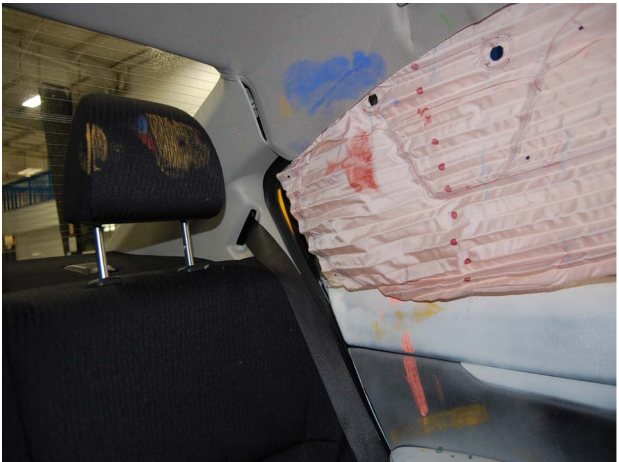
Post-Test Passenger Dummy Head Contact View
