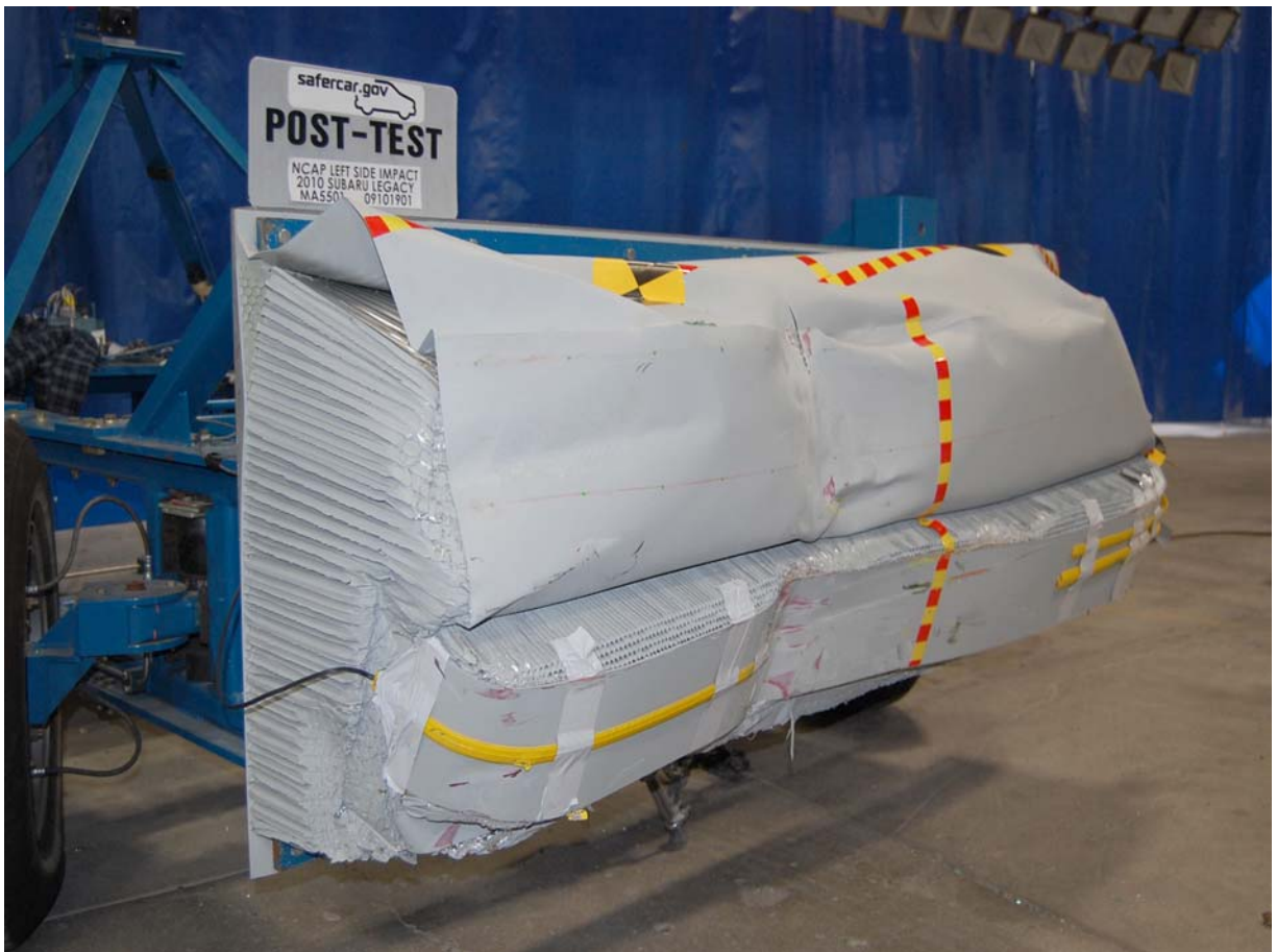
Post-Test Right Side View of Deformable Barrier
