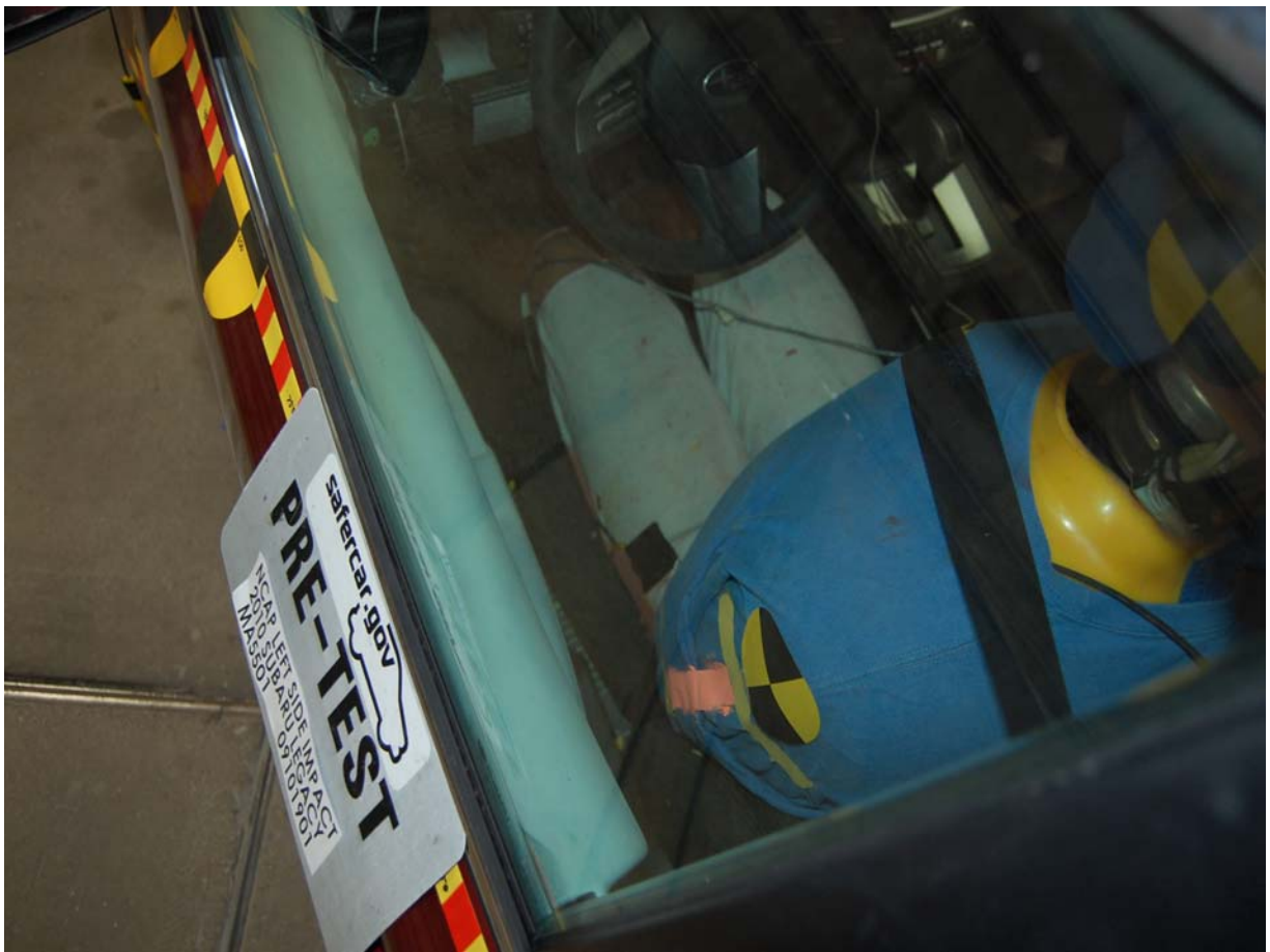
Pre-Test Driver Dummy Clearance From Door
