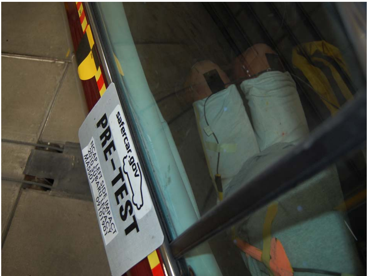
Pre-Test Passenger Dummy Clearance From Door
