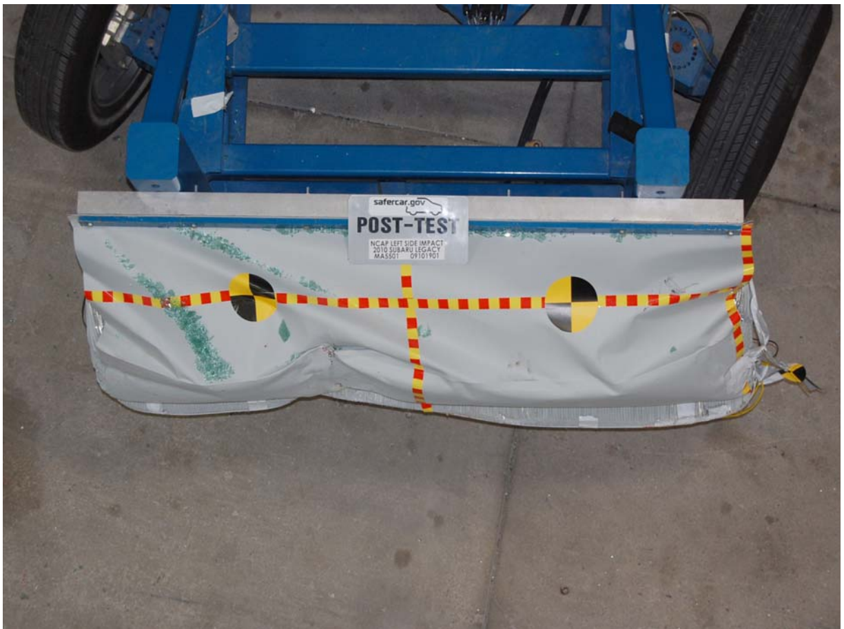
Post-Test Top View of Deformable Barrier
