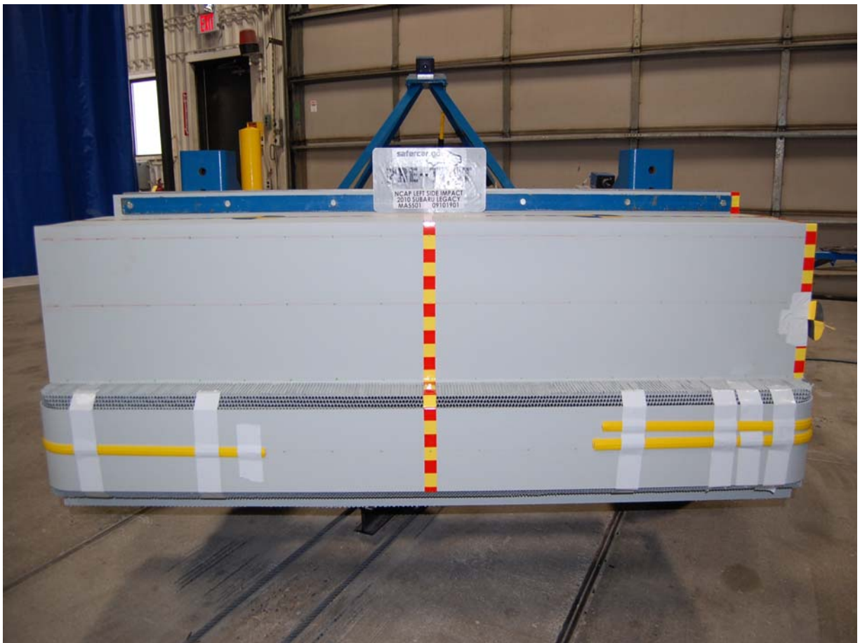
Pre-Test Front View of Deformable Barrier
