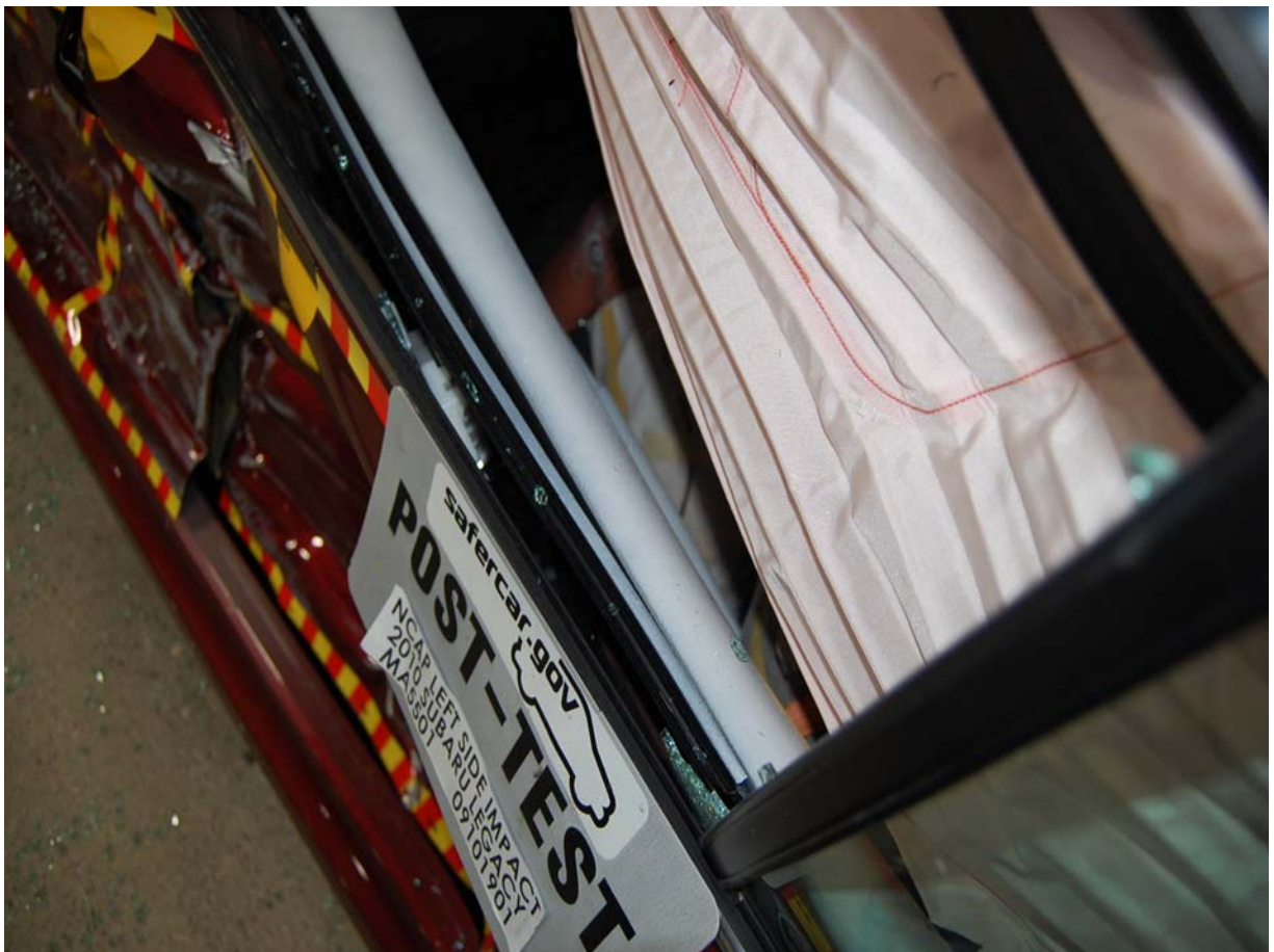
Post-Test Passenger Dummy Clearance From Door
