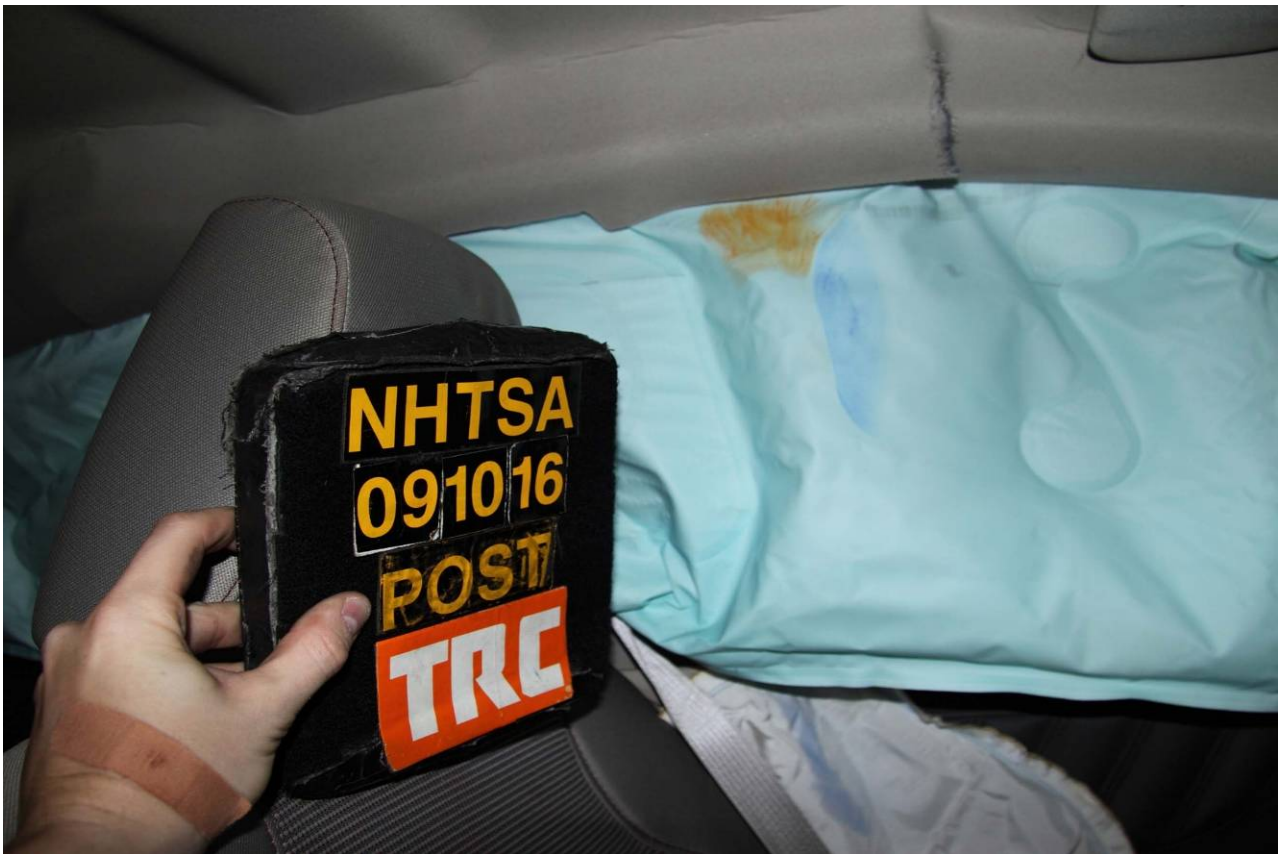
Figure A-54 Post-Test Front SID HIII Contact – View 1
