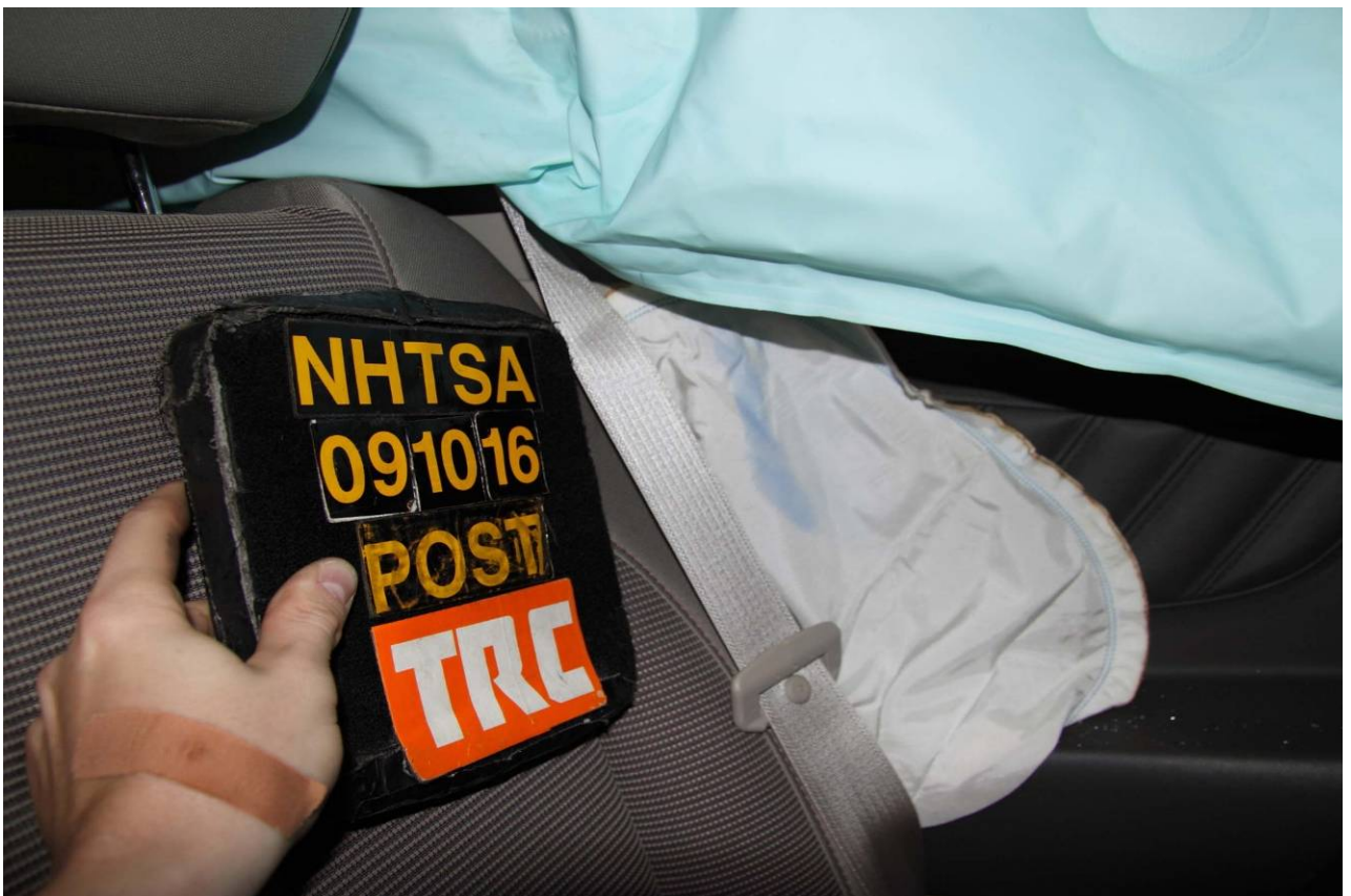
Figure A-55 Post-Test Front SID HIII Contact – View 2
