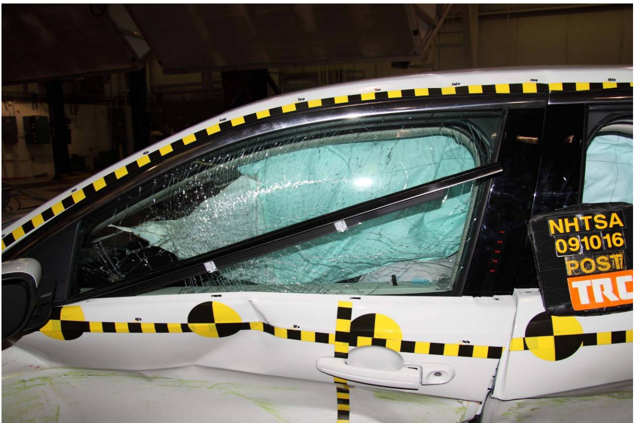
Figure A-44 Post-Test Left View of Front SID HIII
