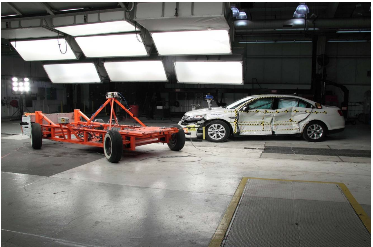
Figure A-62 Post-Test Left Side View of MDB With Impactor Face in Position
