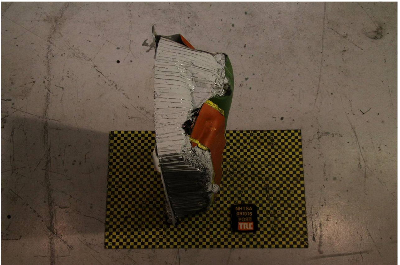
Figure A-20 Post-Test Left Side View of Impactor Face
