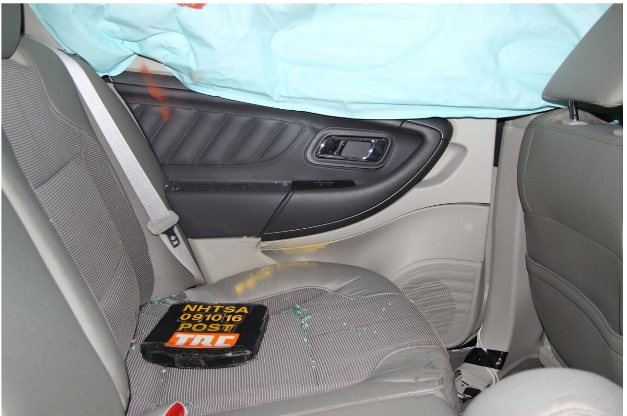
Figure A-58 Post-Test Interior of Rear Side Panel
