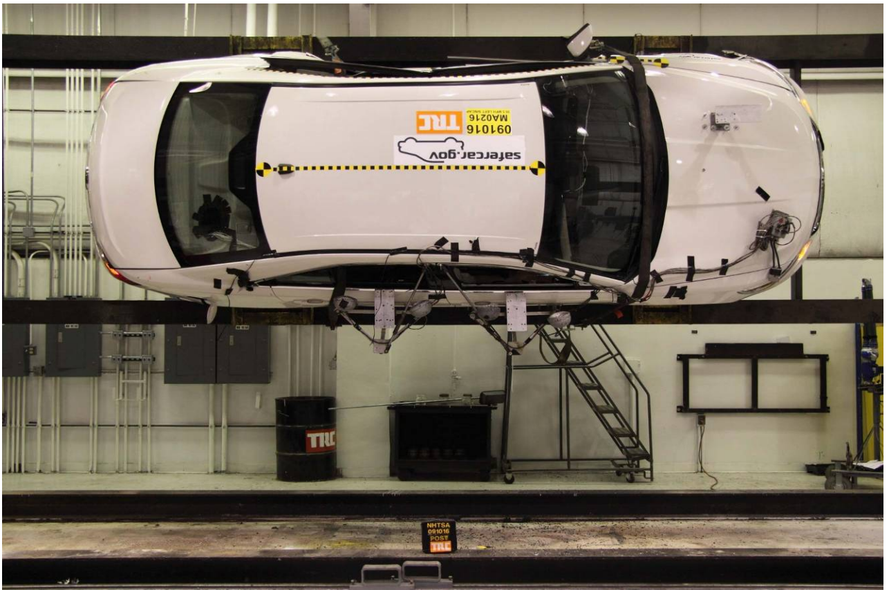
Figure A-76 FMVSS 301 Rollover View at 90°
