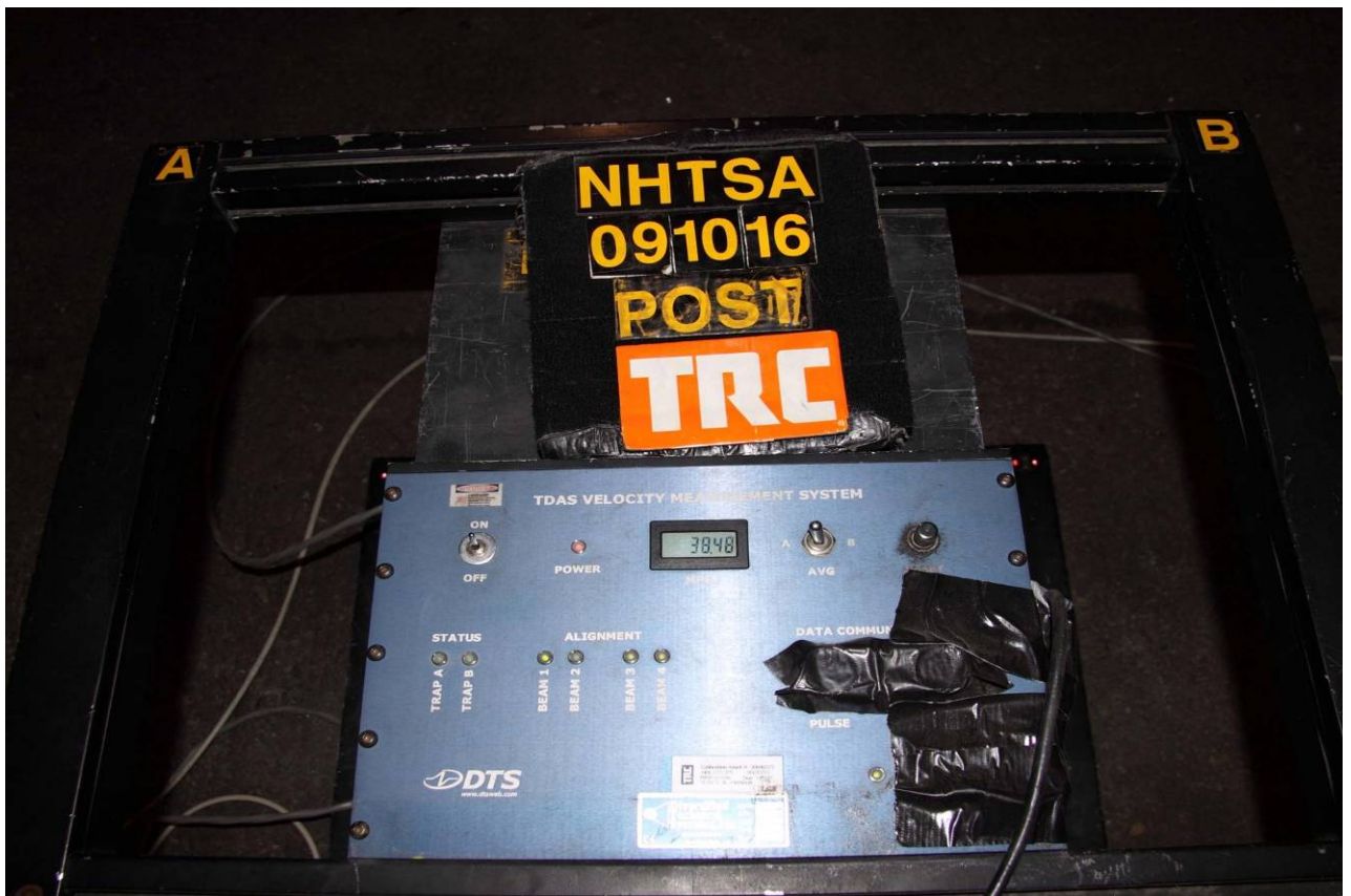
Figure A-73 Post-Test Light Trap Digital Readout
