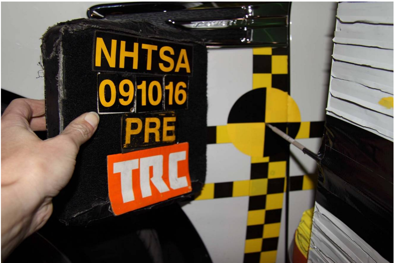
Figure A-63 Pre-Test Primary Impact Point View
