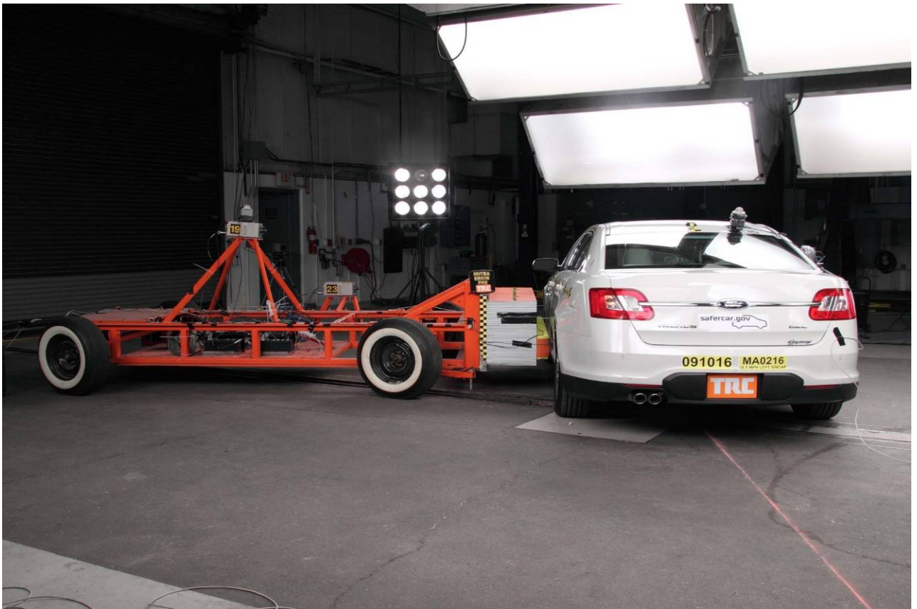
Figure A-65 Pre-Test Right Side View of MDB With Impactor Face in Position
