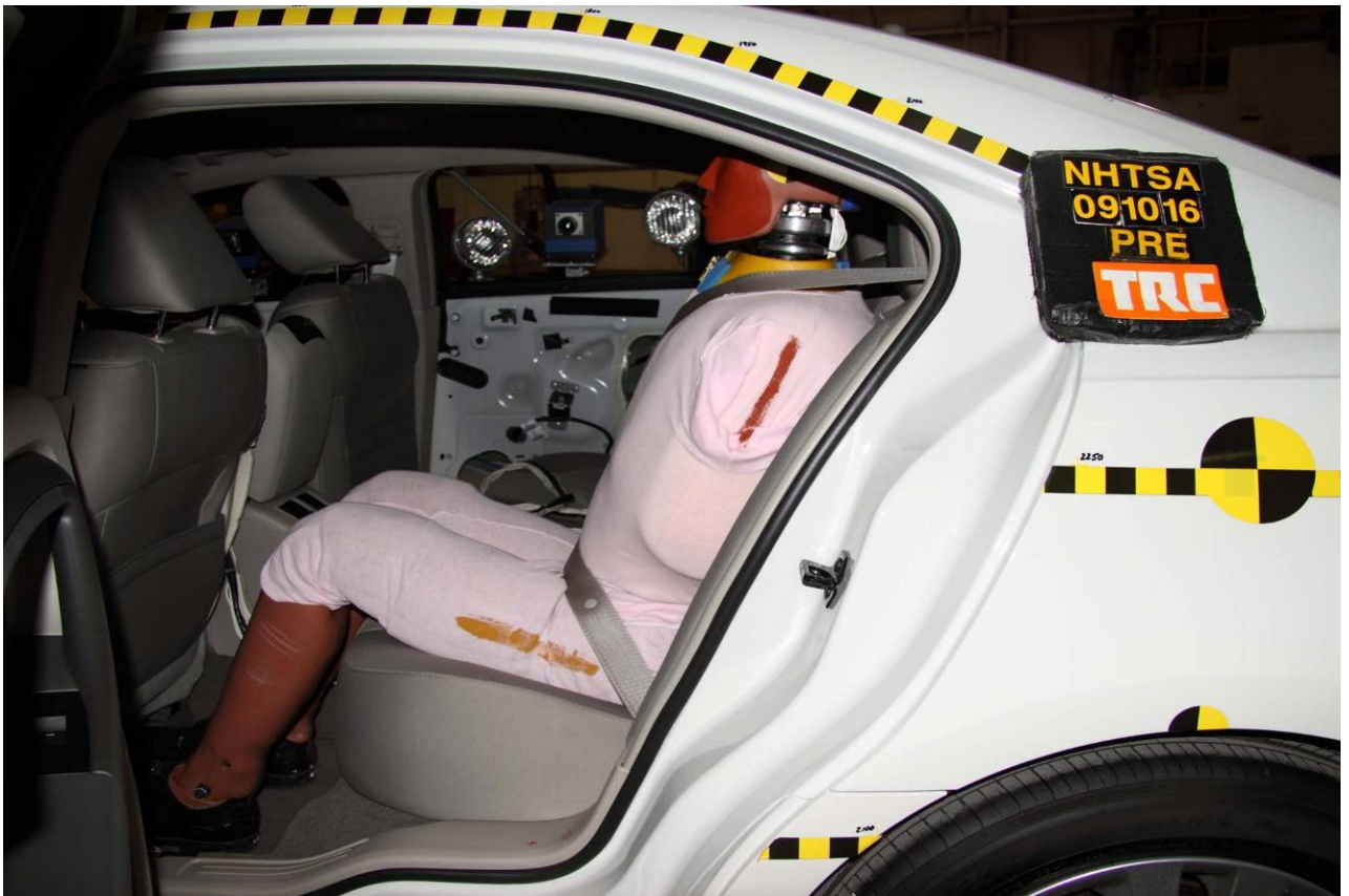
Figure A-50 Pre-Test Left View of Rear SID HIII and Belt Position
