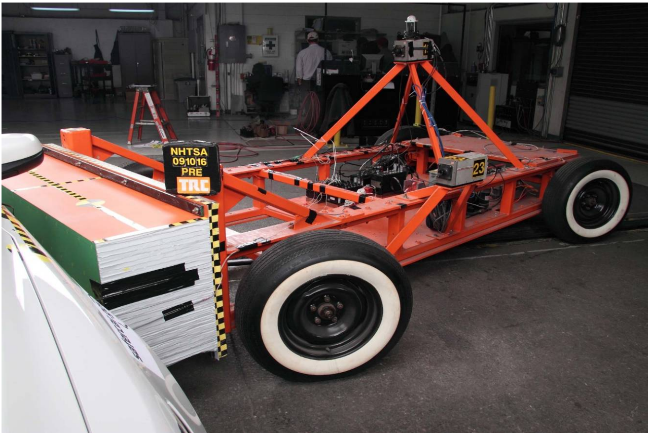
Figure A-69 Pre-Test Left Front View of MDB with Impactor Face in Position
