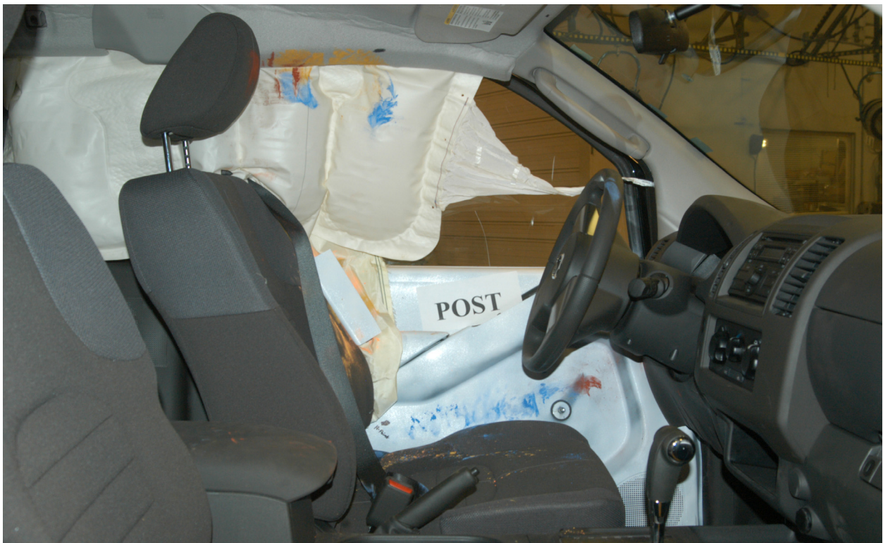
Figure A-38: Post test driver contact locations (2)
