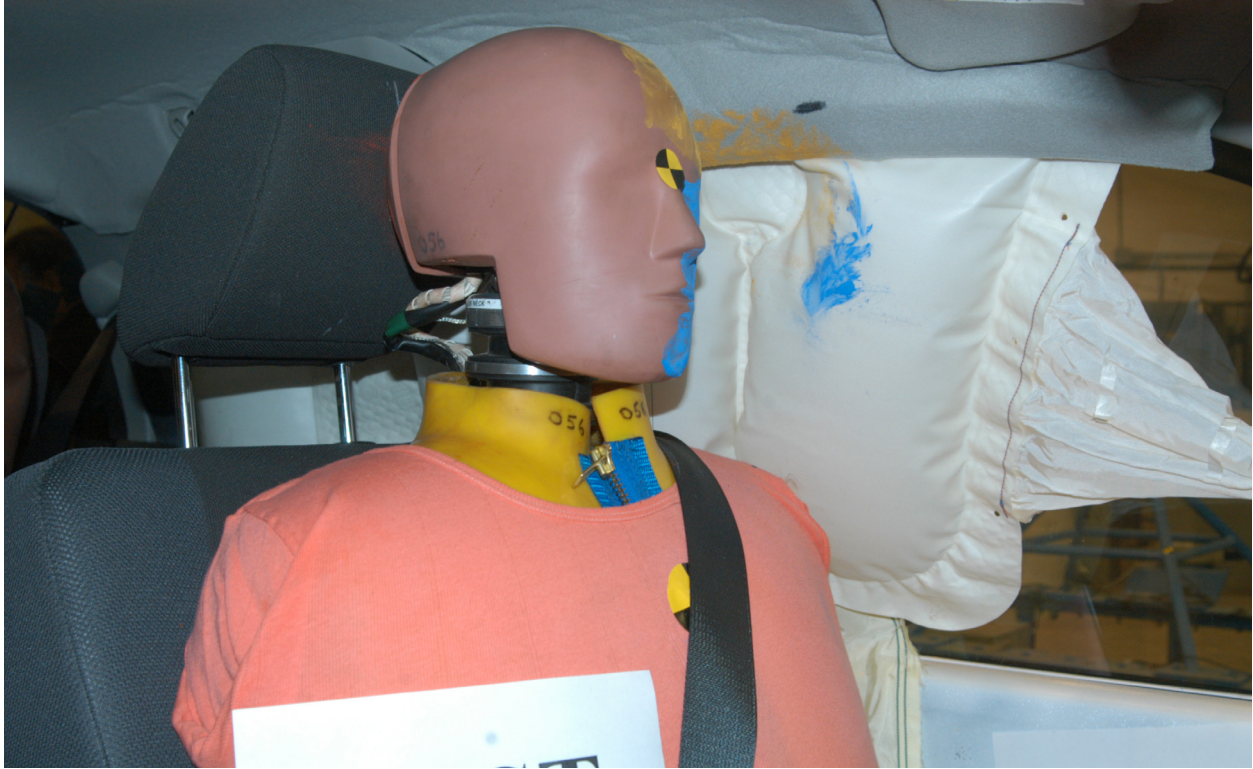
Figure A-37: Post test driver contact locations (1)
