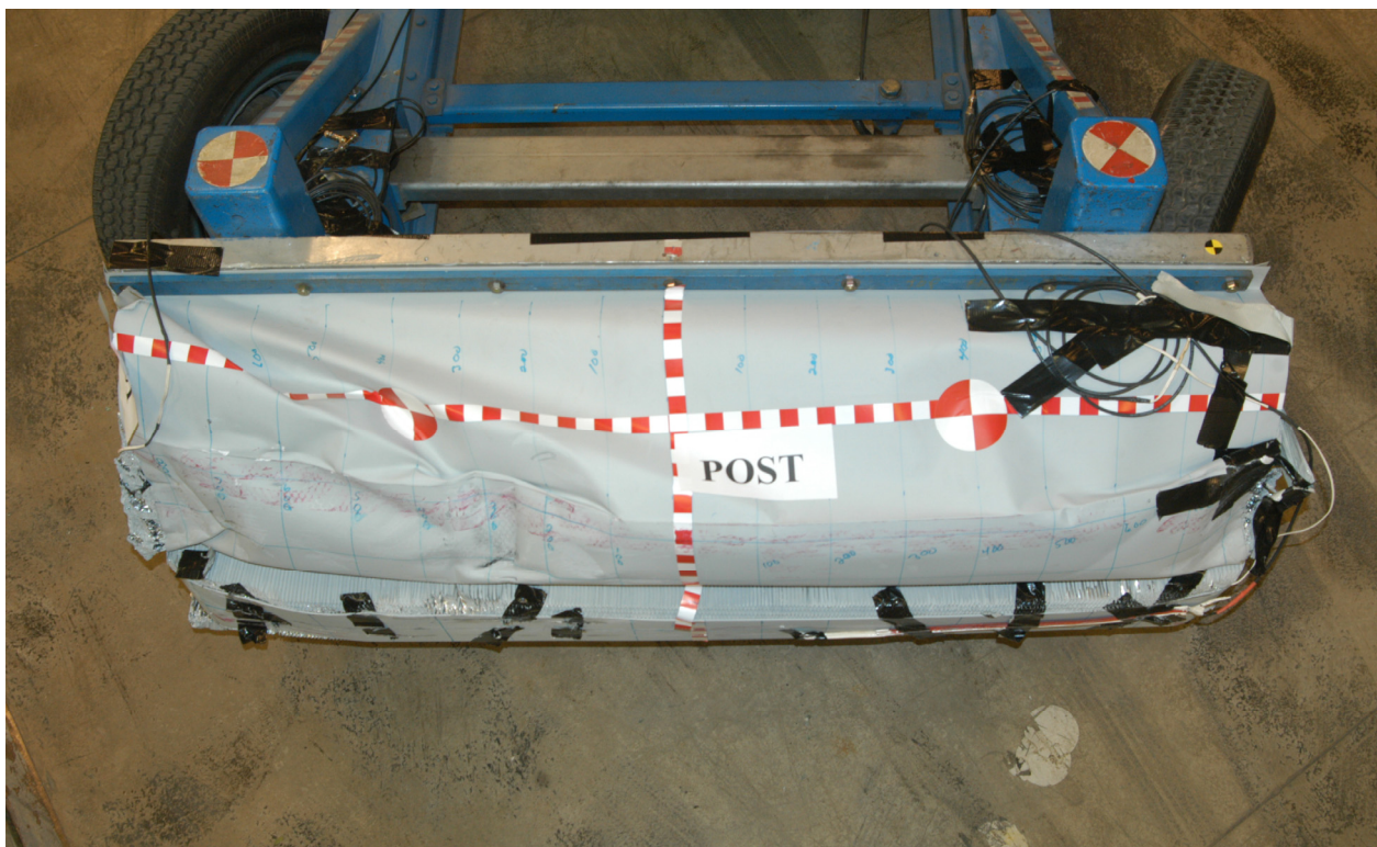
Figure A-42: Post test overhead view of MDB barrier face
