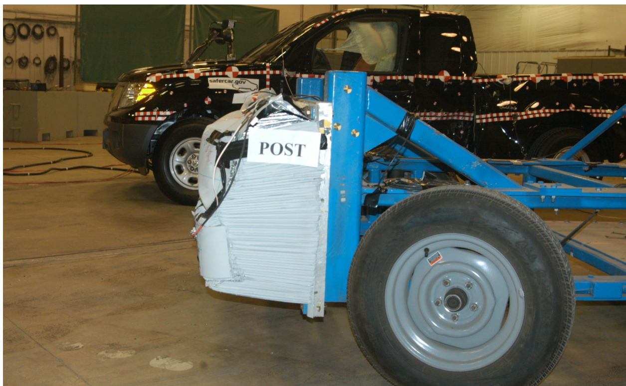
Figure A-46: Post test left side view of MDB barrier face
