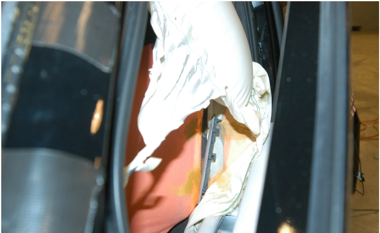
Figure A-34: Post test driver shoulder clearance
