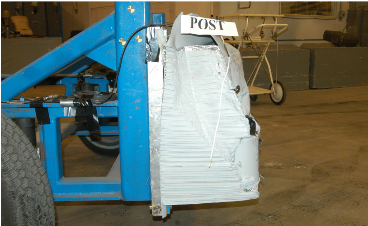
Figure A-44: Post test right side view of MDB barrier face
