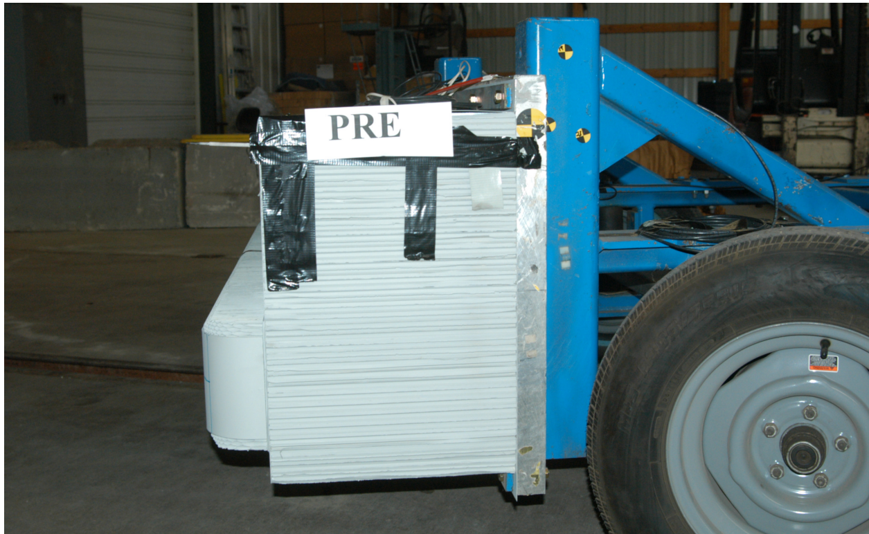
Figure A-45: Pre test left side view of MDB barrier face
