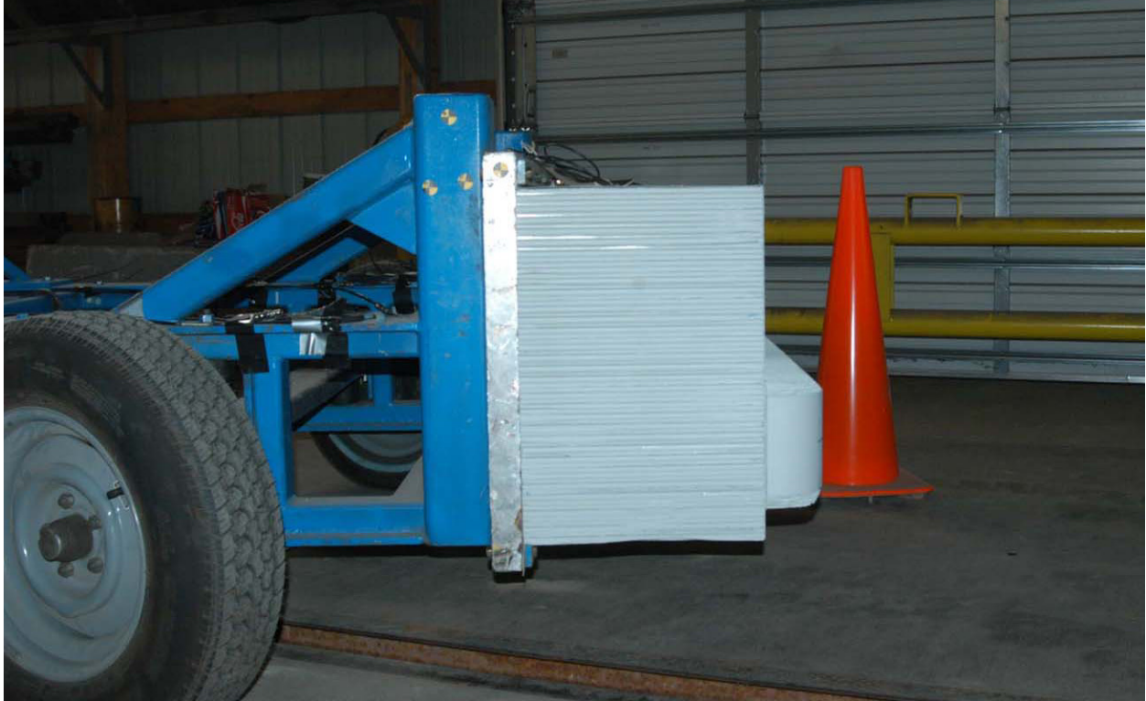
Figure A-43: Pre test right side view of MDB barrier face
