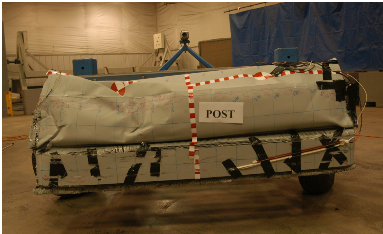
Figure A-40: Post test front view of MDB barrier face
