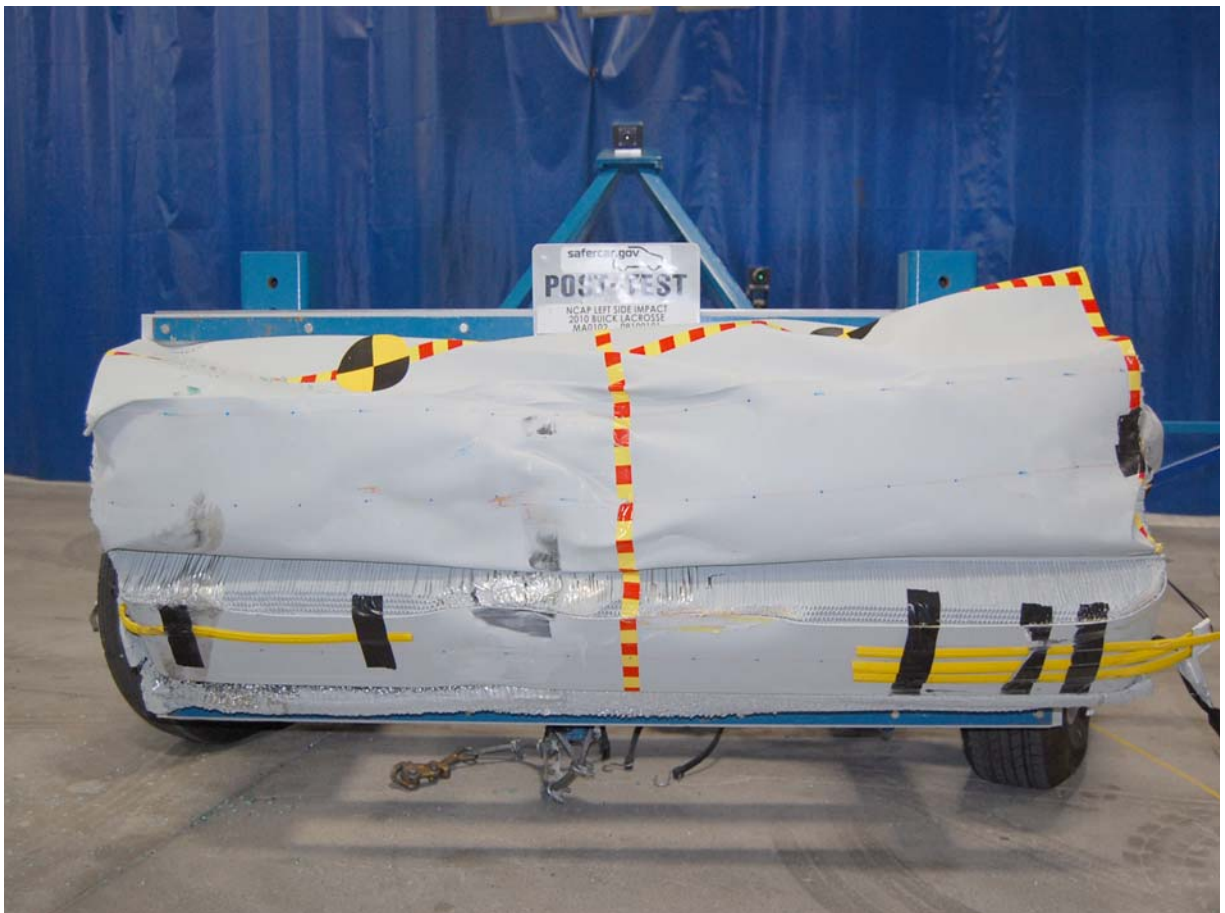
Post-Test Front View of Deformable Barrier
