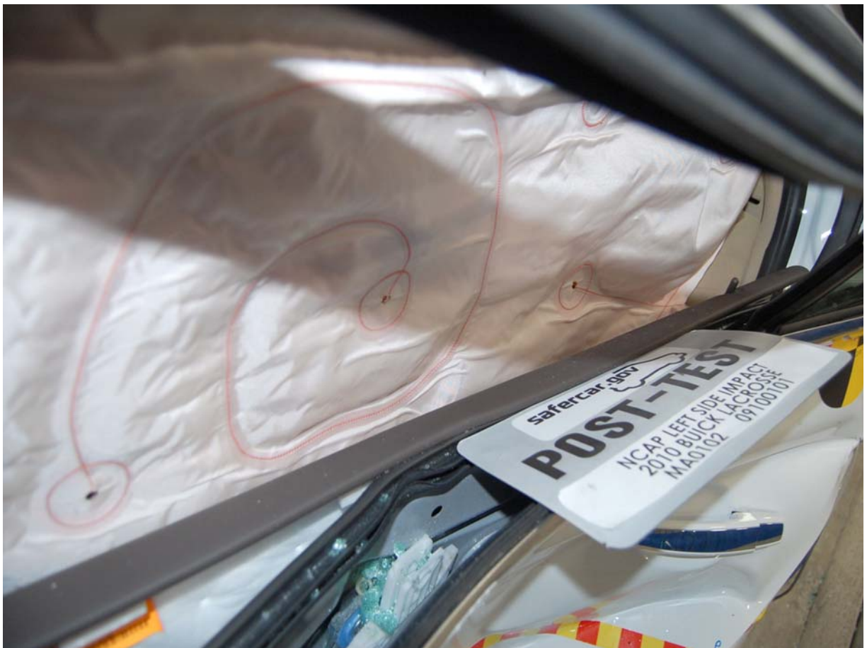
Post-Test Passenger Dummy Clearance From Door
