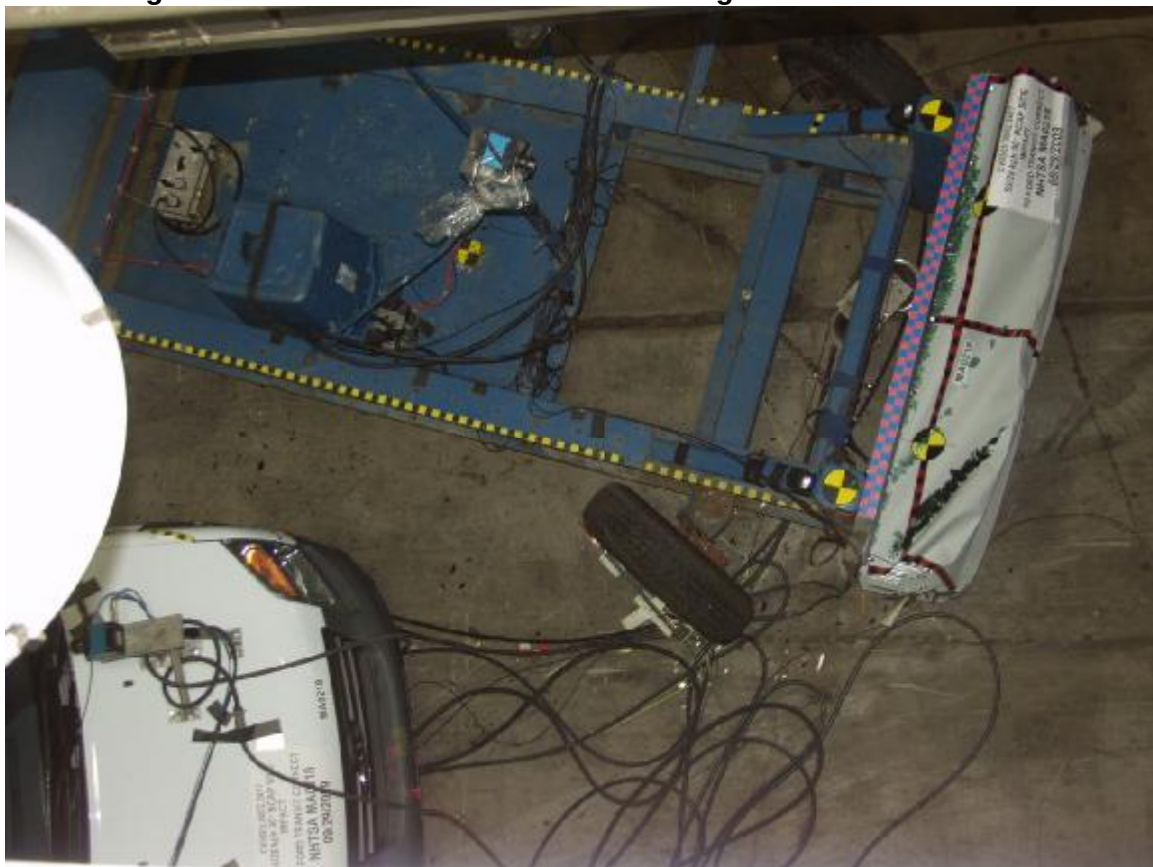
Figure A-32: Post-Test Overhead View of MDB and Vehicle
