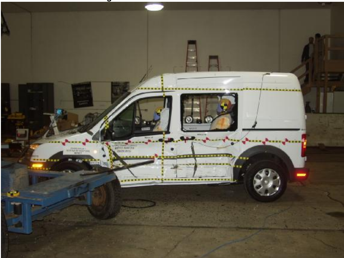
Figure A-10: Post-Test Left Side View
