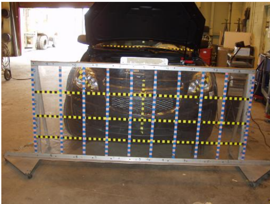
Figure A-1: Load Cell Locations
