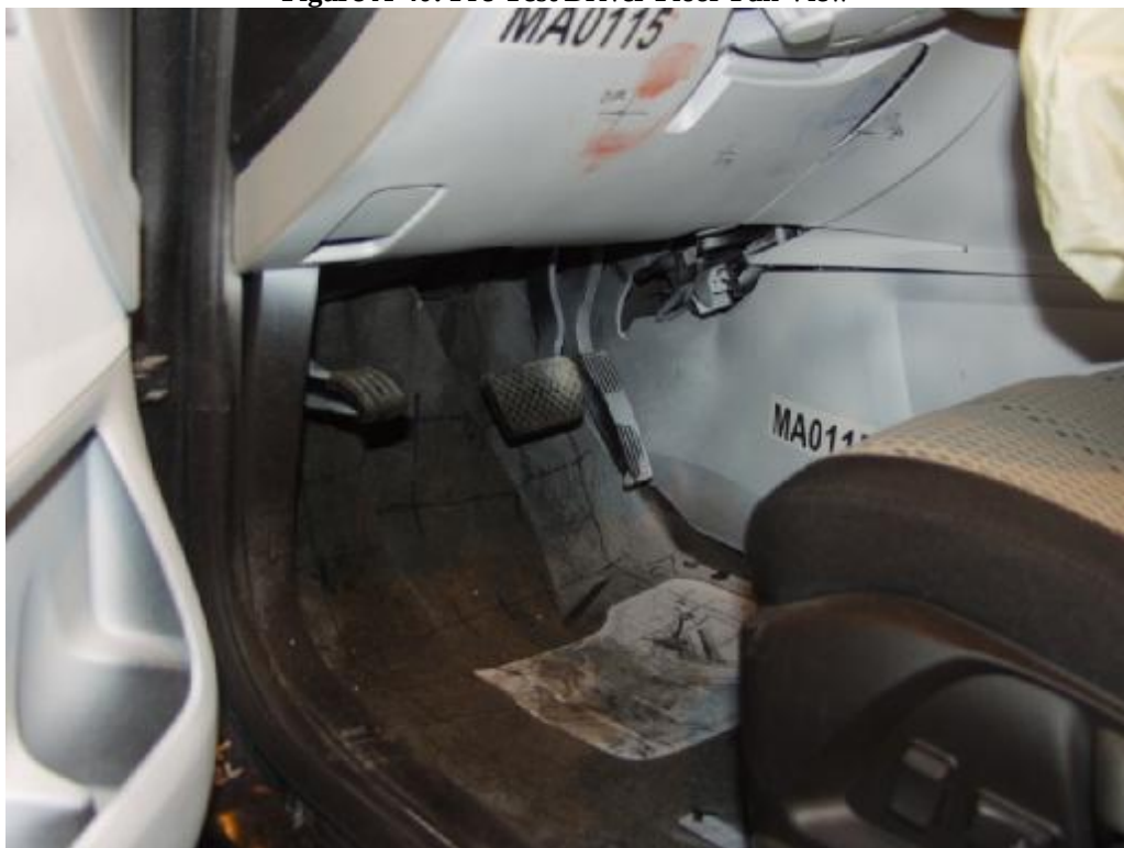
Figure A-41: Post-Test Driver Floor Pan View
