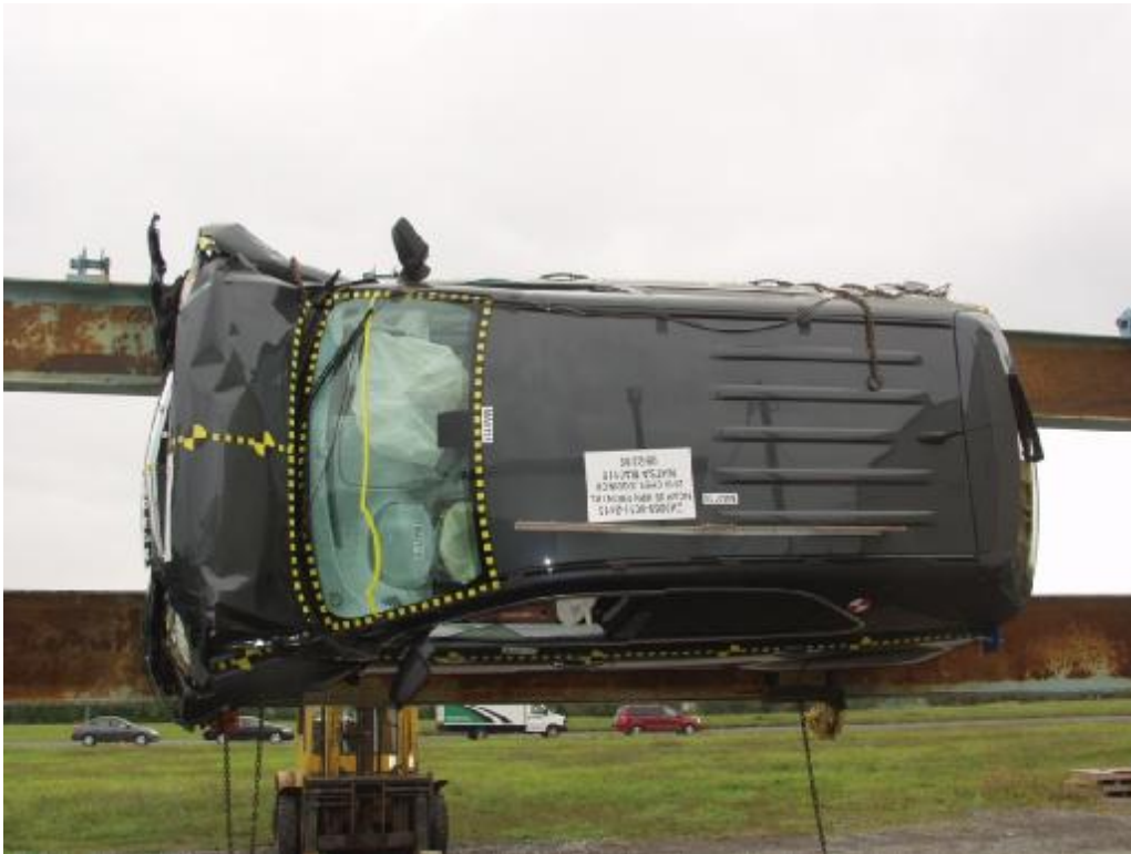
Figure A-60: Rollover View - 270°
