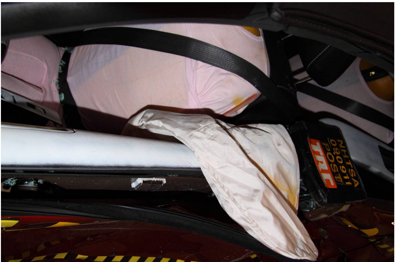
Figure A-47 Post-Test Left View of Front SID HIII and Door Clearance
