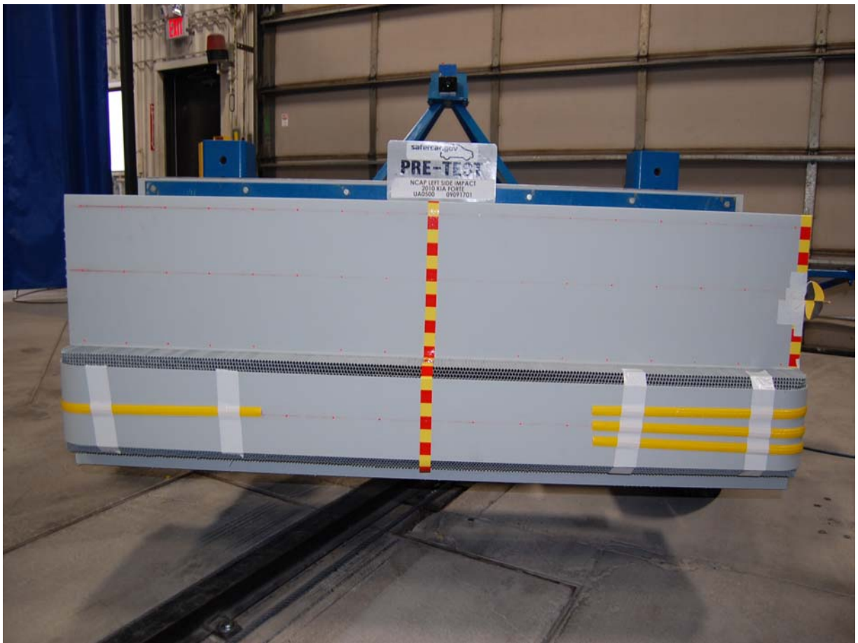
Pre-Test Front View of Deformable Barrier
