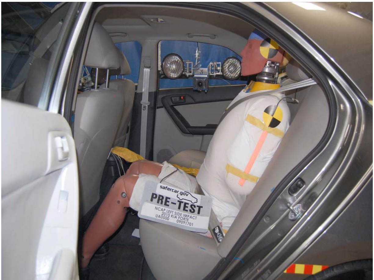
Pre-Test Passenger Dummy (Door Open)
