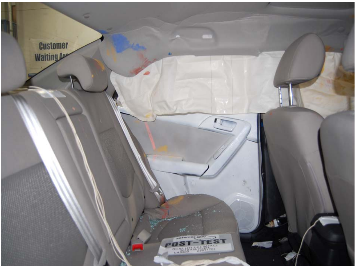
Post-Test Passenger Dummy Contact
