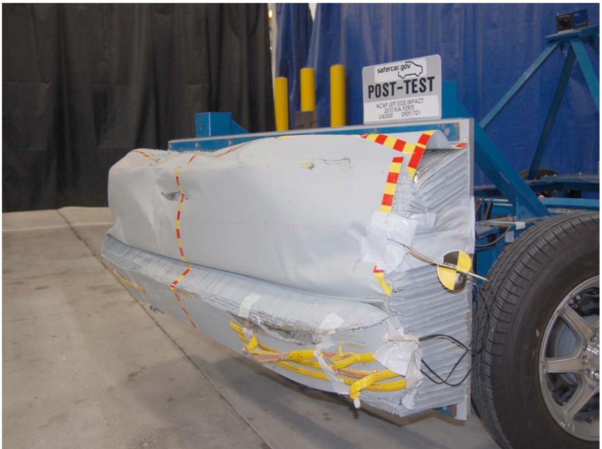
Post-Test Left Side View of Deformable Barrier
