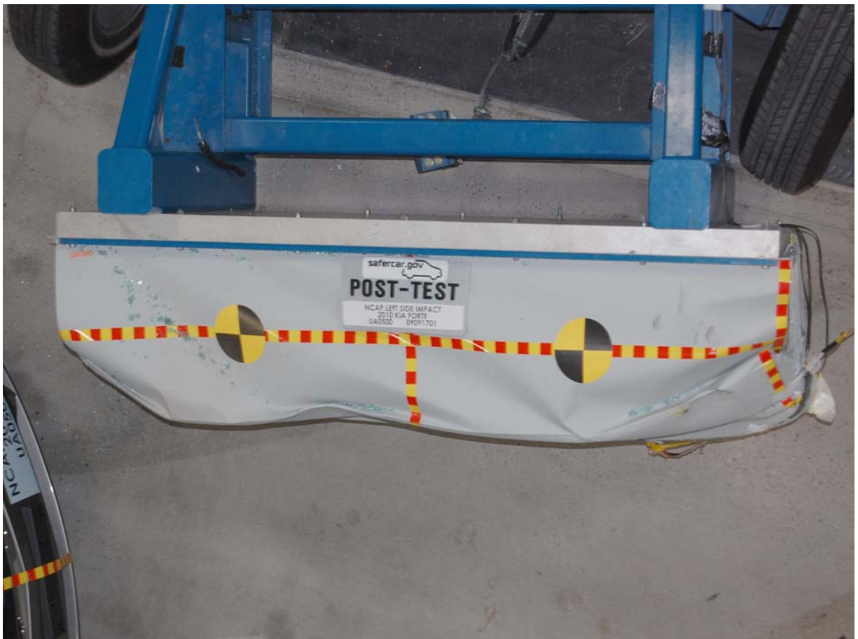
Post-Test Top View of Deformable Barrier
