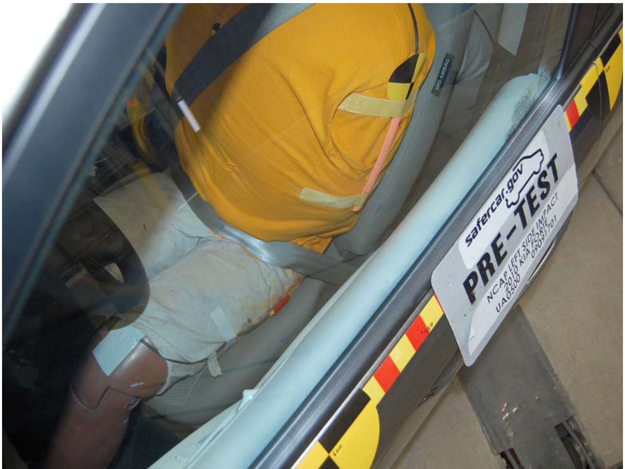
Pre-Test Driver Dummy Clearance From Door
