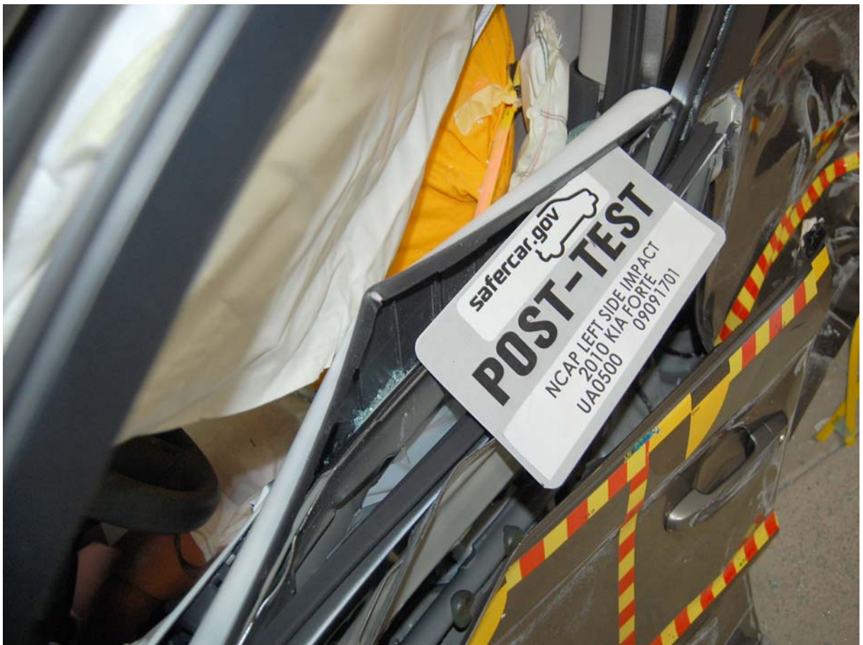
Post-Test Driver Dummy Clearance From Door
