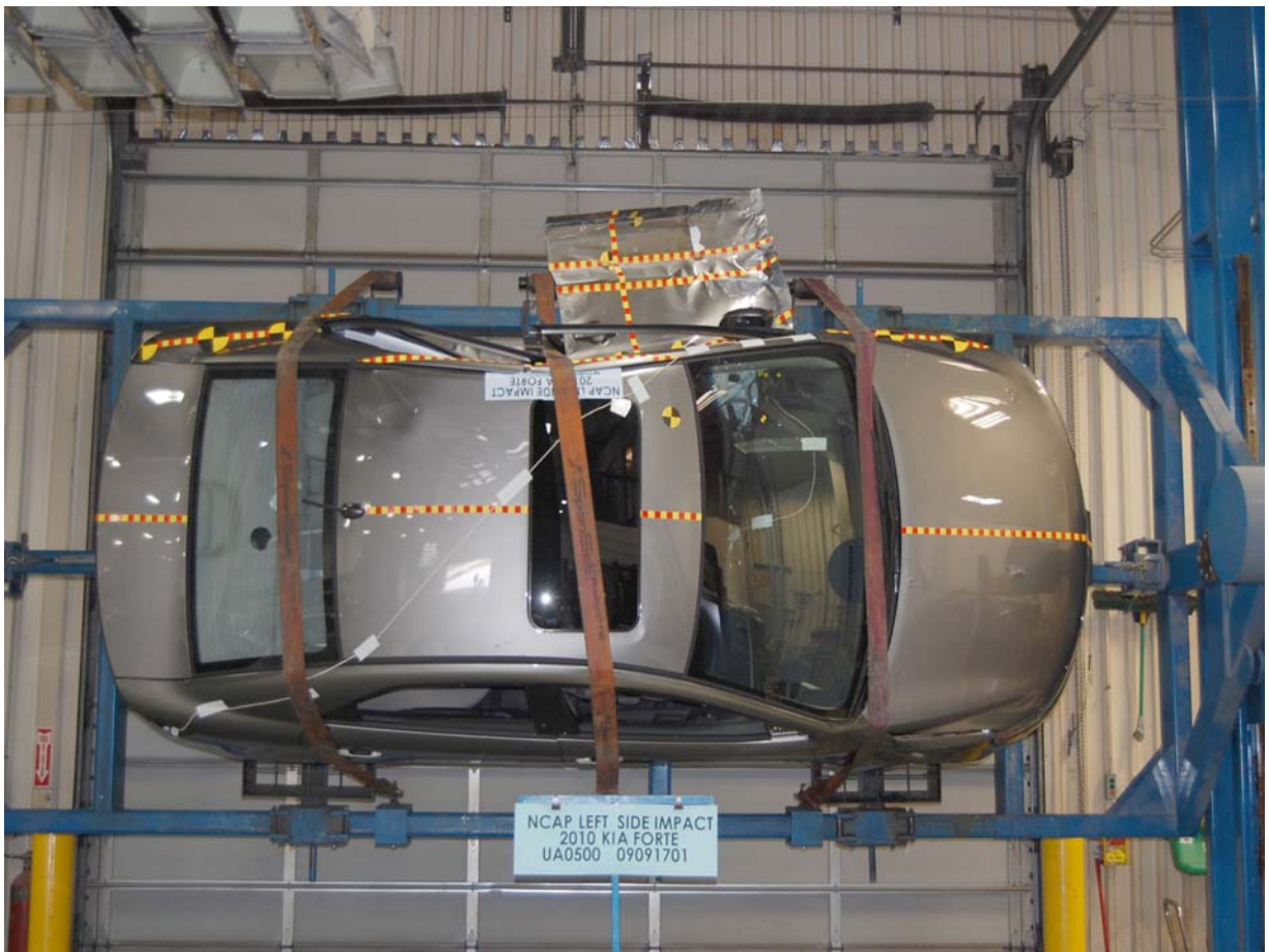
Vehicle on Rollover Device (270 Degrees)
