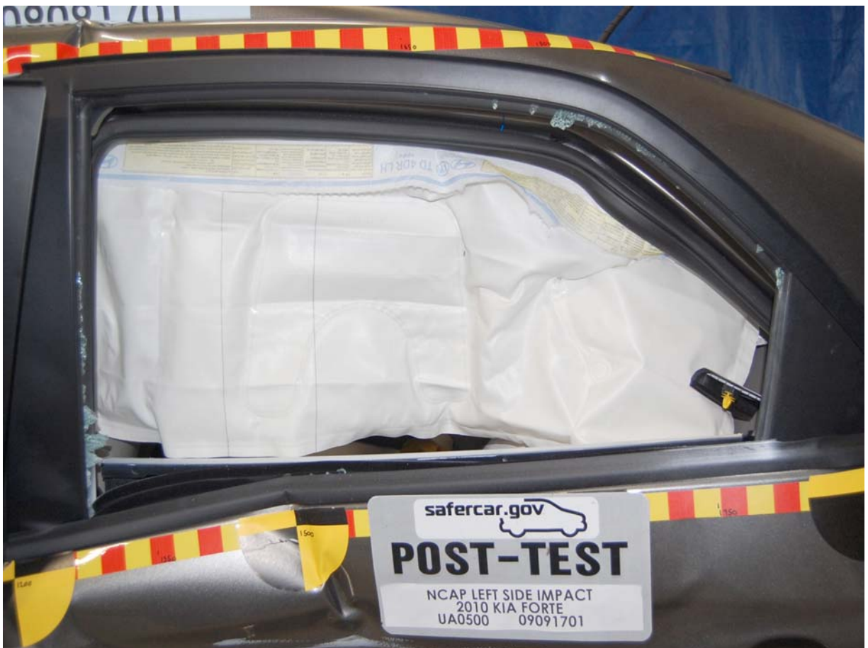
Post-Test Passenger Dummy (Through Window)
