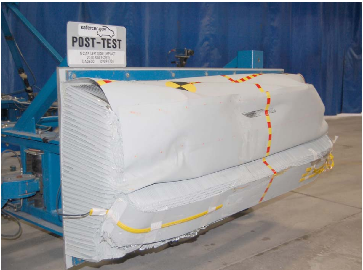
Post-Test Right Side View of Deformable Barrier
