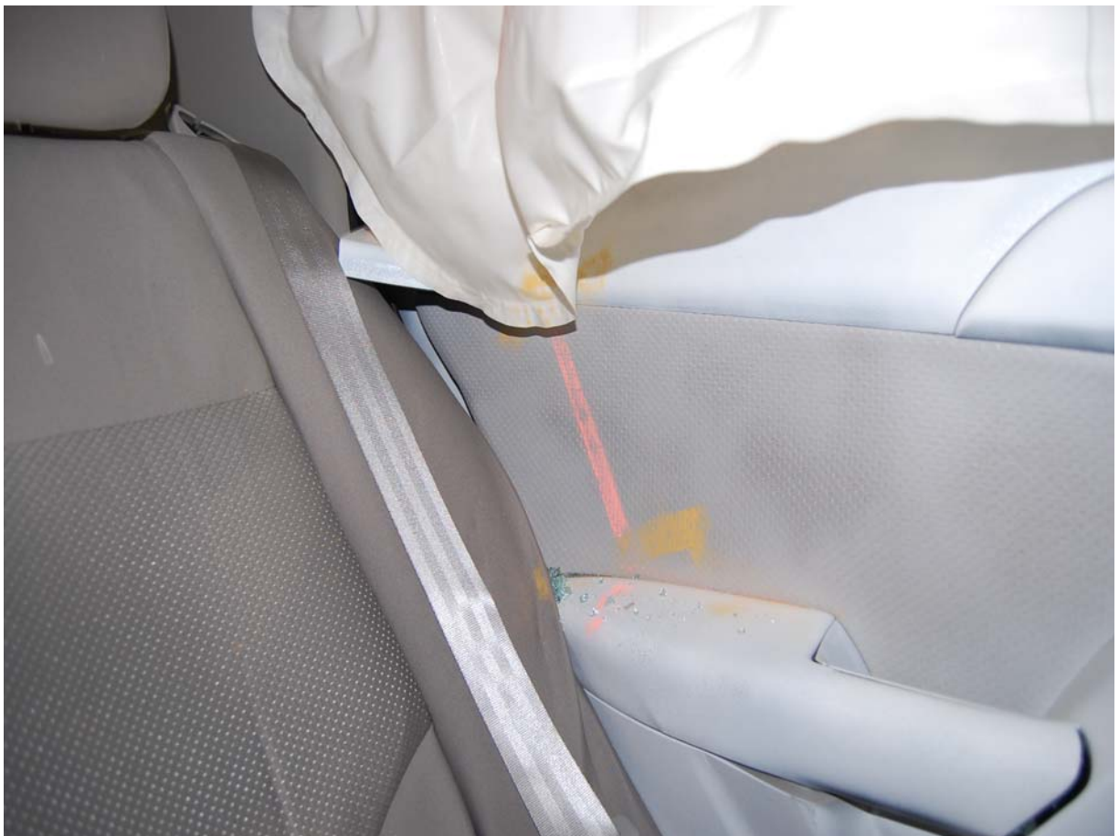
Post-Test Passenger Dummy Upper Torso Contact
