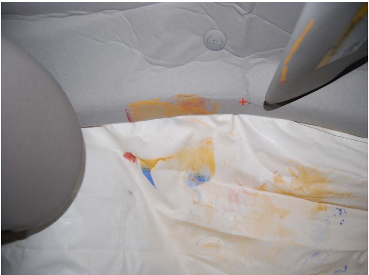
Post-Test Driver Dummy Head Contact View
