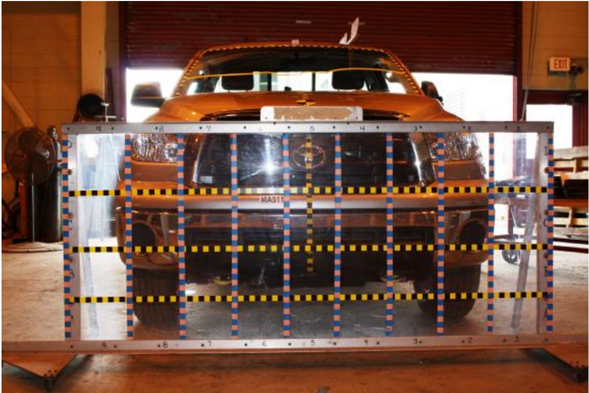
Figure A-1: Load Cell Locations
