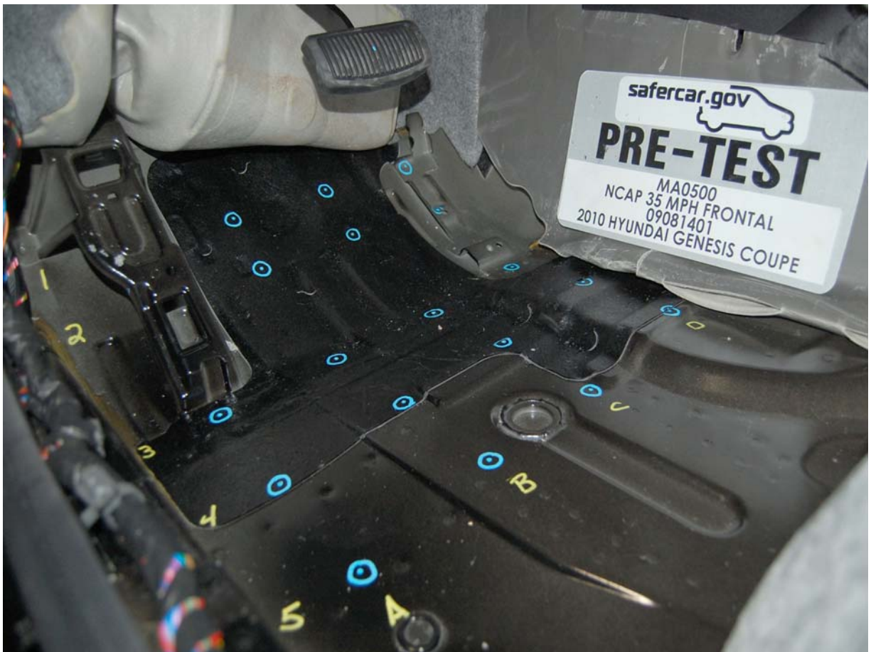
Pre-Test Driver's Side Floorpan
