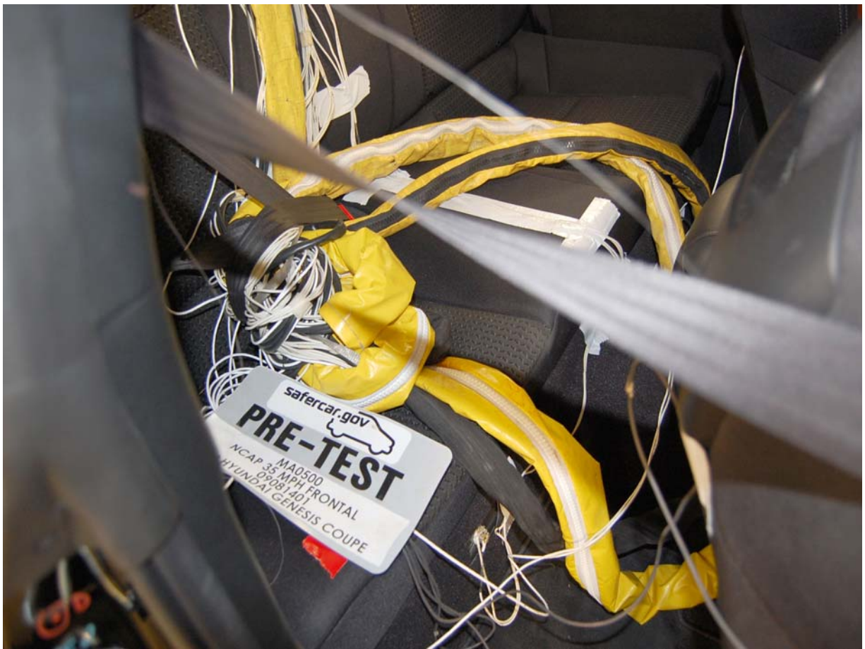
Pre-Test Dummy Cable Routing
