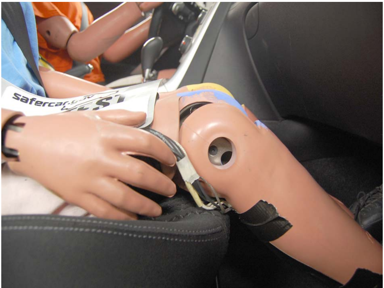
Pre-Test Passenger's Side Knee Bolster
