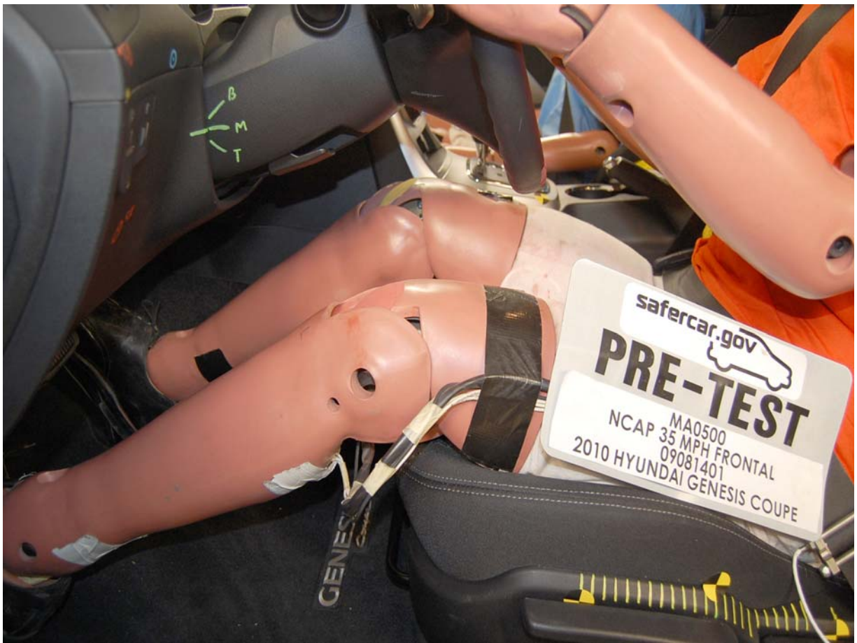
Pre-Test Driver's Side Knee Bolster
