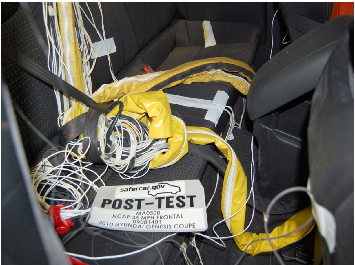
Post-Test Dummy Cable Routing
