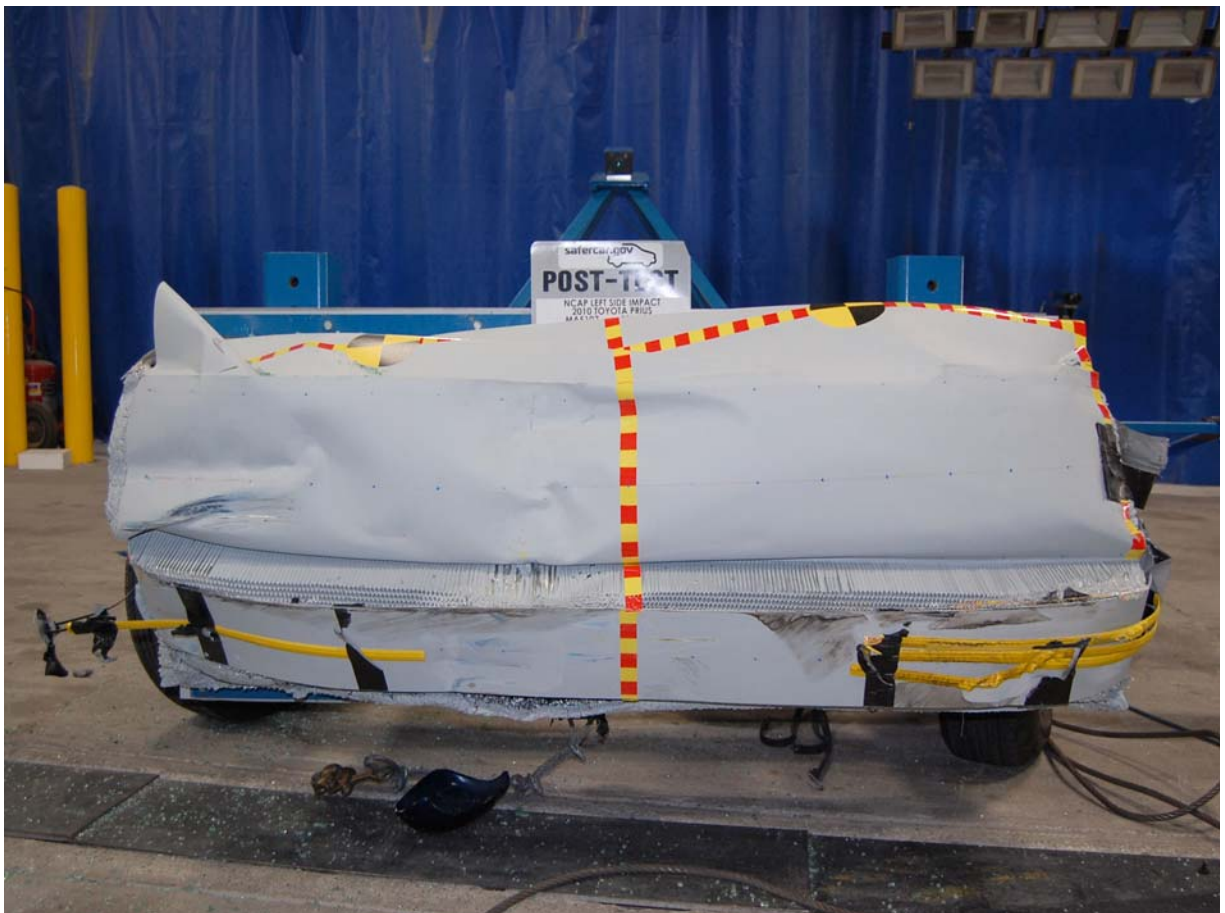
Post-Test Front View of Deformable Barrier
