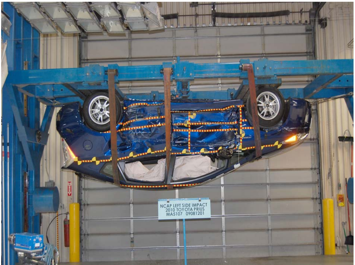
Vehicle on Rollover Device (180 Degrees)
