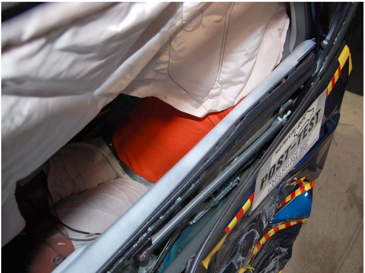
Post-Test Passenger Dummy Clearance From Door
