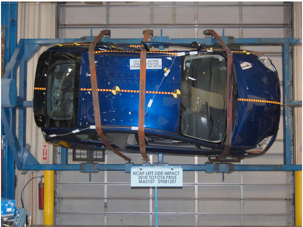
Vehicle on Rollover Device (270 Degrees)
