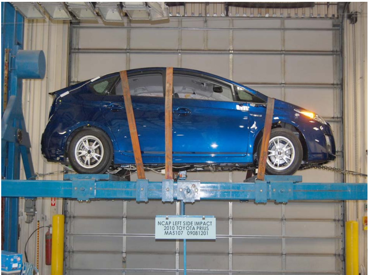
Vehicle on Rollover Device (360 Degrees)
