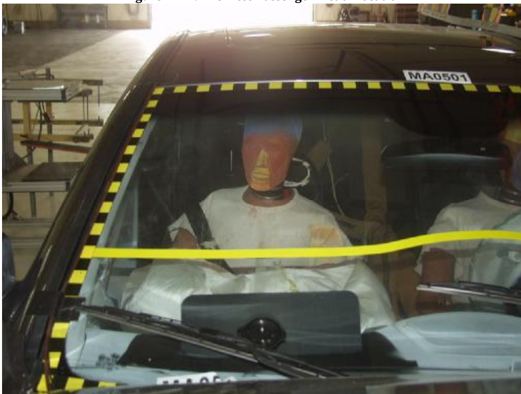
Figure A-45: Post-Test Passenger Head Location
