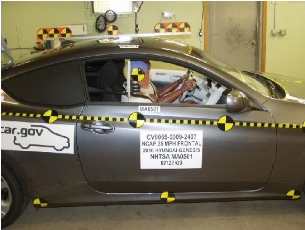
Figure A-46: Pre-Test Passenger Position View
