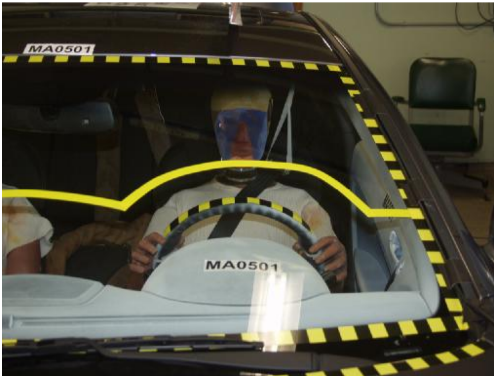
Figure A-30: Pre-Test Driver Head Location
