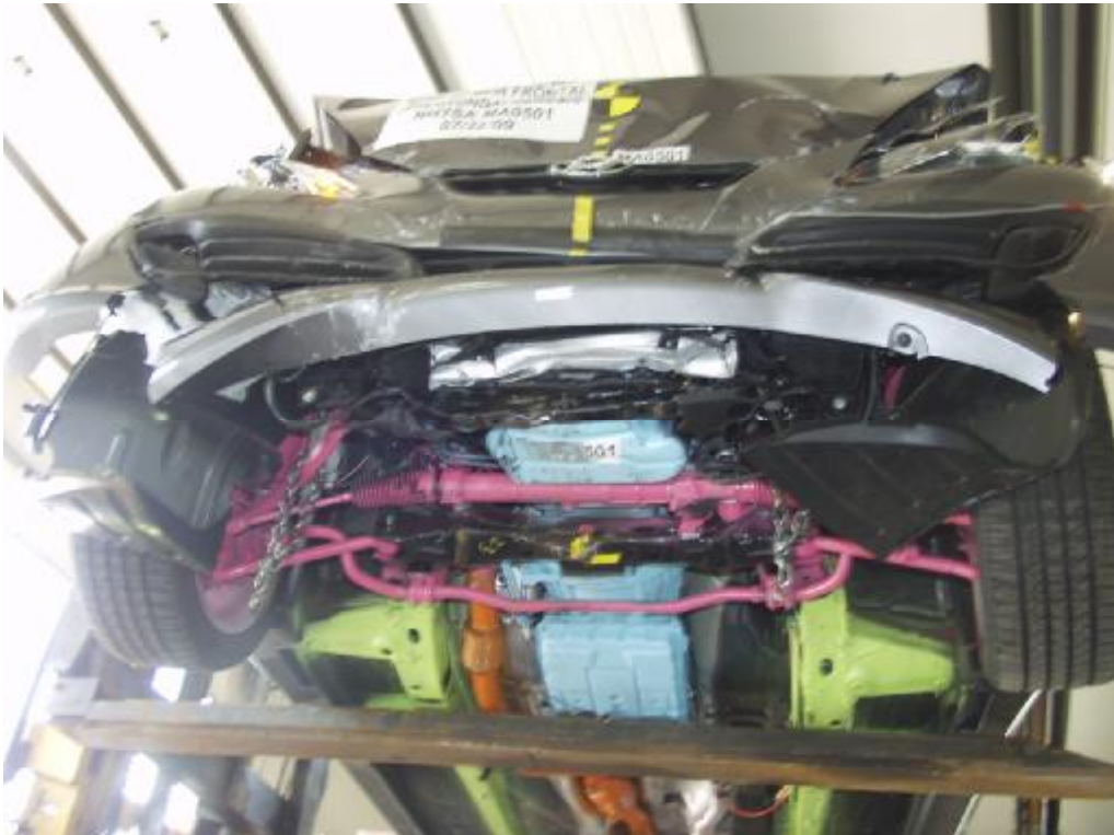
Figure A-25: Post-Test Front Underbody View
