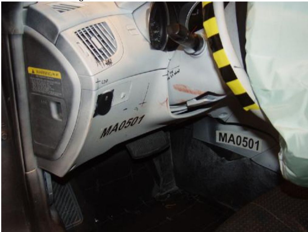
Figure A-39: Post-Test Driver Knee Bolster View
