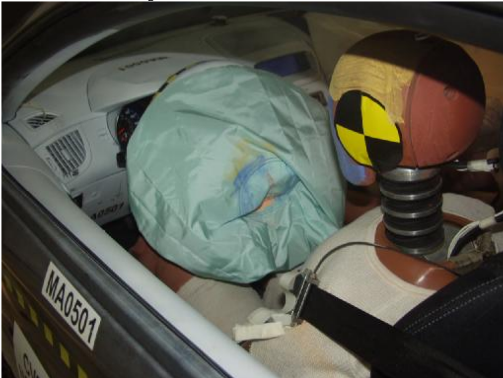
Figure A-43: Post-Test Driver Contact to Airbag
