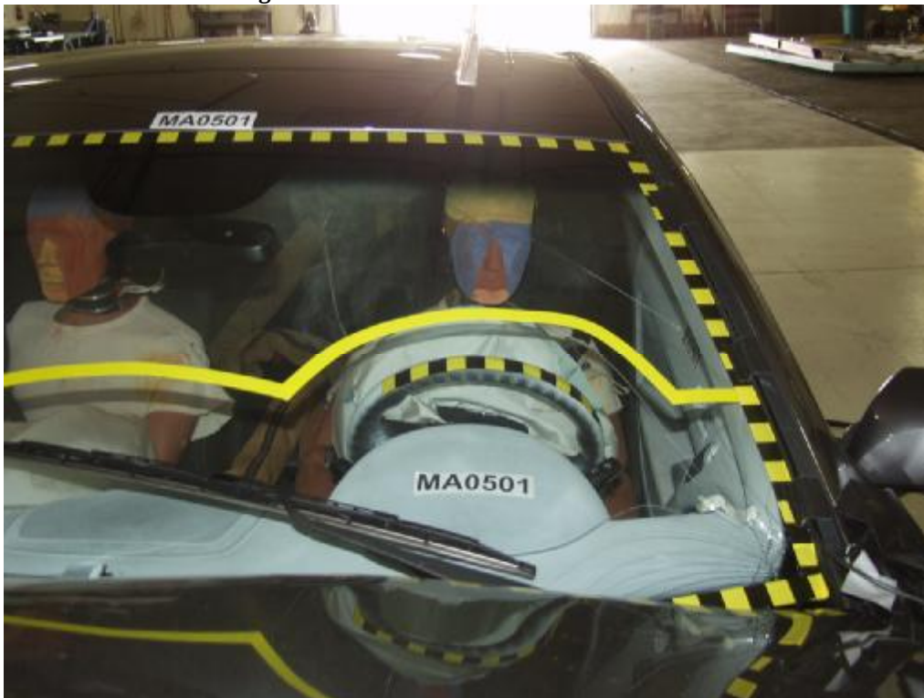
Figure A-31: Post-Test Driver Head Location
