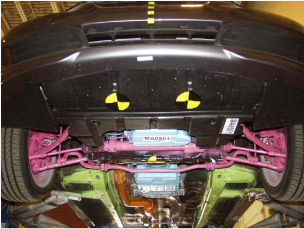
Figure A-24: Pre-Test Front Underbody View
