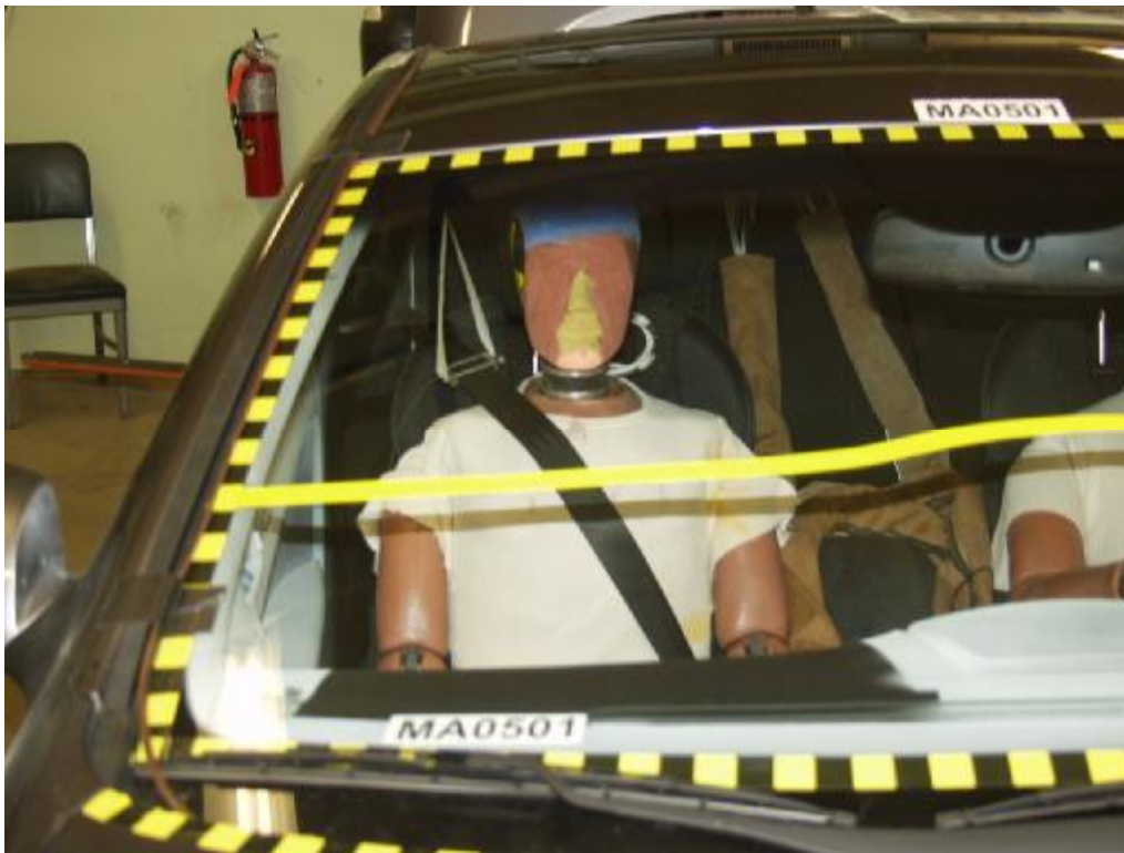
Figure A-44: Pre-Test Passenger Head Location
