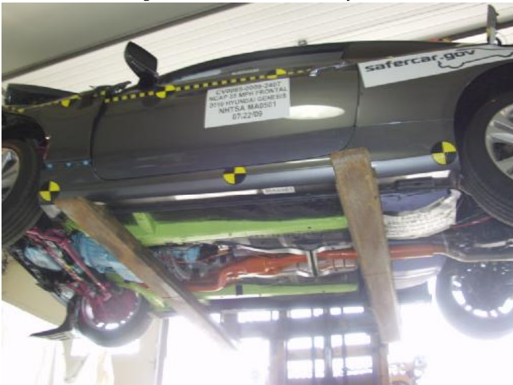
Figure A-27: Post-Test Mid Underbody View
