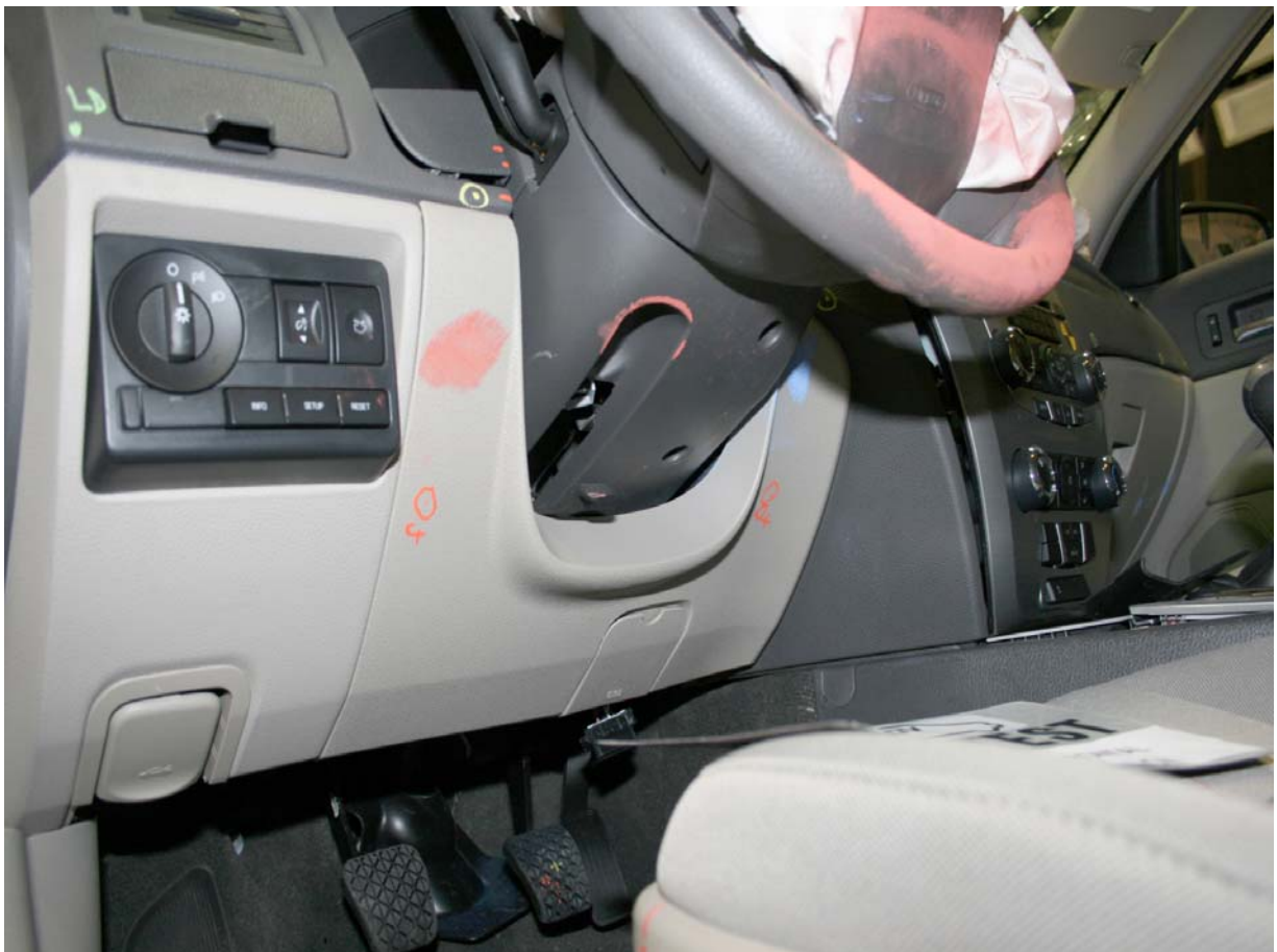
Post-Test Driver's Side Knee Bolster
