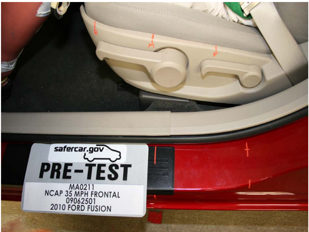
Pre-Test Driver's Seat Fore-Aft Markings
