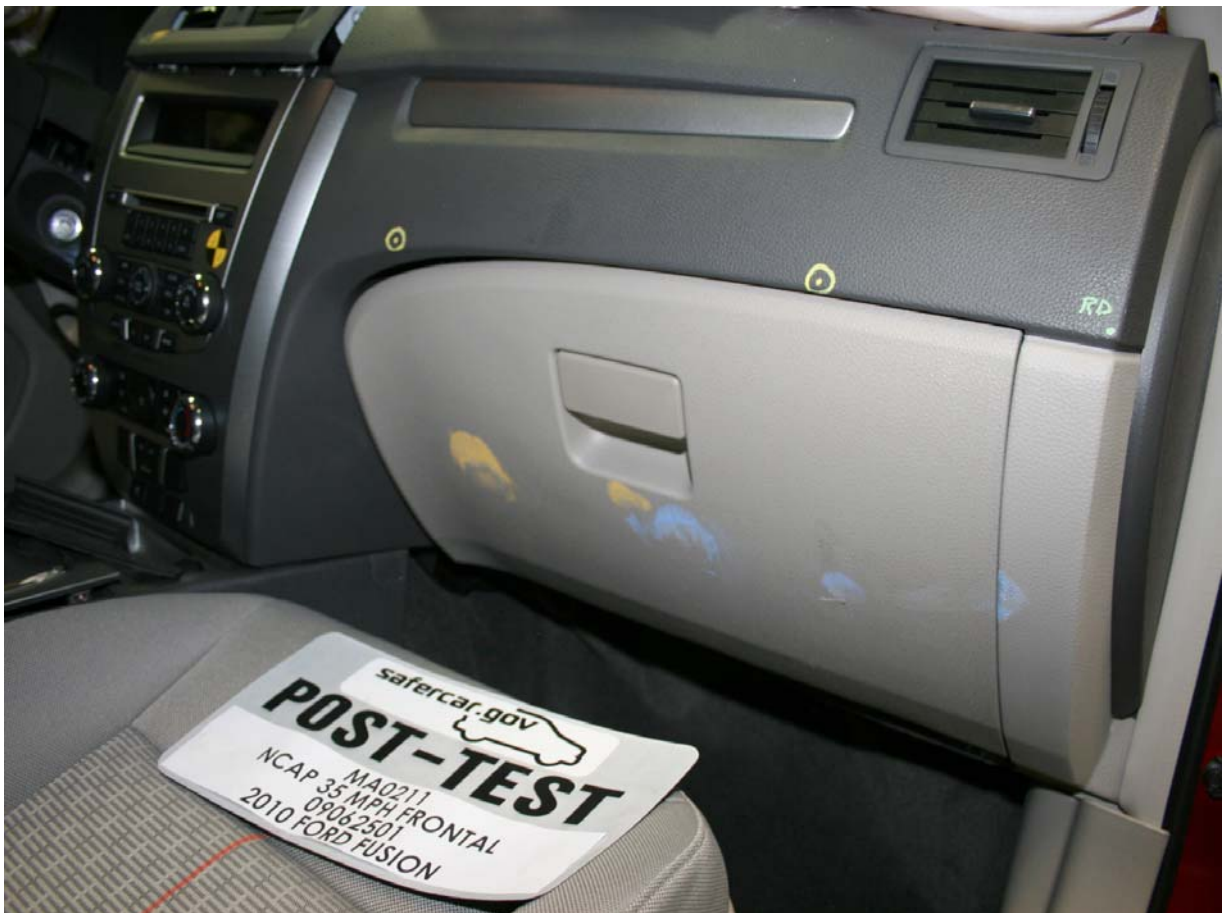
Post-Test Passenger Dummy Knee Contact
