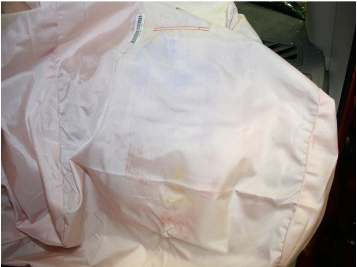
Post-Test Passenger Dummy Airbag Contact
