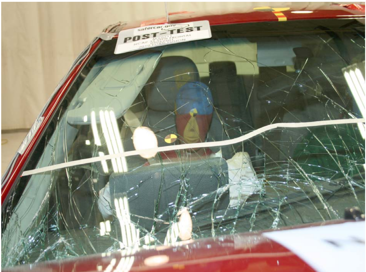
Post-Test Passenger Dummy Front View
