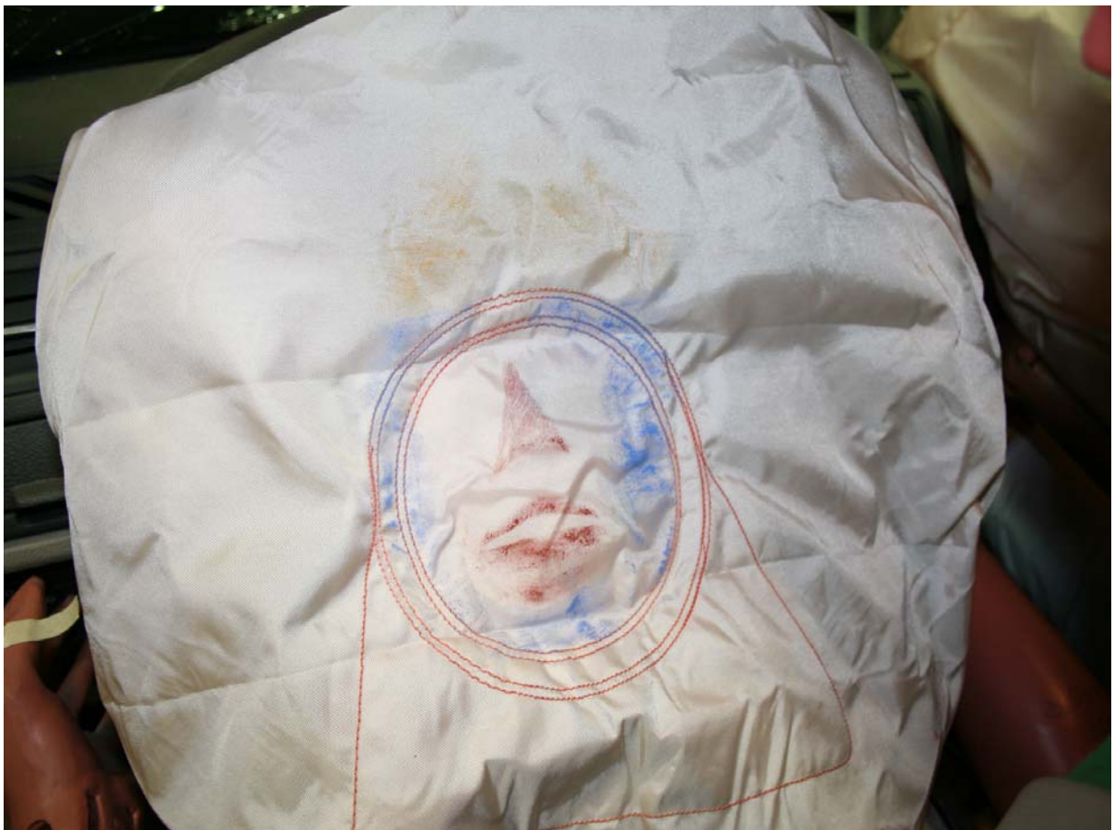
Post-Test Driver Dummy Airbag Contact
