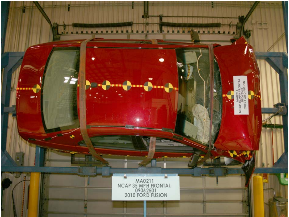
Vehicle at 270 Degrees on Static Rollover Device
