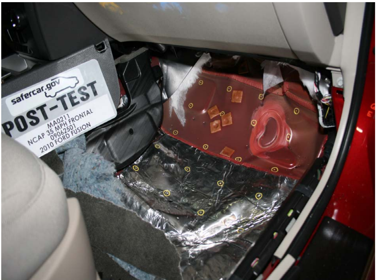
Post-Test Passenger's Side Floorpan
