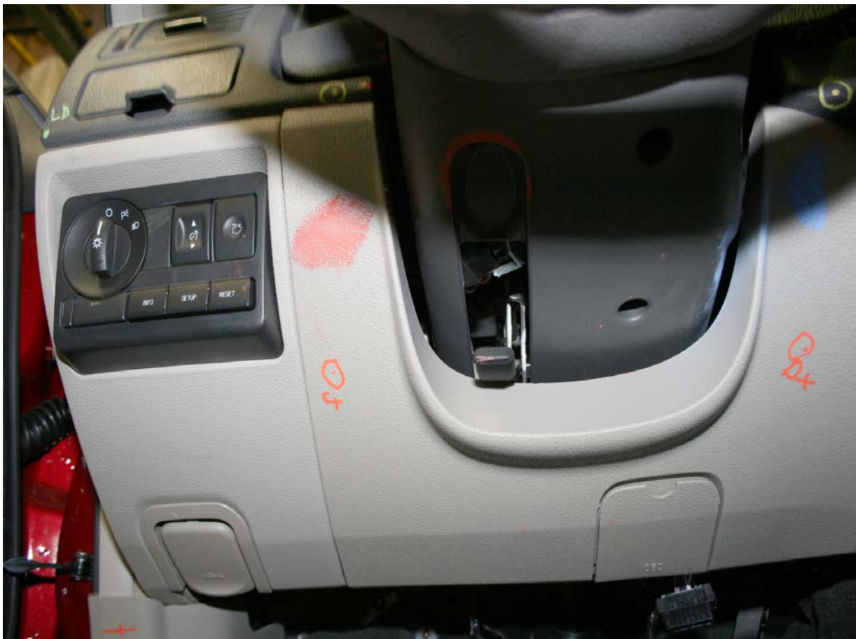
Post-Test Driver Dummy Left Knee Contact
