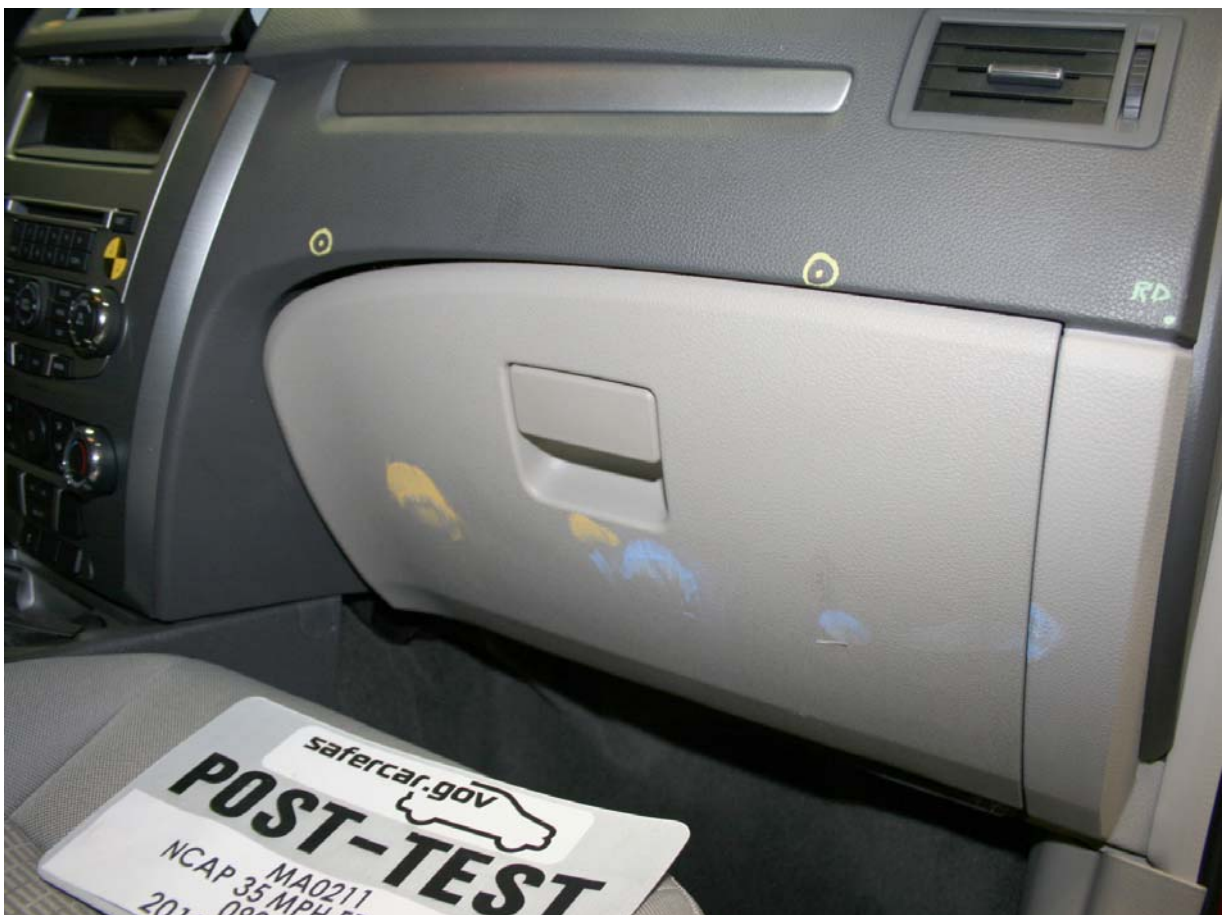
Post-Test Passenger's Side Knee Bolster
