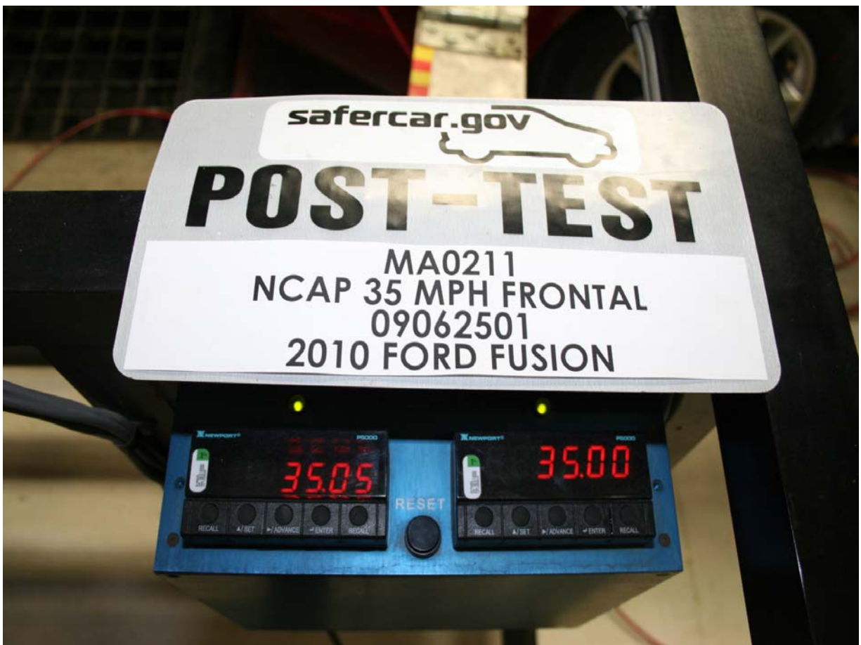
Post-Test Speed Trap Read-Out
