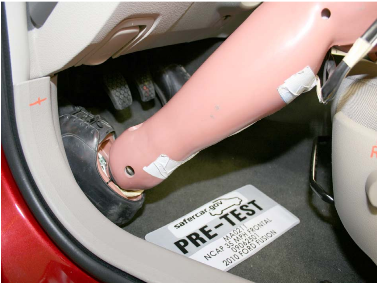
Pre-Test Driver Dummy Feet
