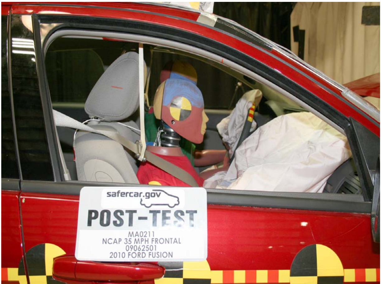
Post-Test Passenger Dummy Window View
