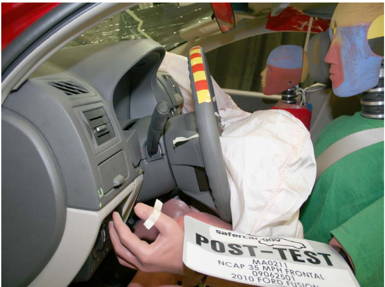
Post-Test View of Steering Column Shear Capsule
