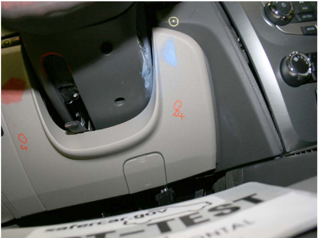
Post-Test Driver Dummy Right Knee Contact
