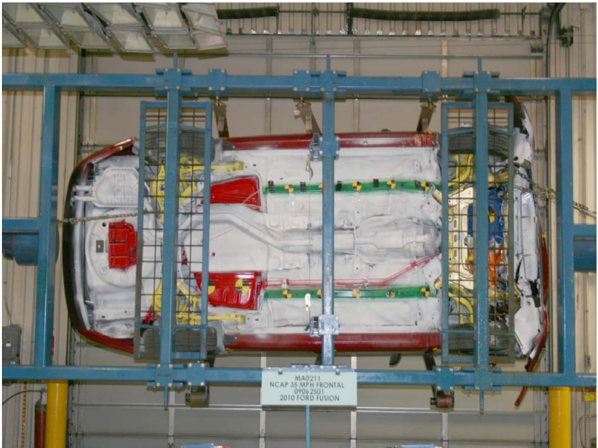
Vehicle at 90 Degrees on Static Rollover Device
