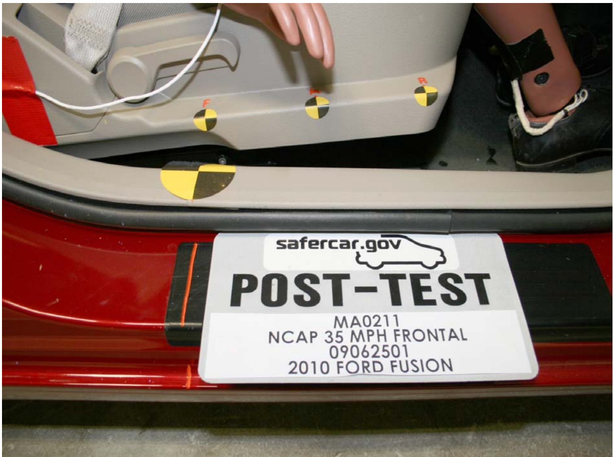
Post-Test Passenger's Seat Fore-Aft Markings
