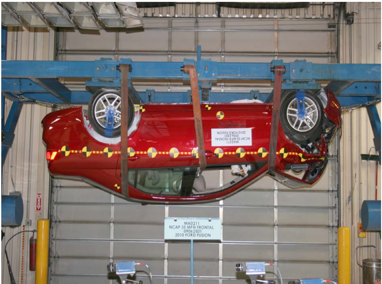
Vehicle at 180 Degrees on Static Rollover Device
