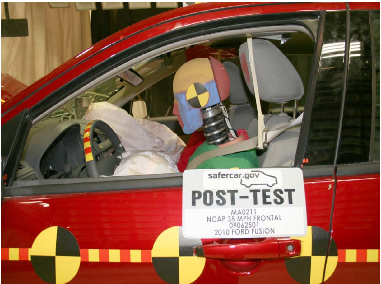
Post-Test Driver Dummy Window View
