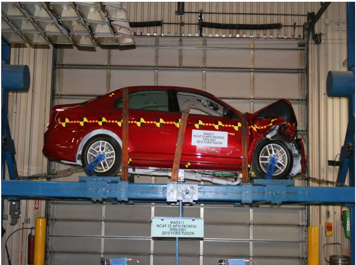
Vehicle at 0 Degrees on Static Rollover Device
