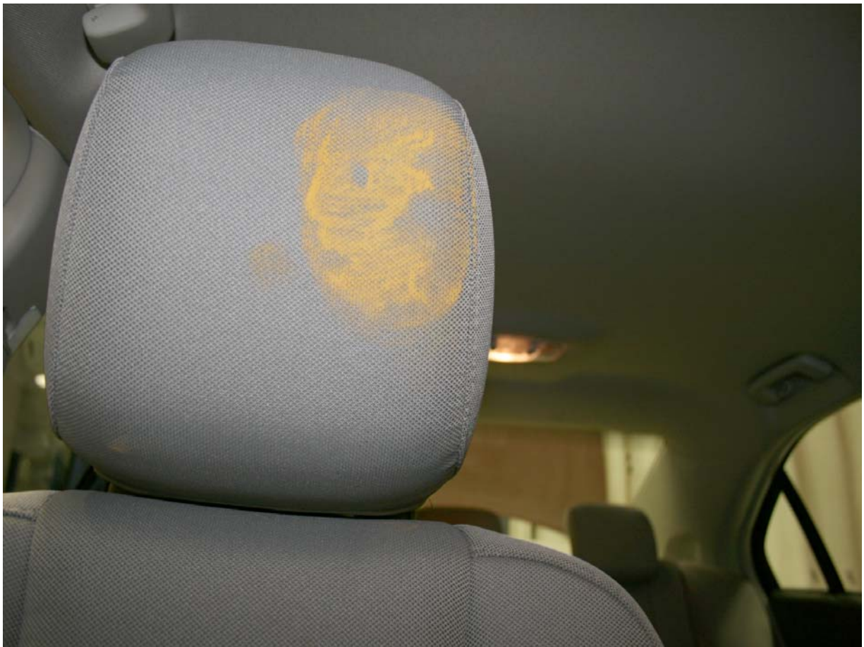
Post-Test Passenger Dummy Head Contact
