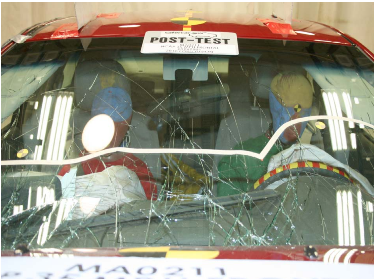
Post-Test Windshield View
