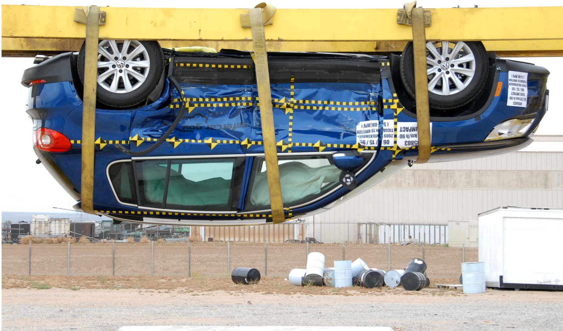
Figure A-63: Vehicle on Rollover Device (180°)
