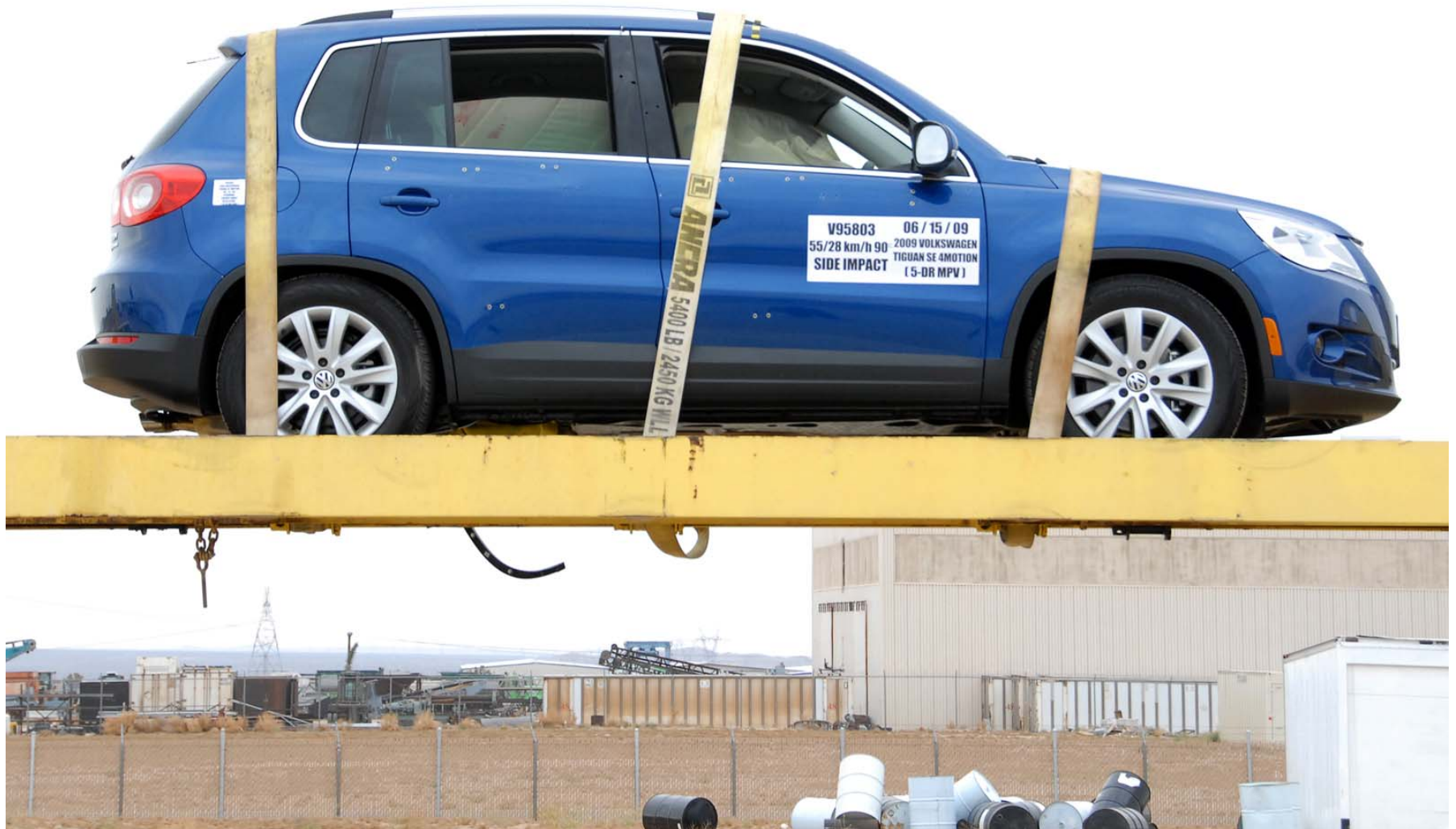
Figure A-61: Vehicle on Rollover Device (0°)
