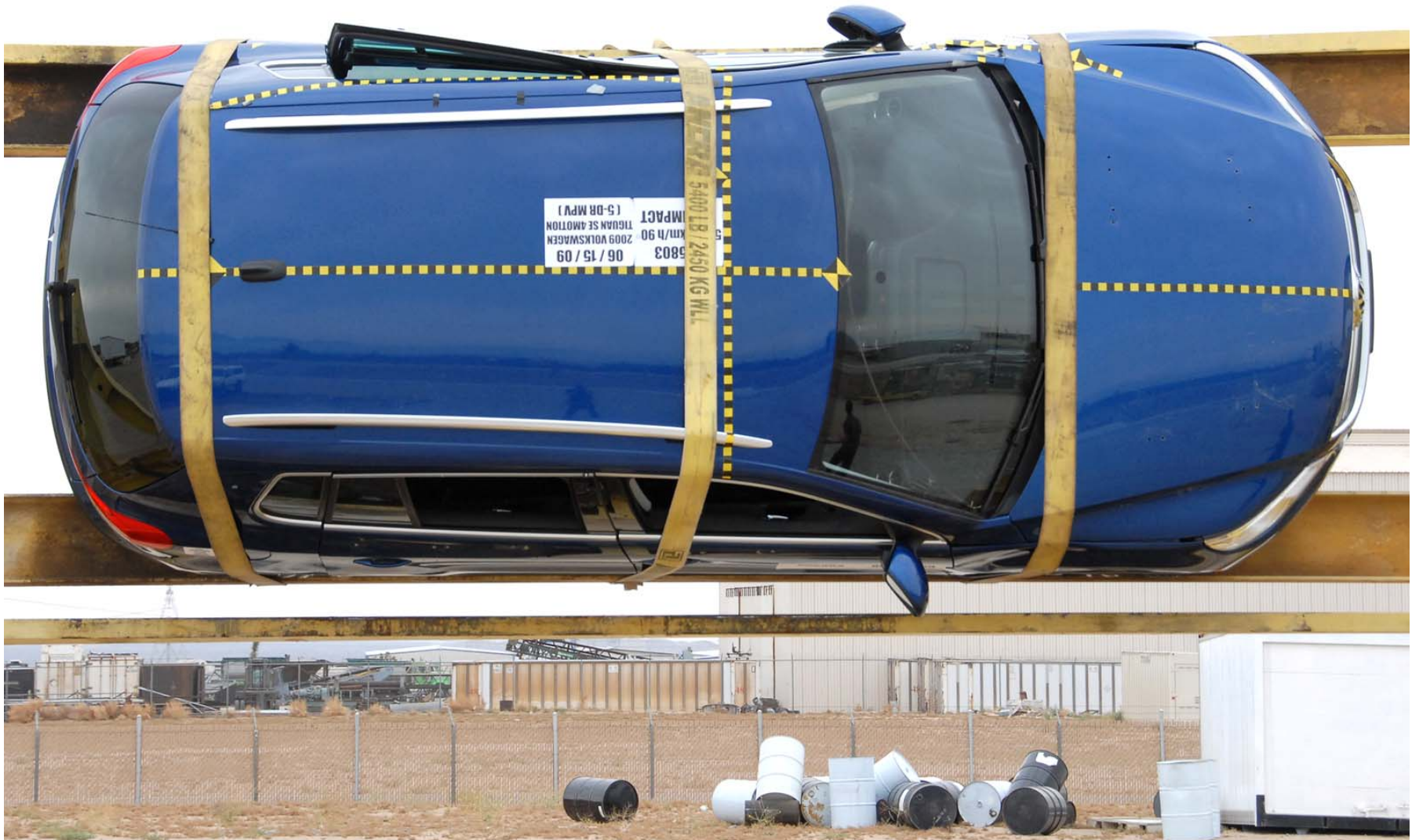
Figure A-62: Vehicle on Rollover Device (90°)
