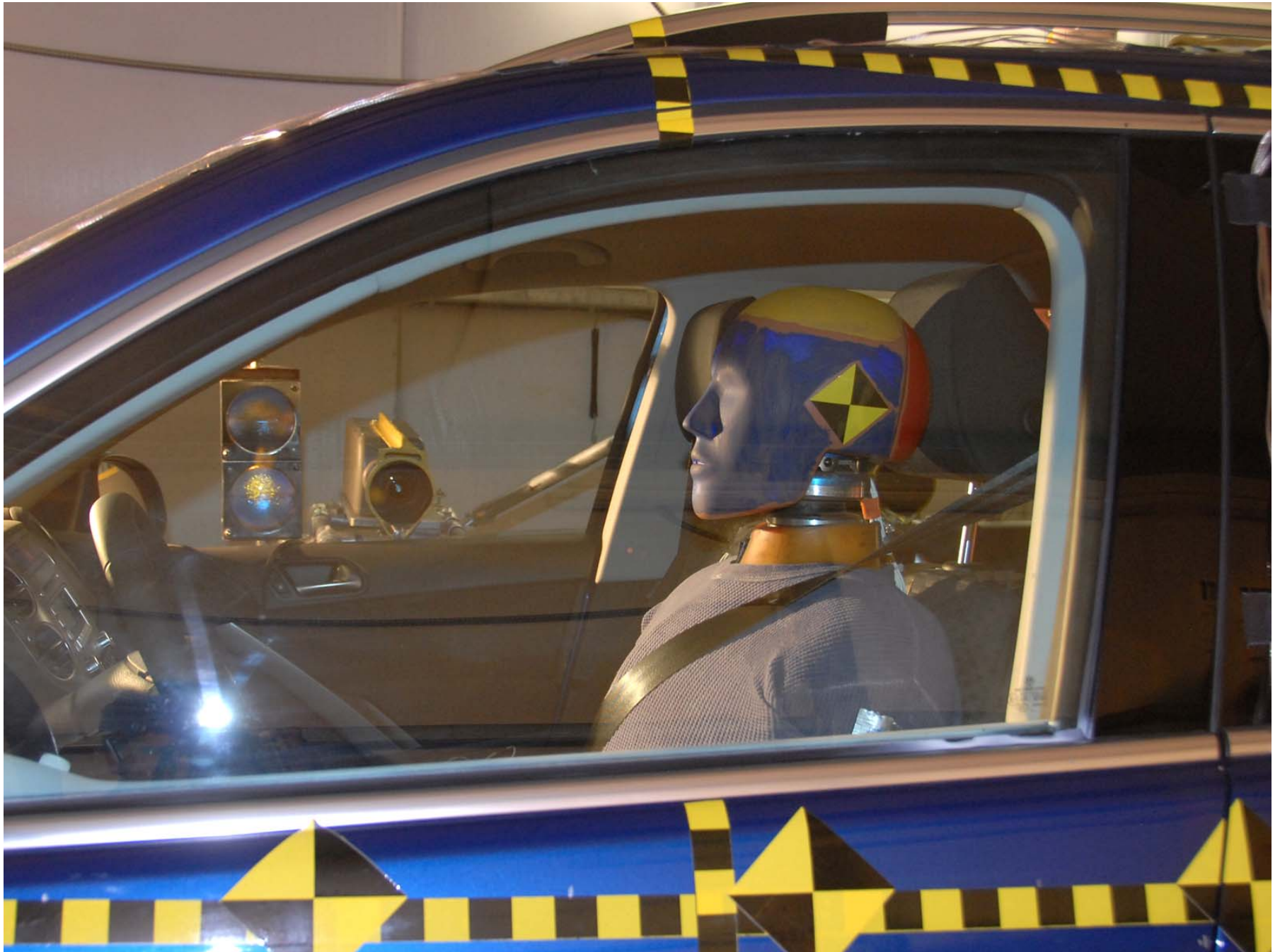
Figure A-36: Pre-Test Driver Dummy (Through Window)
