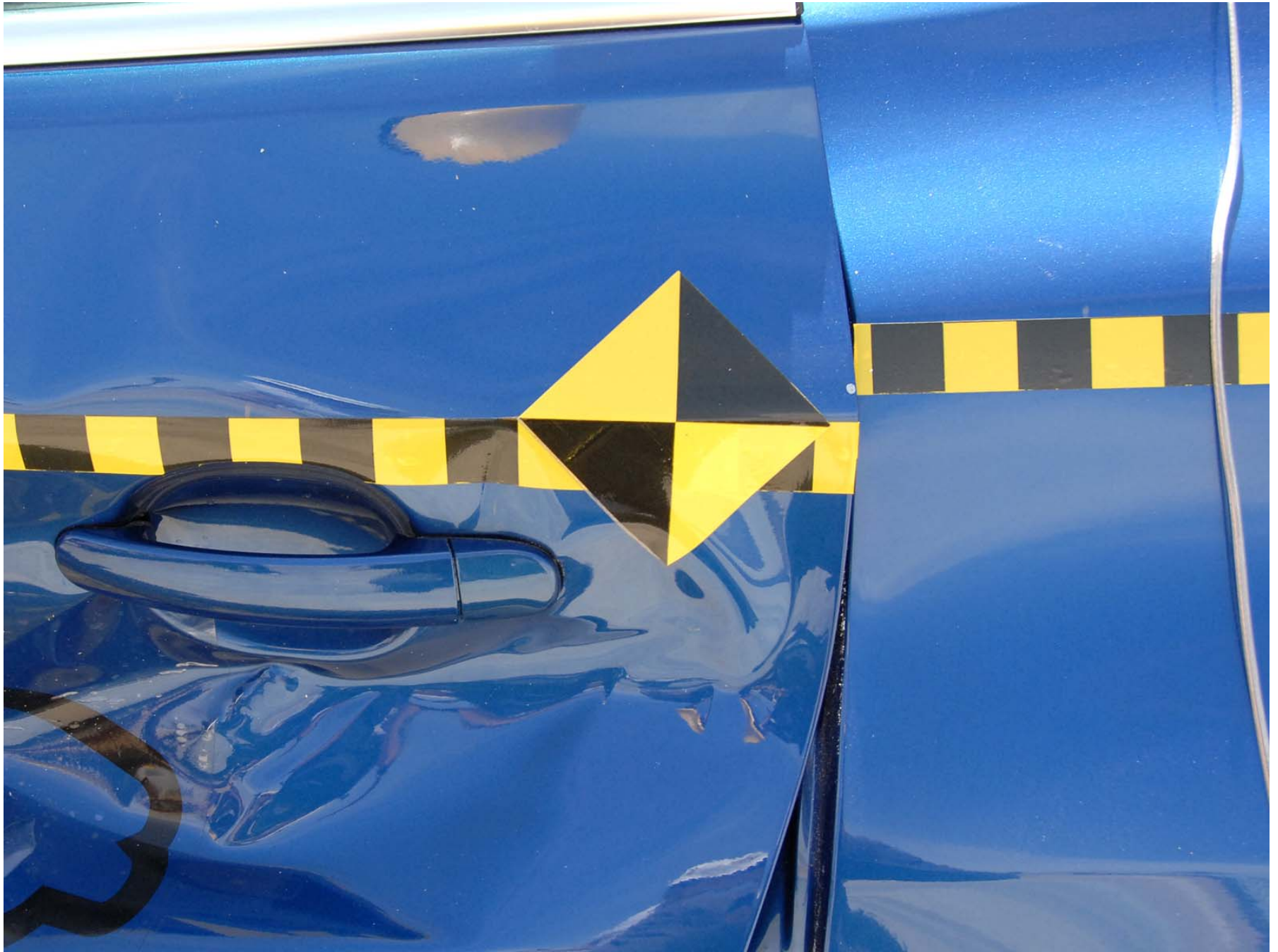
Figure A-34: Post-Test Left Rear Door
