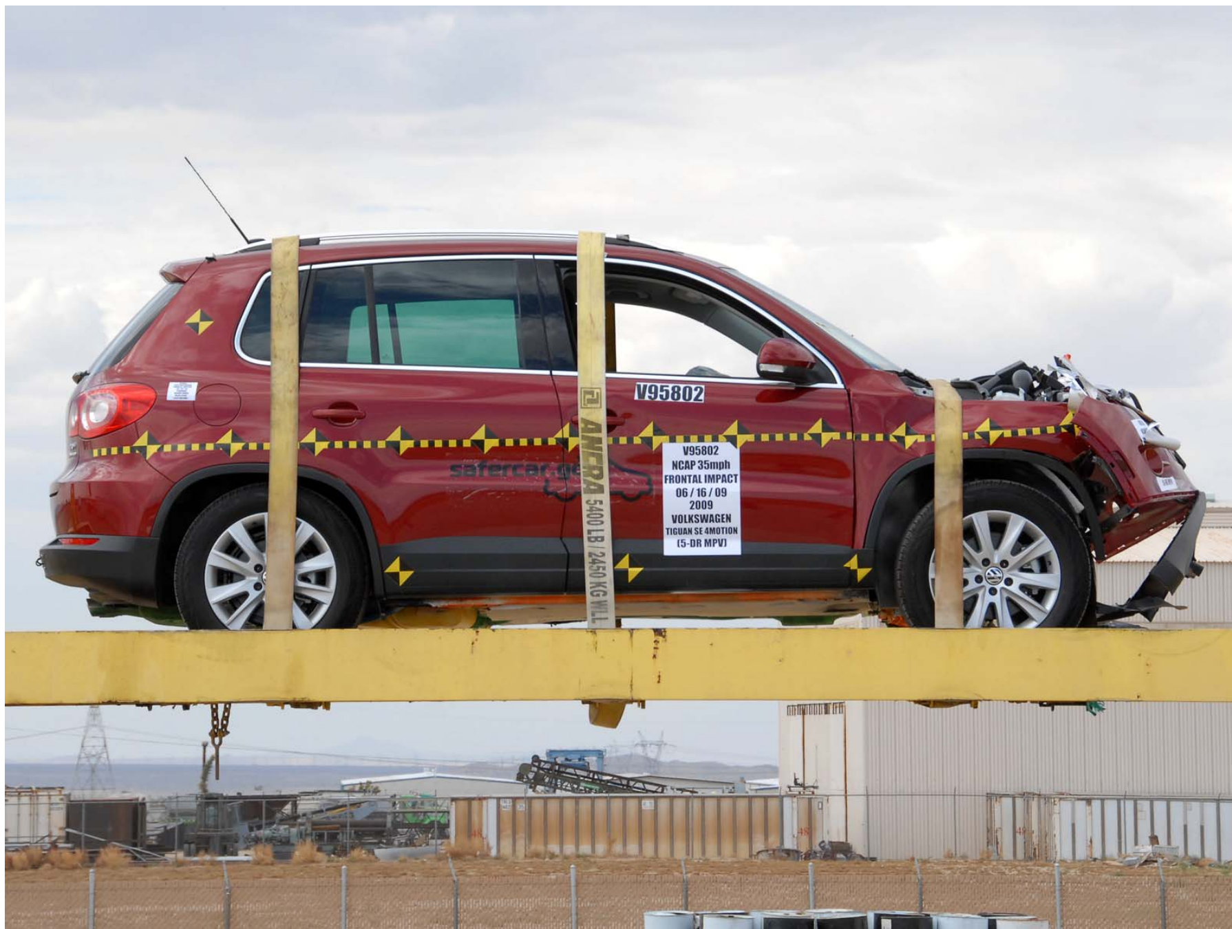
Figure A-62: Vehicle on Rollover Device (360°)
