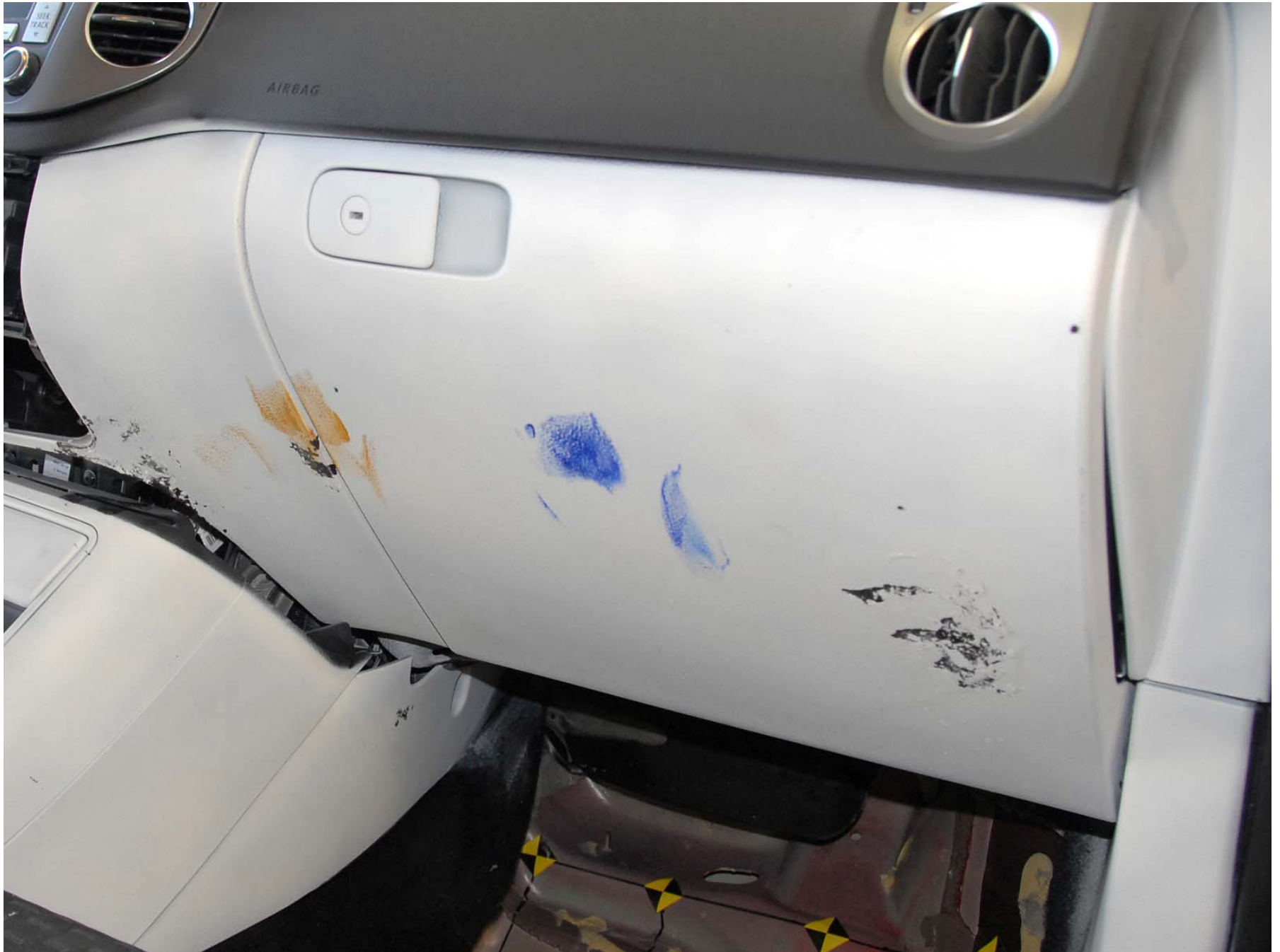
Figure A-53: Post-Test Passenger Side Glove Box
