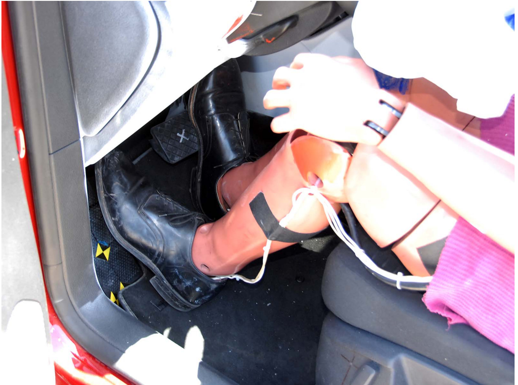
Figure A-37: Post-Test Driver Dummy Feet
