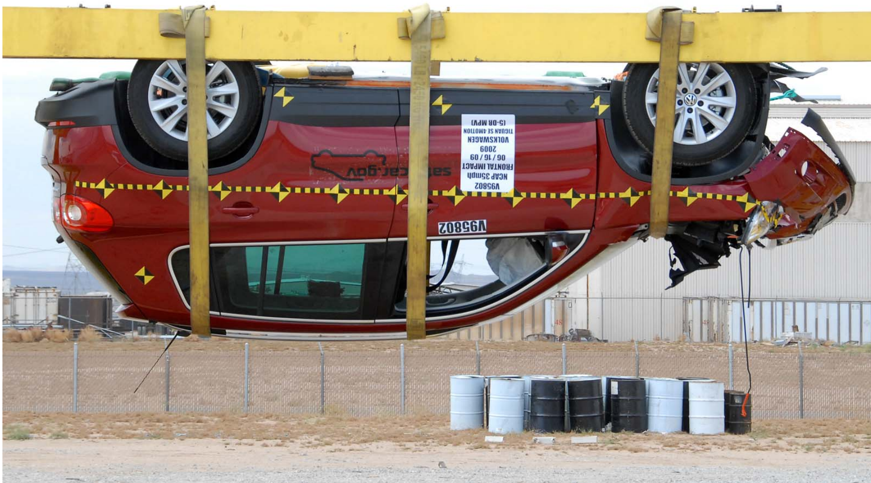
Figure A-60: Vehicle on Rollover Device (180°)
