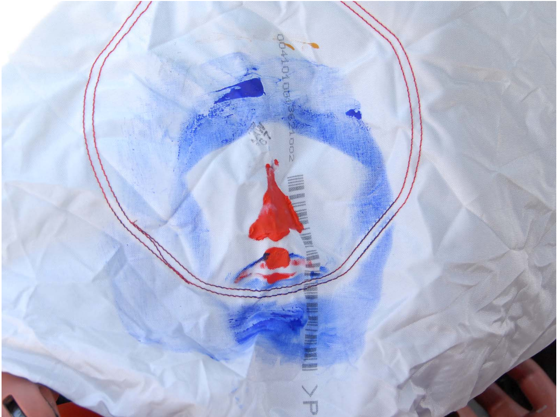
Figure A-43: Post-Test Driver Dummy Airbag Contact
