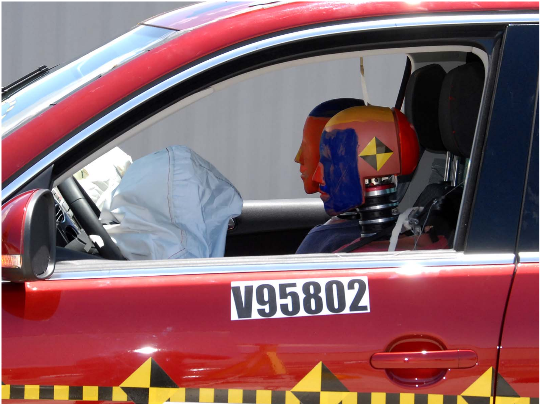
Figure A-33: Post-Test Driver Dummy (Through Window)
