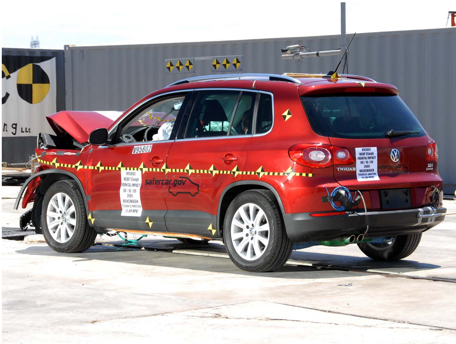
Figure A-15: Post-Test Left Rear \frac{3}{4} View
