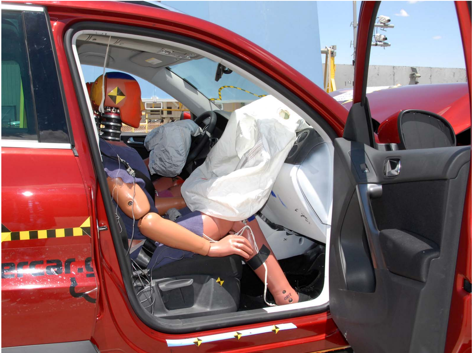
Figure A-49: Post-Test Passenger Dummy (Door Open)
