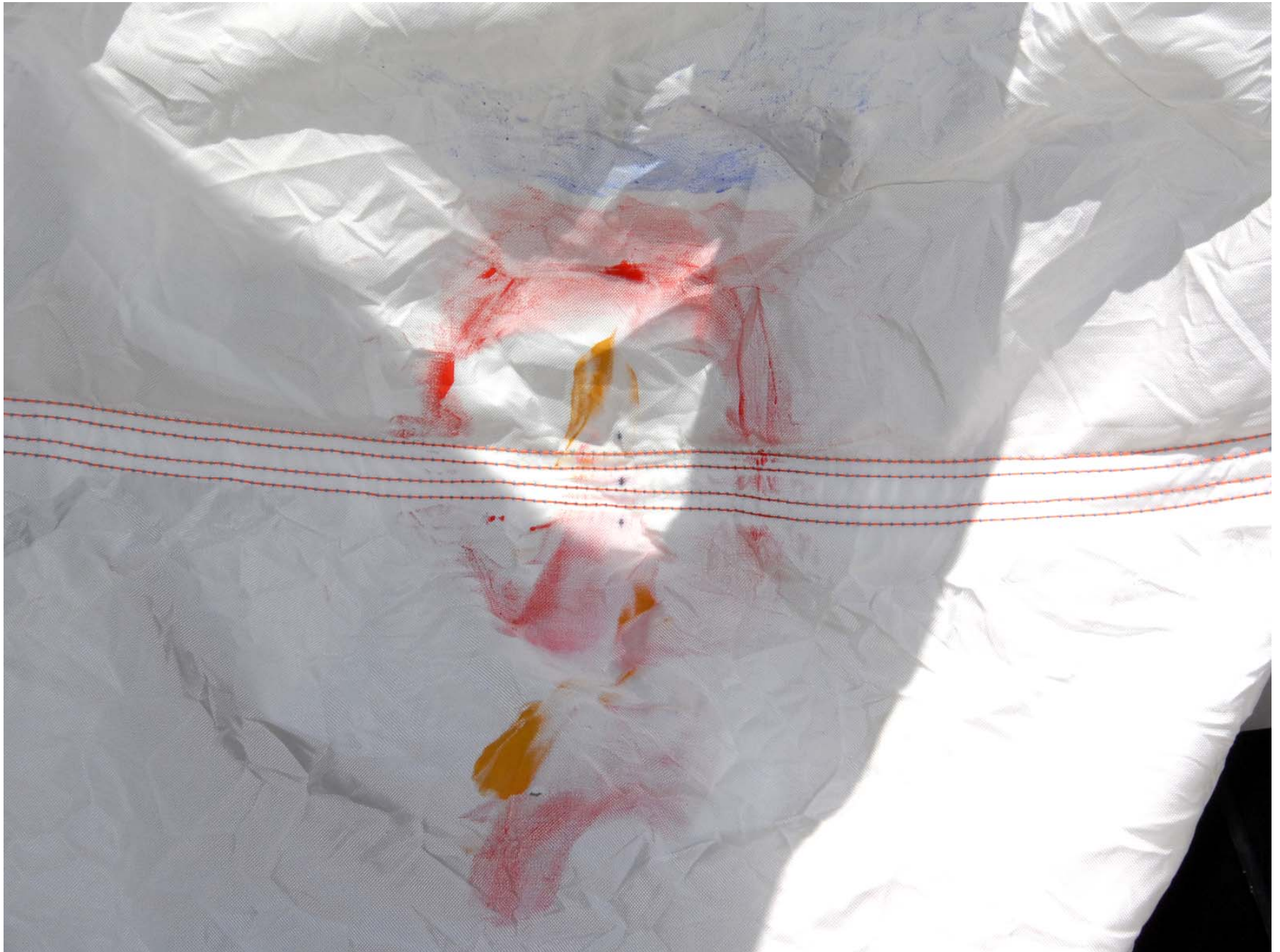
Figure A-57: Post-Test Passenger Dummy Airbag Contact
