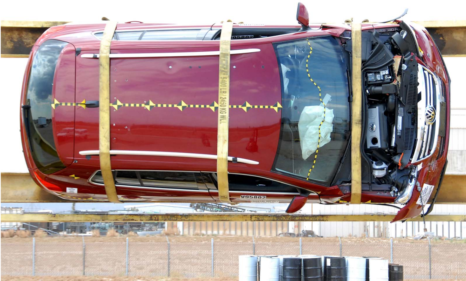
Figure A-59: Vehicle on Rollover Device (90°)
