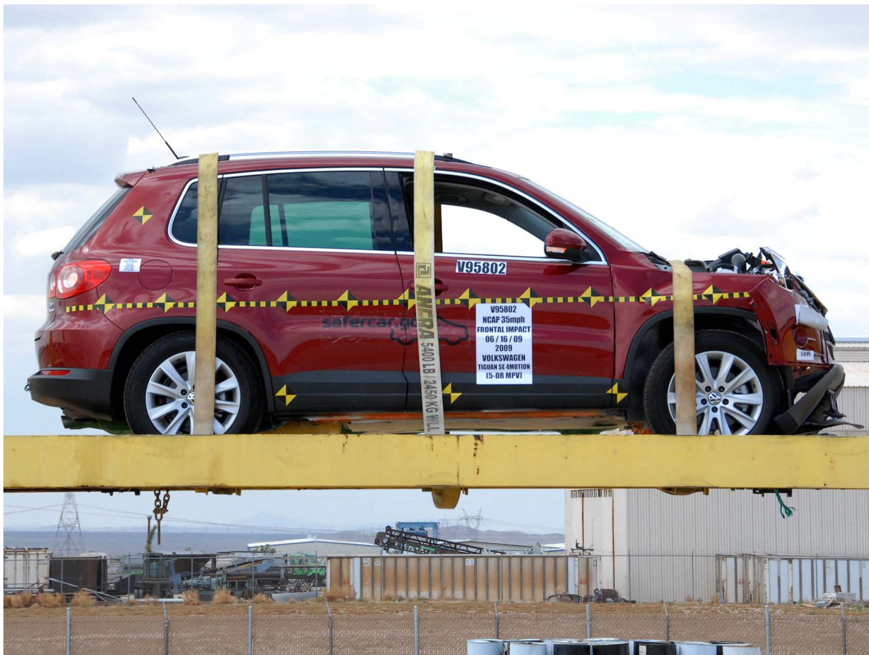
Figure A-58: Vehicle on Rollover Device (0°)
