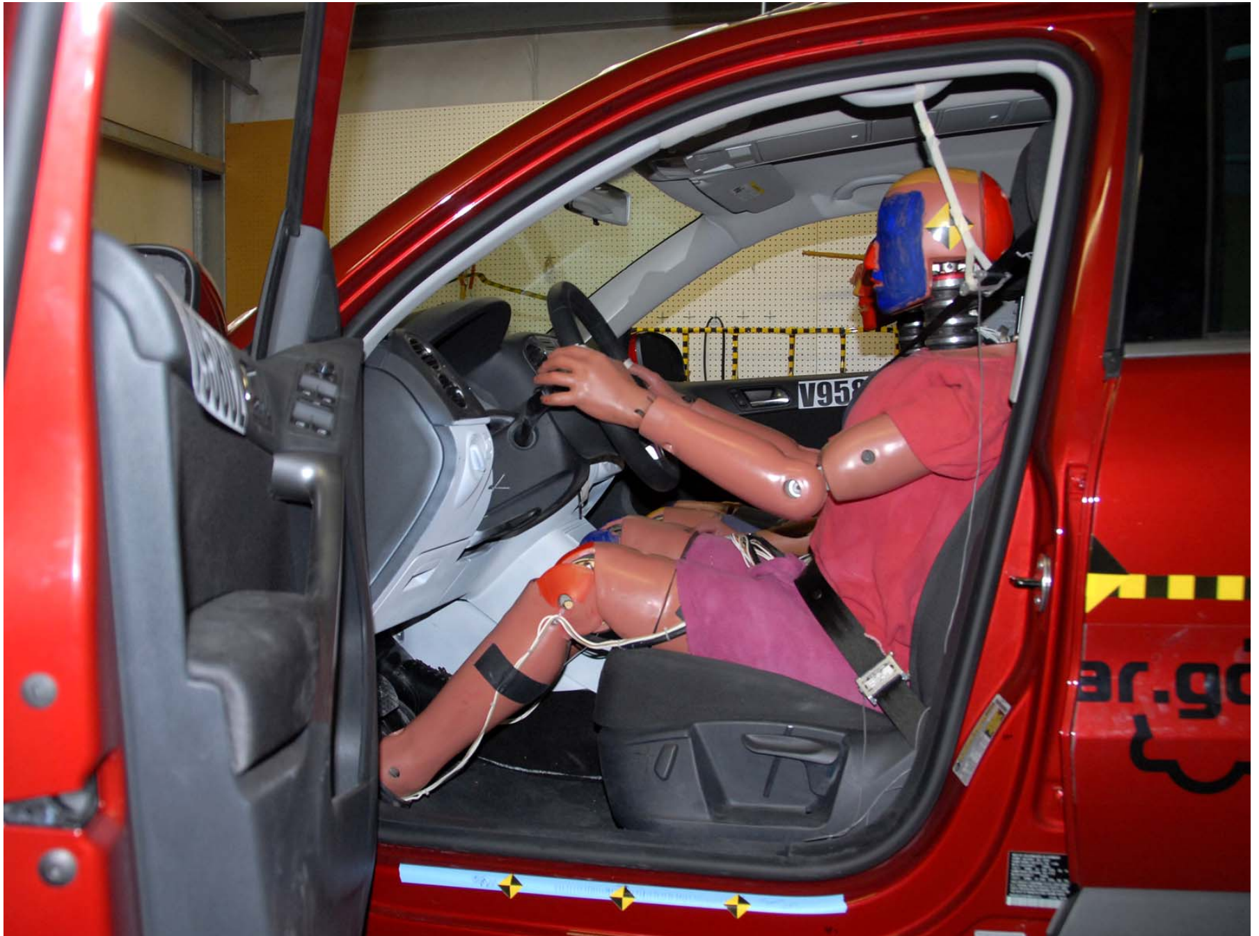
Figure A-34: Pre-Test Driver Dummy (Door Open)
