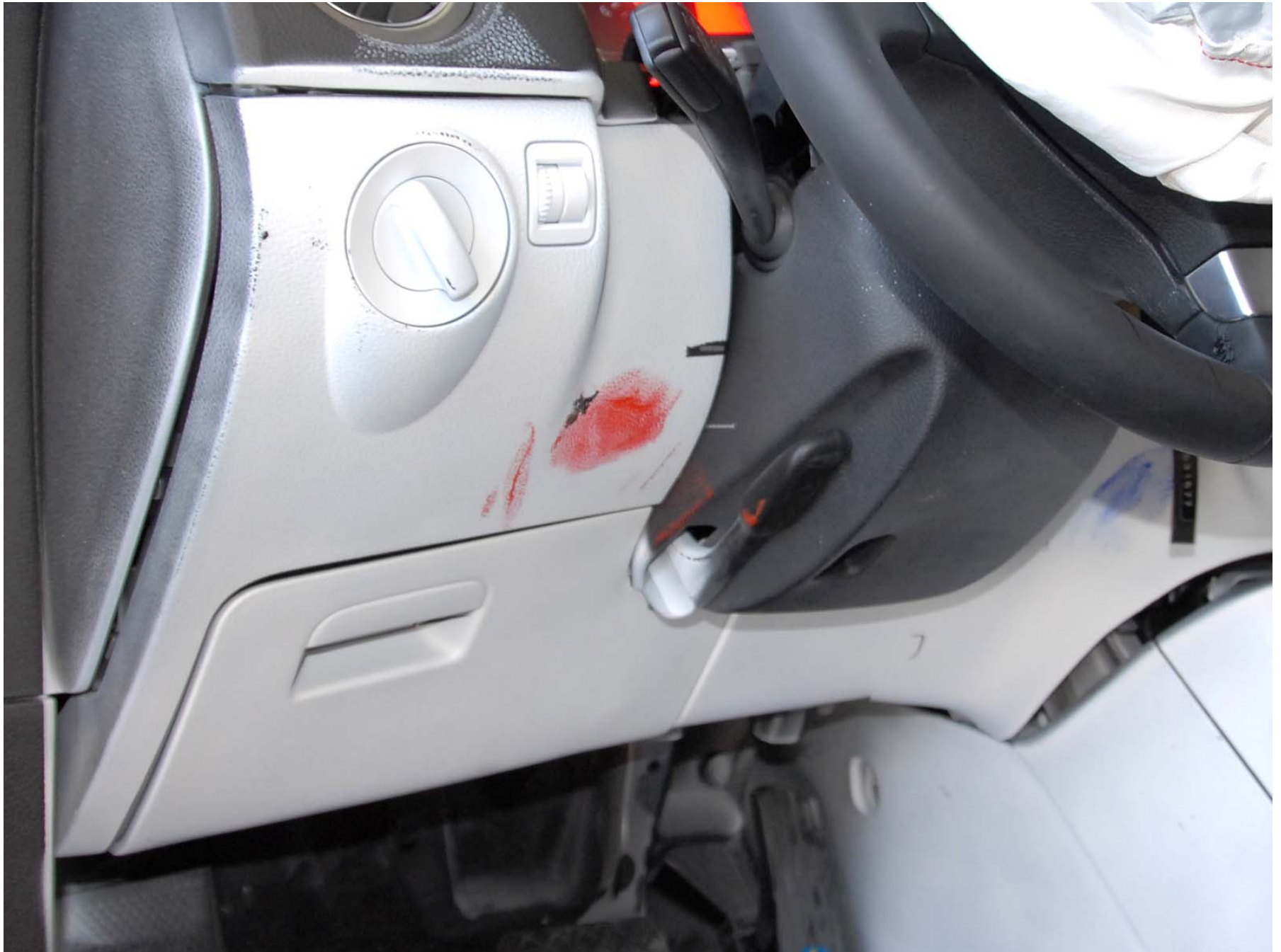
Figure A-39: Post-Test Driver Side Knee Bolster
