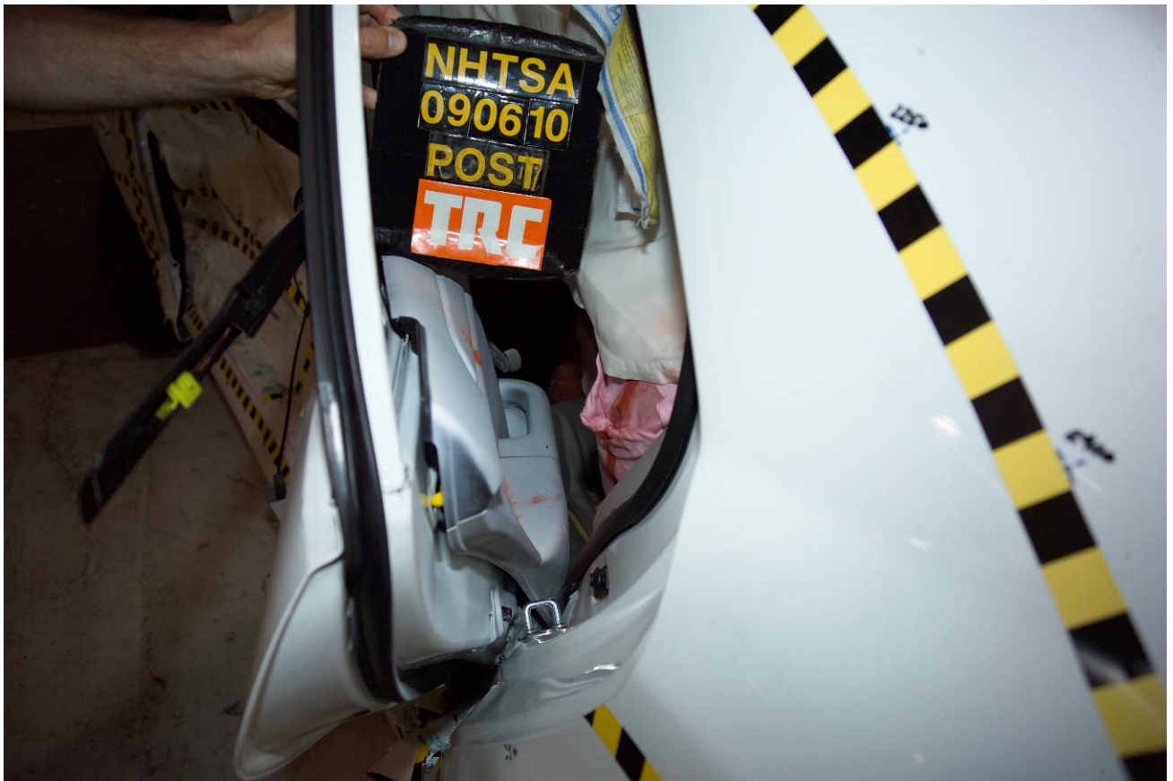
Figure A-62 Post-Test Left Rear Door Separation – View 1
