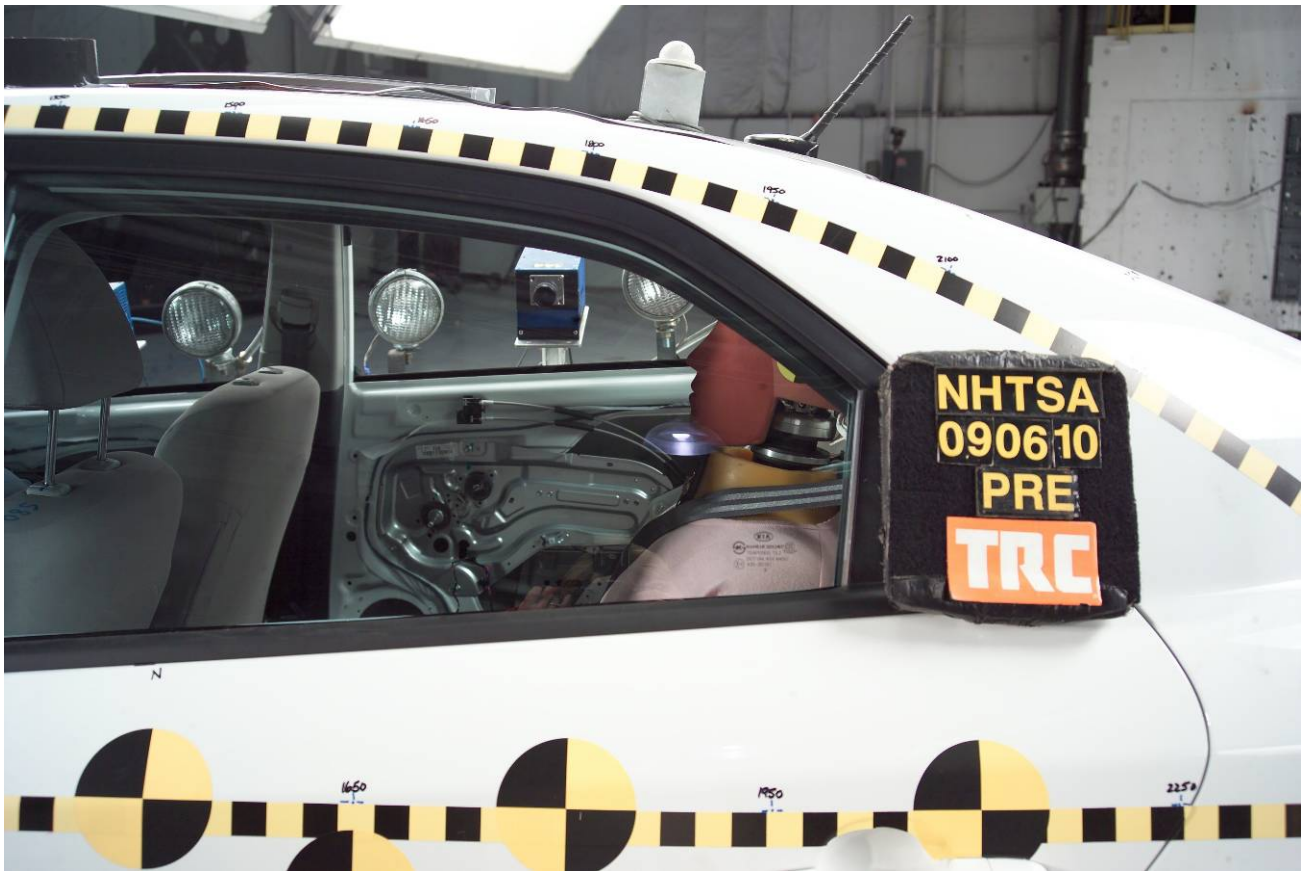
Figure A-46 Pre-Test Left View of Rear SID HIII
