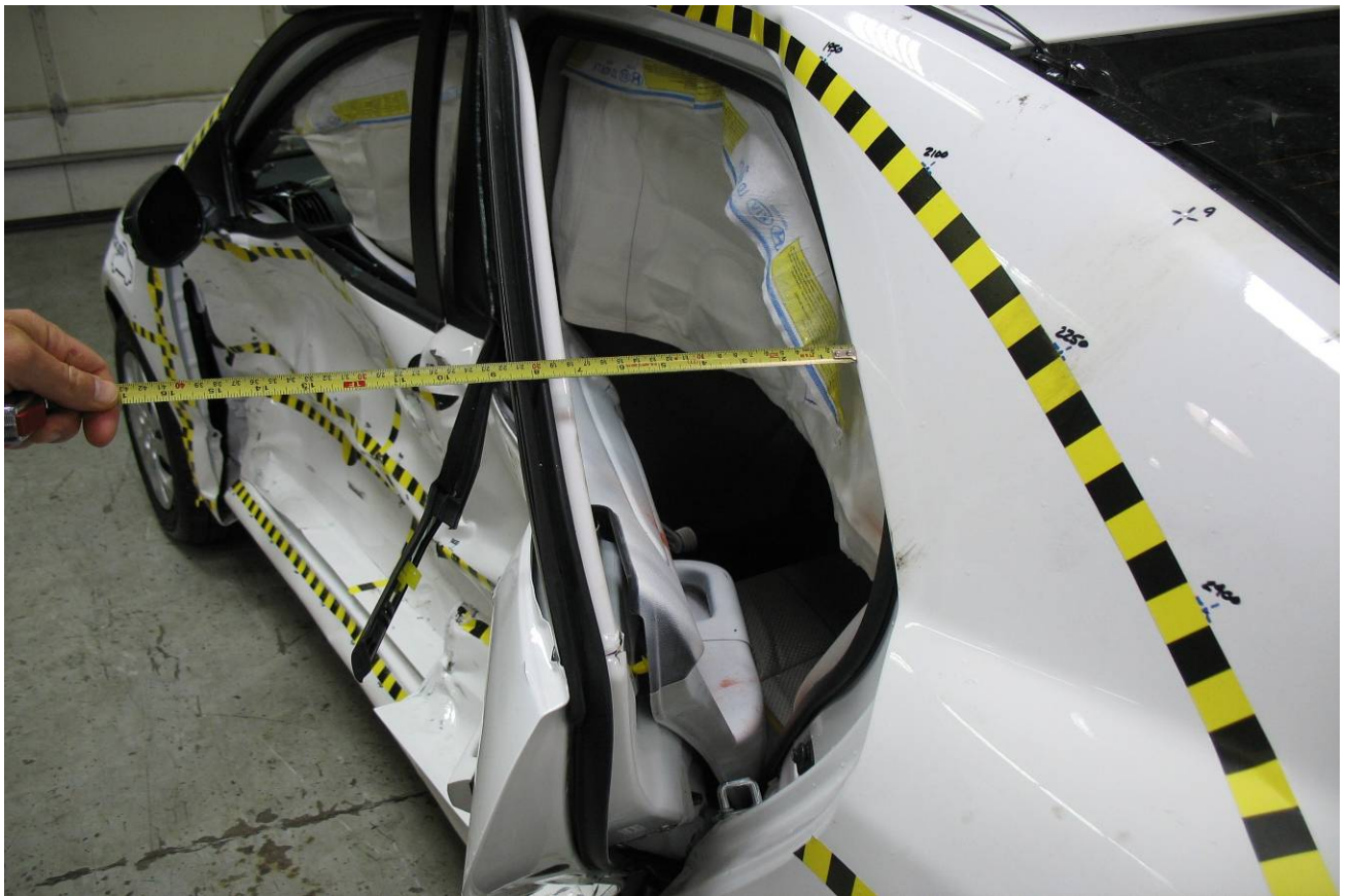
Figure A-64 Post-Test Left Rear Door Separation – View 3
