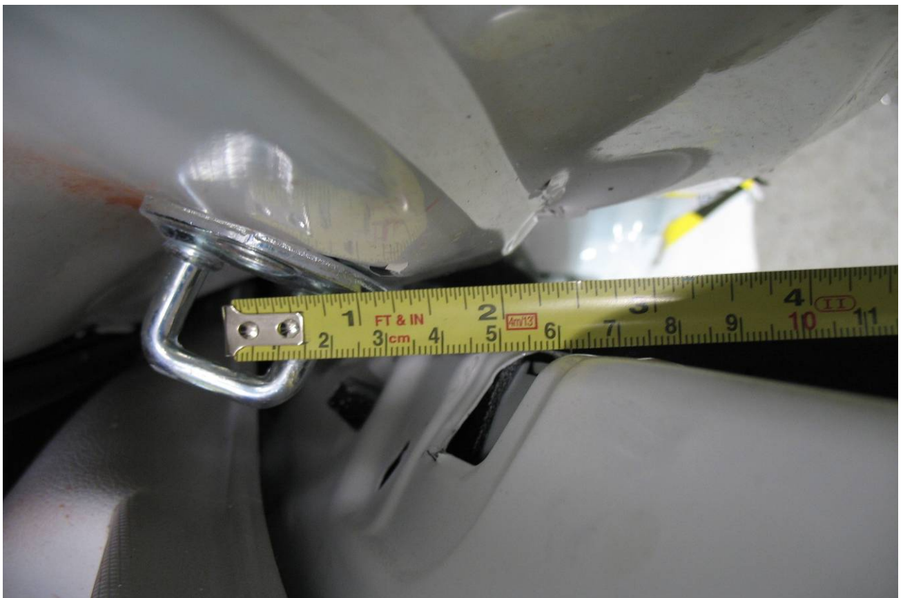
Figure A-65 Post-Test Left Rear Door Separation – View 4
