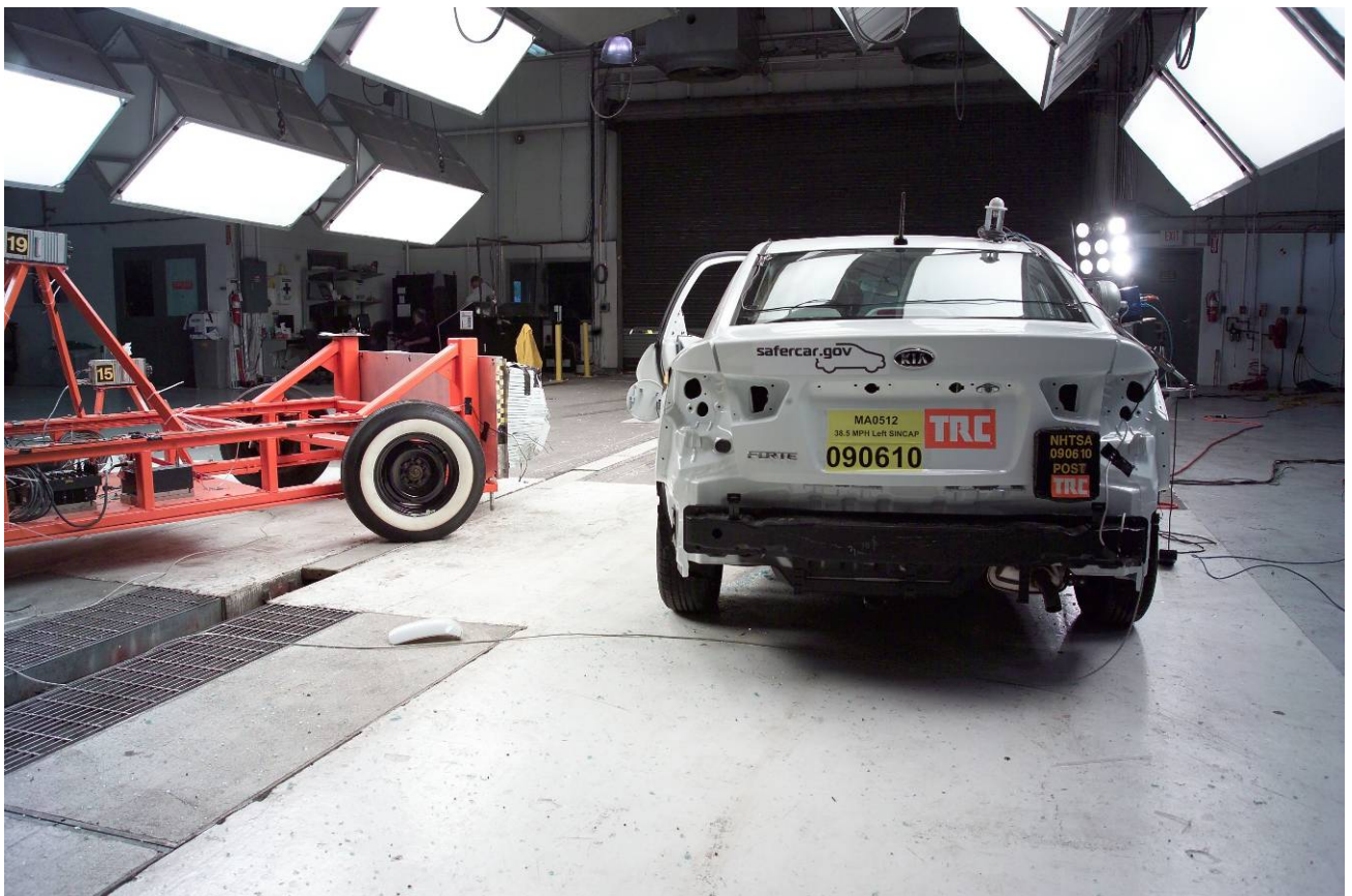
Figure A-71 Post-Test Right Side View of MDB With Impactor Face in Position
