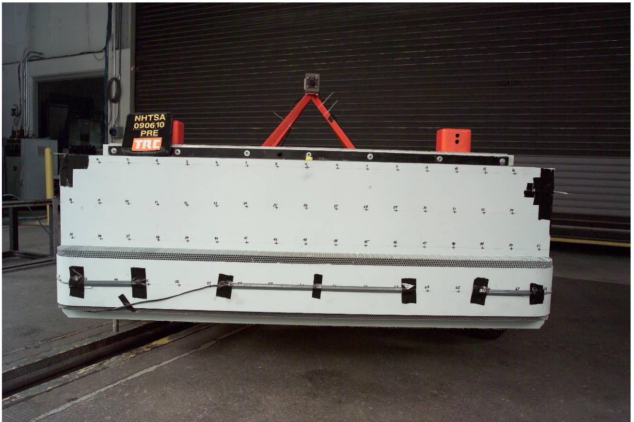
Figure A-35 Pre-Test View of MDB Showing Contact Switches in Place
