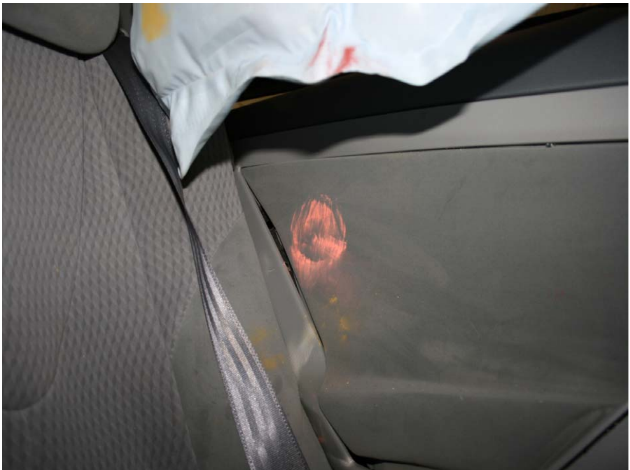
Post-Test Passenger Dummy Door Contact View
