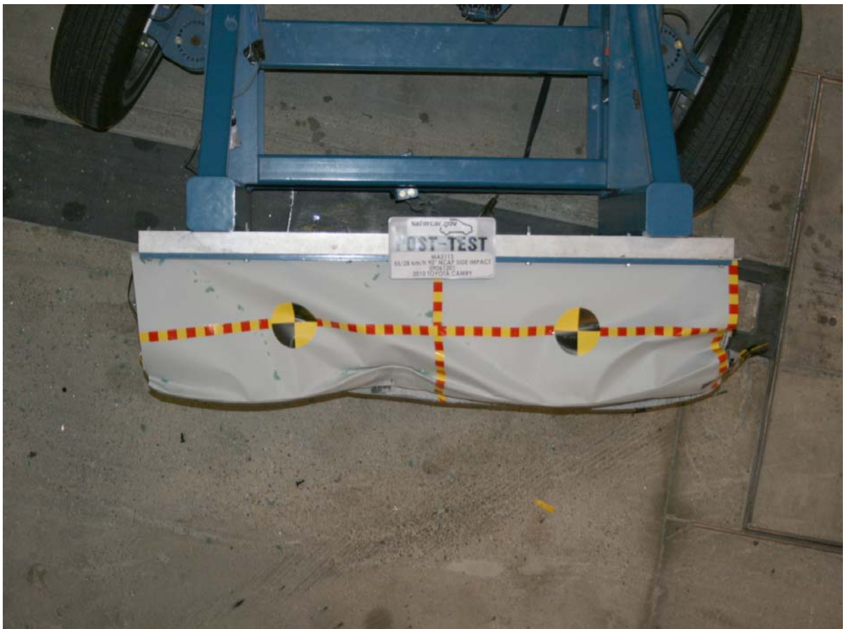
Post-Test Top View of MDB Impactor Face
