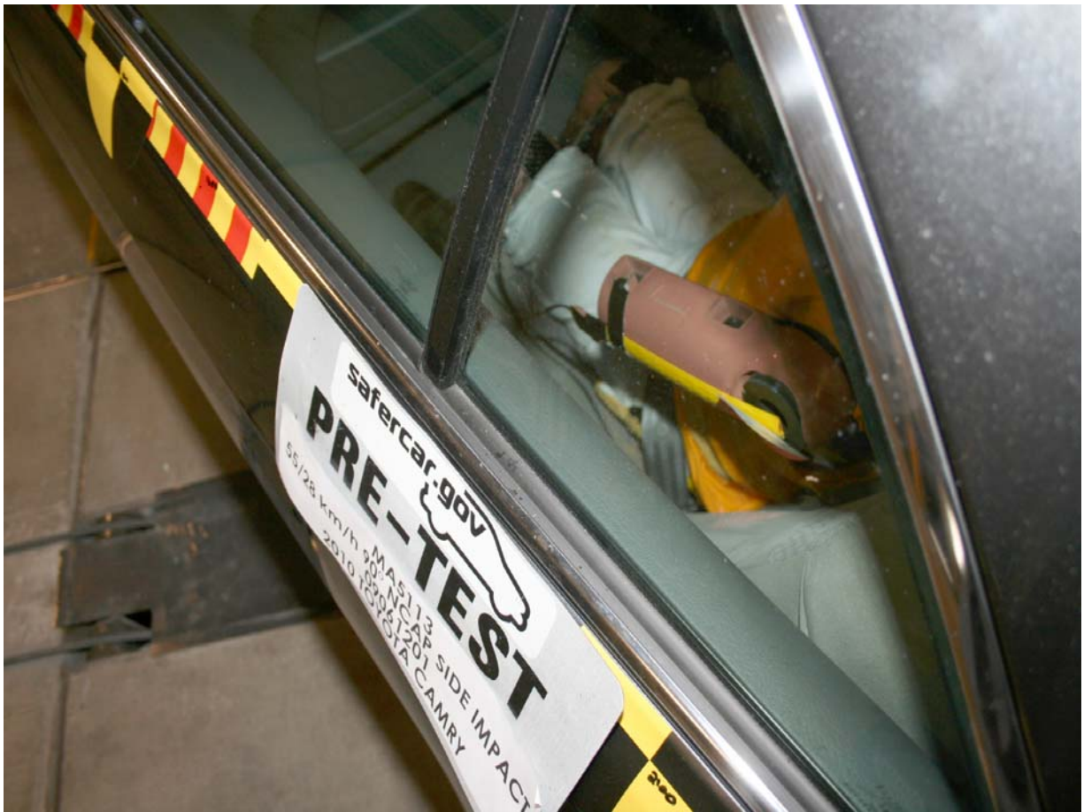
Pre-Test Passenger Dummy and Door Clearance View
