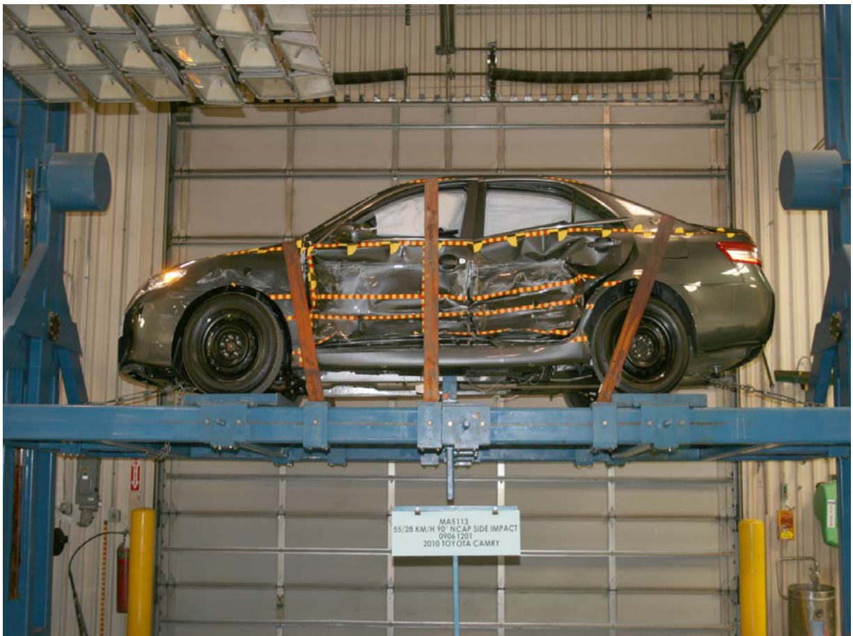
FMVSS No. 301/305 Rollover 0 Degrees
