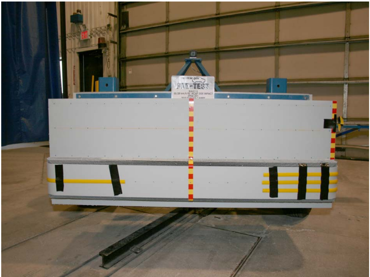
Pre-Test Front View of MDB Impactor Face
