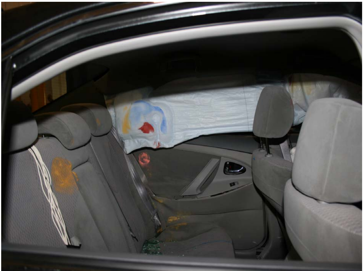
Post-Test Passenger Dummy Head Contact View 2
