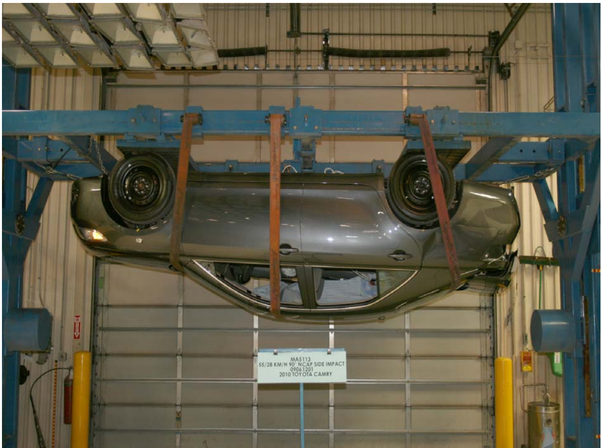
FMVSS No. 301/305 Rollover 180 Degrees
