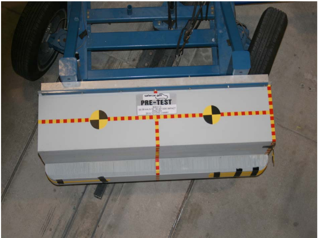
Pre-Test Top View of MDB Impactor Face
