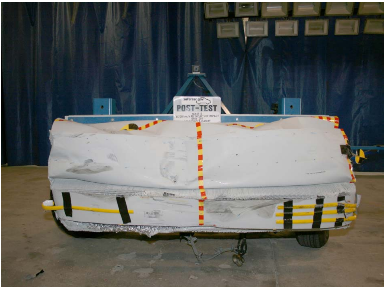
Post-Test Front View of MDB Impactor Face
