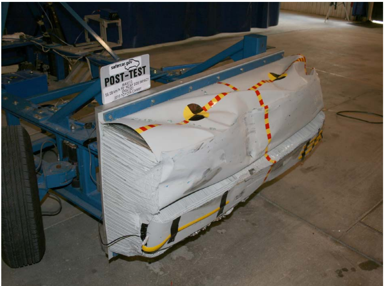
Post-Test Right Side View of MDB Impactor Face
