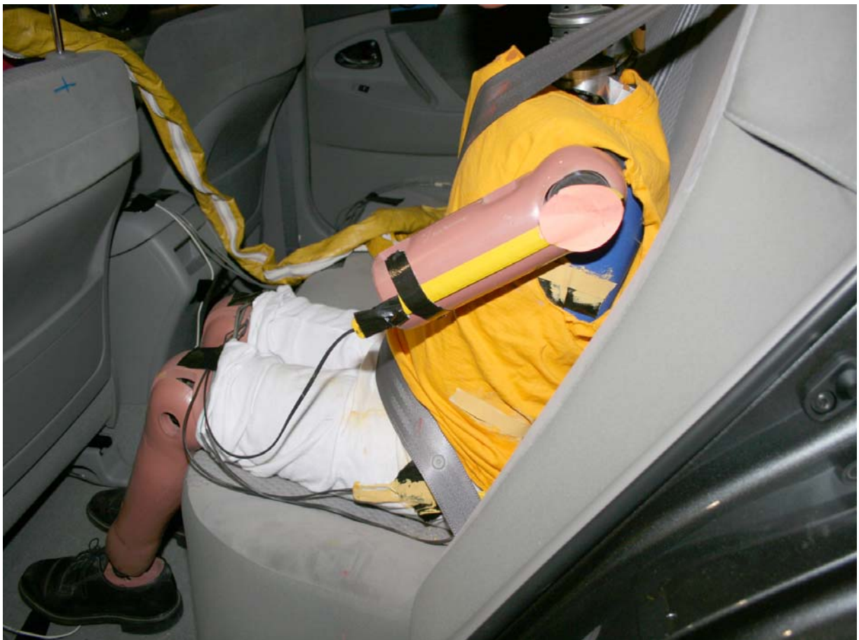
Pre-Test Close-Up Left Side View of Passenger Seat Back Showing Seat Back Positioning
