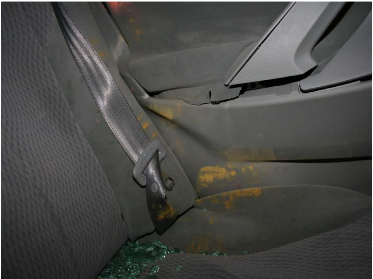
Post-Test Passenger Dummy Door Contact View 2
