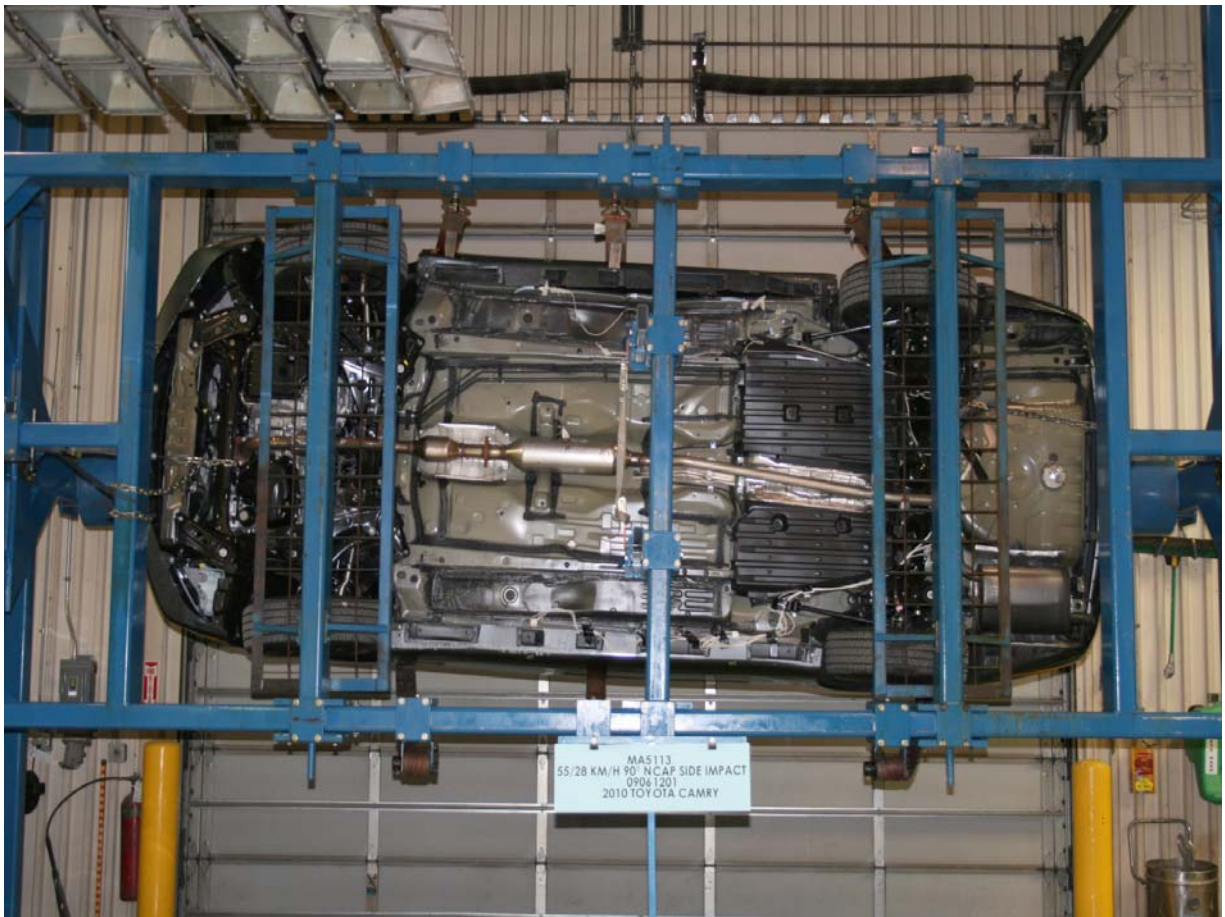
FMVSS No. 301/305 Rollover 270 Degrees
