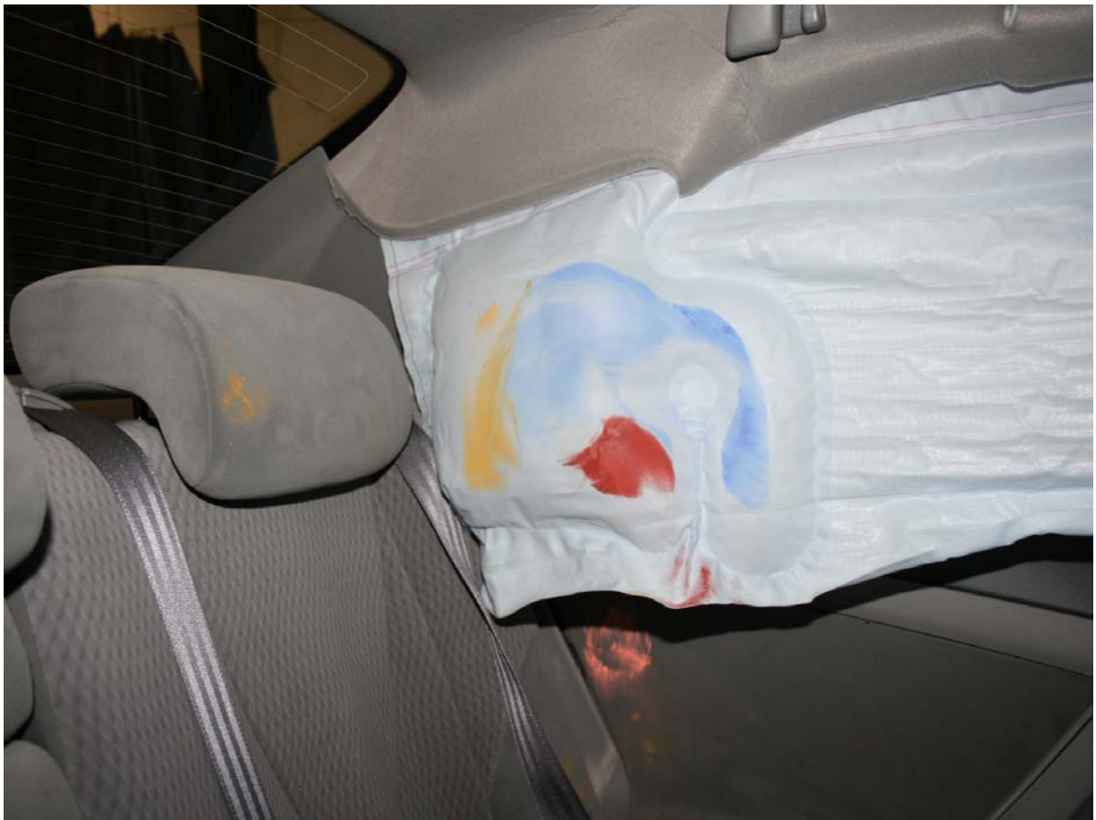
Post-Test Passenger Dummy Head Contact View
