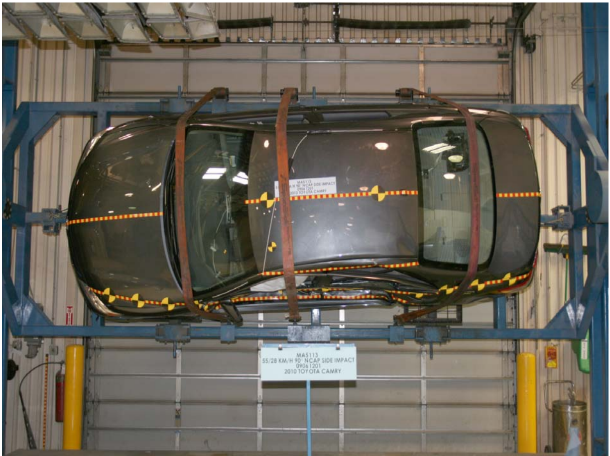
FMVSS No. 301/305 Rollover 90 Degrees
