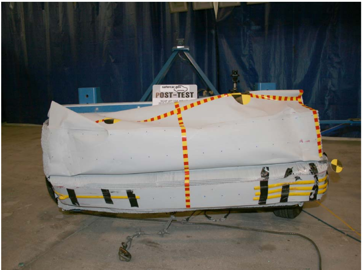
Post-Test Front View of Deformable Barrier
