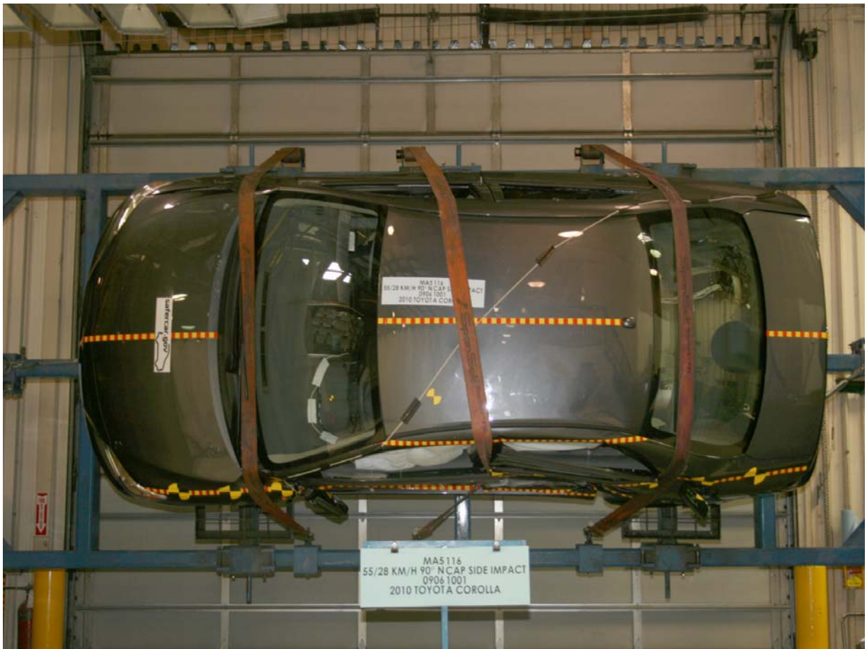
FMVSS No. 301/305 Rollover 90 Degrees
