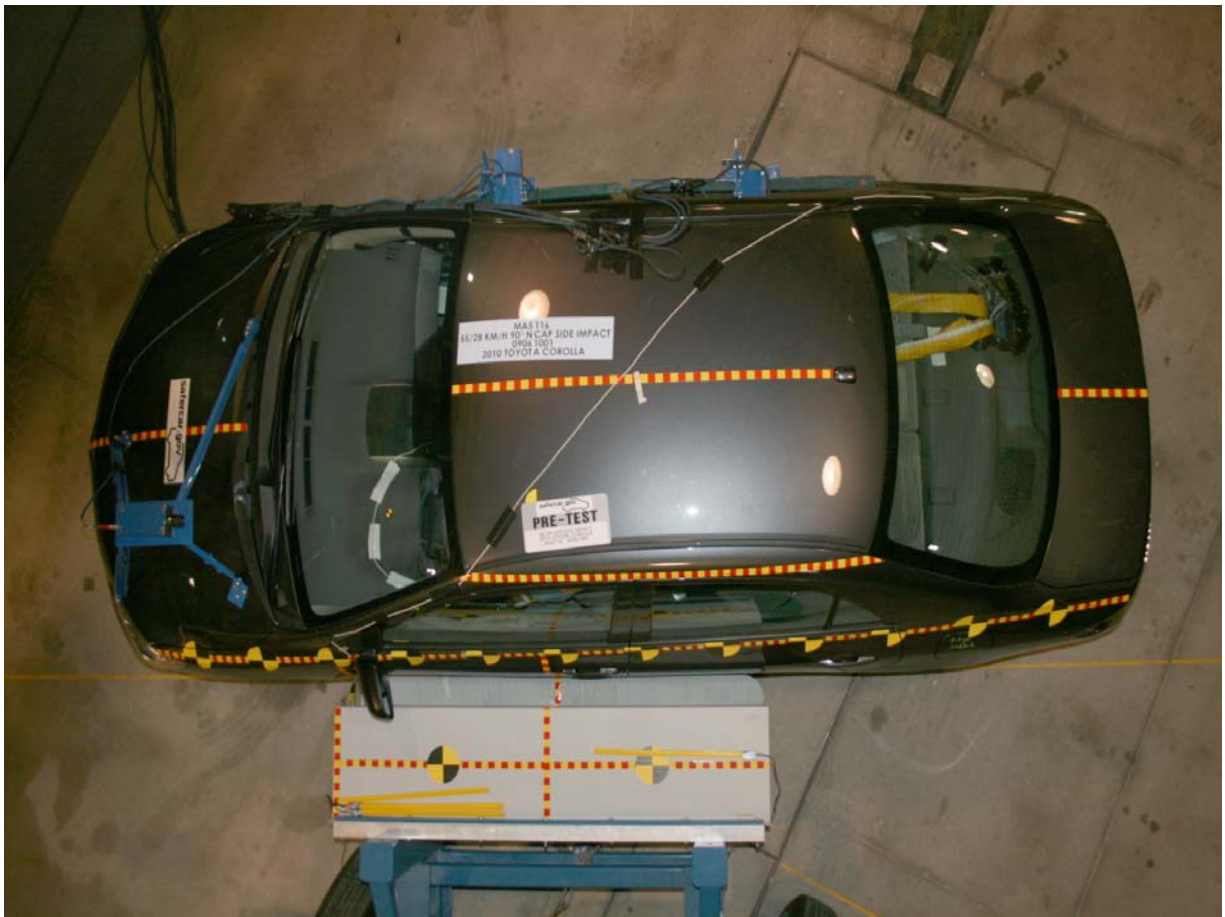
Pre-Test Overhead View of the Test Vehicle with MDB Positioned Against the Side of the Test Vehicle at the Ideal Impact Point
