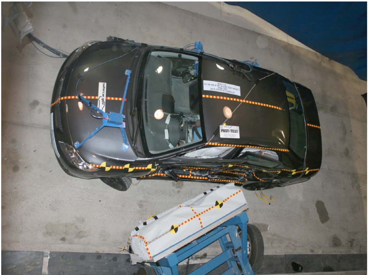
Post-Test Overhead View of the Test Vehicle and MDB
