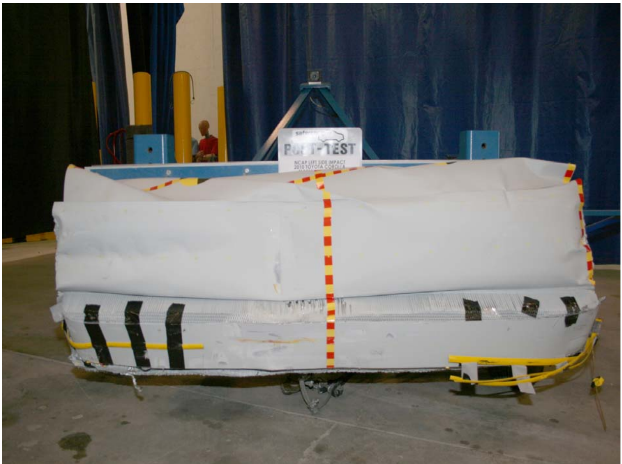
Post-Test Front View of MDB Impactor Face
