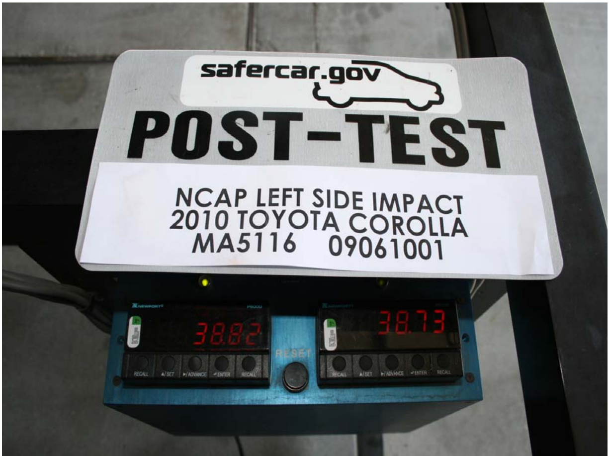
Post-Test Primary and Redundant Speed Trap Velocity Read-Out with Placard Showing NHTSA Number
