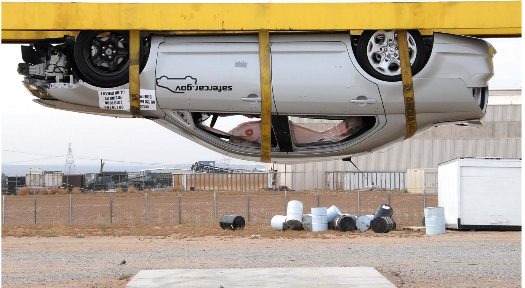
Figure A-66: FMVSS 301/305 Rollover 180°
