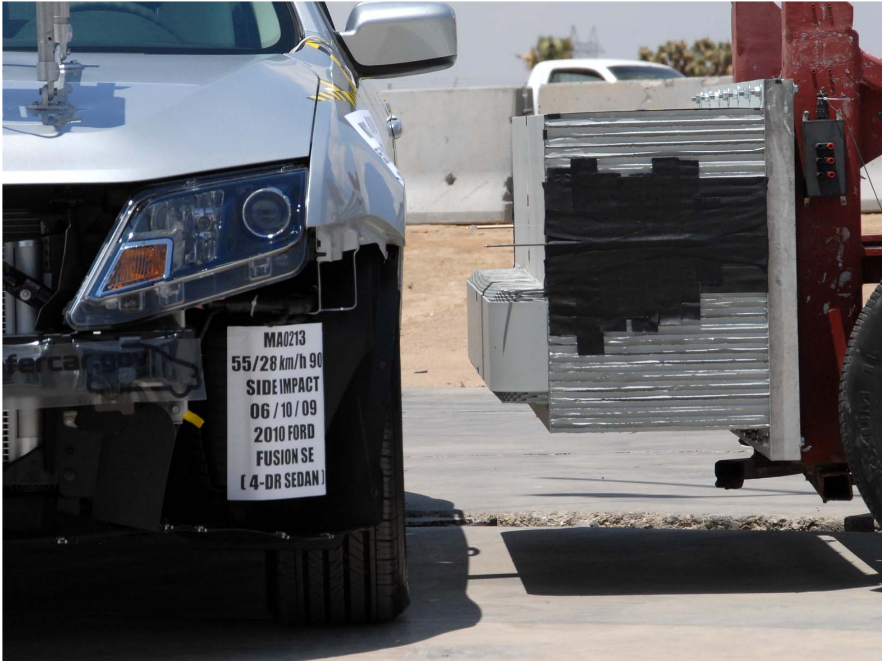
Figure A-17: Pre-test Left Side View of MDB Positioned Against the Side of the Test Vehicle at the Ideal Impact Point
