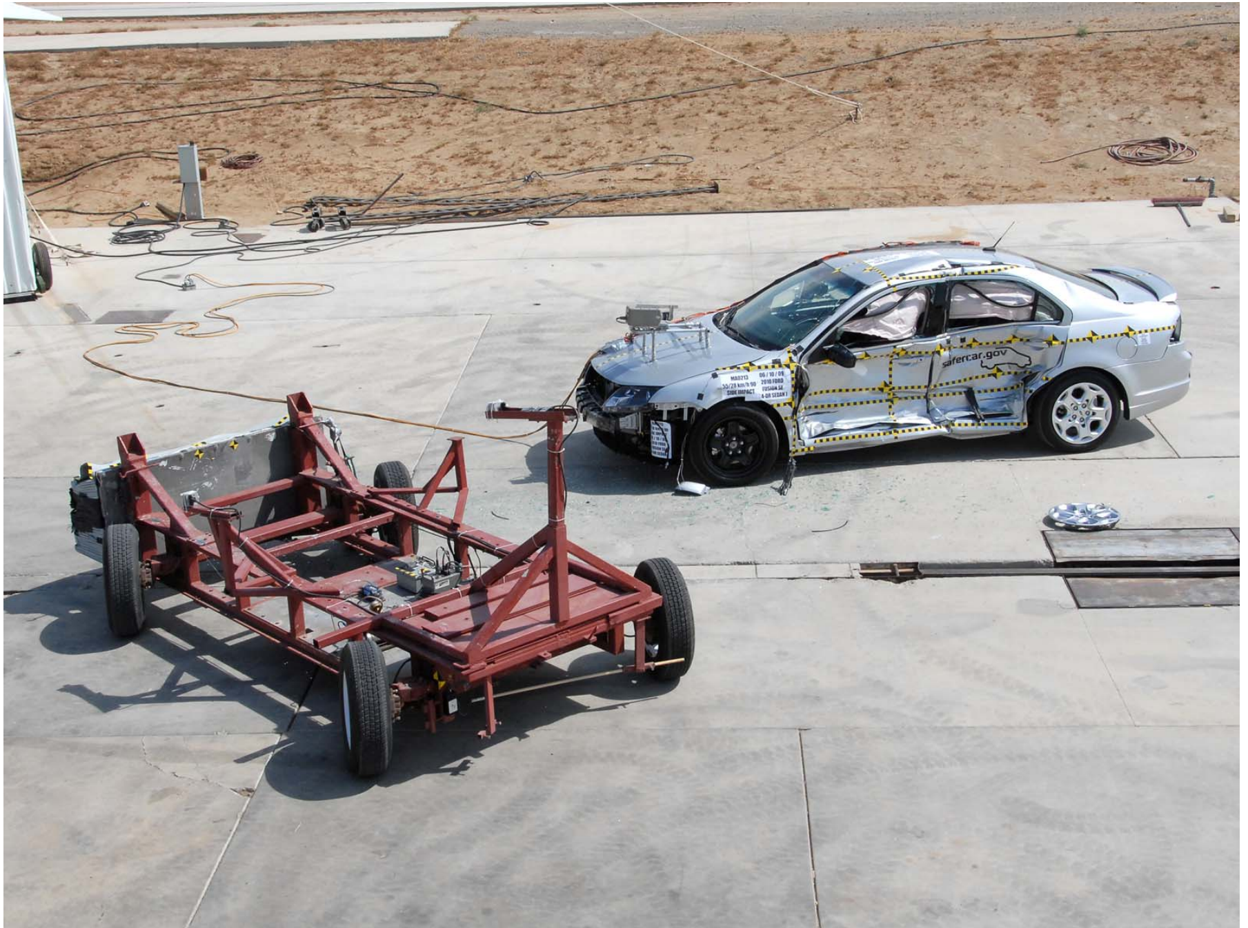
Figure A-16: Post-test Overhead View of the Test Vehicle and MDB
