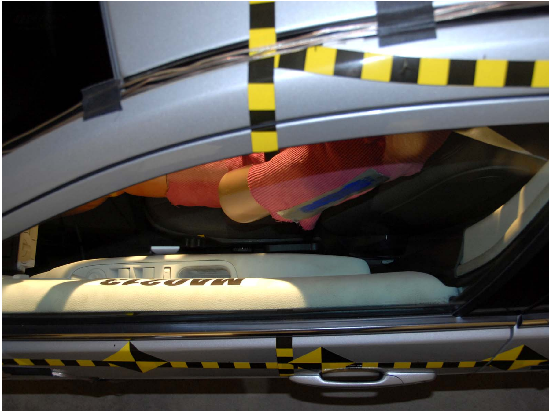
Figure A-32: Pre-test Driver Dummy and Door Clearance View
