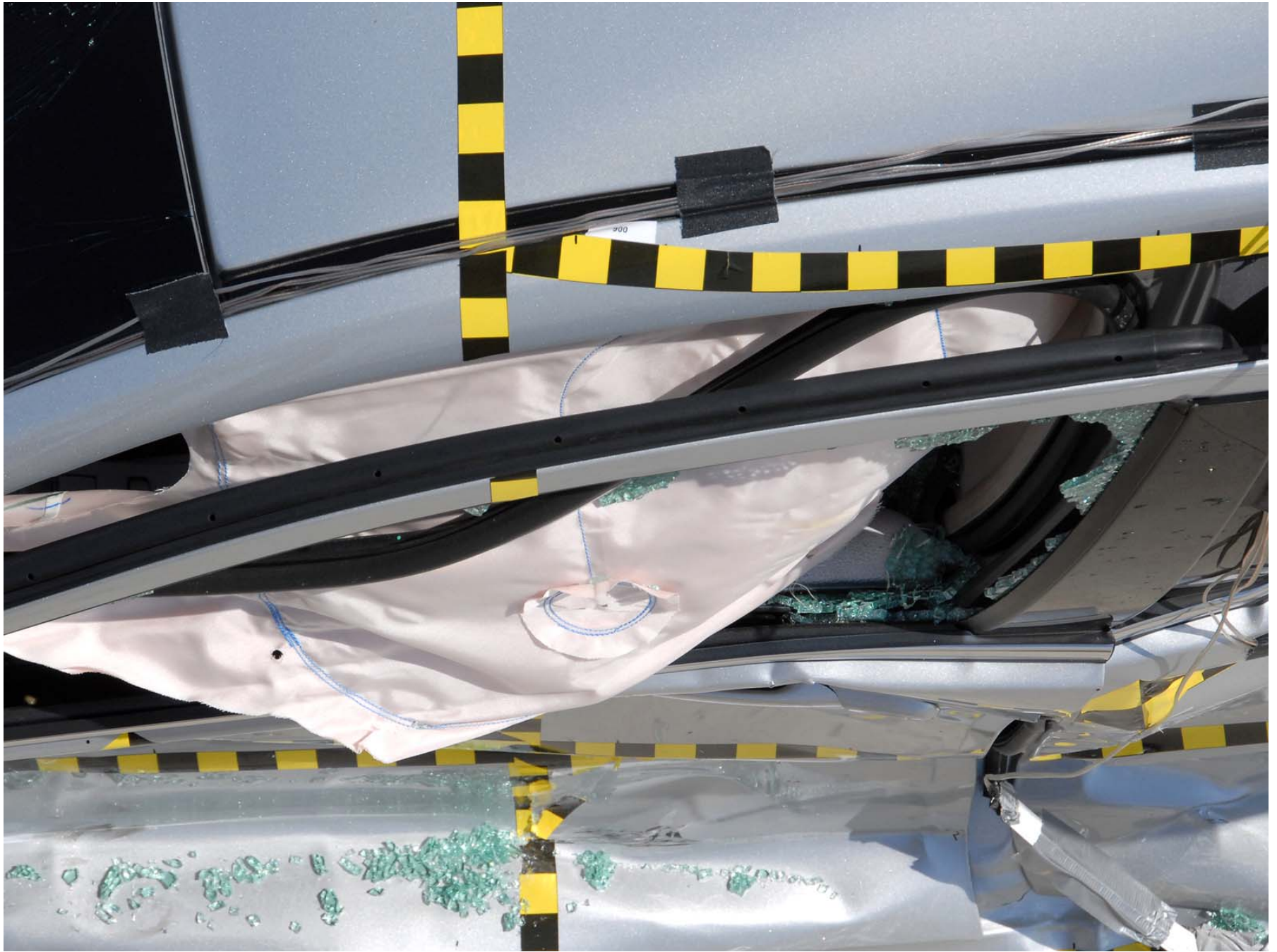
Figure A-33: Post-test Driver Dummy and Door Clearance View
