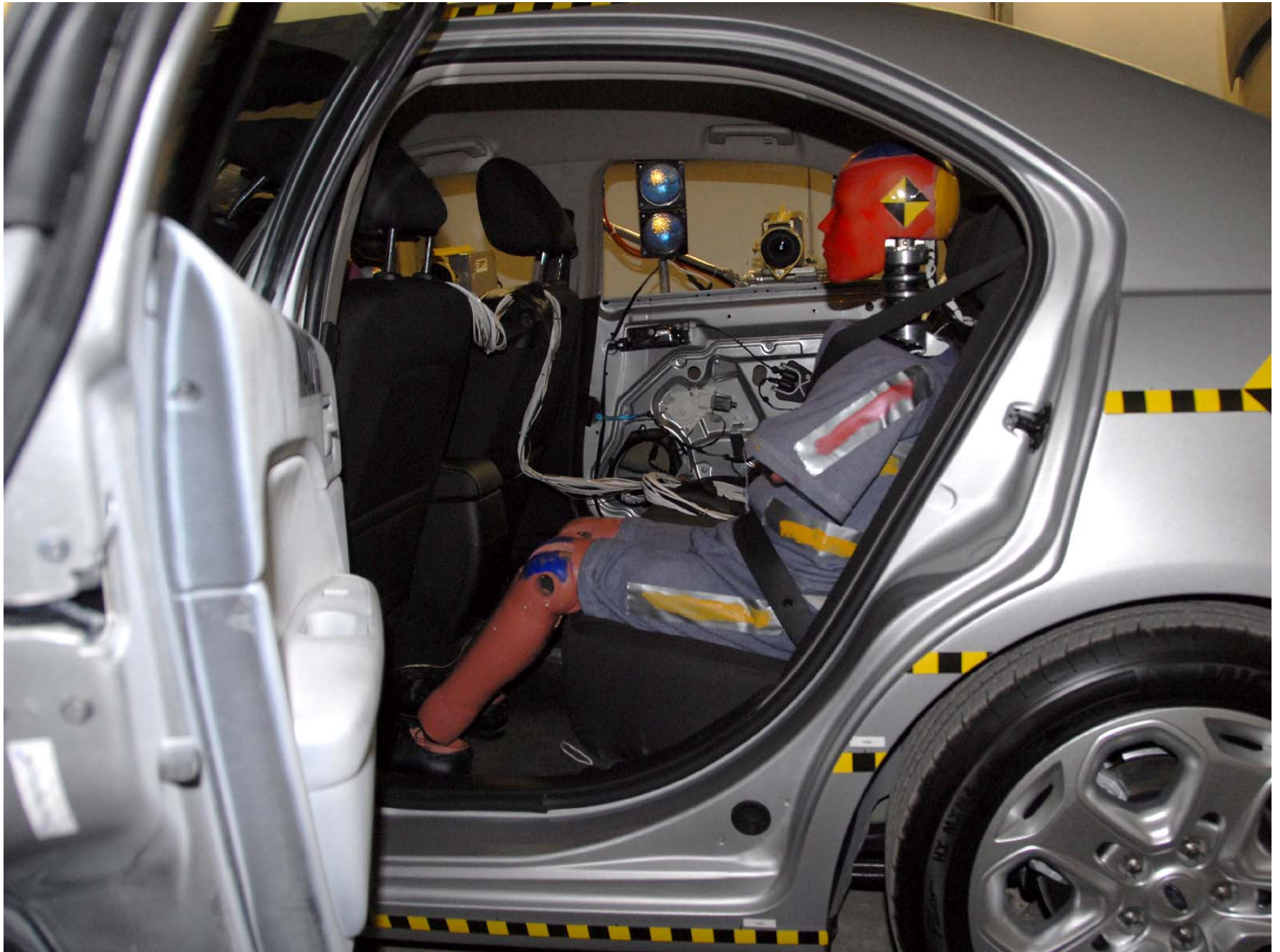
Figure A-40: Pre-test Left Side View of Passenger Dummy Showing Belt, Chalking, and Contact Switches (Door Open)
