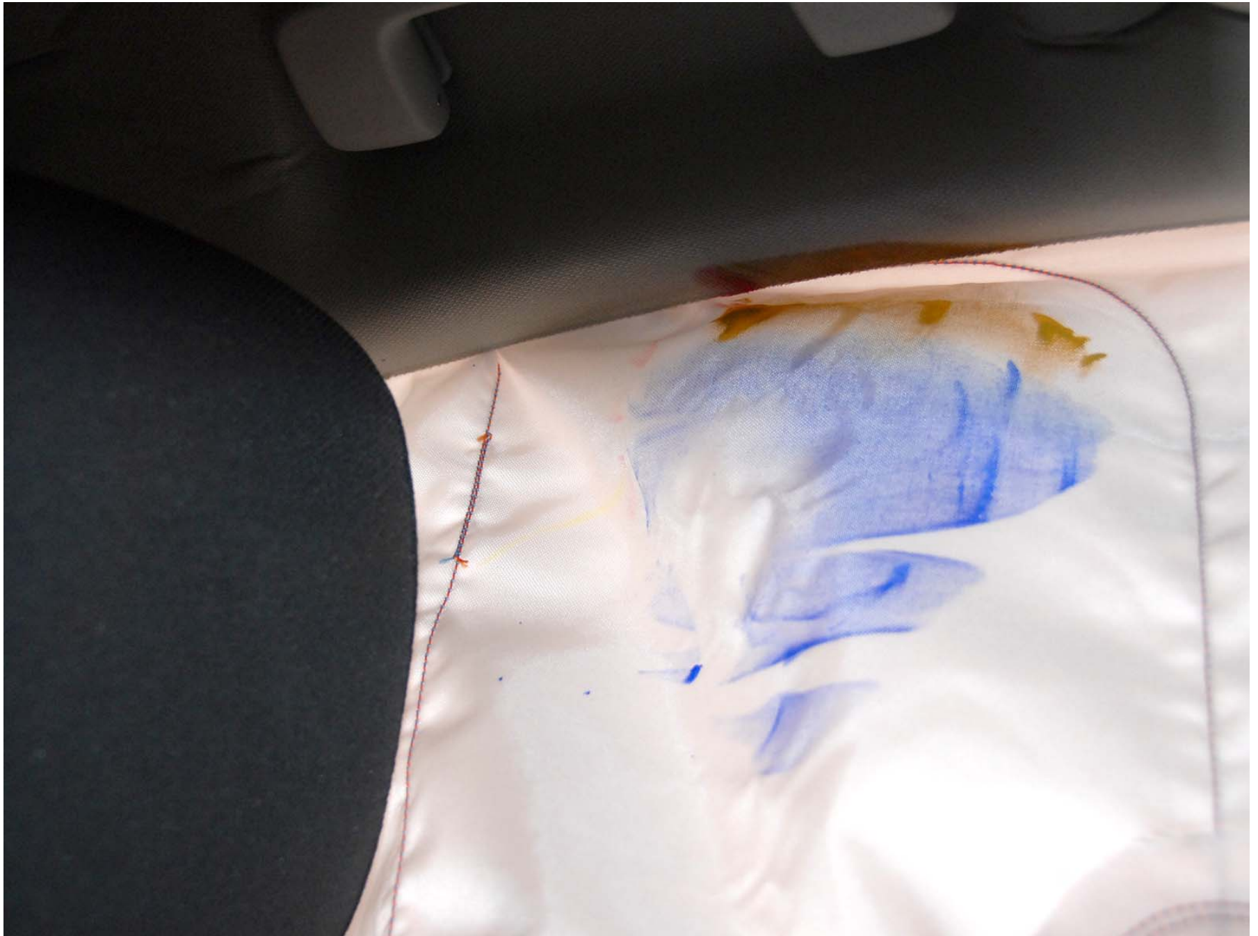
Figure A-38: Post-test Driver Dummy Head Contact View
