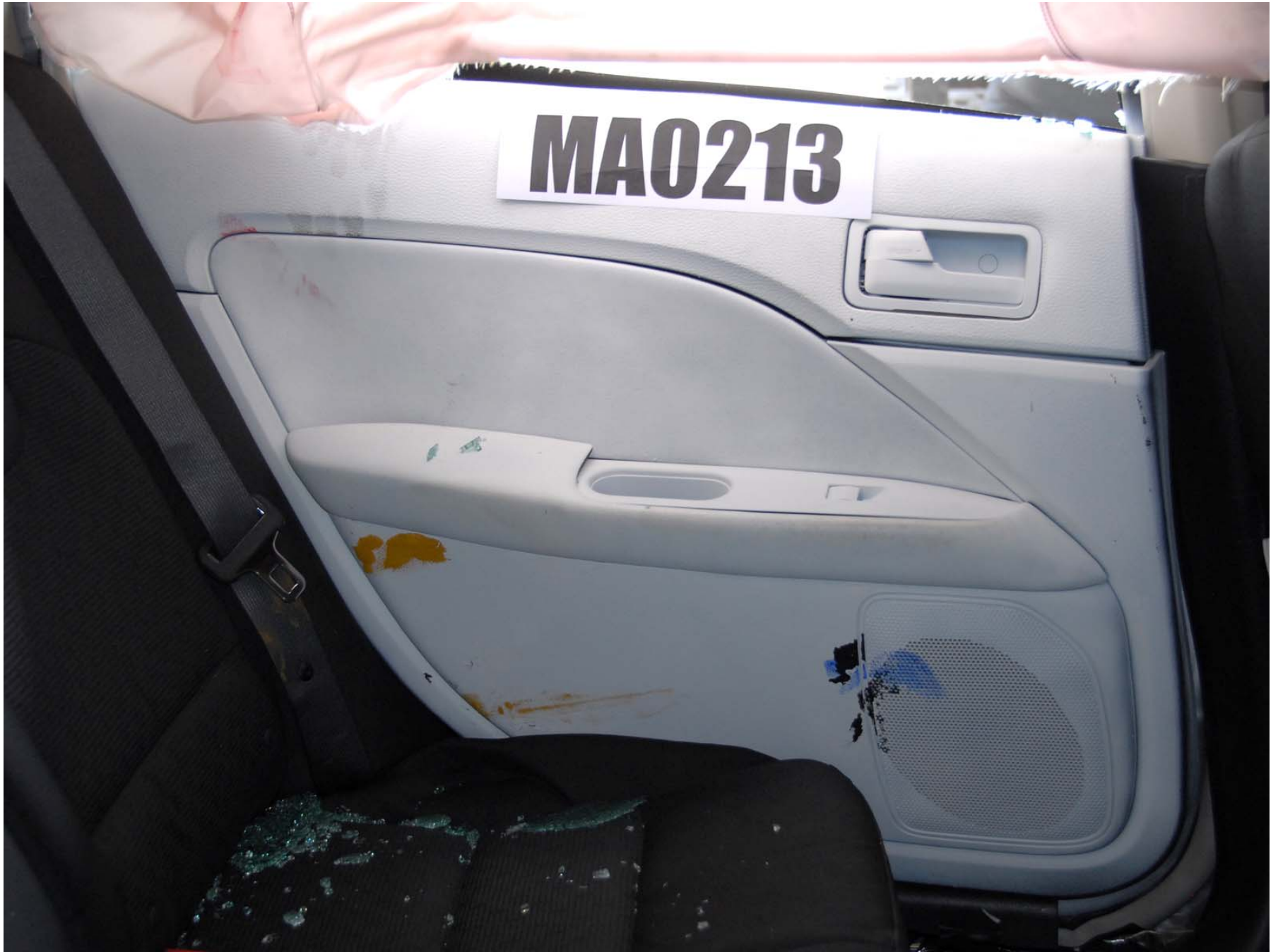
Figure A-52: Post-test Passenger Dummy Door Contact View
