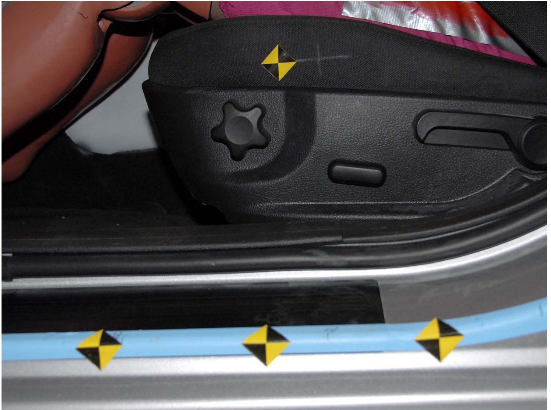
Figure A-30: Pre-test Close-Up Left Side View of Driver Seat Track Showing Seat Positioning
