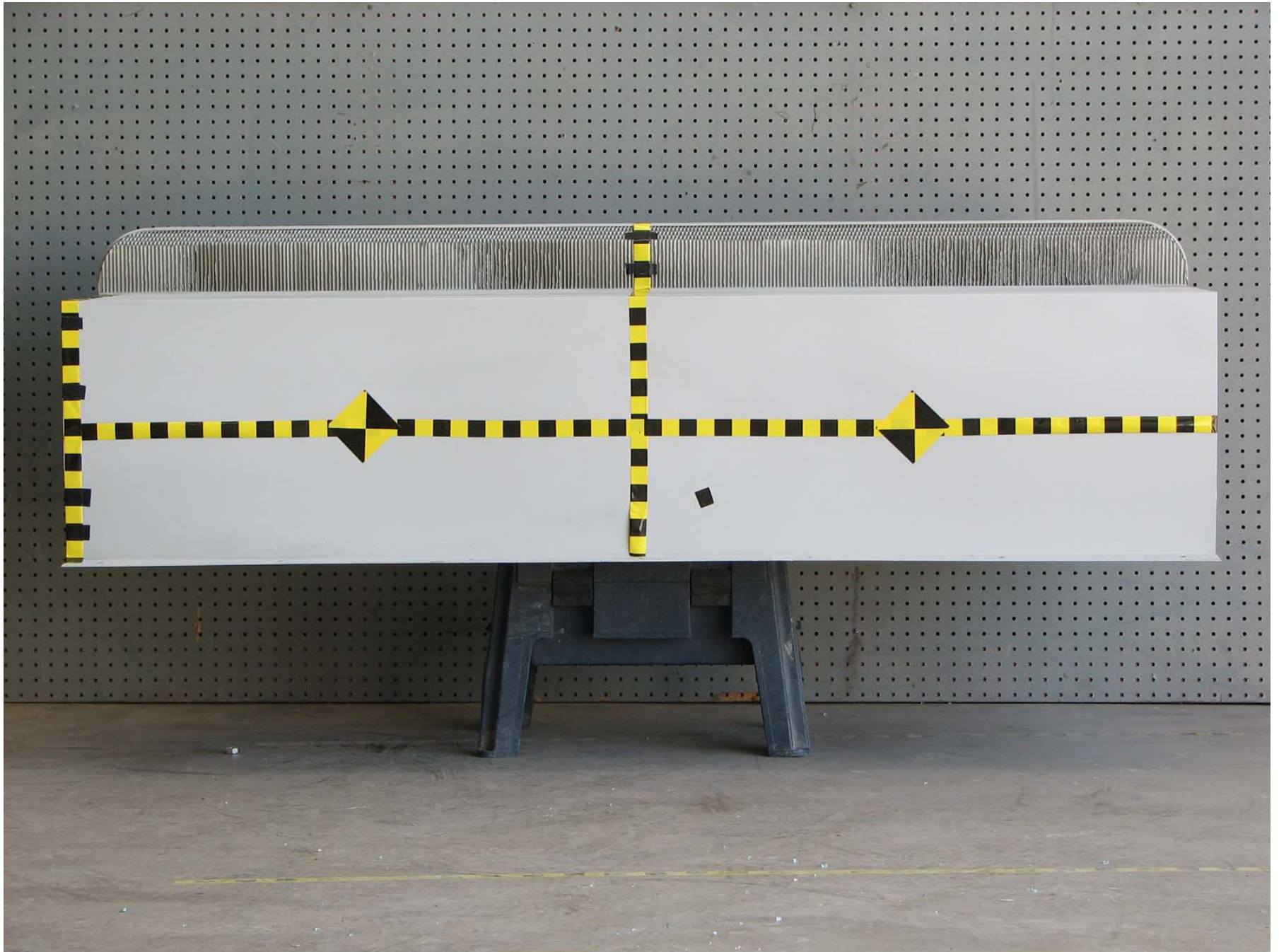
Figure A-57: Pre-test Top View of MDB Impactor Face
