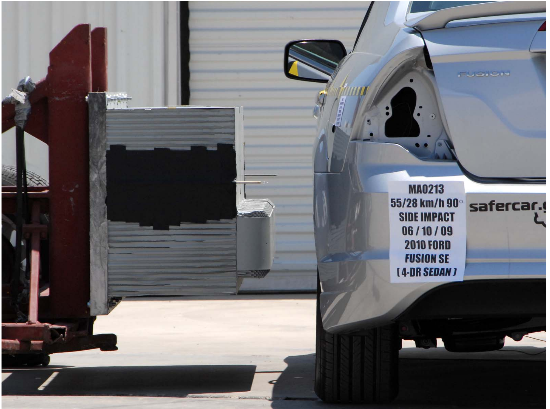
Figure A-18: Pre-test Right Side View of MDB Positioned Against the Side of the Test Vehicle at the Ideal Impact Point
