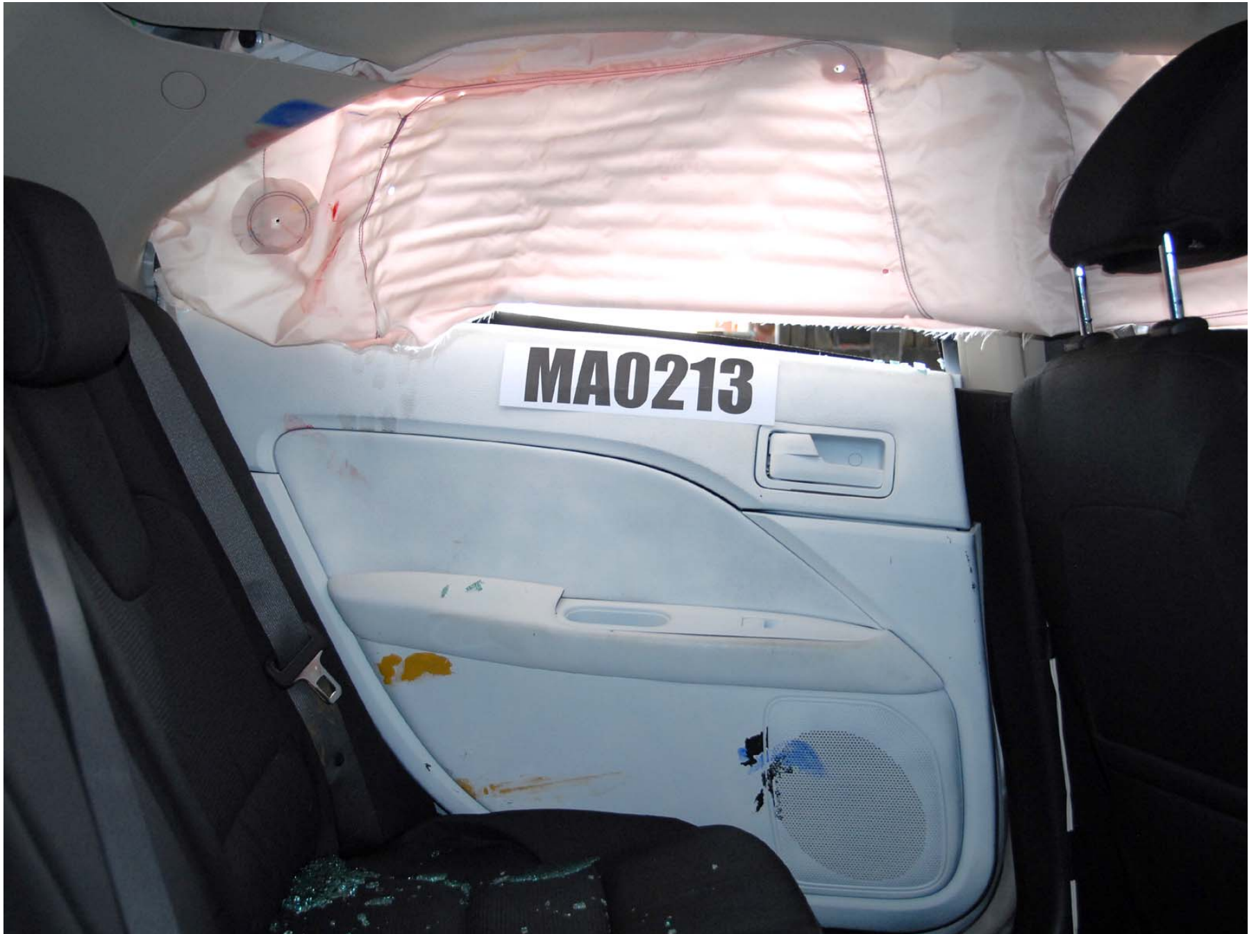
Figure A-50: Post-test Passenger Inner Door Panel View (with Dummy Removed)
