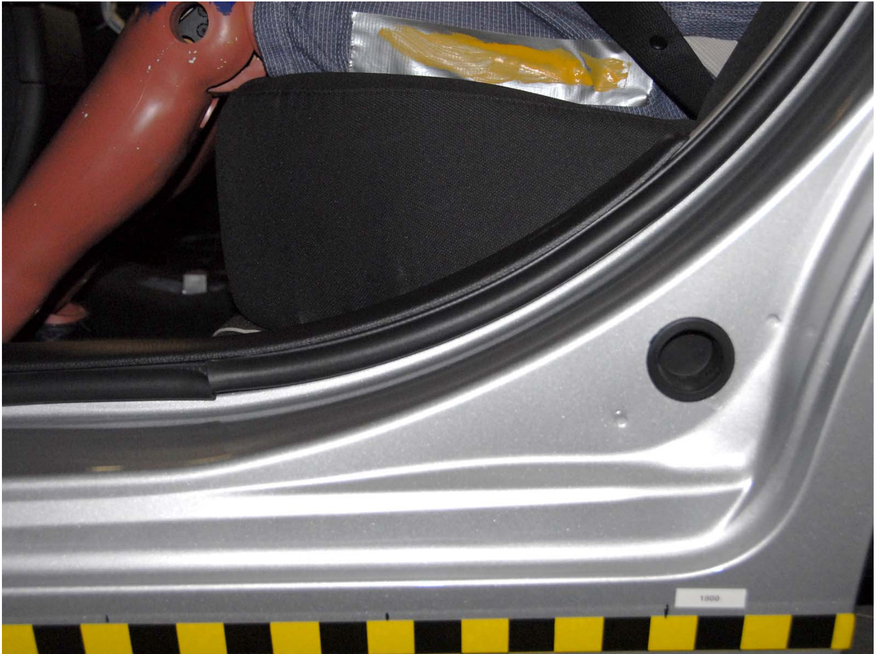
Figure A-43: Pre-test Close-Up Left Side View of Passenger Seat Track Showing Seat Positioning
