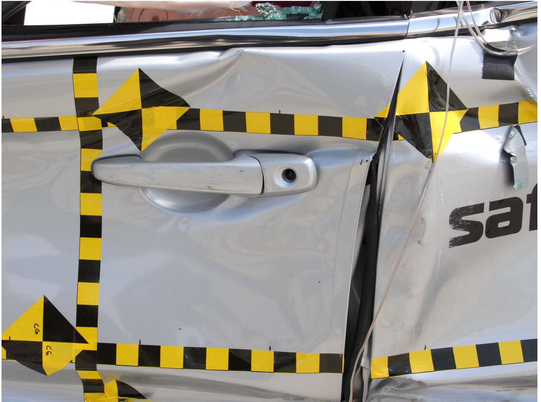
Figure A-22: Post-test Left Front Door Latch Close-Up
