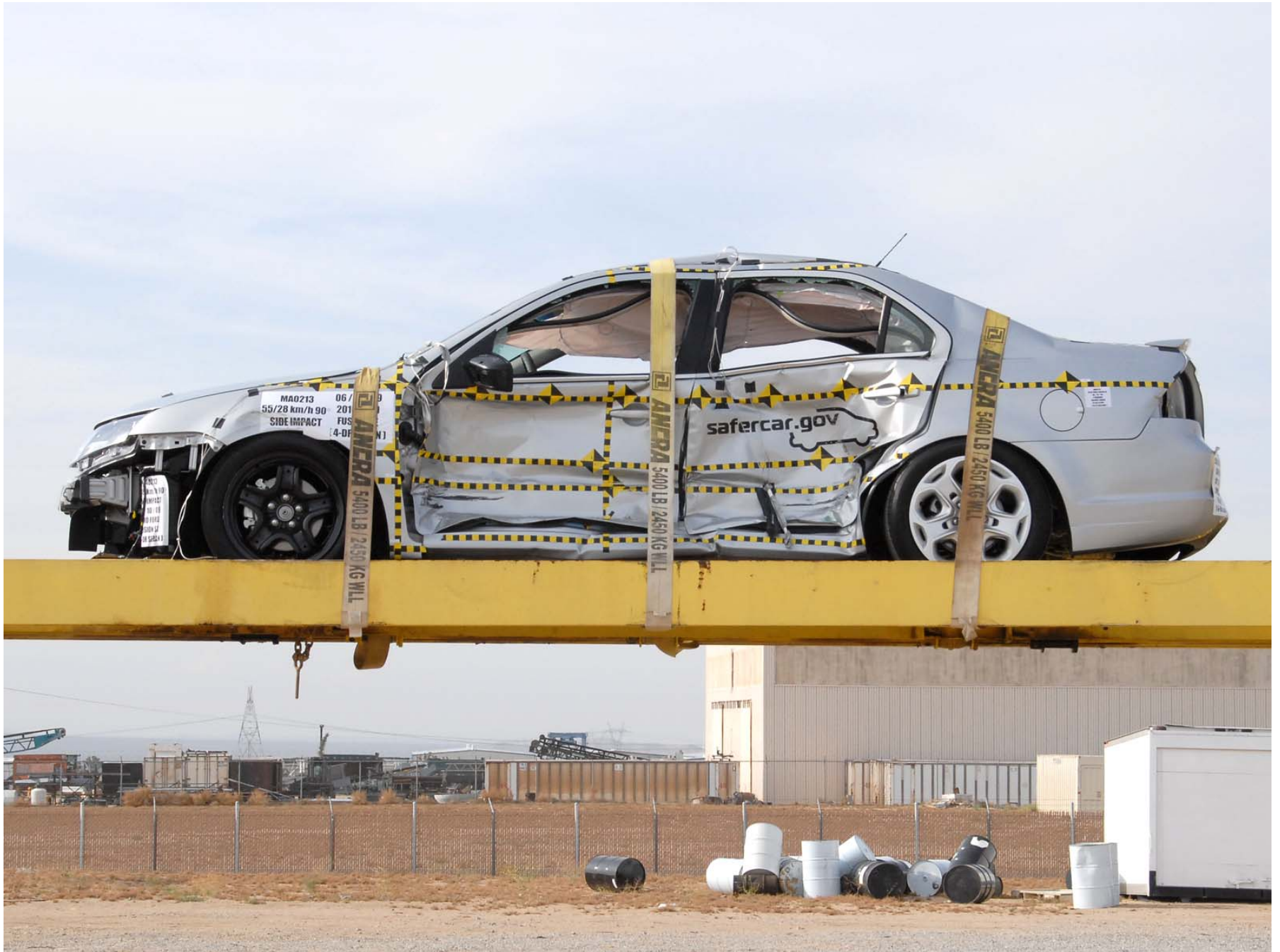
Figure A-64: FMVSS 301/305 Rollover 0°
