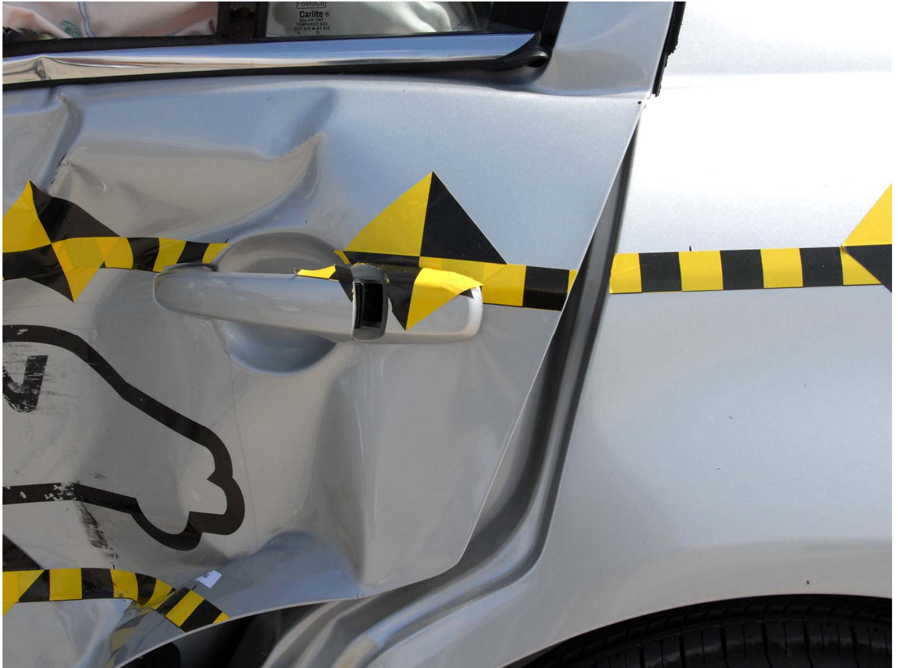
Figure A-24: Post-test Left Rear Door Latch Close-Up
