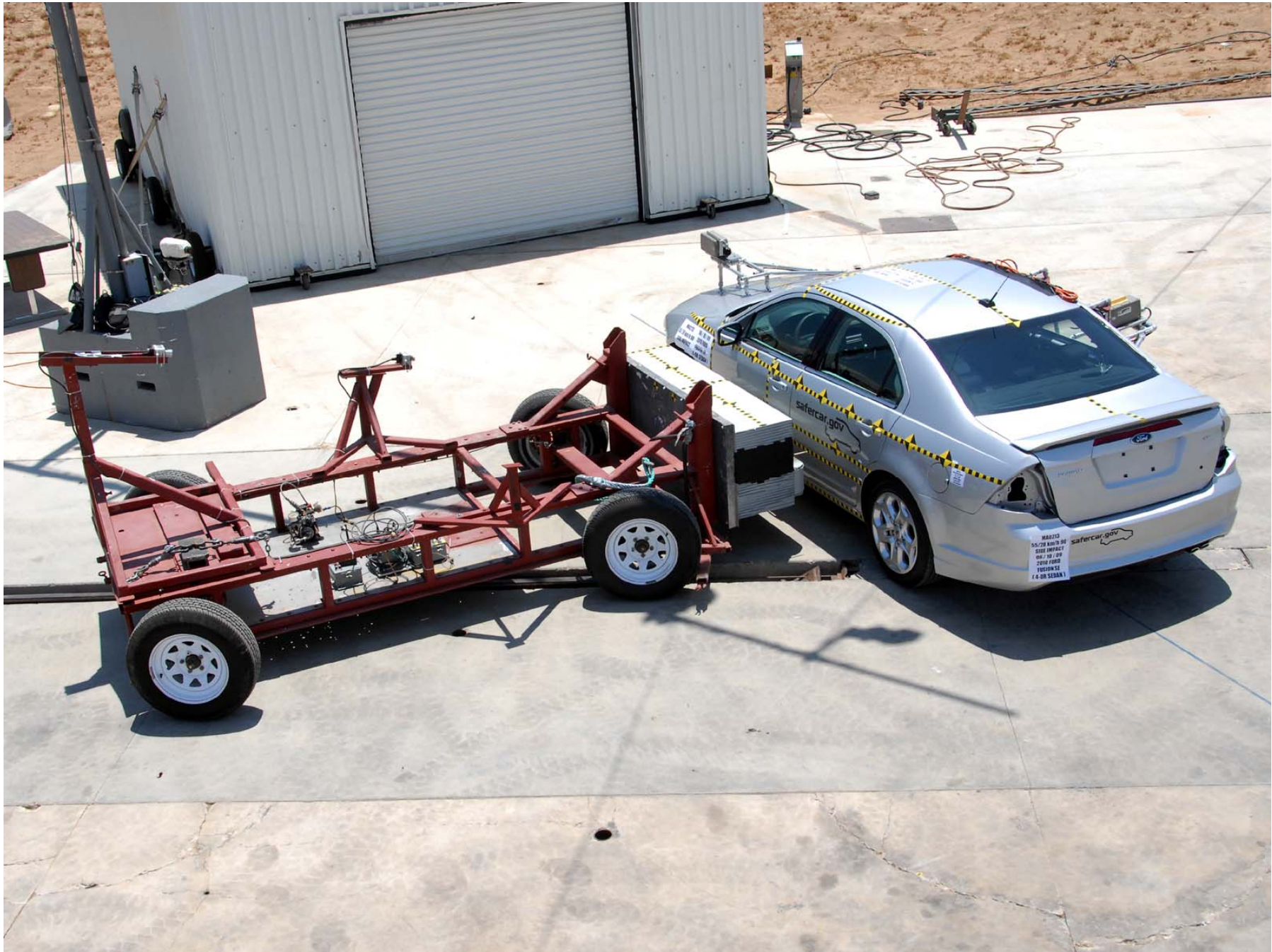
Figure A-15: Pre-test Overhead View of the Test Vehicle with MDB Positioned Against the Side of the Test Vehicle
