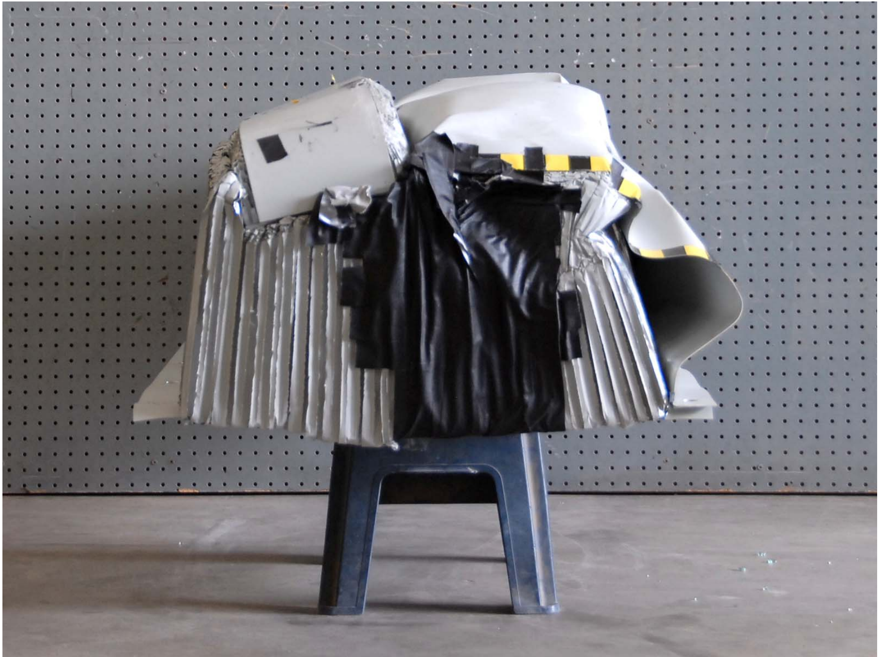
Figure A-60: Post-test Left Side View of MDB Impactor Face
