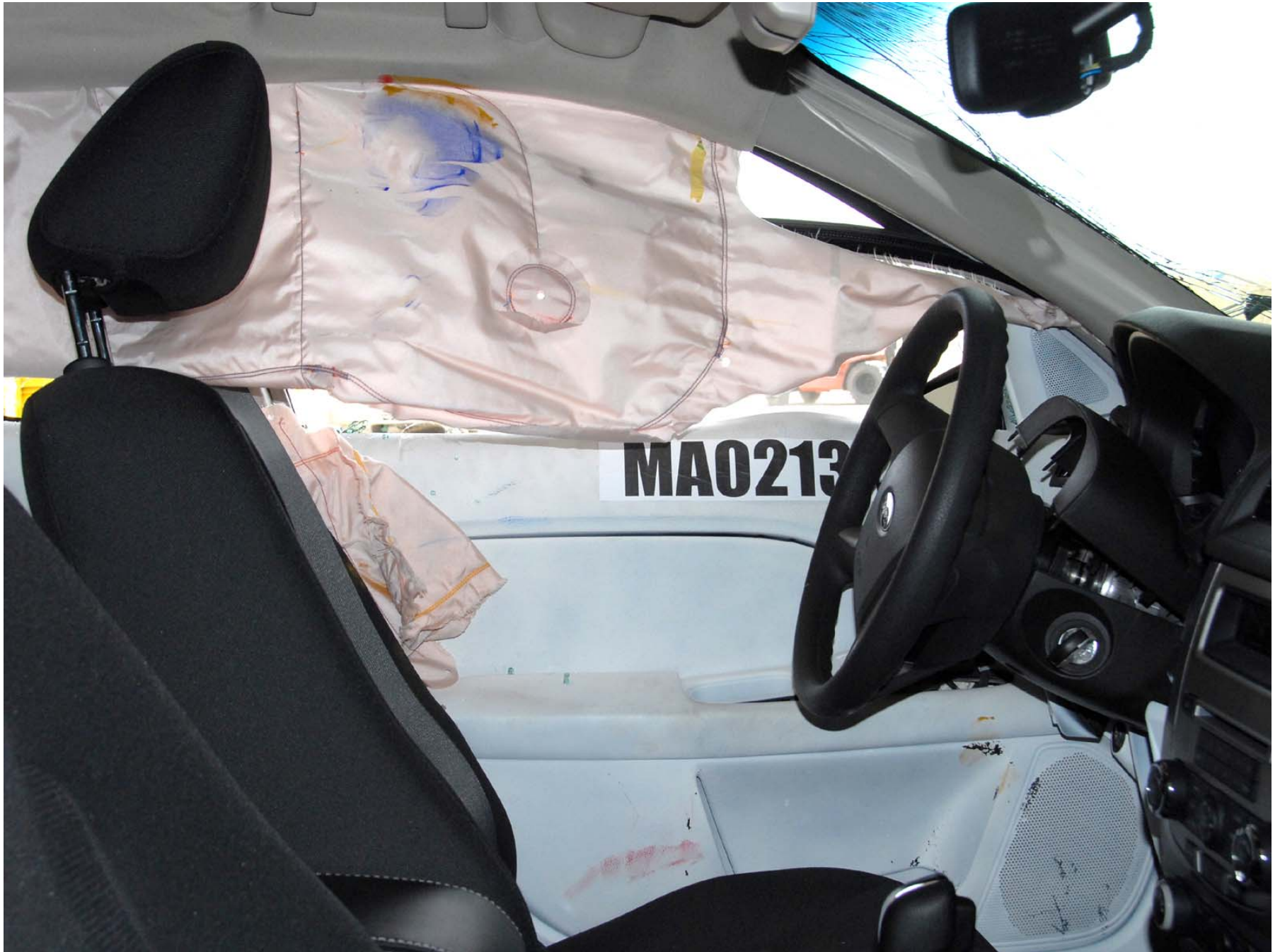
Figure A-37: Post-test Driver Inner Door Panel View (with Dummy Removed)
