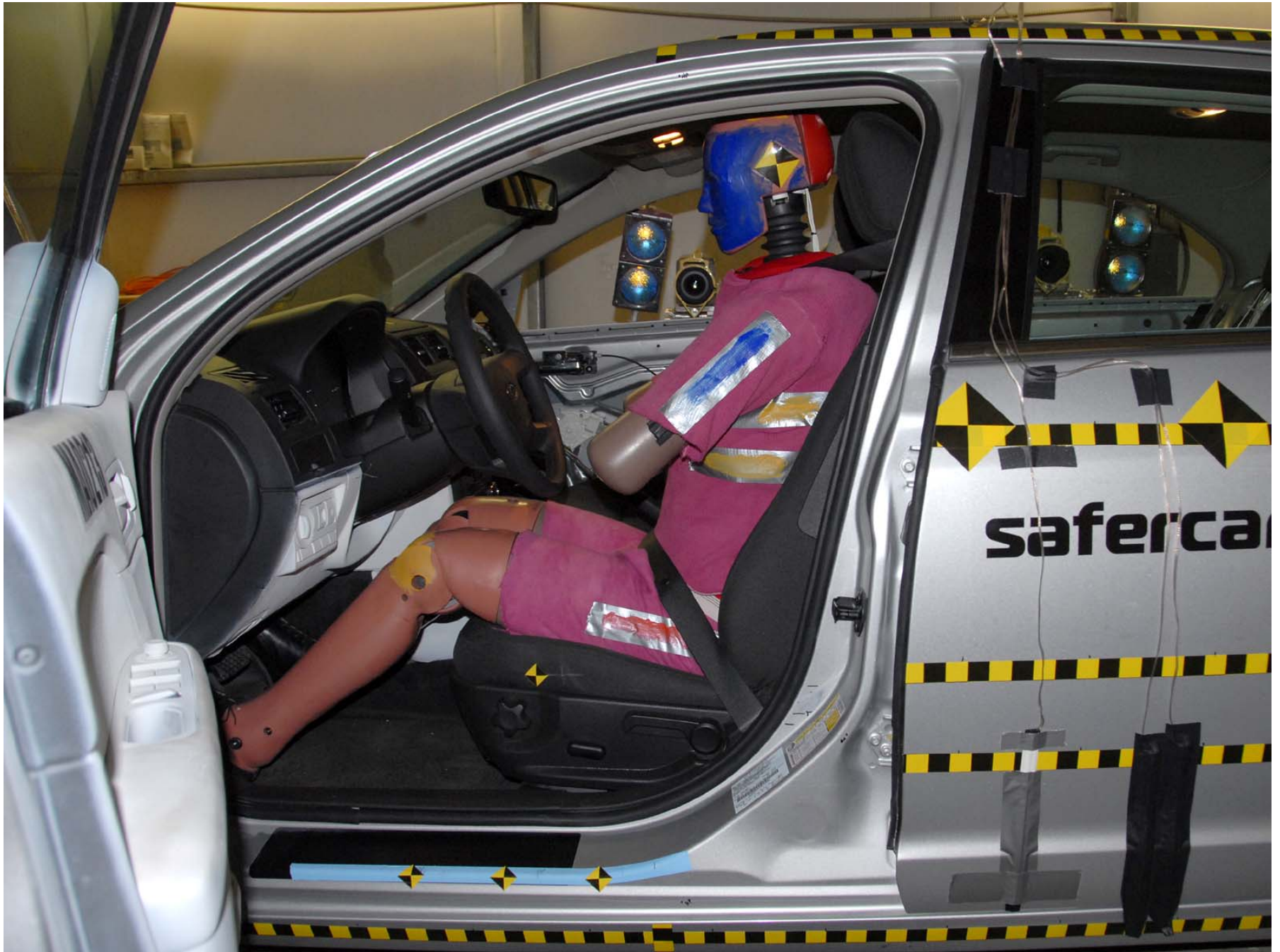
Figure A-27: Pre-test Left Side View of Driver Dummy Showing Belt, Chalking, and Contact Switches (Door Open)
