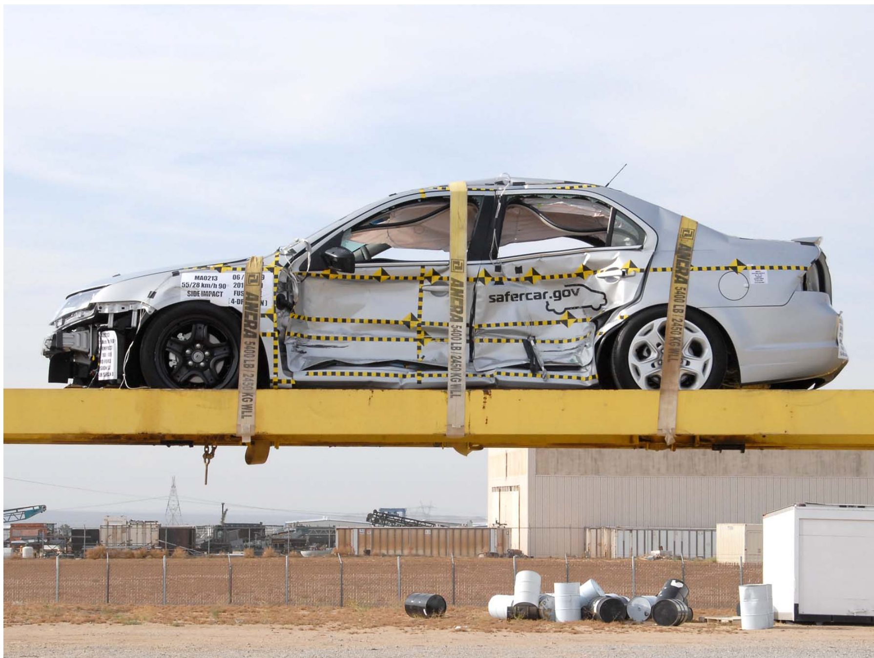
Figure A-64: FMVSS 301/305 Rollover 0°
