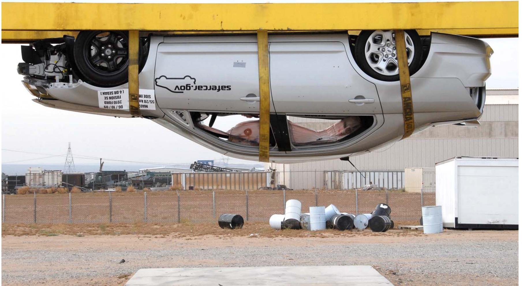
Figure A-66: FMVSS 301/305 Rollover 180°
