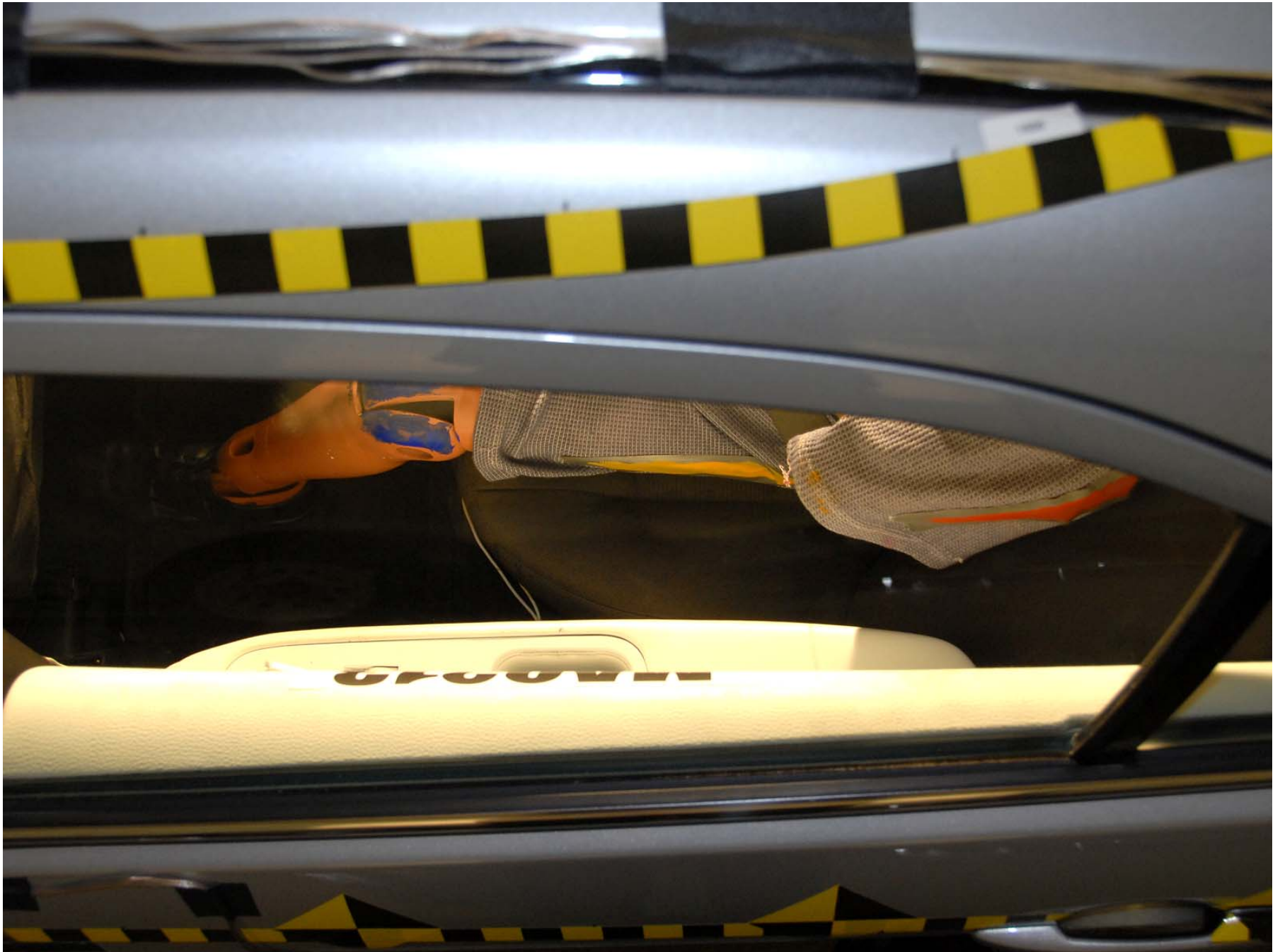
Figure A-45: Pre-test Passenger Dummy and Door Clearance View
