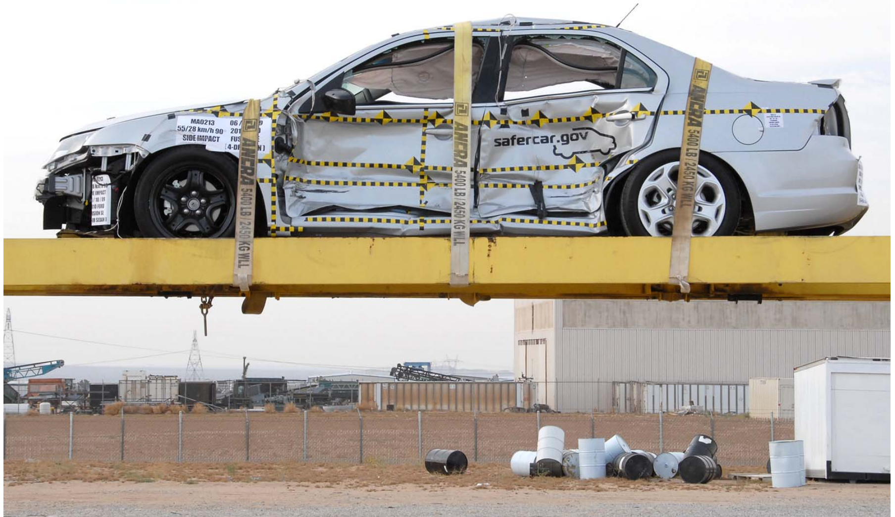
Figure A-68: FMVSS 301/305 Rollover 360°
