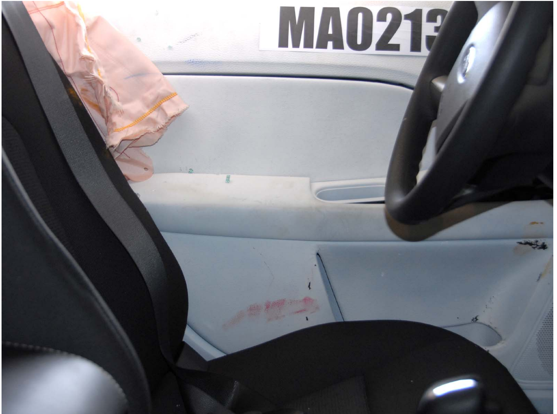
Figure A-39: Post-test Driver Dummy Door Contact View
