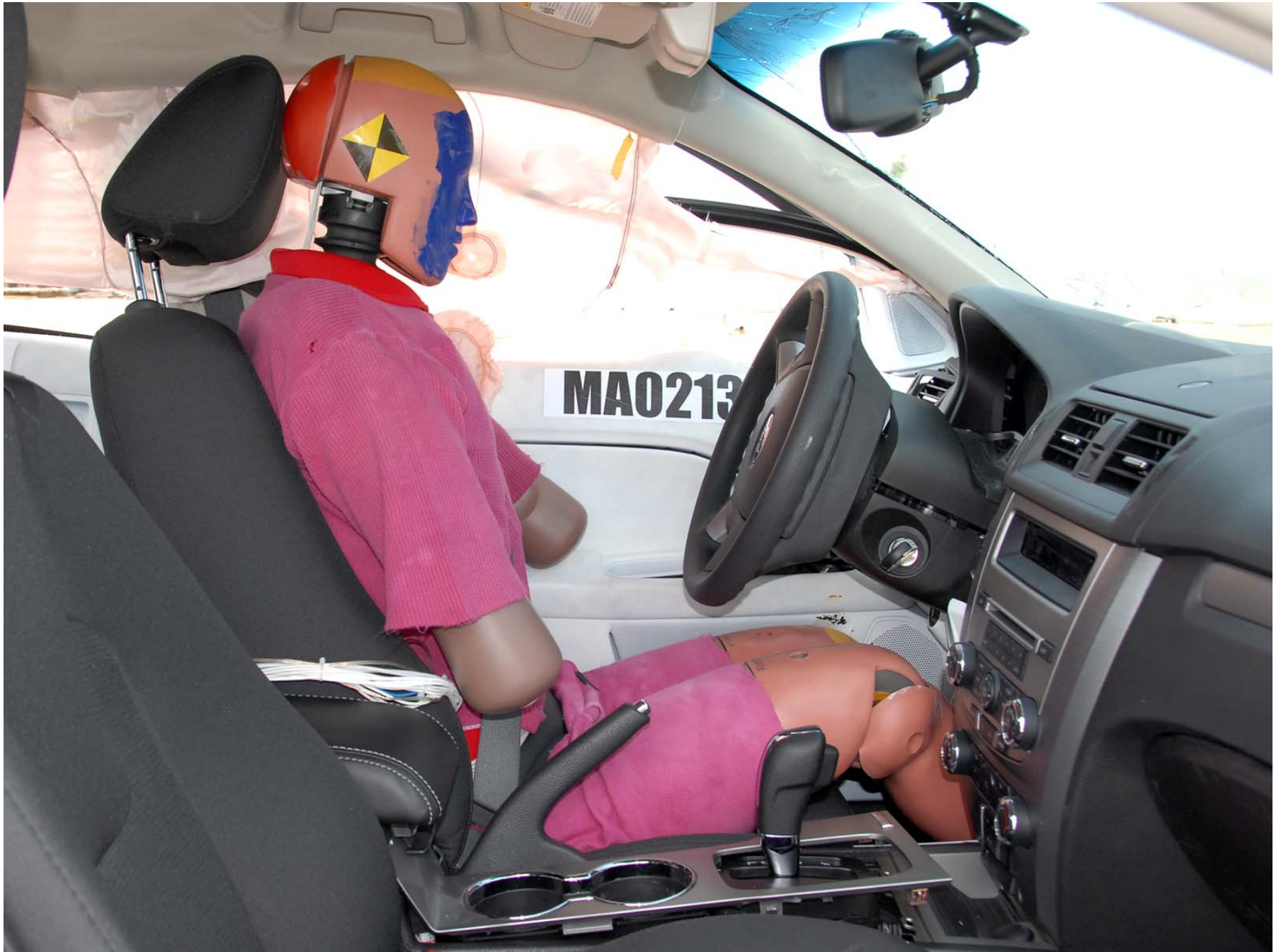
Figure A-35: Post-test Right Side View of Front Seat of Occupant Compartment (Through Window with Dummy)
