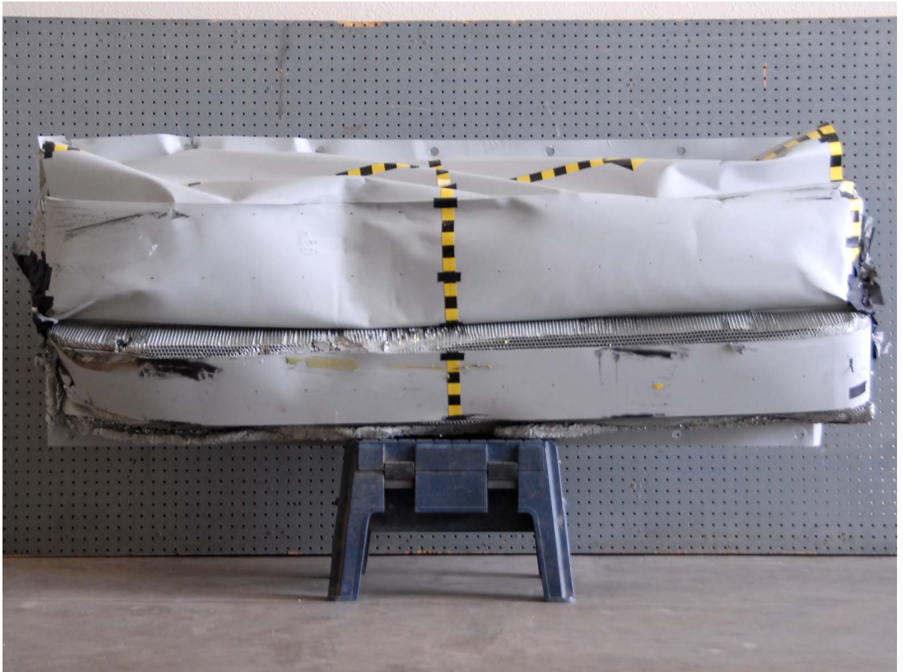
Figure A-56: Post-test Front View of MDB Impactor Face
