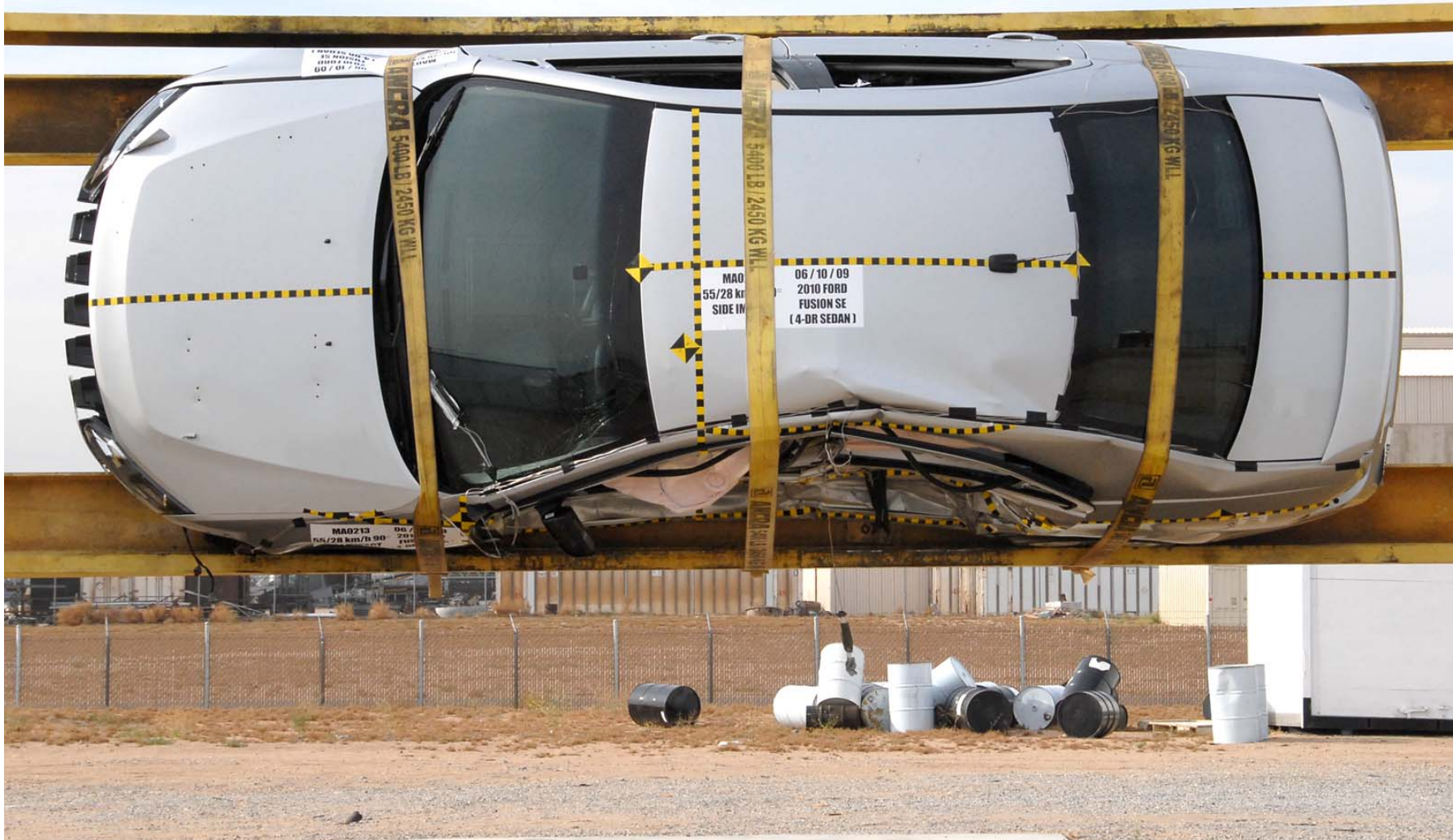
Figure A-65: FMVSS 301/305 Rollover 90°
