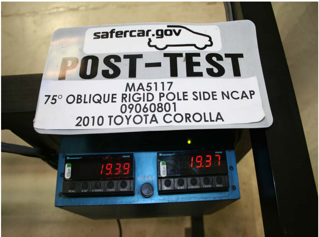
Post-Test Primary and Redundant Speed Trap Read-Out
