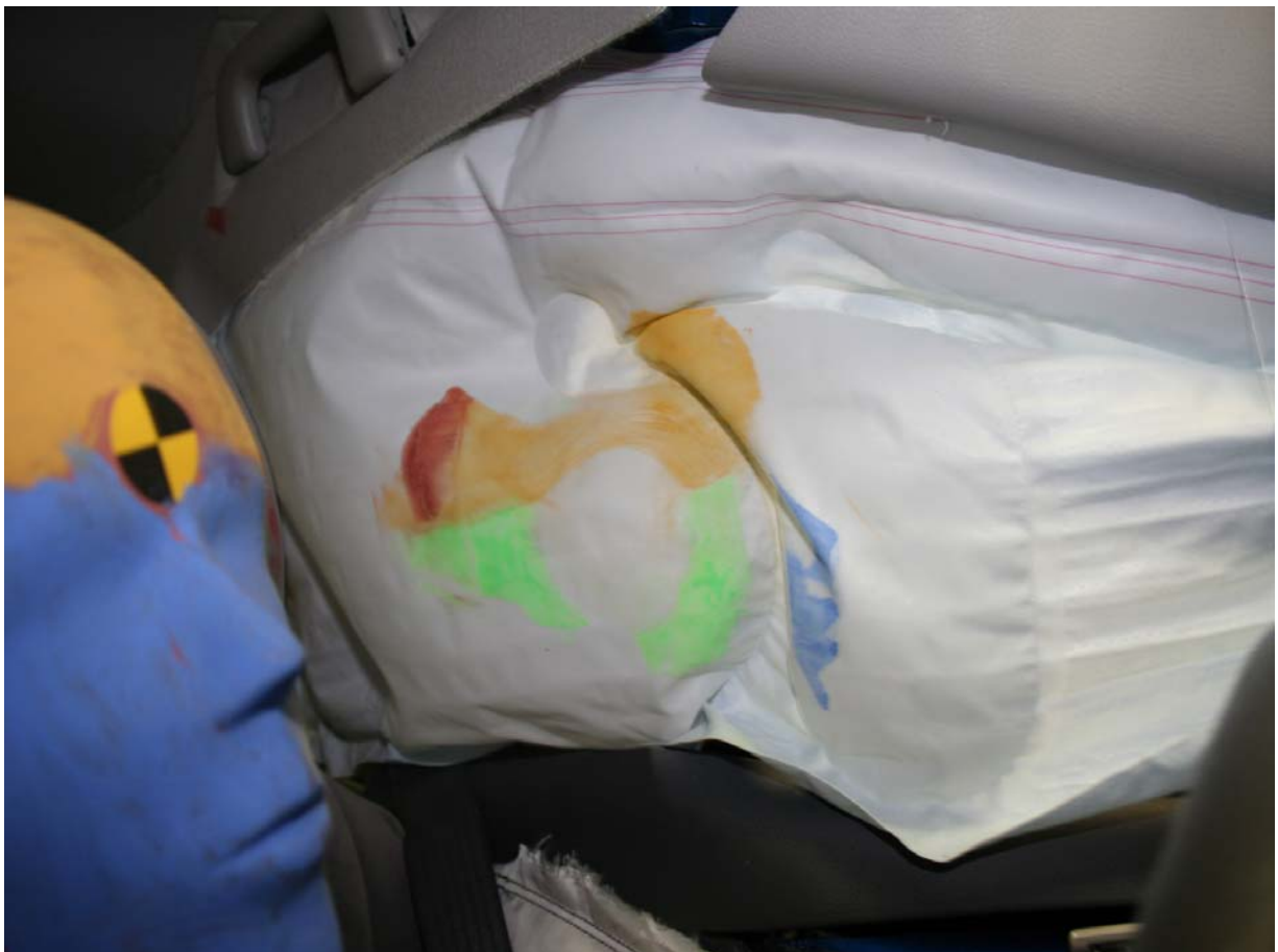
Post-Test Dummy Close-Up Head Contact with Side Airbag View, if applicable
