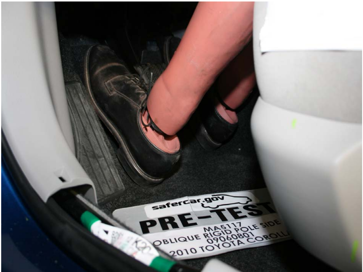
Pre-Test Placement of Dummy's Feet
