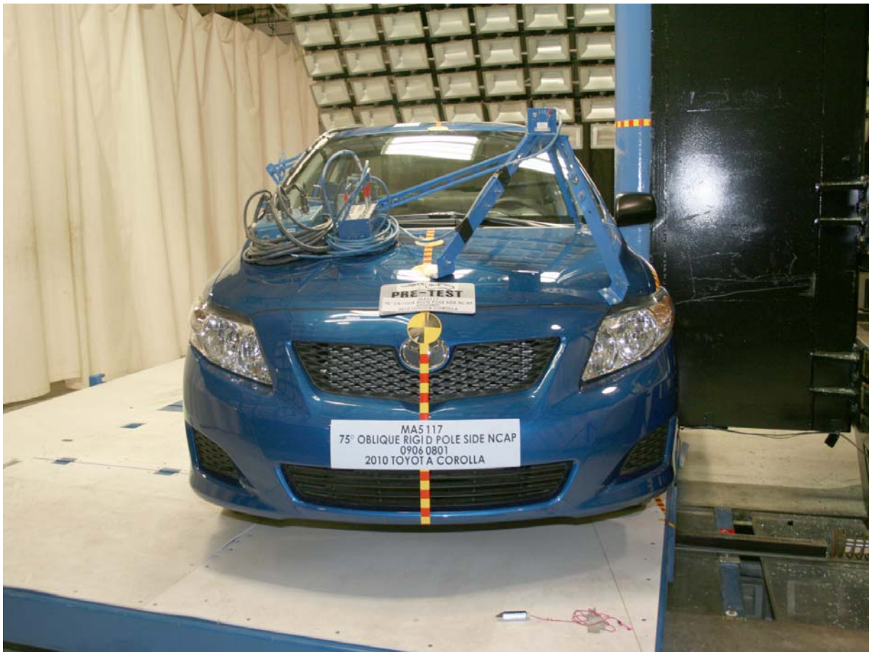
Pre-Test Frontal View of Test Vehicle
