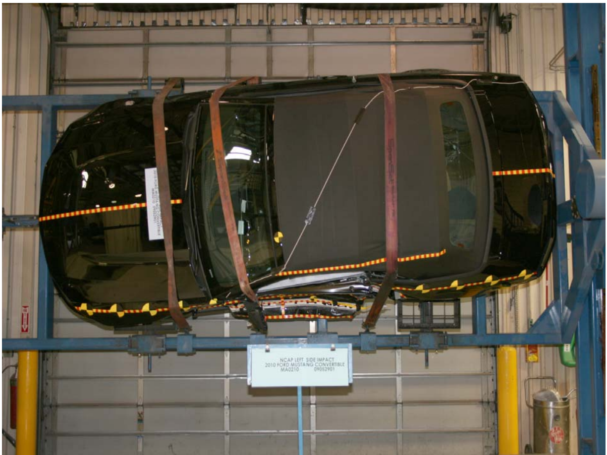
FMVSS No. 301/305 Rollover 90 Degrees
