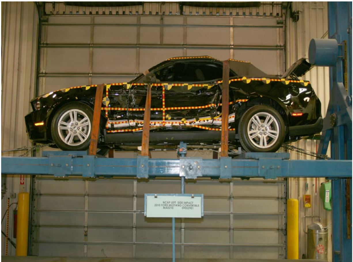
FMVSS No. 301/305 Rollover 360 Degrees
