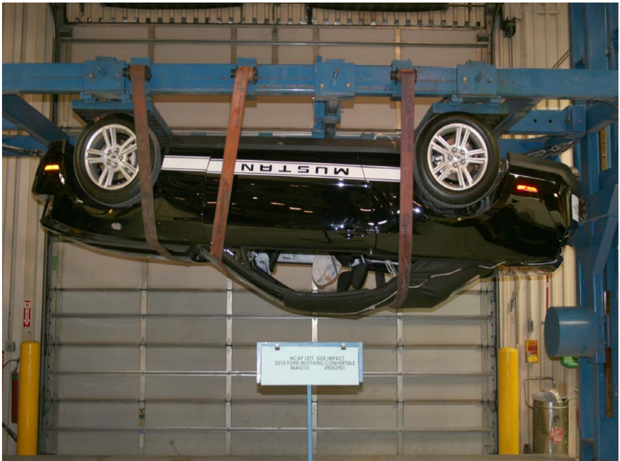
FMVSS No. 301/305 Rollover 180 Degrees
