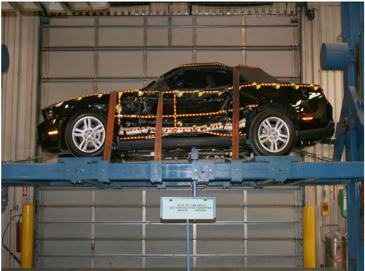
FMVSS No. 301/305 Rollover 0 Degrees
