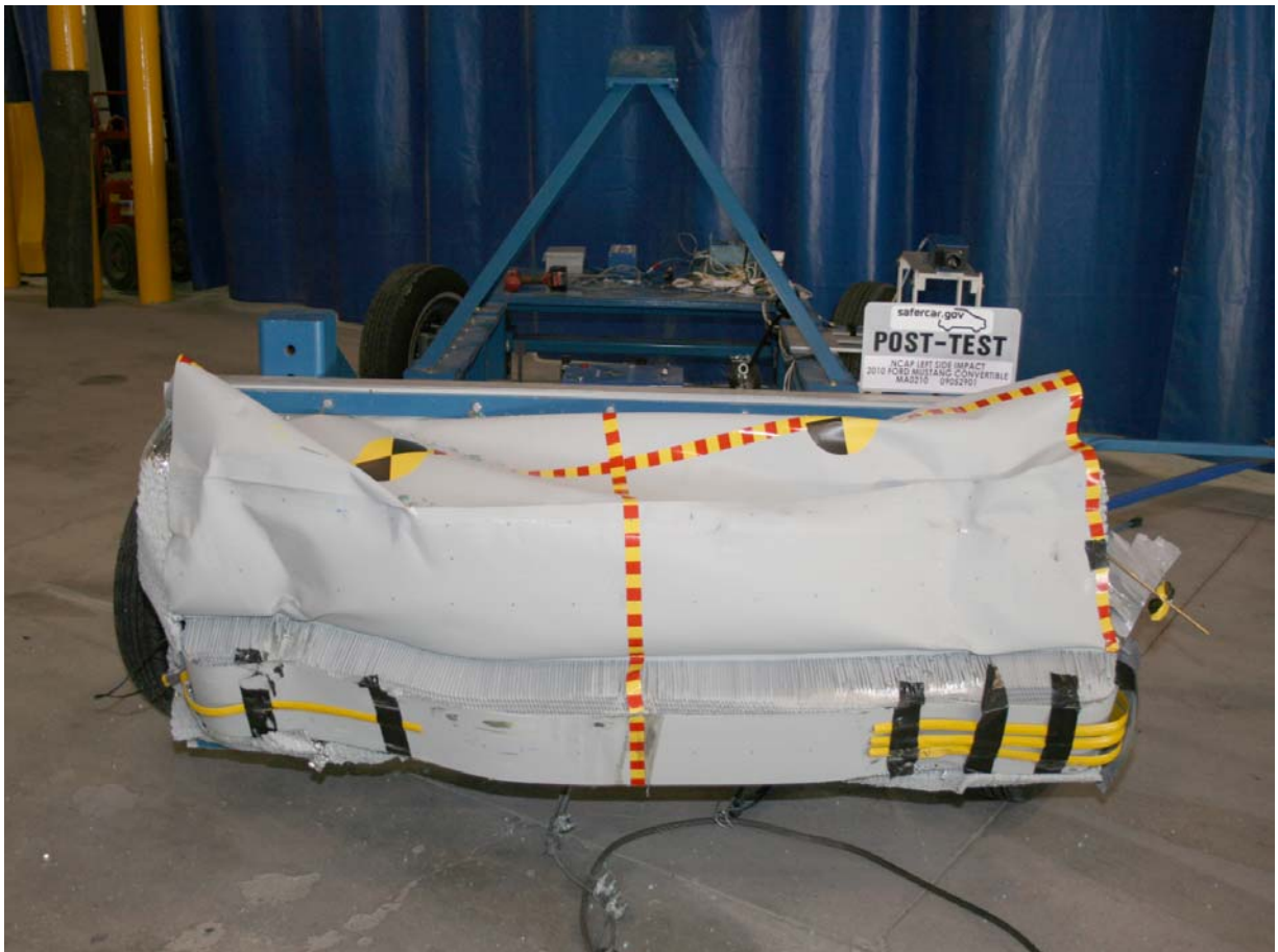
Post-Test Front View of MDB Impactor Face
