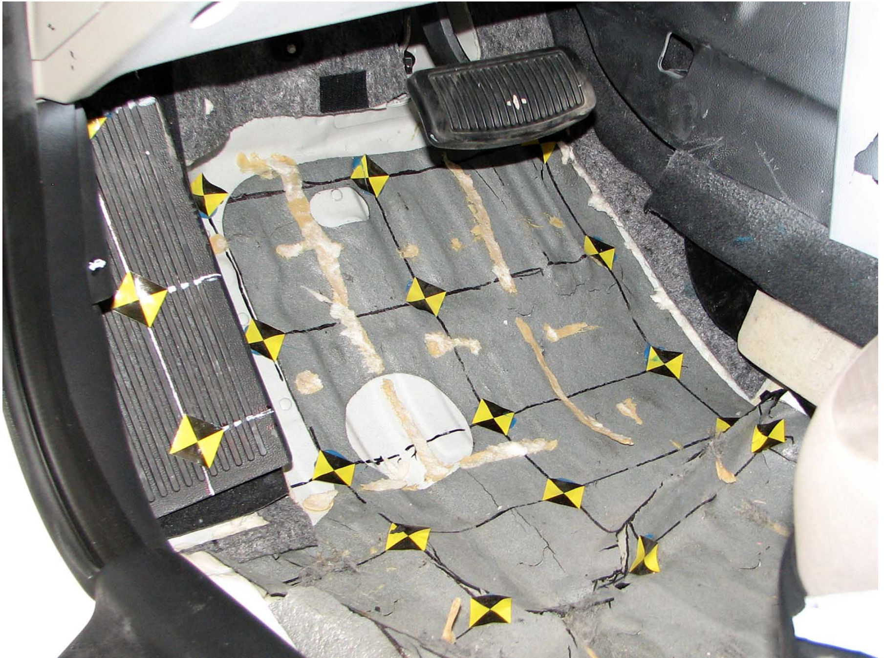
Figure A-41: Post-Test Driver's Side Floorpan
