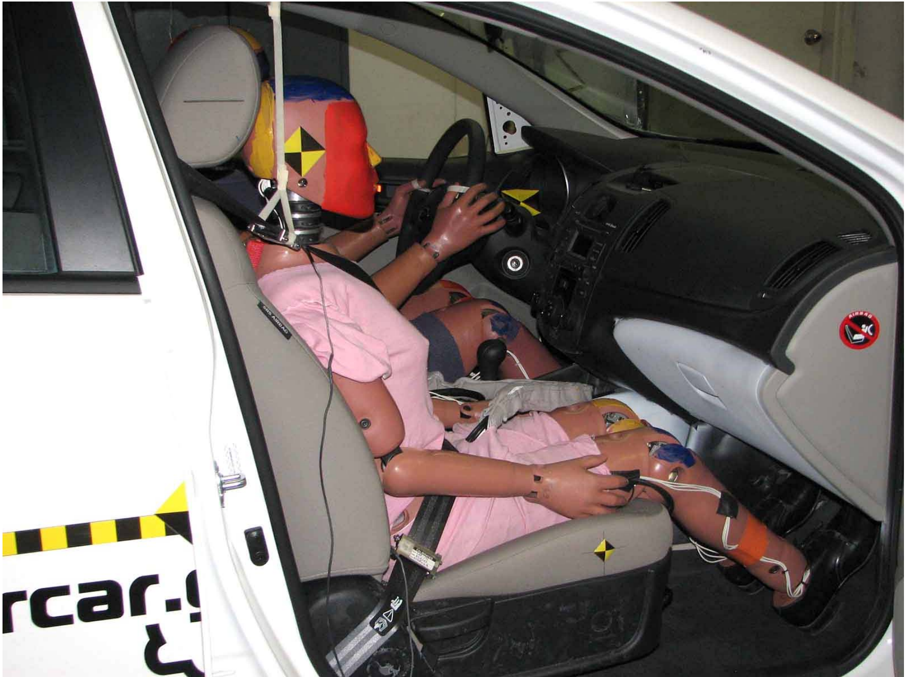
Figure A-51: Pre-Test Passenger Dummy and Vehicle Interior
