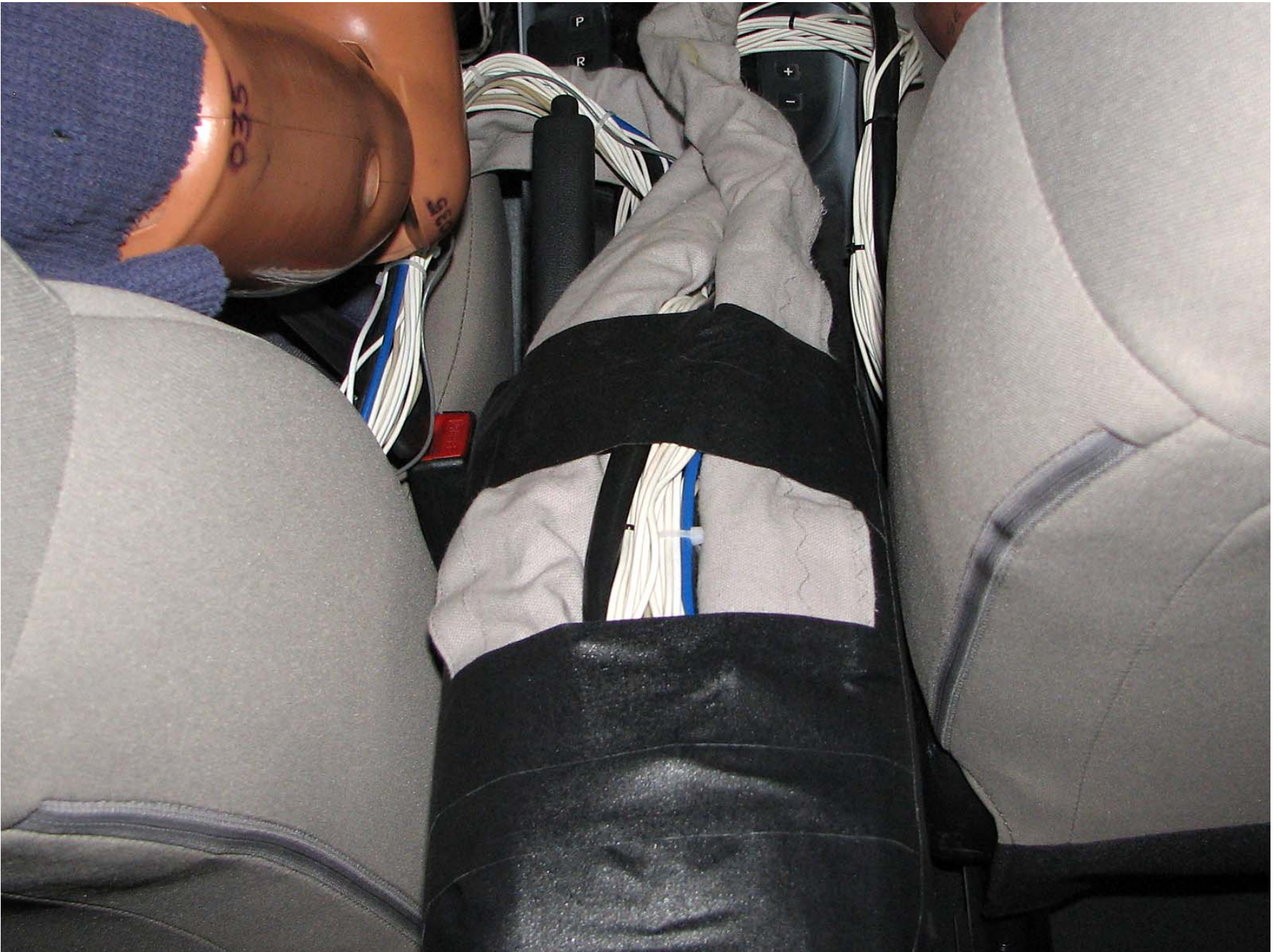
Figure A-26: Pre-Test Dummy Cable Routing
