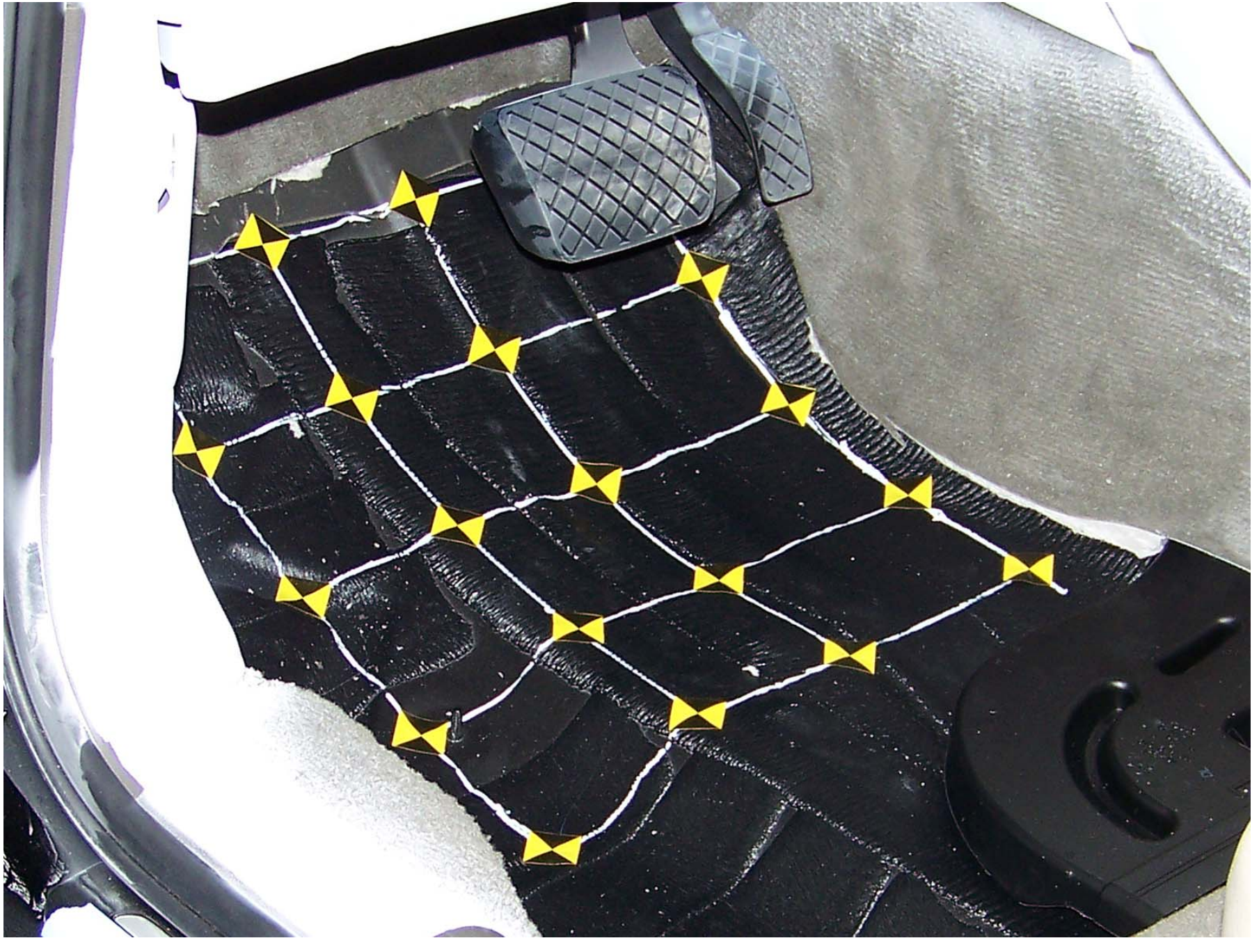
Figure A-40: Pre-Test Driver Side Floor Pan
