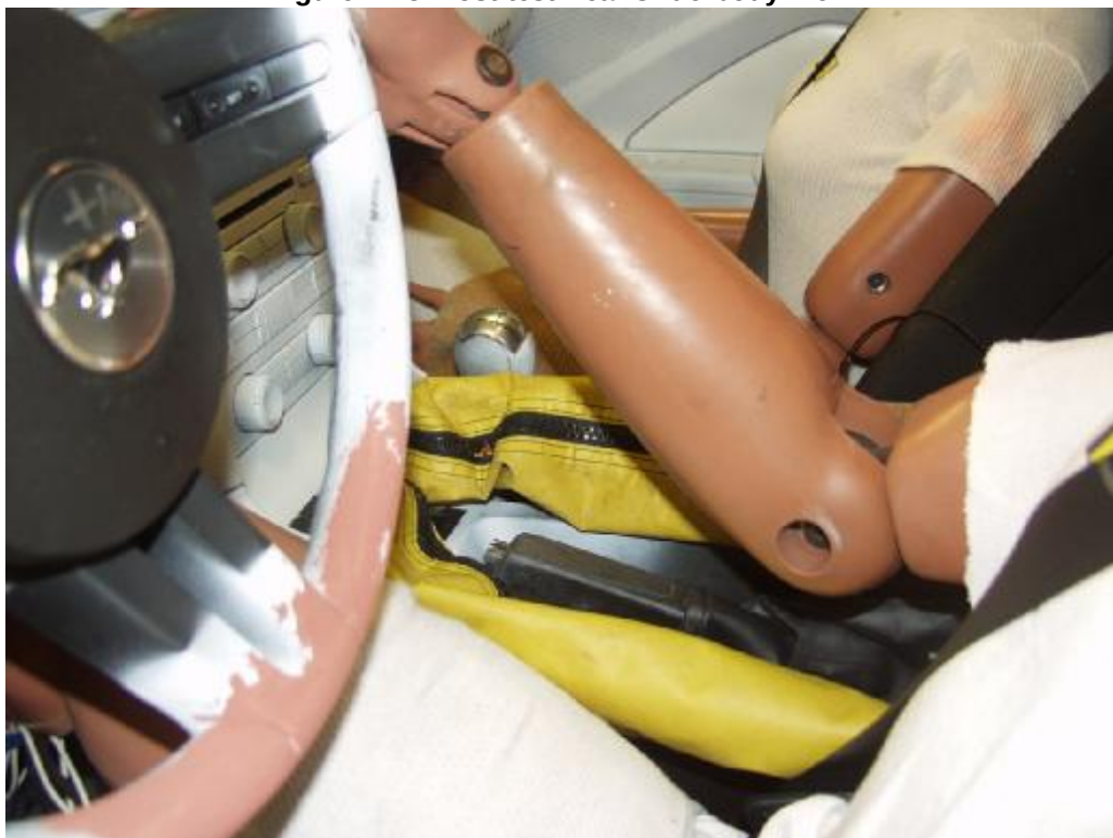
Figure A-26 Pre-test Dummy Cable Routing
