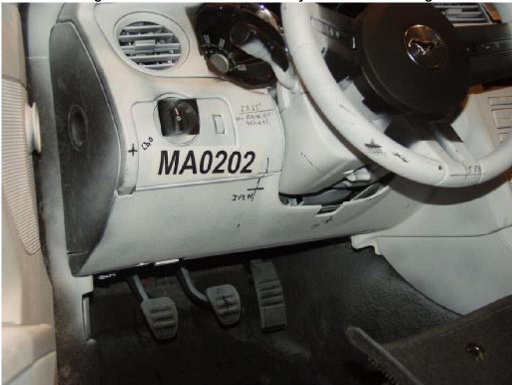
Figure A-43 Pre-test View of the Steering Column Shear Capsule
