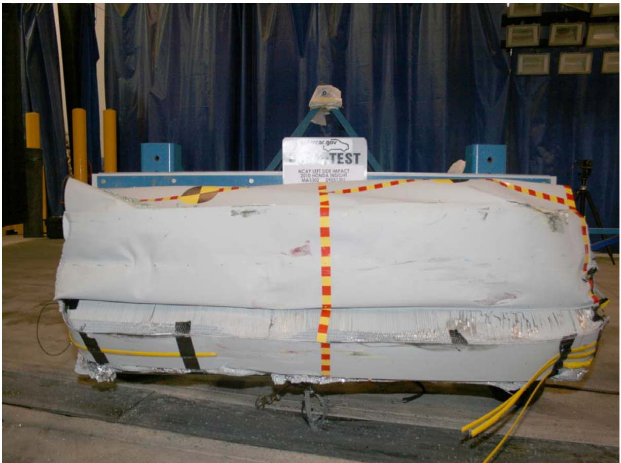
Post-Test Front View of Deformable Barrier
