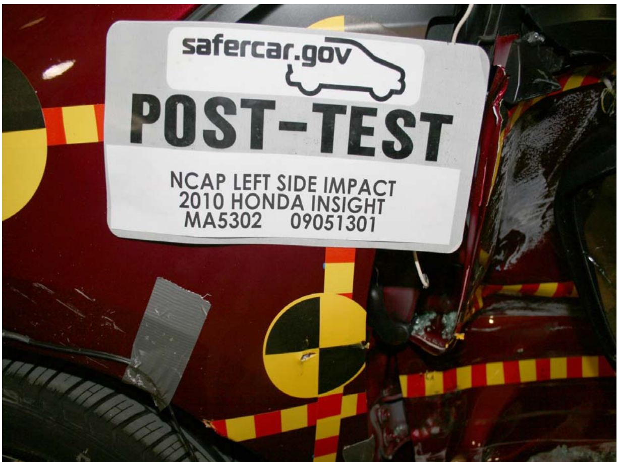
Post-Test Left Impact Point
