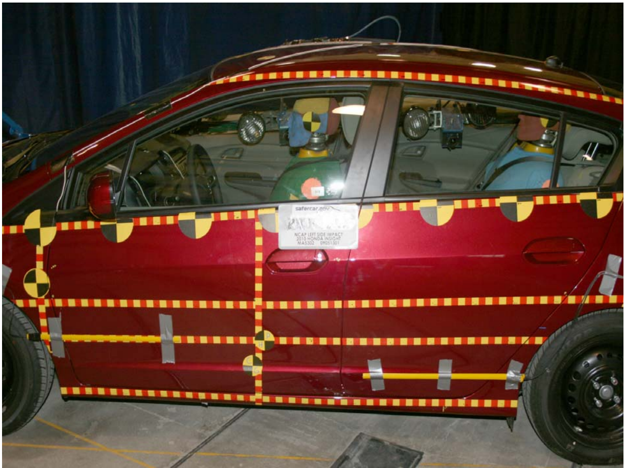
Pre-Test Left Side Impact Close-up
