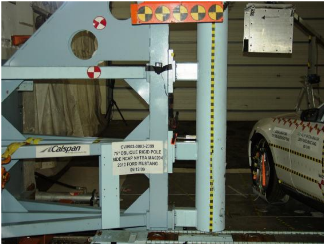
Figure A-57: Pre-Test Pole Barrier Side View
