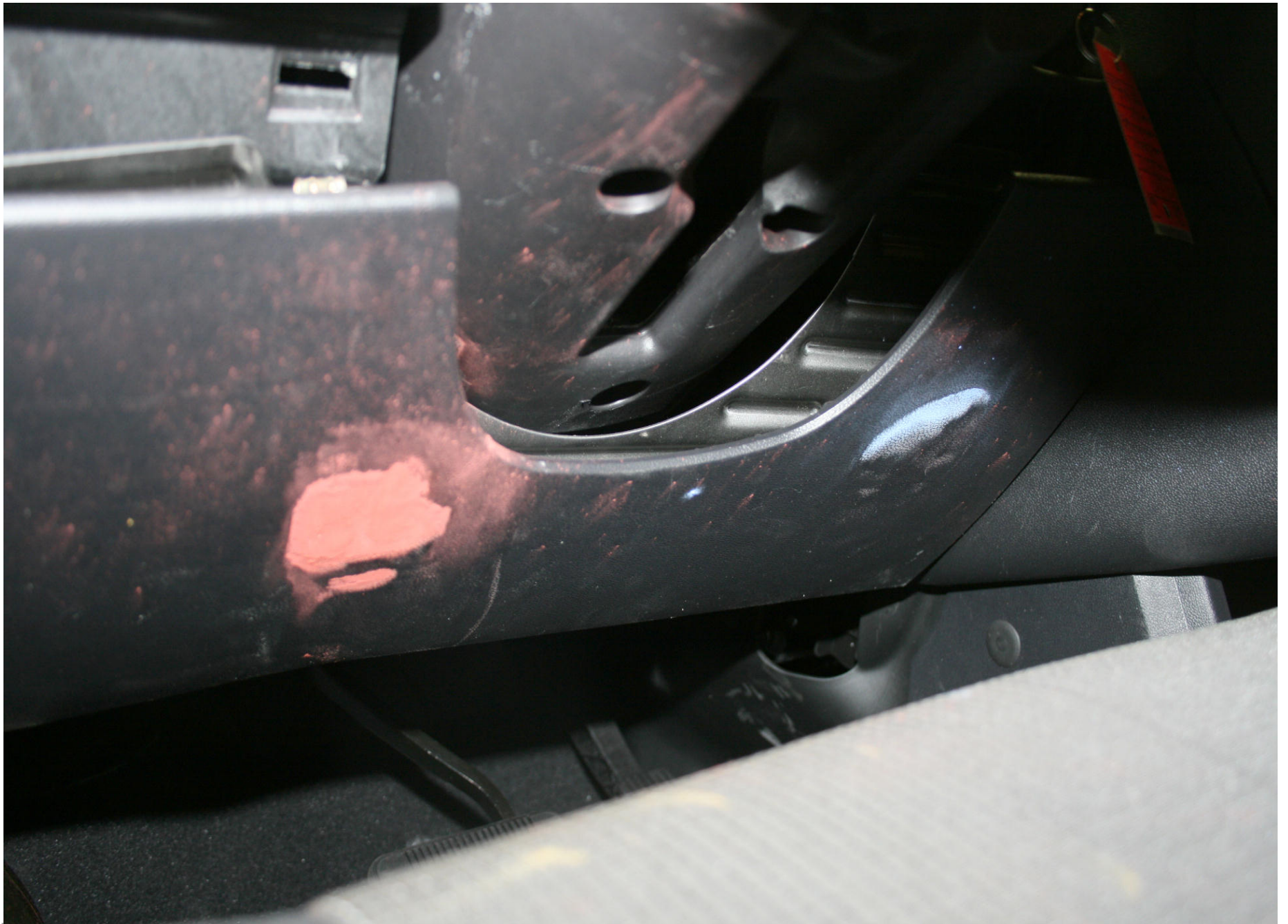
Post-Test Driver Dummy Knee Contact
