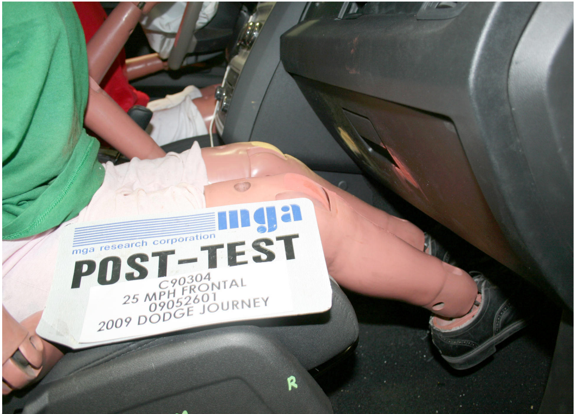
Post-Test Passenger Side Knee Bolster View
