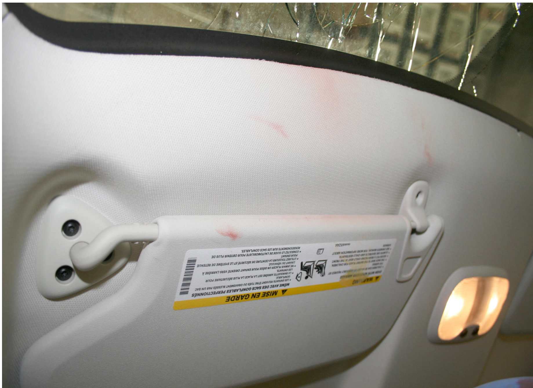
Post-Test Passenger Dummy Head Contact (headliner, visor)
