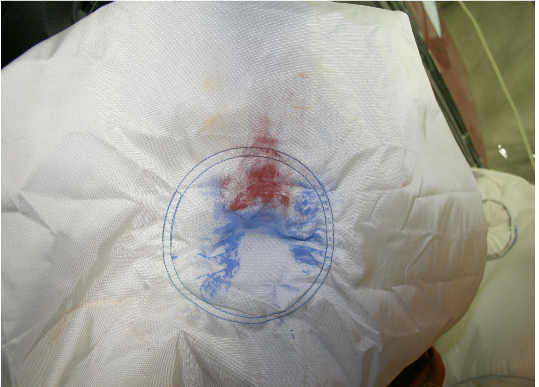
Post-Test Driver Dummy Airbag Contact
