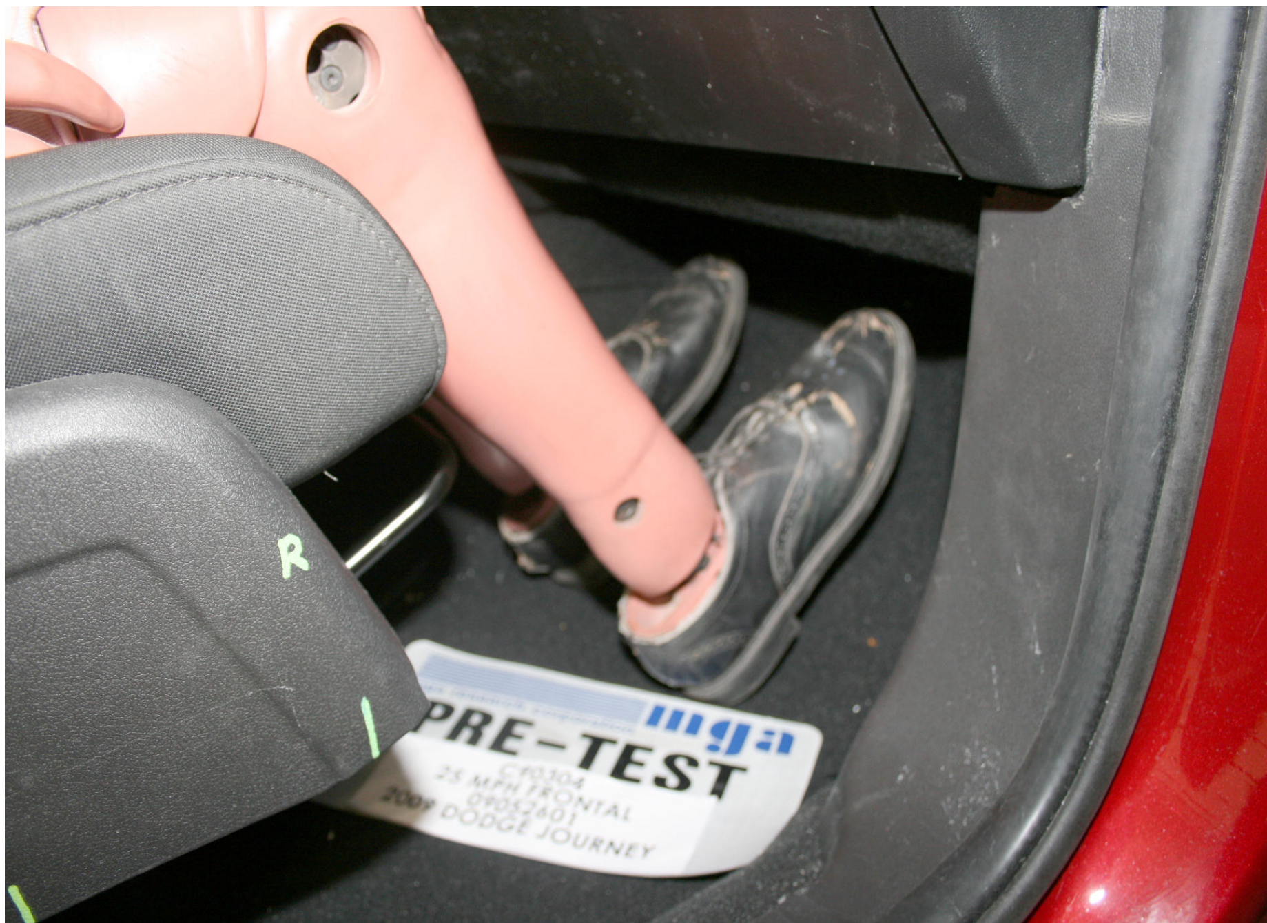
Pre-Test Passenger Dummy Feet Position
