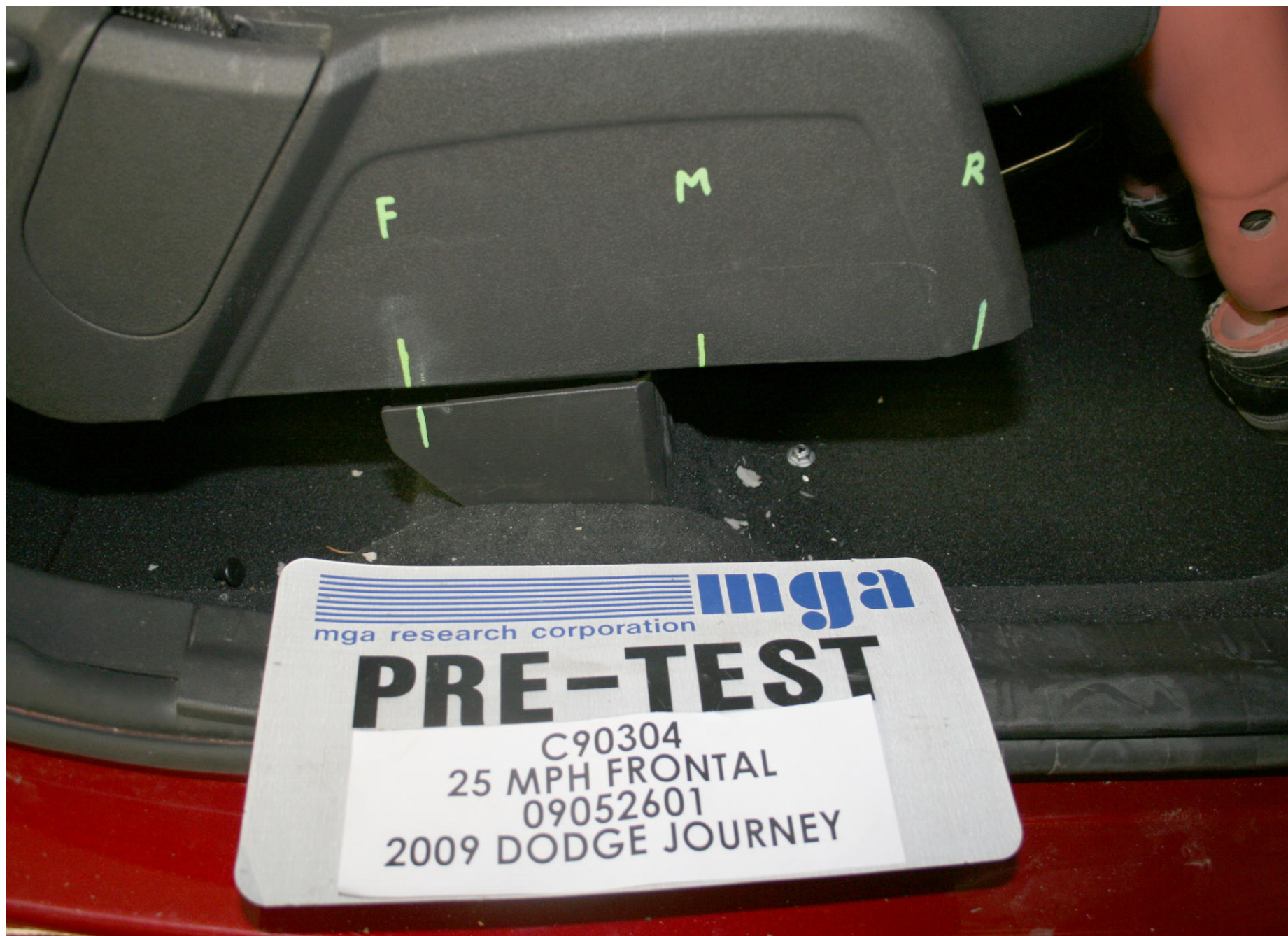
Pre-Test Passenger Dummy Seat Position
