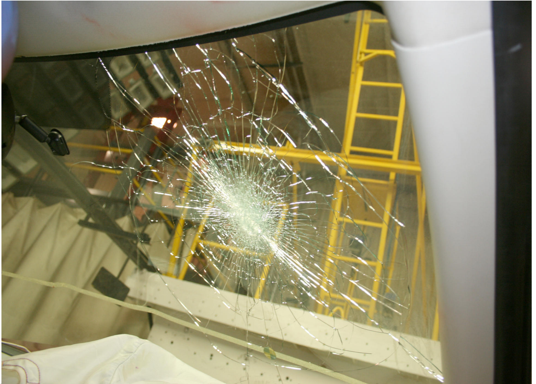
Post-Test Passenger Dummy Head Contact (windshield)
