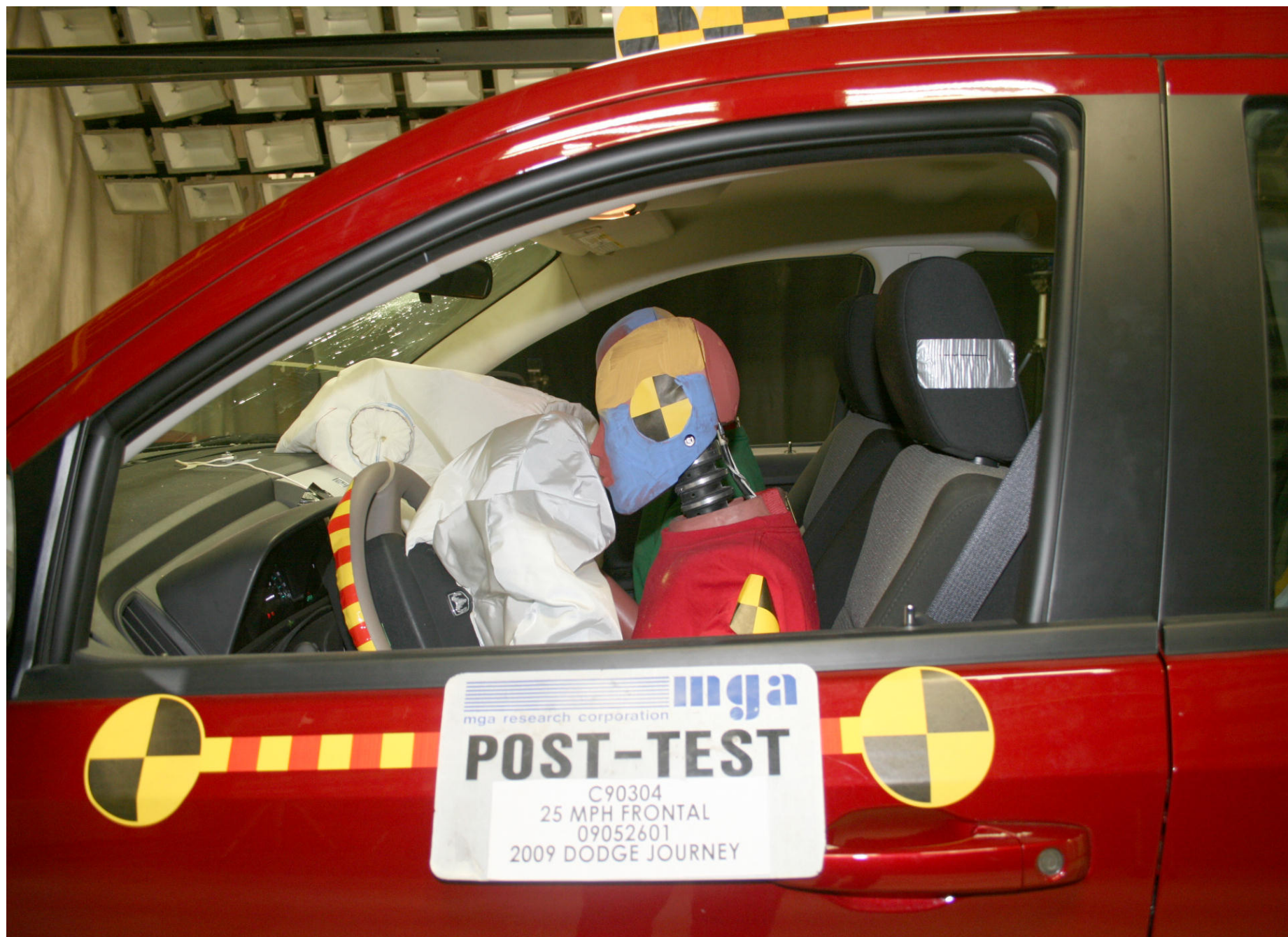
Post-Test Driver Dummy Position Left Side View
