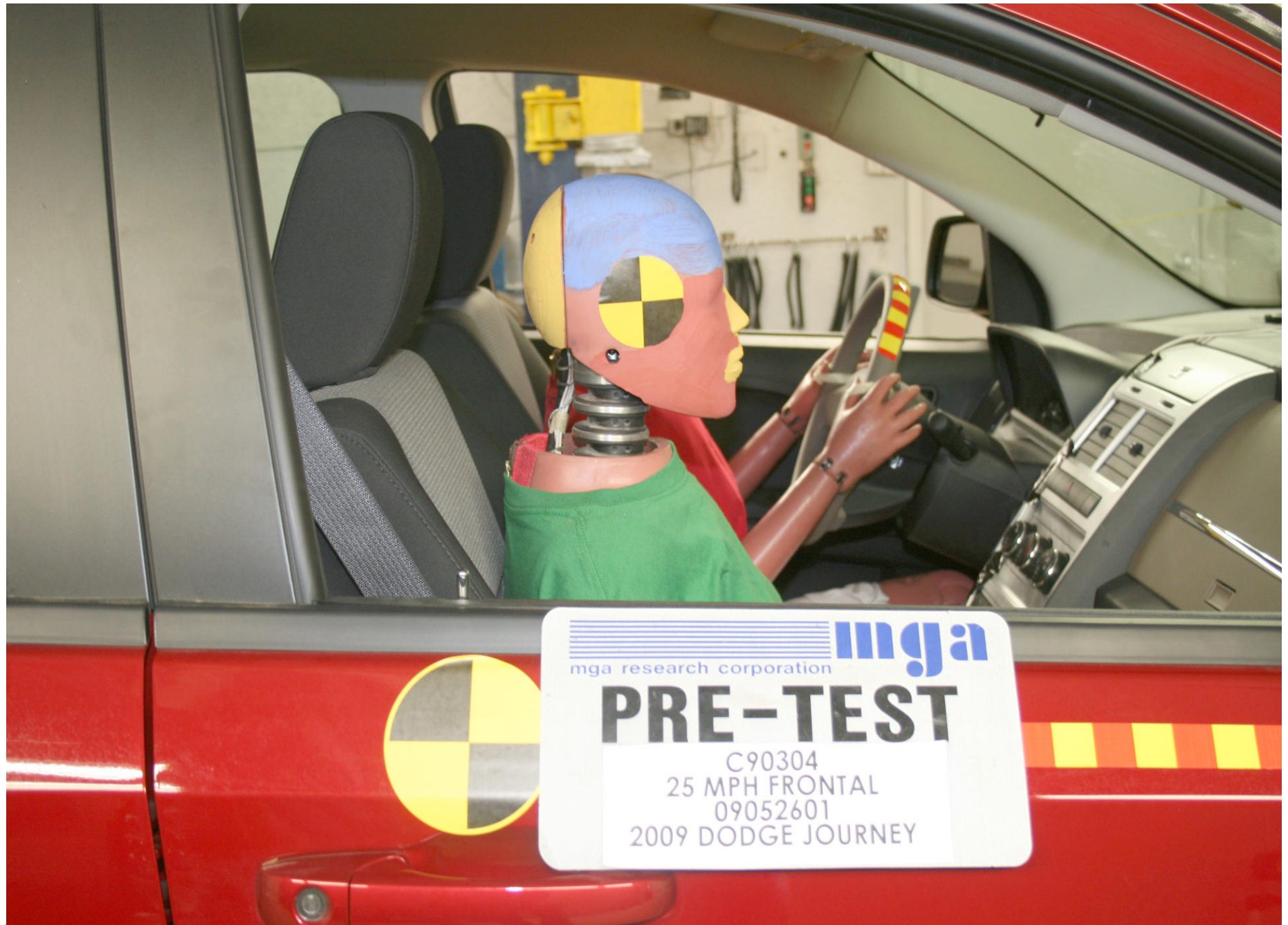
Pre-Test Passenger Dummy Position Right Side View
