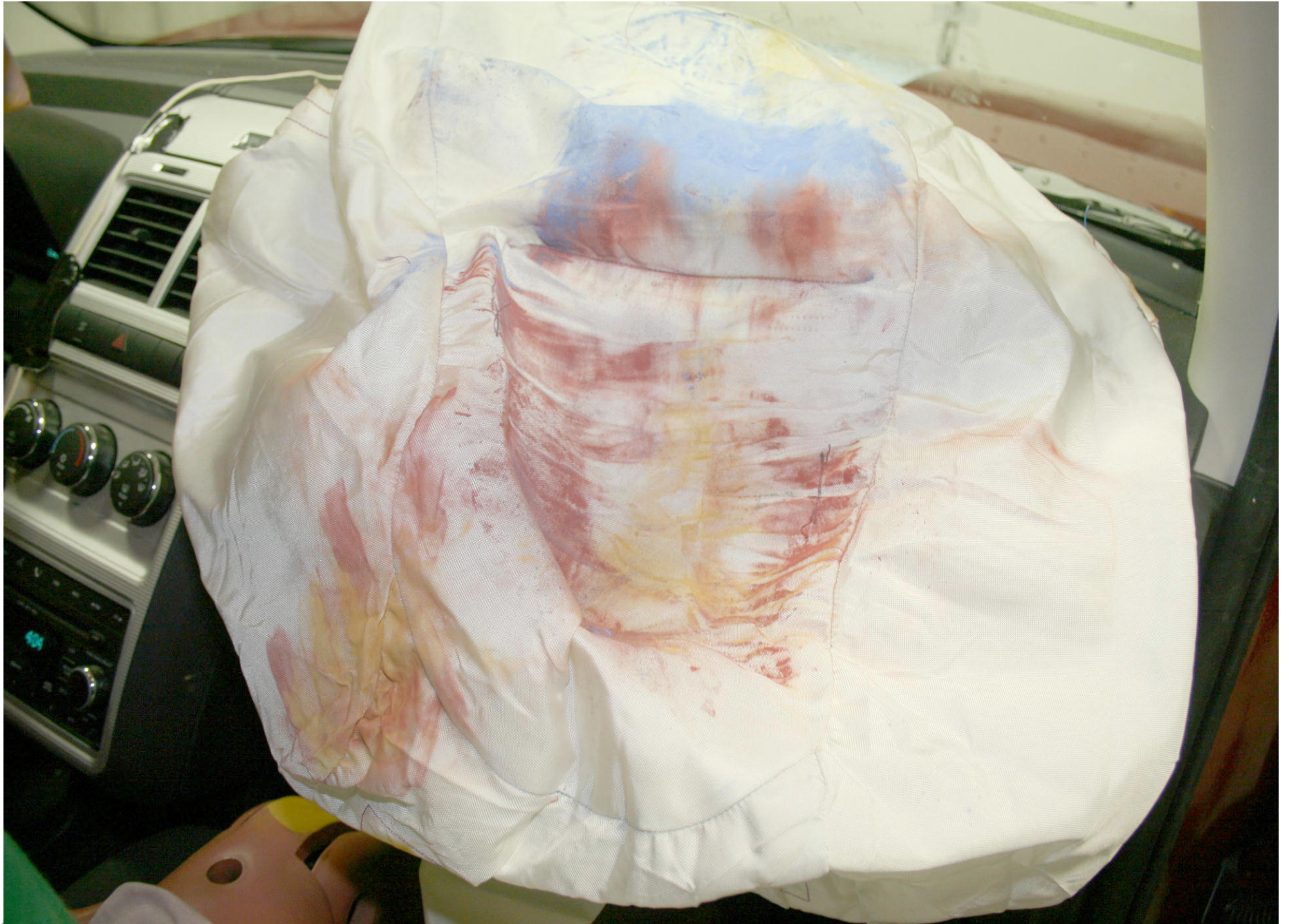
Post-Test Passenger Dummy Airbag Contact
