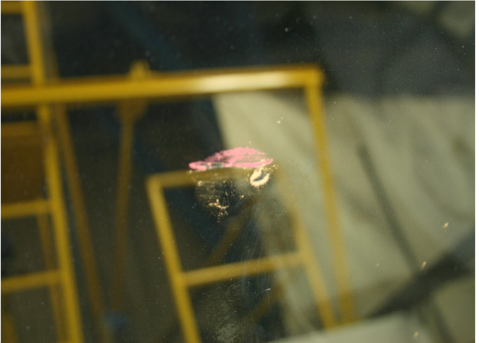
Post-Test Driver Dummy Head Contact (windshield)
