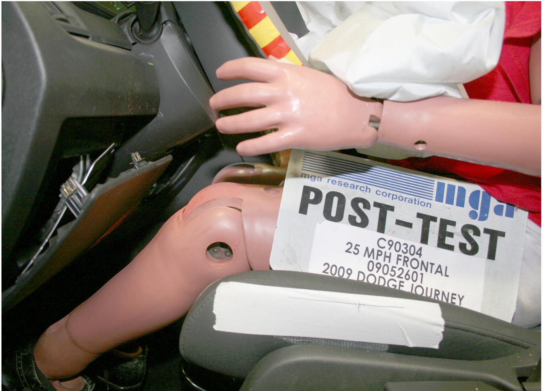
Post-Test Driver Side Knee Bolster View
