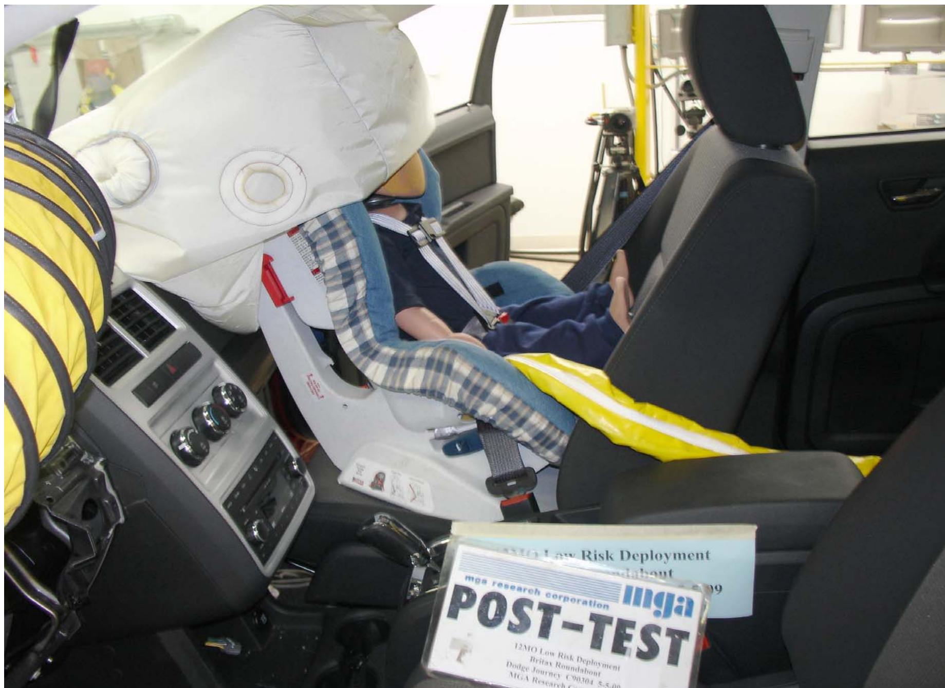
Post-Test 12 Mo Pass. Dummy Left Side View (Britax Roundabout)
