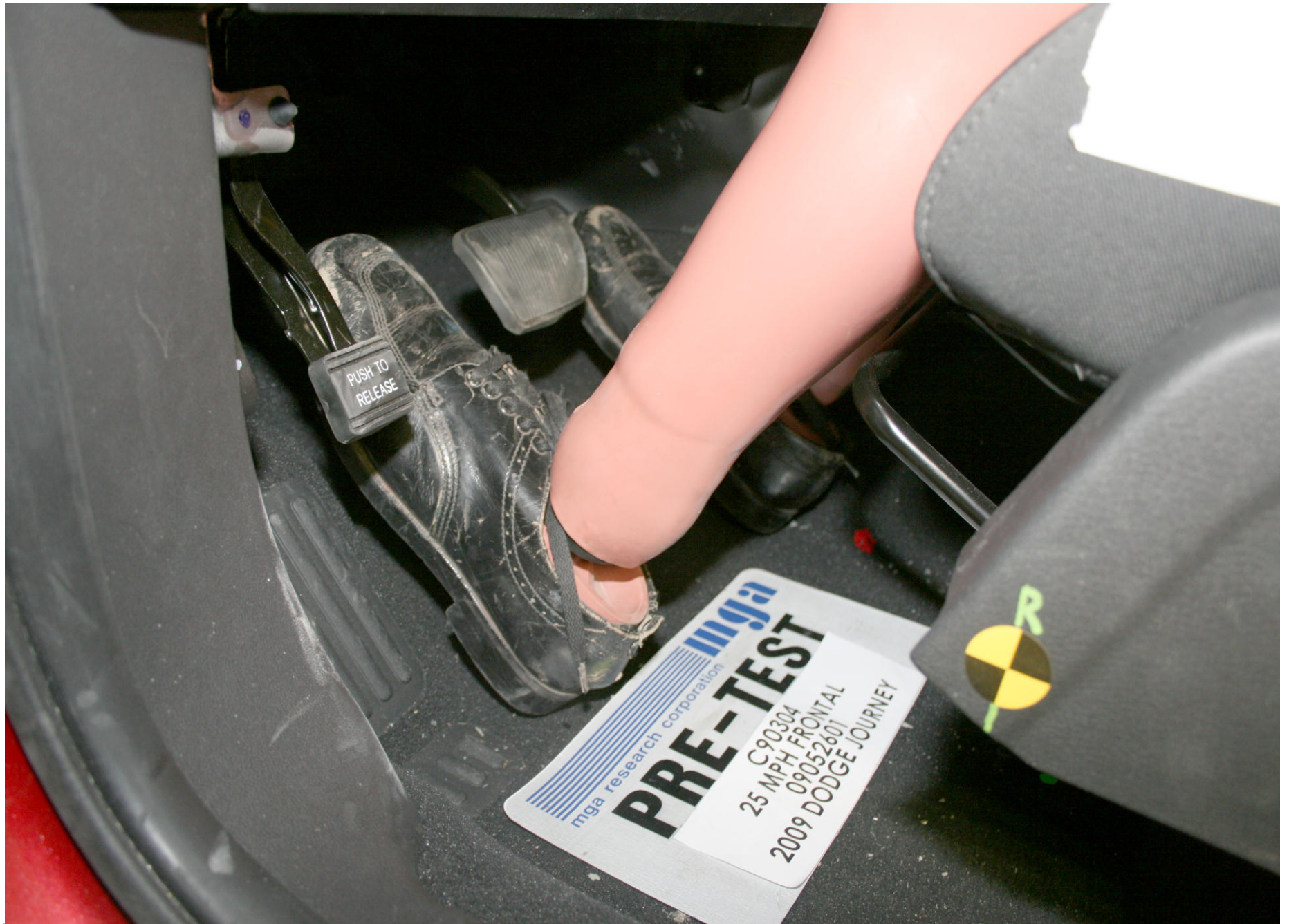
Pre-Test Driver Dummy Feet Position
