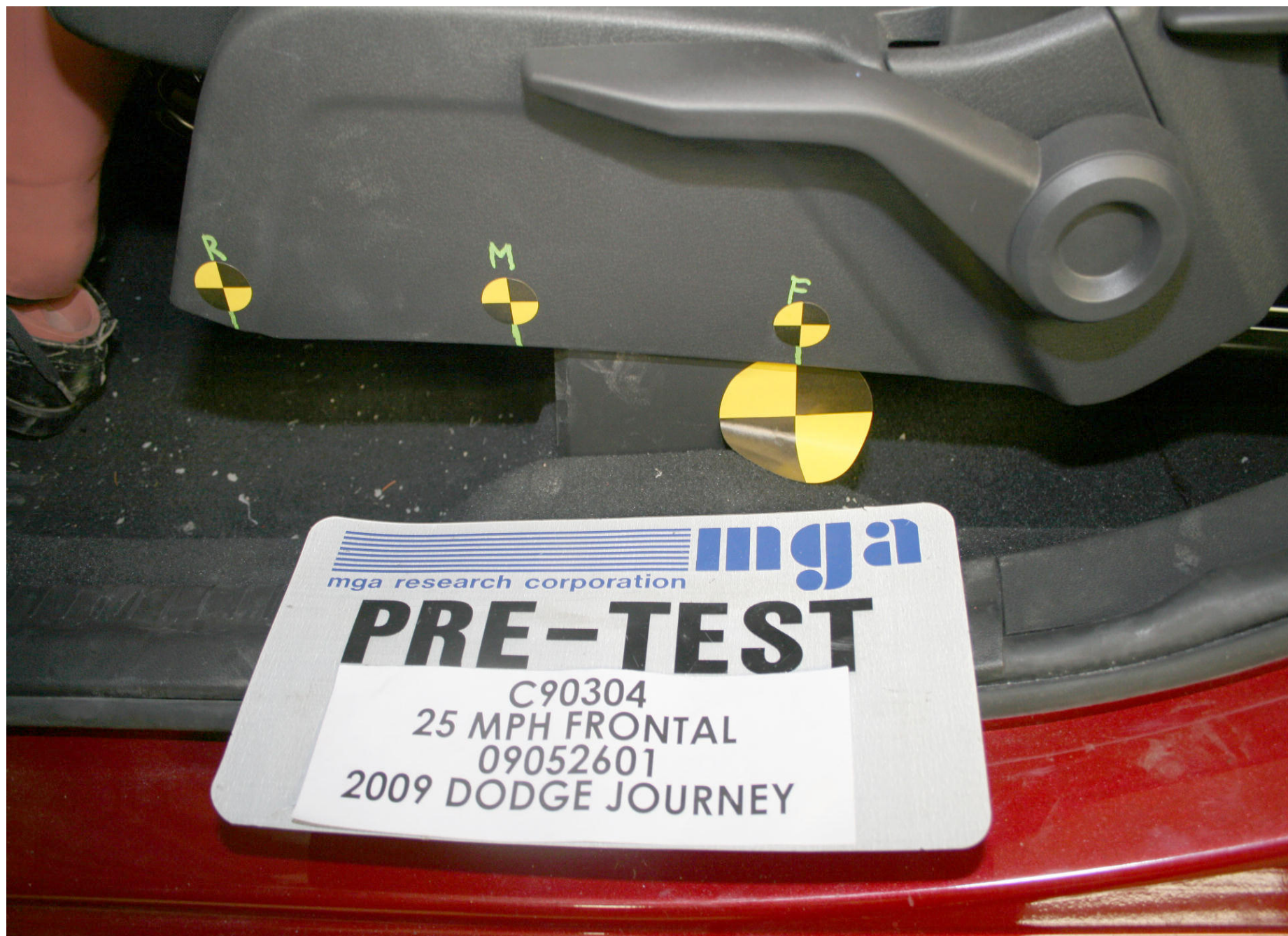
Pre-Test Driver Dummy Seat Position
