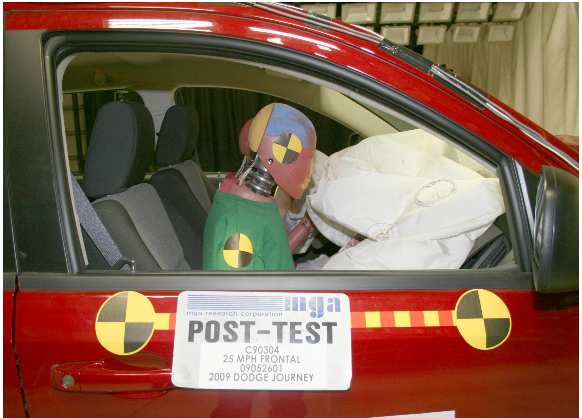
Post-Test Passenger Dummy Position Right Side View
