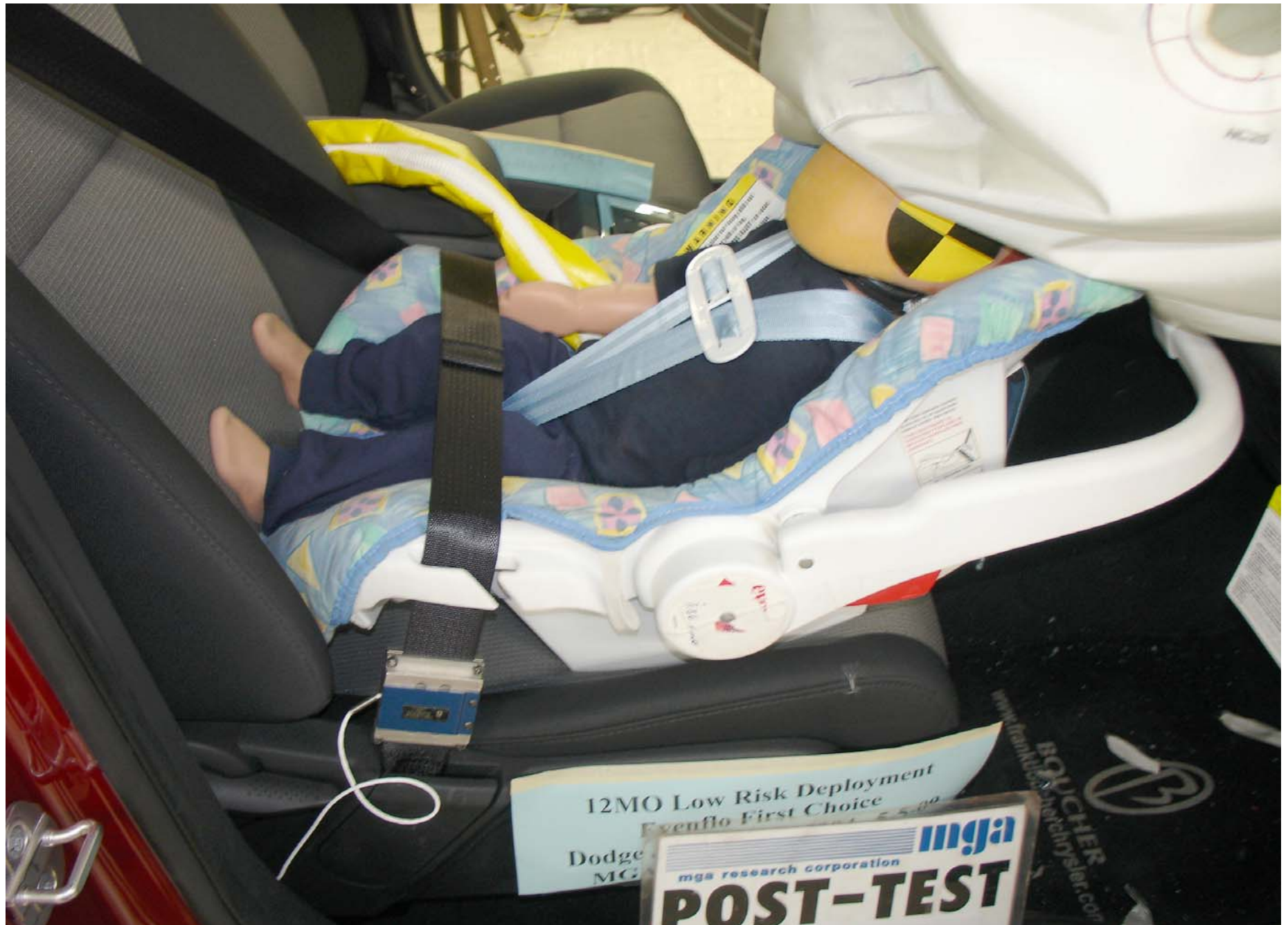
Post-Test 12 Mo Pass. Dummy Right Side View (Evenflo First Choice)
