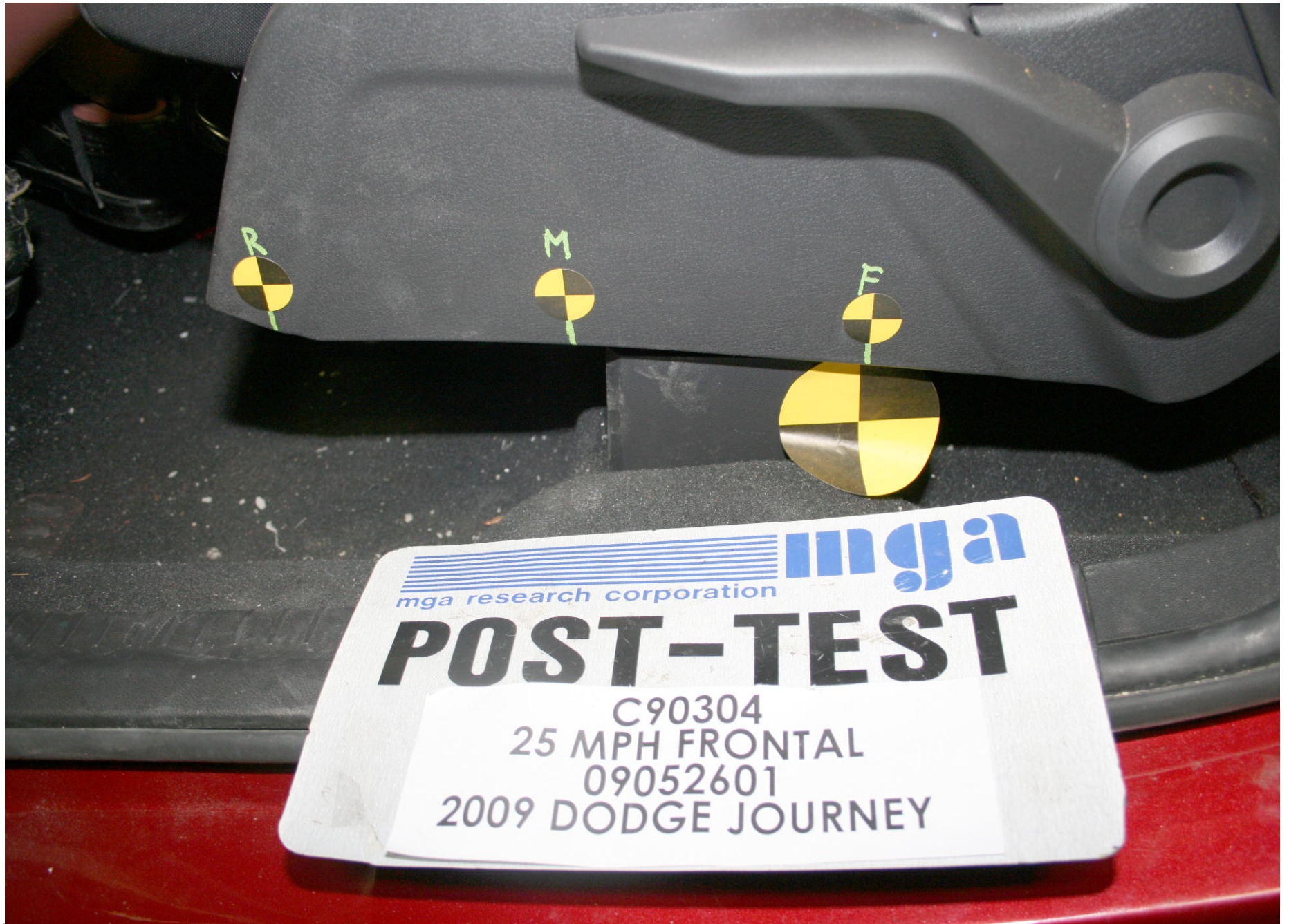
Post-Test Driver Dummy Seat Position
