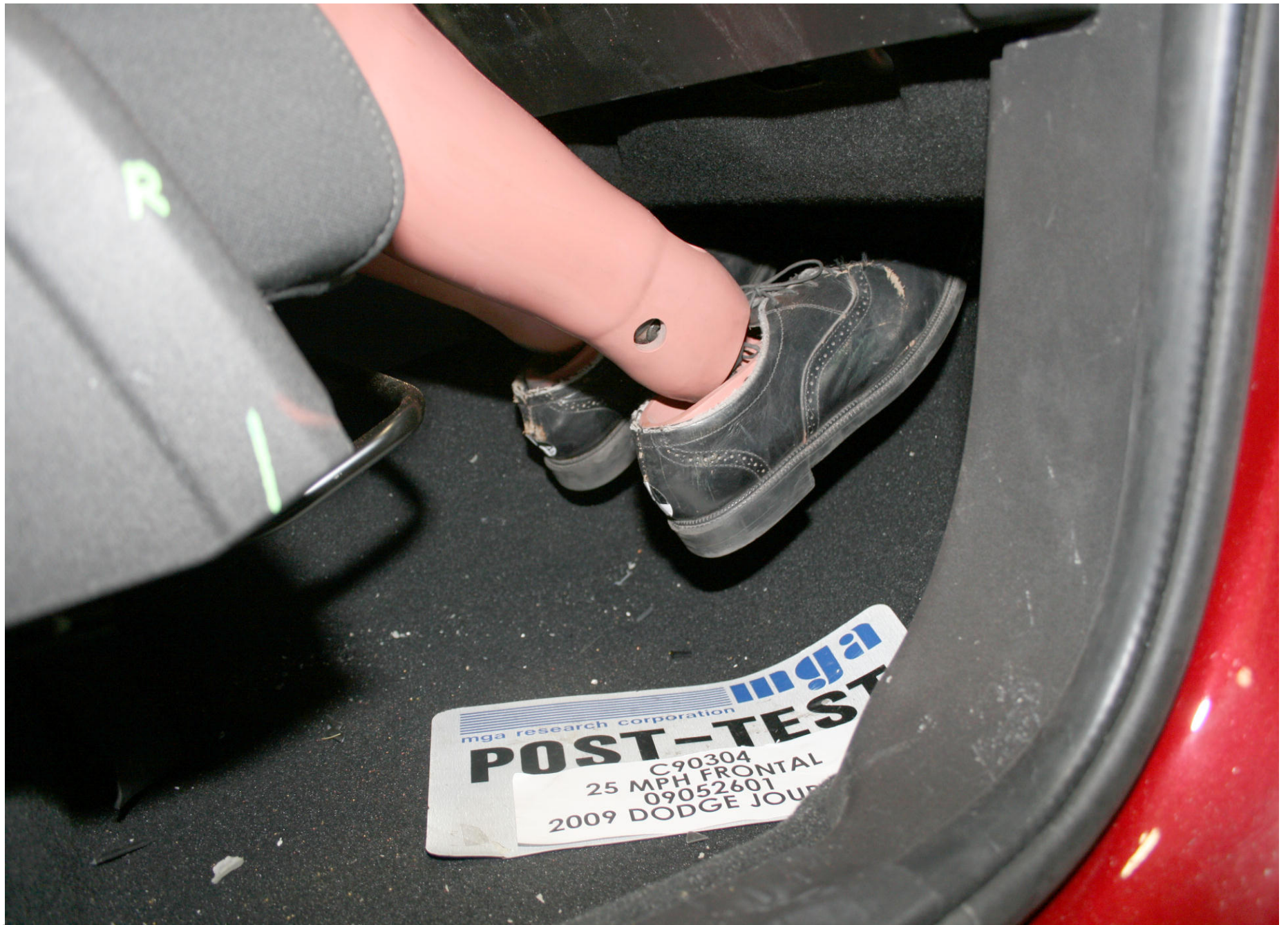
Post-Test Passenger Dummy Feet Position
