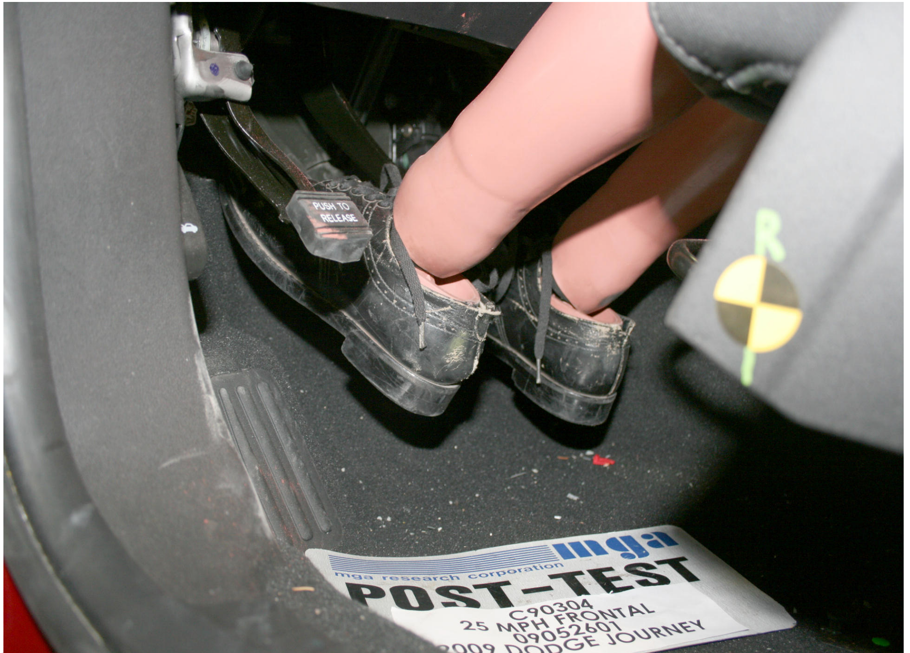
Post-Test Driver Dummy Feet Position
