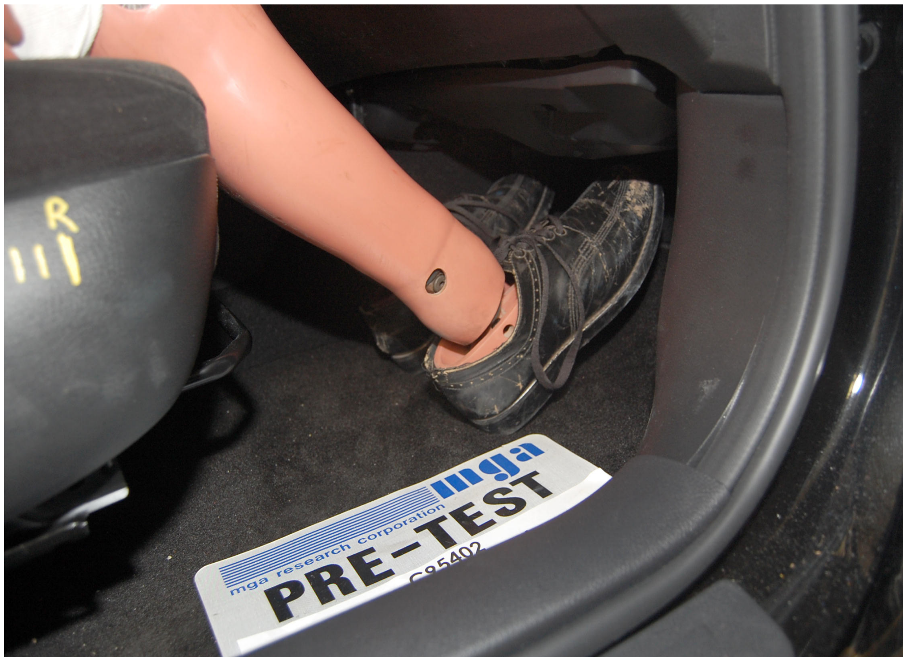
Pre-Test Passenger Dummy Feet Position
