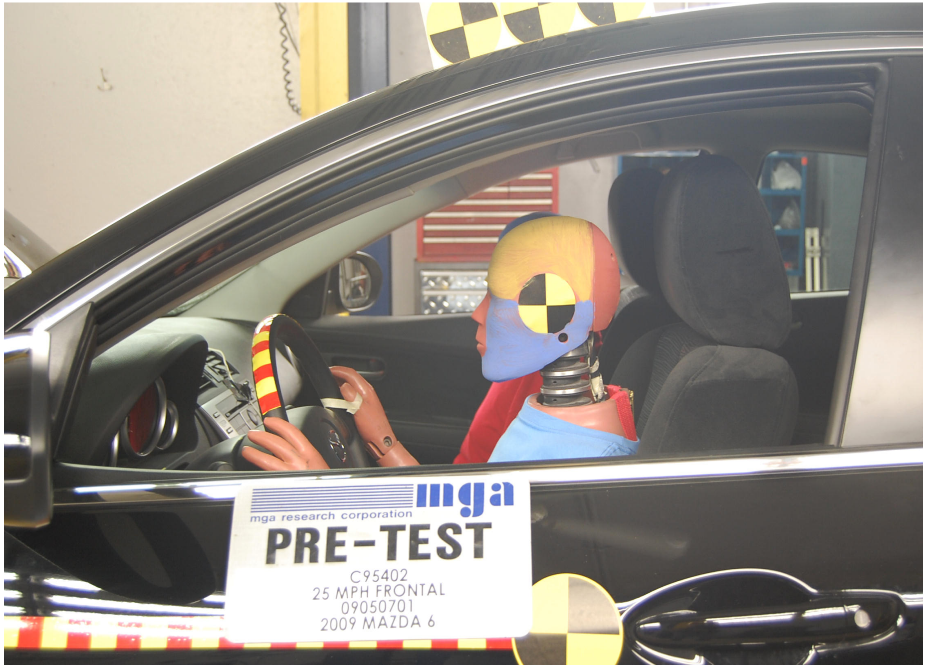
Pre-Test Driver Dummy Position Left Side View
