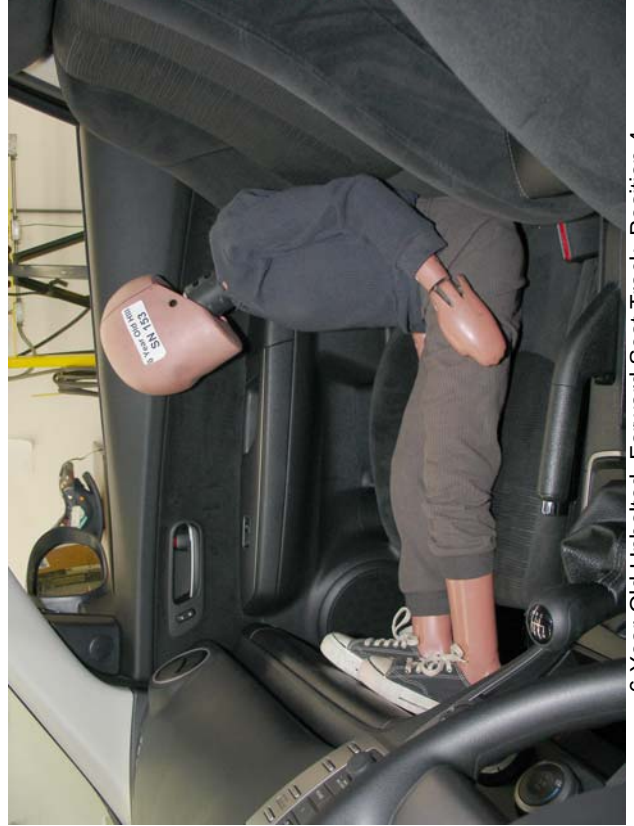
6-Year-Old Unbelted, Forward Seat Track, Position 4
