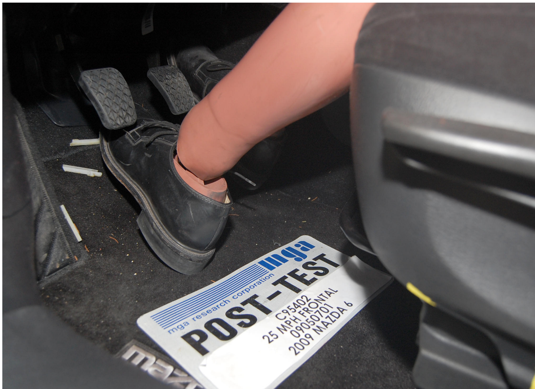
Post-Test Driver Dummy Feet Position
