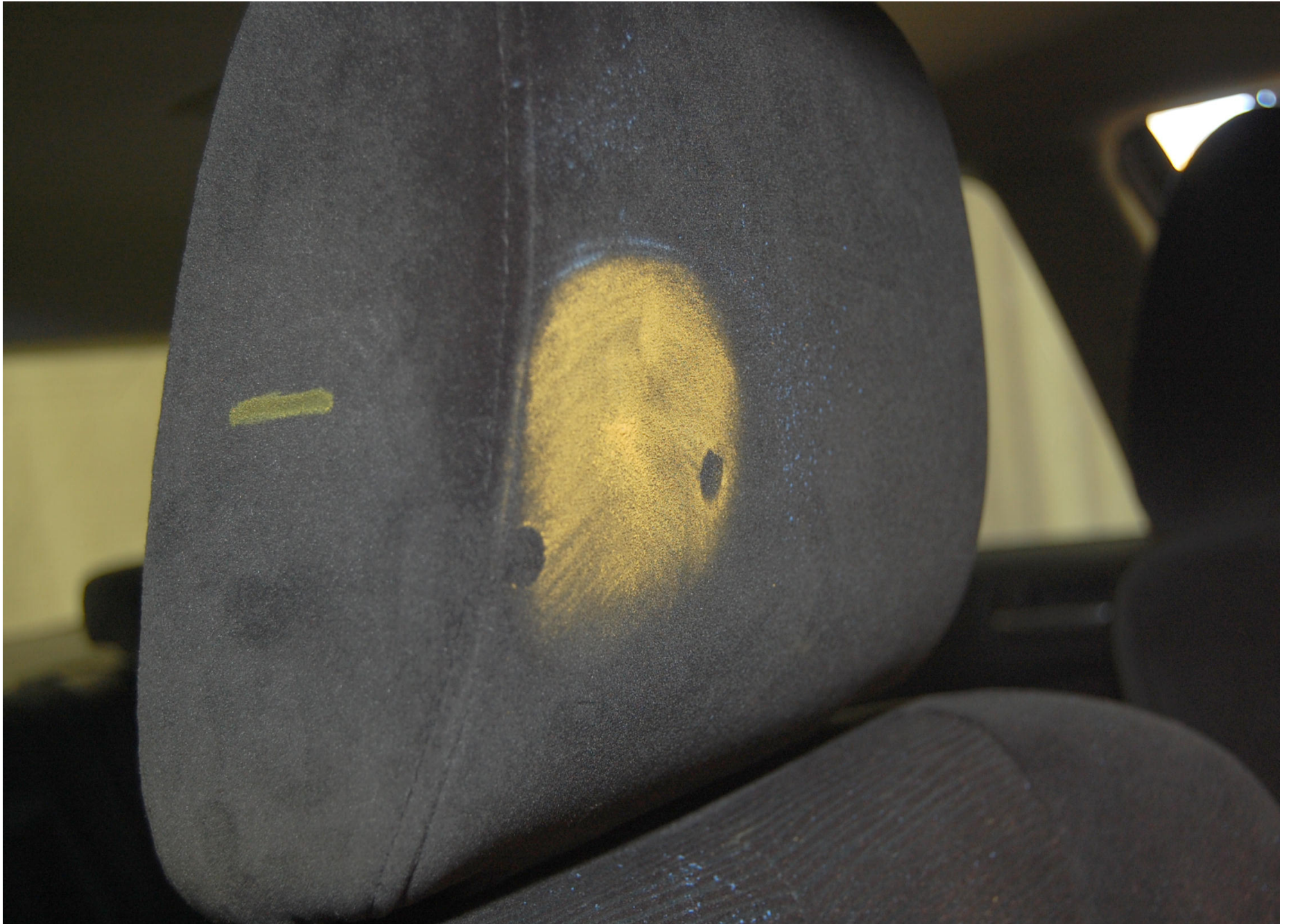
Post-Test Passenger Dummy Head Contact (headrest)
