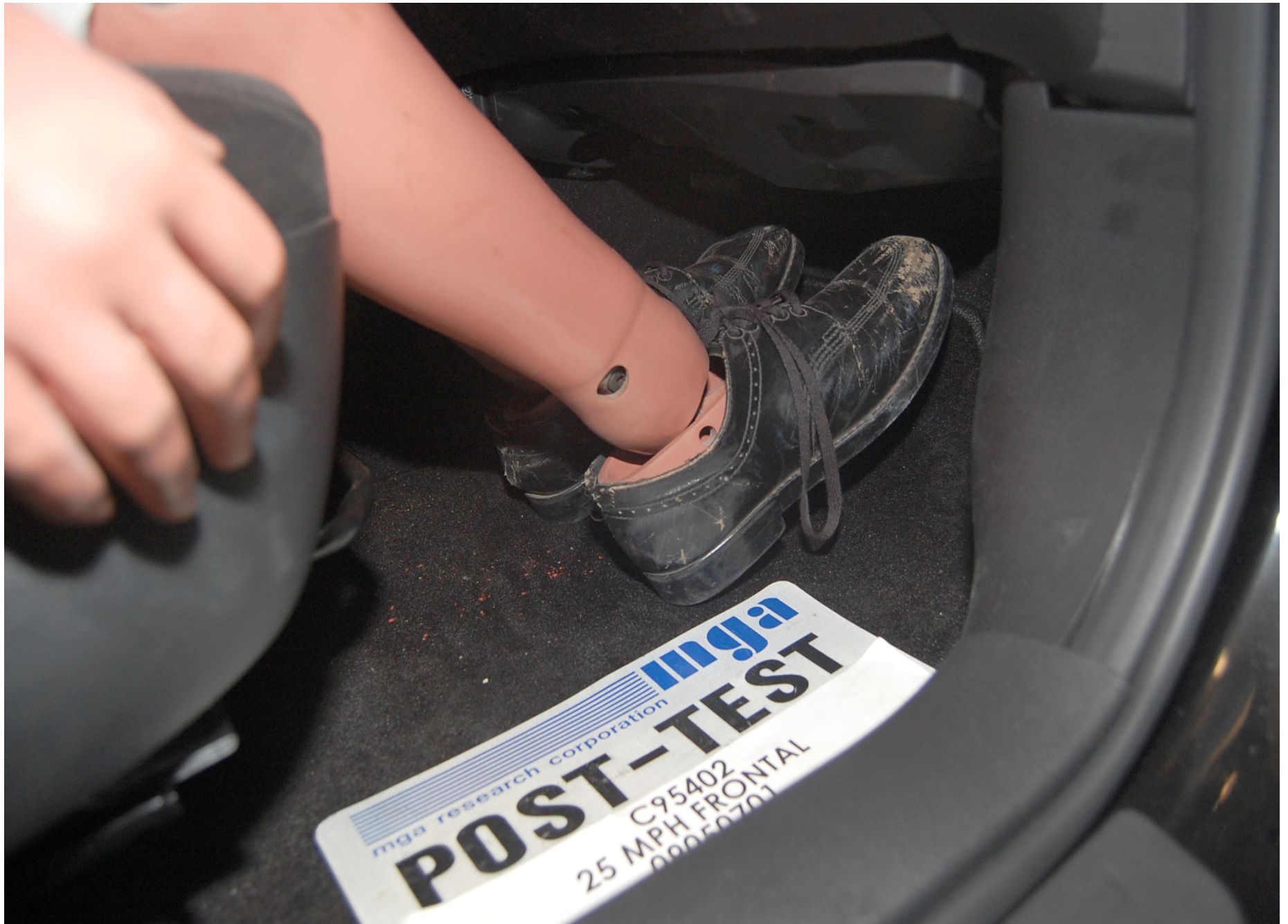
Post-Test Passenger Dummy Feet Position
