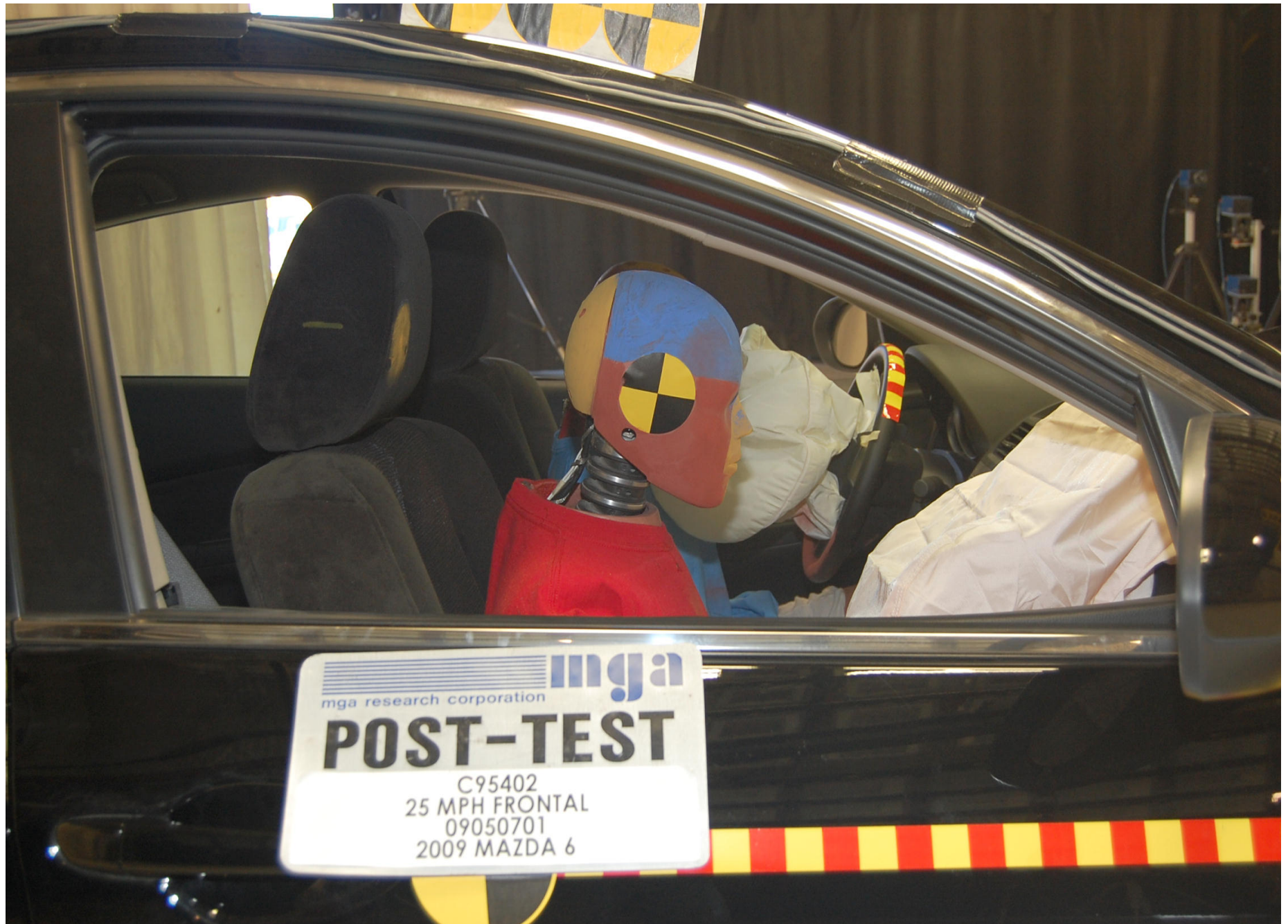
Post-Test Passenger Dummy Position Right Side View
