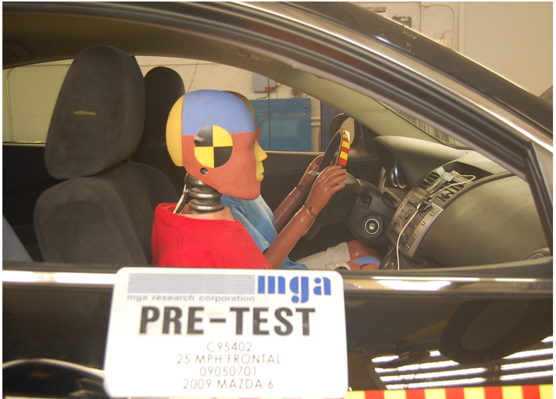
Pre-Test Passenger Dummy Position Right Side View
