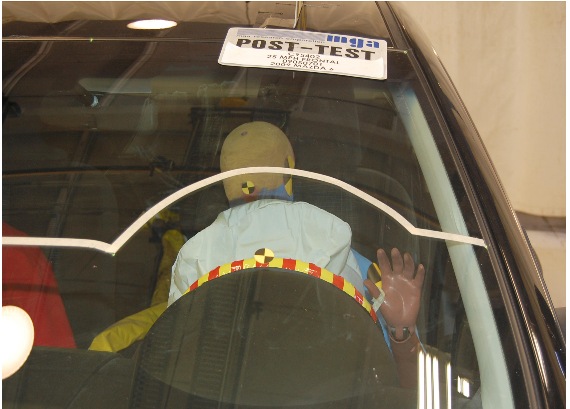
Post-Test Driver Dummy Front View (head position)
