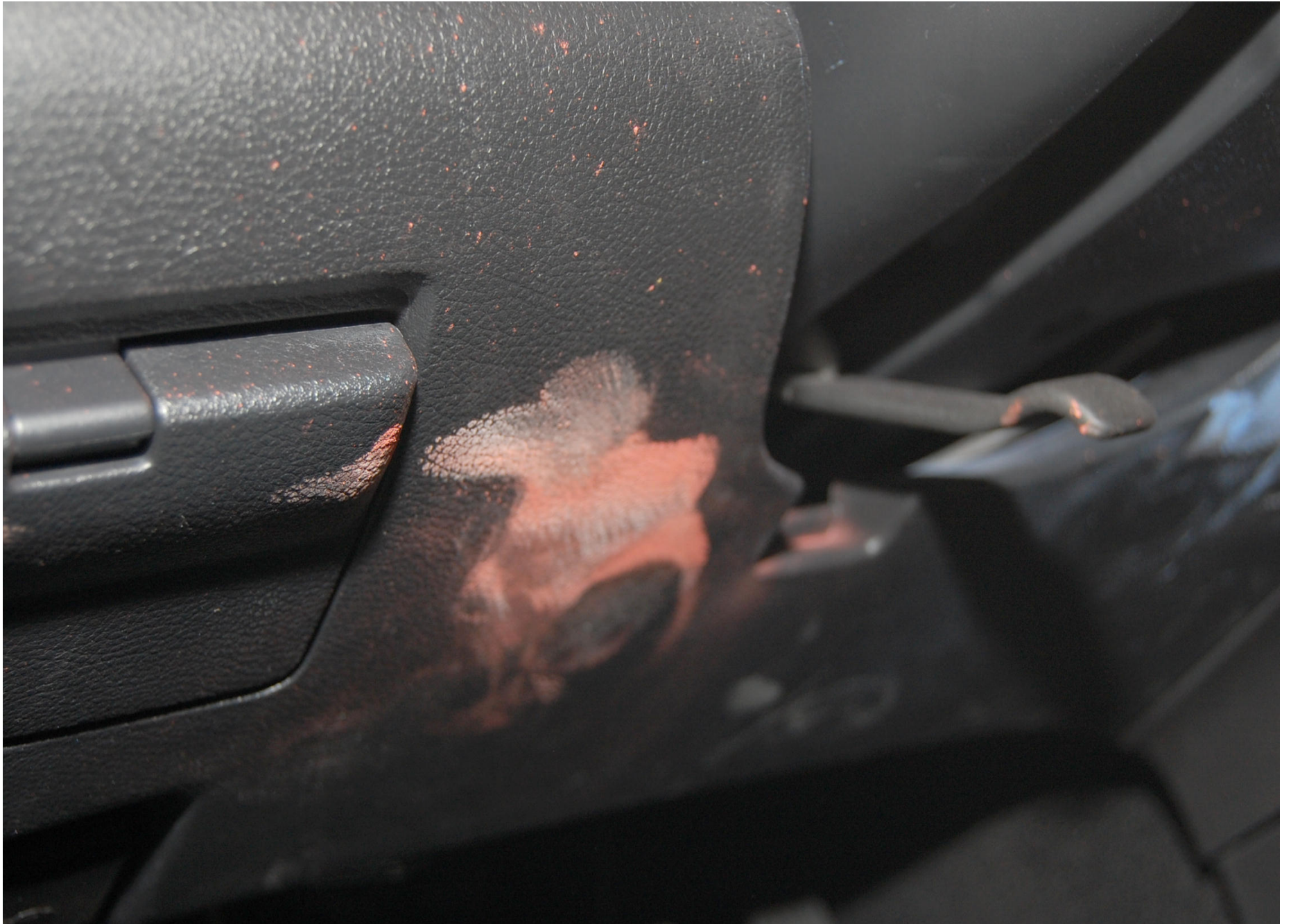
Post-Test Driver Dummy Knee Contact (left side view)
