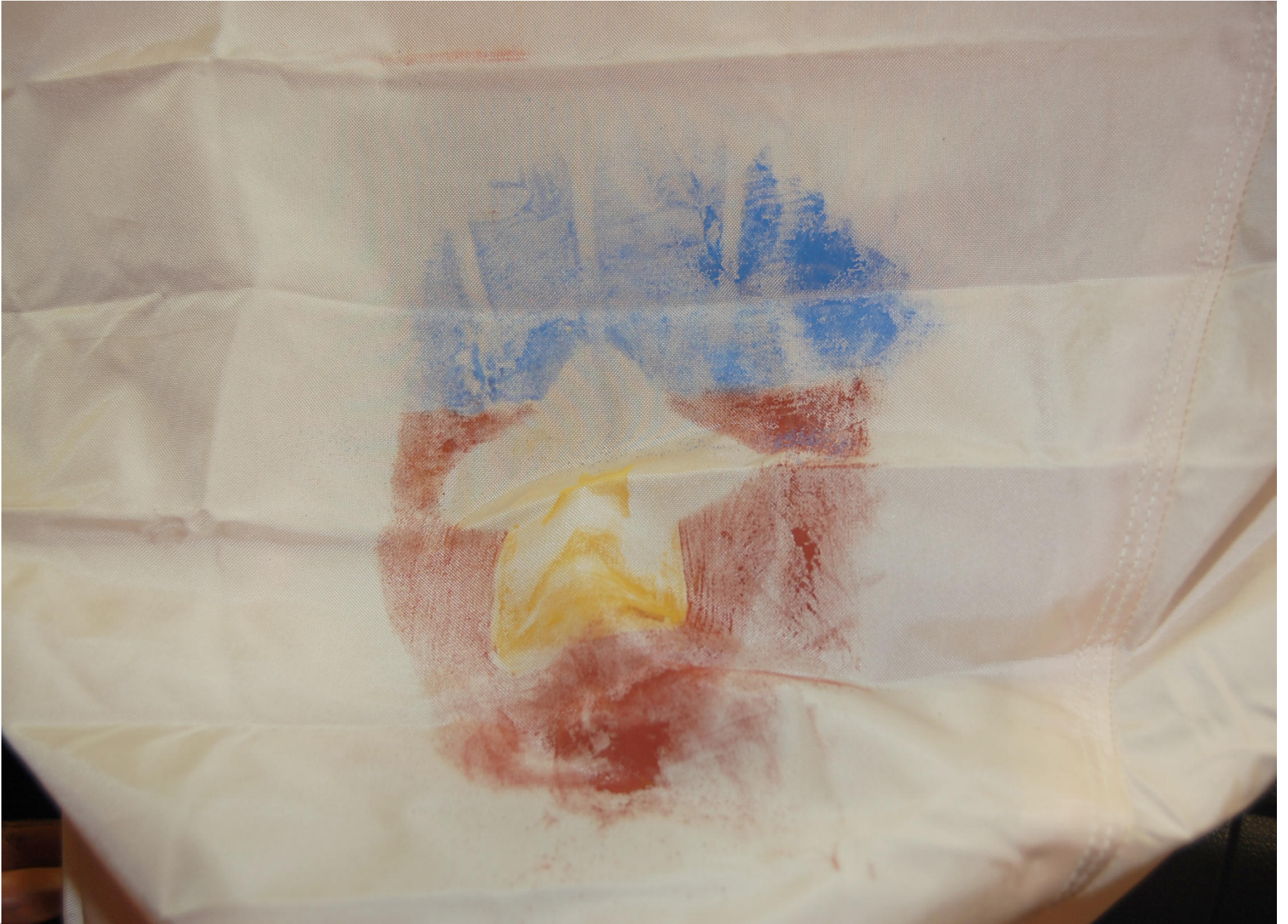
Post-Test Passenger Dummy Airbag Contact
