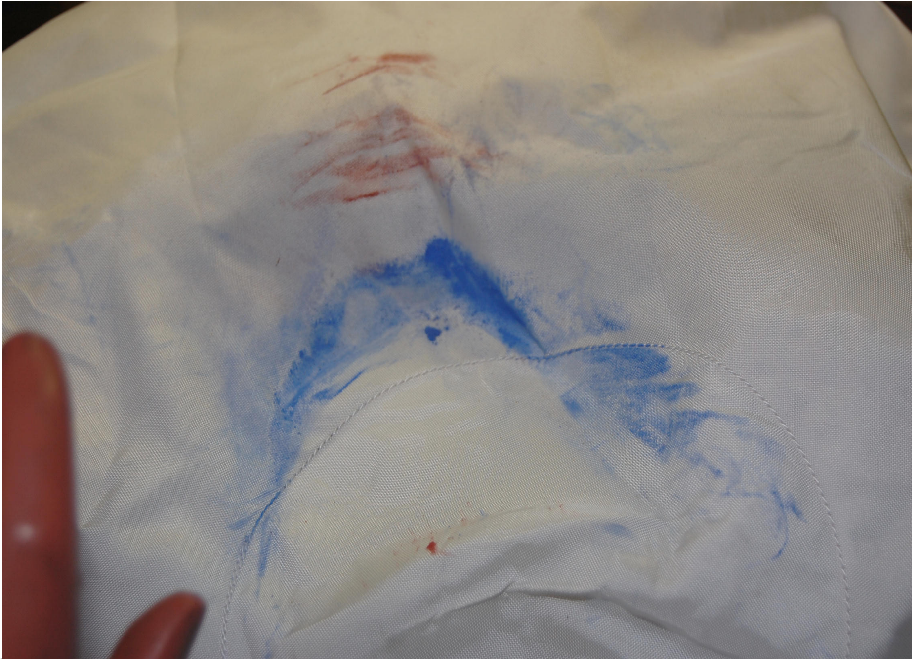
Post-Test Driver Dummy Airbag Contact
