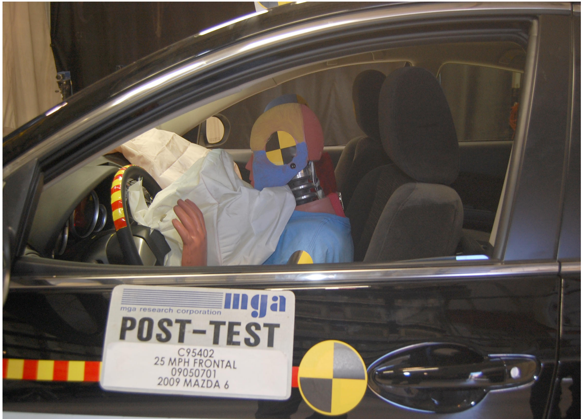
Post-Test Driver Dummy Position Left Side View
