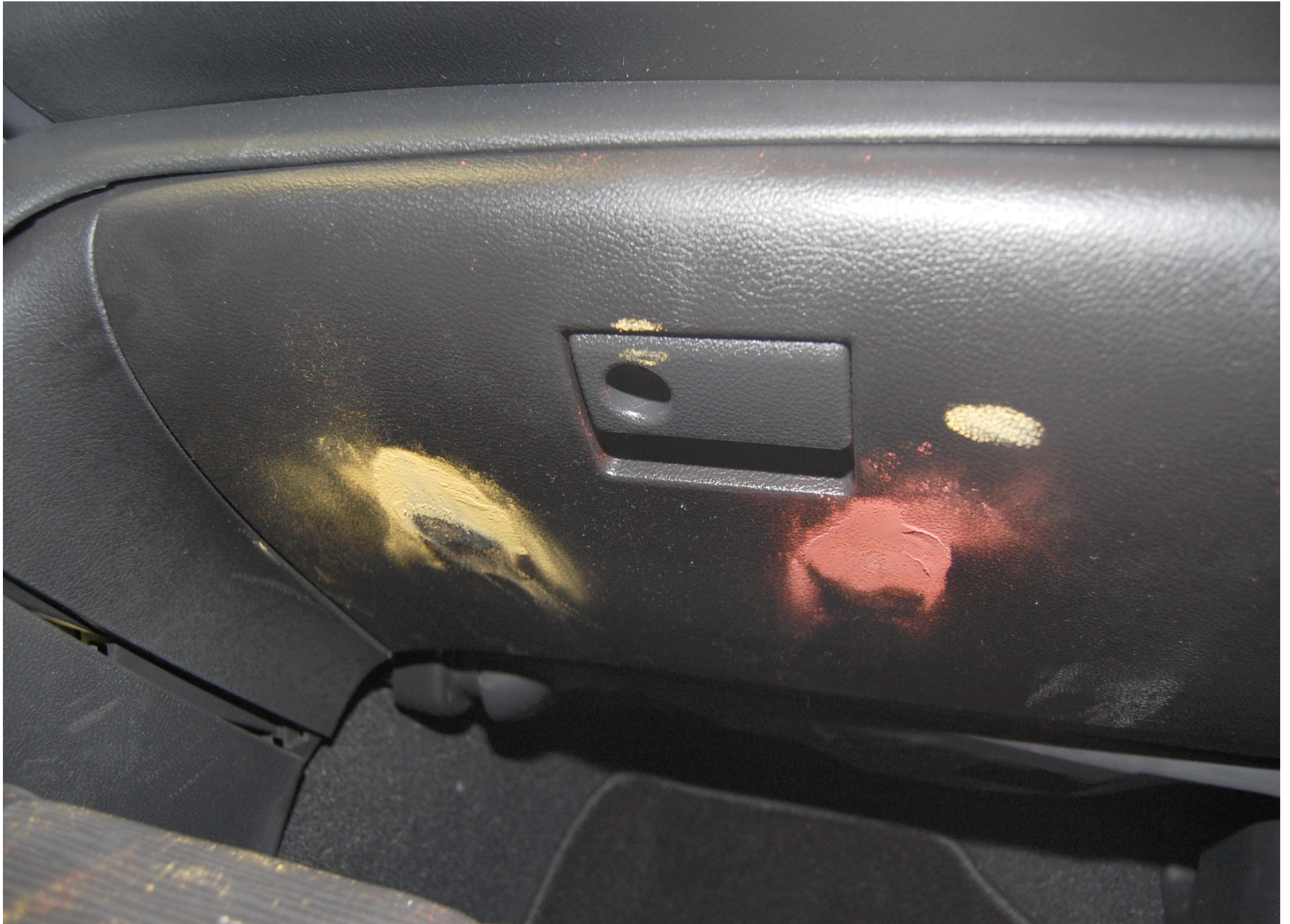
Post-Test Passenger Dummy Knee Contact
