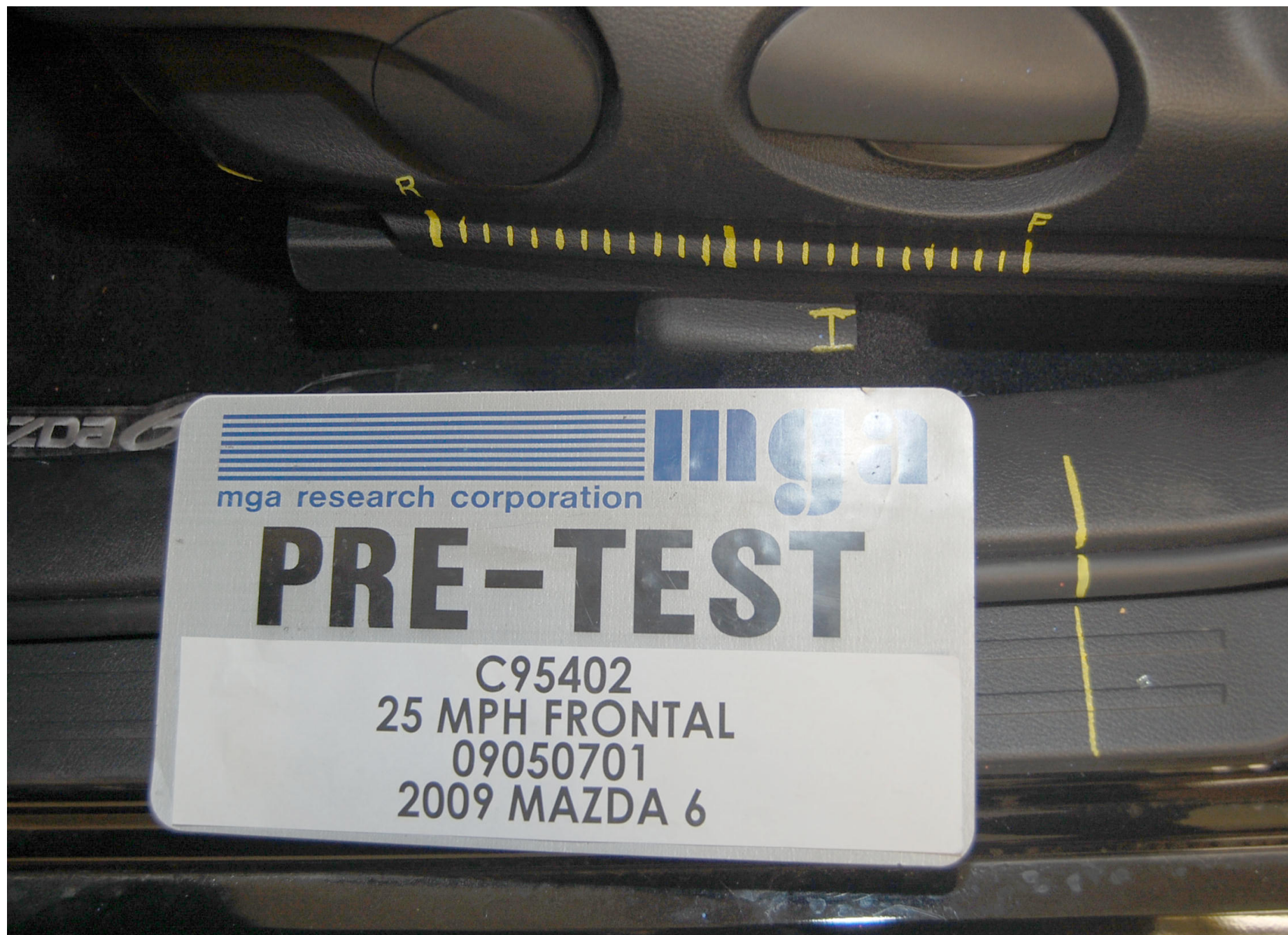
Pre-Test Driver Dummy Seat Position
