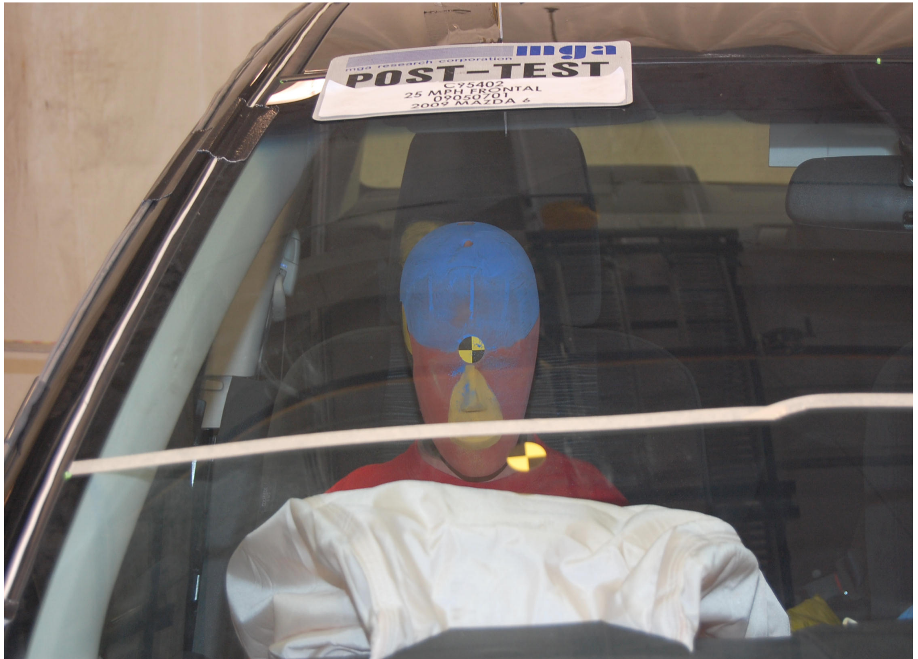
Post-Test Passenger Dummy Front View (head position)
