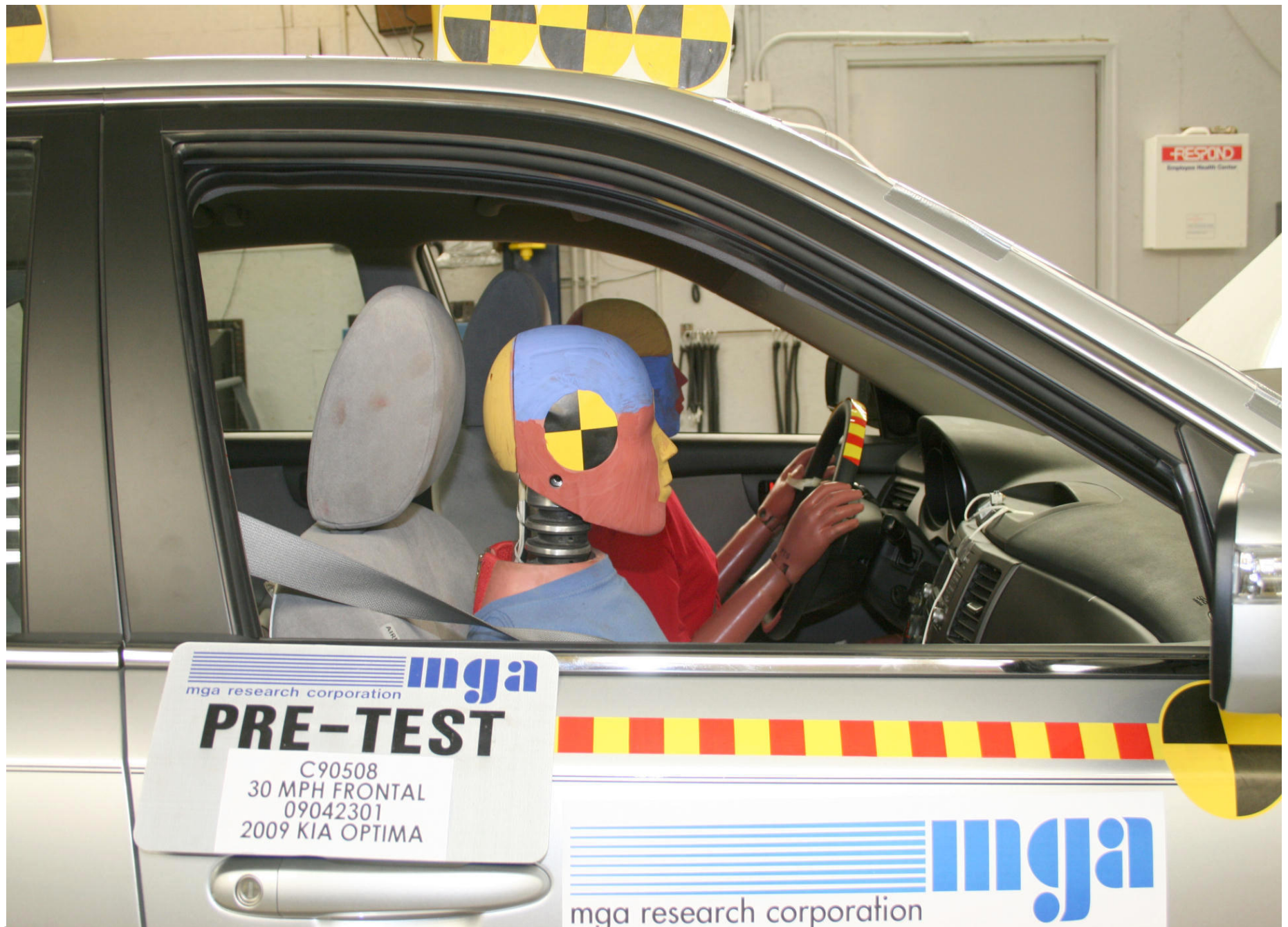
Pre-Test Passenger Dummy Position Right Side View
