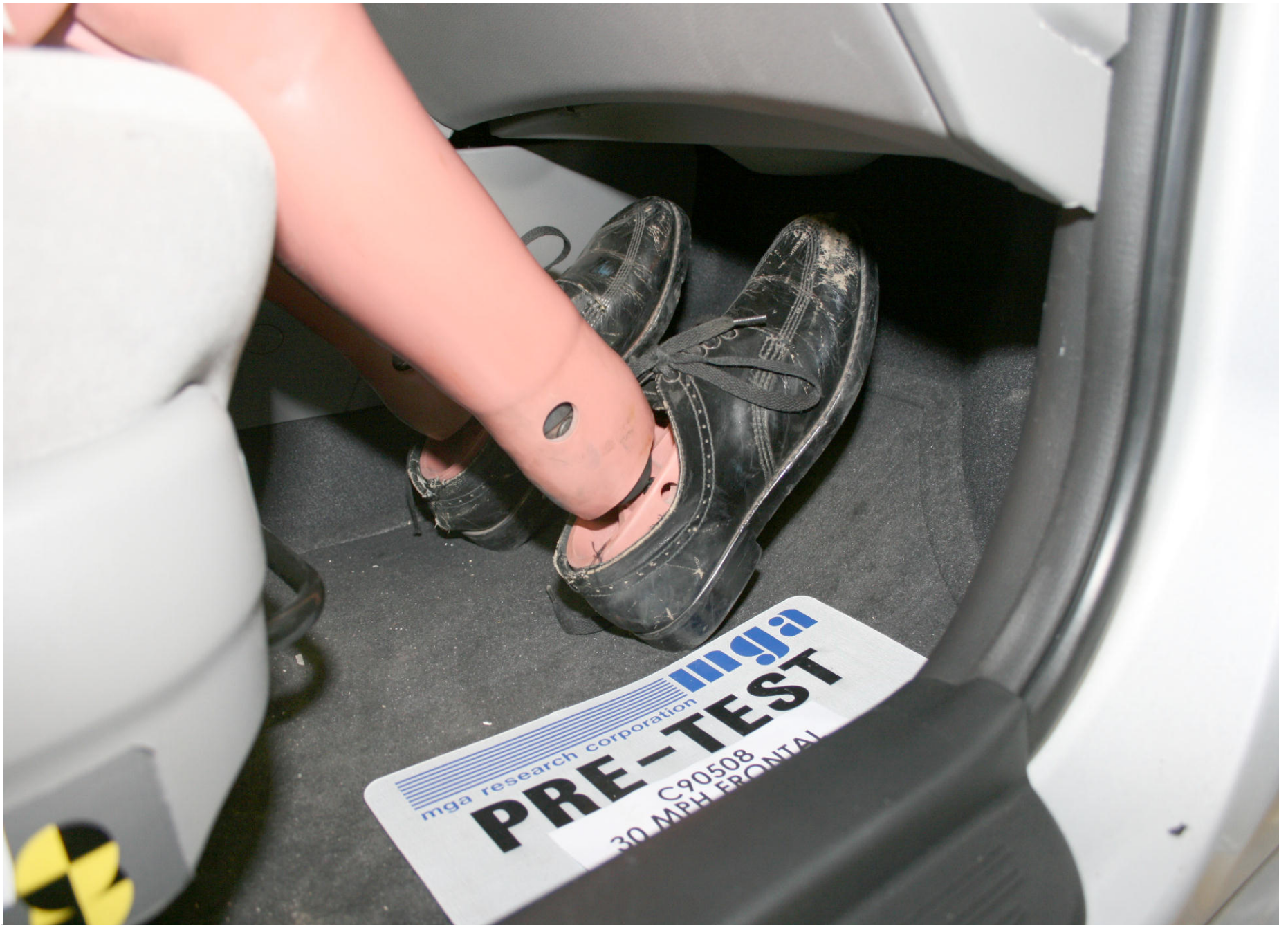
Pre-Test Passenger Dummy Feet Position
