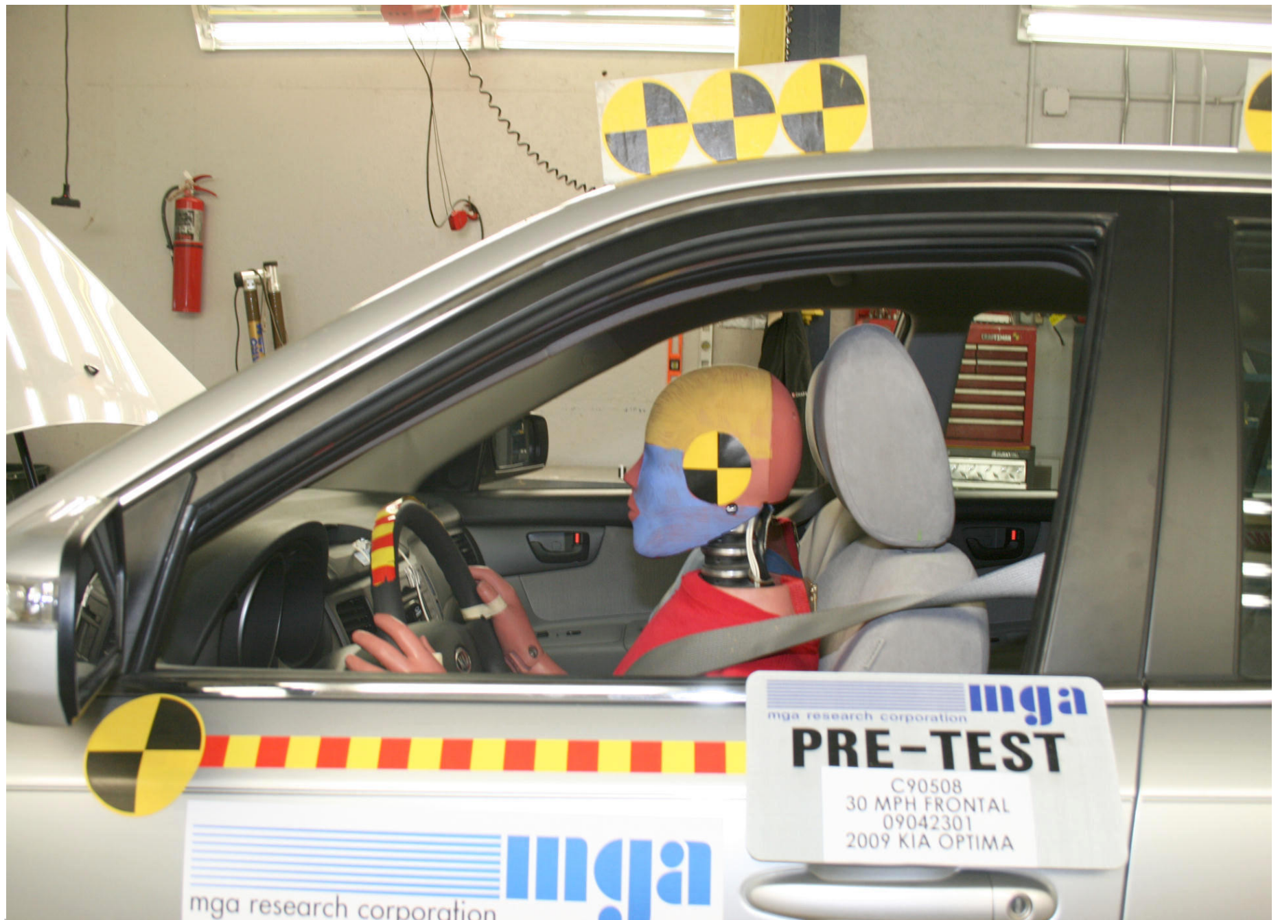
Pre-Test Driver Dummy Position Left Side View
